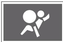
The air bag warning lamp turns on when the START/STOP switch is in the ON status, and it turns off when there is no abnormality in the air bag system.
