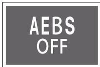
The AEBS OFF indicator turns on when the START/STOP switch is in the ON status and it turns off approximately 4 seconds later.
