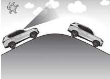
On an uphill road or a downhill road, a vehicle on the same lane cannot be detected and the AEBS performance is lowered so that unnecessary warning or braking is applied or the system may not operate.
