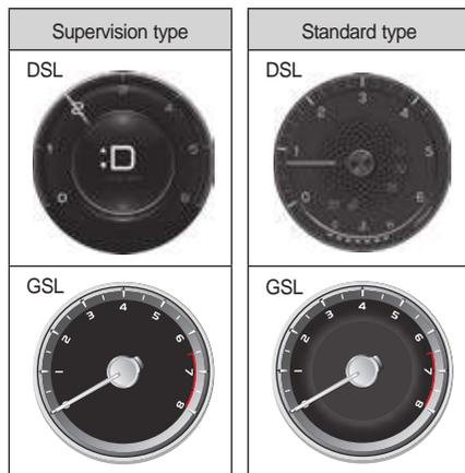
It indicates the revolutions of the engine per minute. Multiplying the number pointed to by the needle by 1,000 is the current engine RPM.
