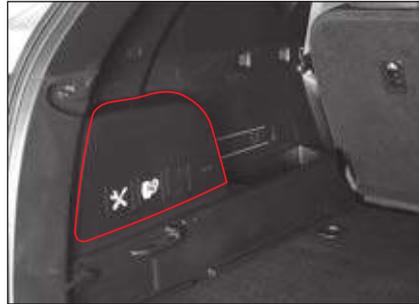
The service kit for tire repair is stored in the storage box at the rear left side of the luggage compartment with the OVM tools.
