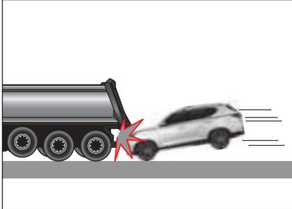
Generally, most drivers apply a sudden brake when an accident occurs, so the front part of the vehicle becomes lower. Therefore, the vehicle often moves beneath the opposing vehicle in the event of an accident against a tall vehicle such as a bus or a truck. In such case, the air bag may not inflate.
