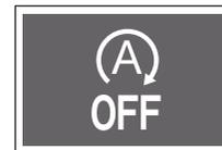
When you press the ISG ON/OFF switch, the indicator is lit. Press the switch again to turn off the indicator.
