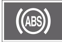
This warning light turns on when the START/STOP switch is in the ON status and it turns off if the system is normal.
