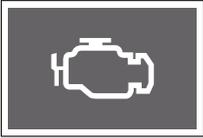
The engine check indicator turns on when the START/STOP switch is in the ON status and turns off the engine is started.
