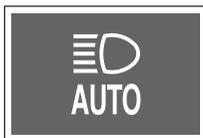
The HBA indicator turns on when the START/STOP switch is in the ON status and turns off approximately 4 seconds later.
