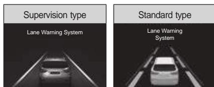
If both lanes are recognized with the vehicle speed of 60 km/h or higher, the lanes are displayed in white.
