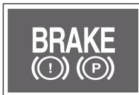
The brake warning light turns on when the START/STOP switch is in the ON status and turns off approximately 4 seconds later.
