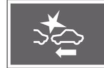
The AEBS warning light turns on when the START/STOP switch is in the ON status and turns off approximately 4 seconds later.
