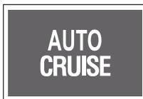
The auto cruise indicator turns on when the cruise control is activated and it turns off when the cruise control is deactivated.
