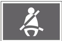
If the driver seat and front passenger seat occupants do not fasten the seat belt, the seat belt warning light blinks along with a warning buzzer.
