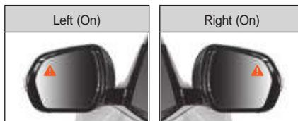
When a vehicle in the rear and side warning area of the vehicle is detected, the yellow warning light indicator on the outside rearview mirror turns on.
