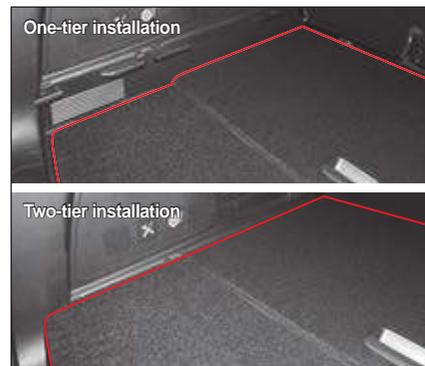
If the luggage board is installed at two tier, the height of the floor can be adjusted evenly when folding the rear seats (1st row, 2nd row).
