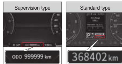
The total mileage of the vehicle is displayed in kilometers. The maximum mileage to be displayed is 999999 km.
