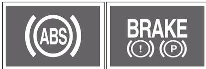
If the EBD system is abnormal, the ABS warning light and the brake warning light turn on at the same time.
