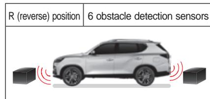
When the gear shift lever is placed in the R (reverse) position, 2 front obstacle detection sensors and 4 rear obstacle detection sensors are activated at the same time.
