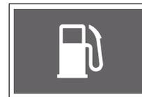
If the remaining fuel level is insufficient, the low fuel level warning light turns on. However, the time for the warning light to turn on may vary depending on the vehicle status or the degree of slope.
