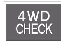
The 4WD CHECK warning indicator turns on if the 4WD switch unit is abnormal.
