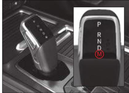
This is the position where the driver can shift the gear manually.
