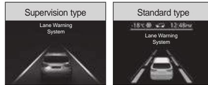
When detecting the lanes according to the vehicle condition, the detected lane is displayed in white and alarm can be issued at the detected lane.
