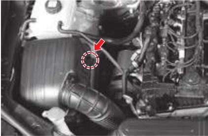
If the vehicle is operated in very dusty or sandy areas, replace more often than at the usual recommended intervals. If it is dirty, shake the element to remove dust. Clean the inside of the air cleaner housing and cover with a damp cloth.
