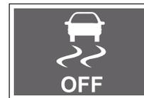
When you deactivate the ESP by pressing and holding down the ESP OFF switch (for 3 seconds or more), the indicator turns on.
