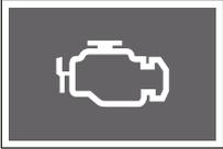
The engine check indicator turns on when various sensors (including automatic transmission) and equipment related to the engine control are abnormal.
