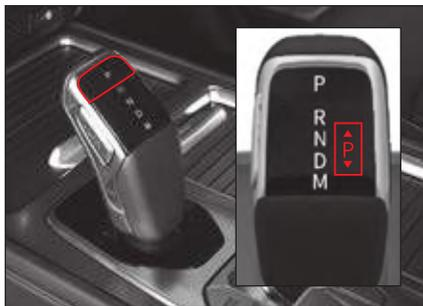
Select this position to park, start the engine, warm-up, and stop the vehicle for a long time.
