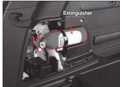
The extinguisher is stored in the storage box at the rear left side of the luggage compartment with the OVM tools.
