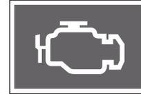
The engine check indicator on the instrument cluster turns on when the fuel system of the engine or main electrical systems are not working properly. At this time, the driving power of the engine may decrease or the engine may turn off.
