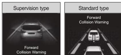
If the distance to the front vehicle is so close that a collision can occur or the front vehicle disappears from the front view due to lane change, etc. while the intelligent cruise control is activated, the message is displayed on the instrument cluster.
