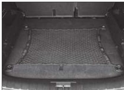
Any loose objects can be stowed securely using the luggage net. Hook the net up to the luggage compartment.
