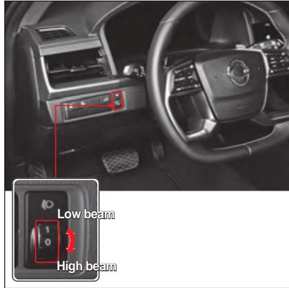
The front and rear slope of the vehicle may vary depending on the number of occupants, weight and center of gravity of luggage.
