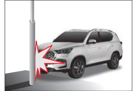
In the event of a collision with a narrow object such as a street light, utility pole or tree, the degree of impact applied to the sensor may not be enough, so the air bag may not inflate.
