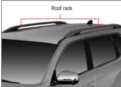
The luggage can be loaded onto the top of the vehicle roof using the roof rack.
