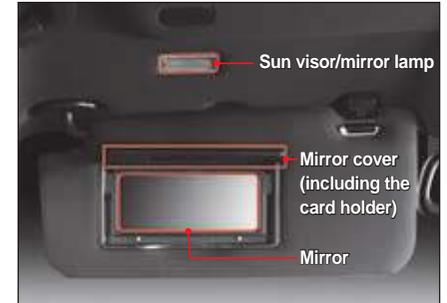
When you pull the sun visor down and open the mirror cover, the lamp turns on.
