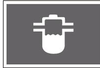
If water in the fuel filter exceeds a prescribed level, the water separator warning light turns on and the driving force of the engine decreases in addition to the warning buzzer.
