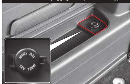
The power socket (12 V/10 A, 120 W) is provided in the vehicle to enable the use of a separate electrical device.
