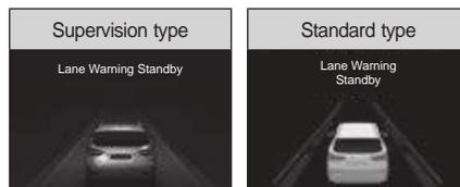
If the vehicle speed is less than 60 km/h or both lanes are not recognized, the shaded lanes are displayed.
