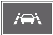
This indicator light up on the instrument cluster when the LKAS is activated.
