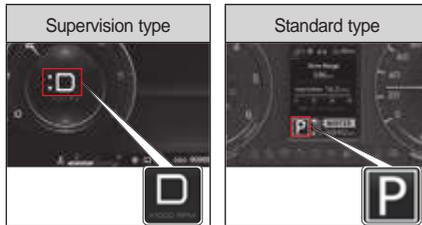
It displays the current position (P, R, N, D) of the gear shift lever and the gear stage (1~8stages) in the M (manual) mode.
