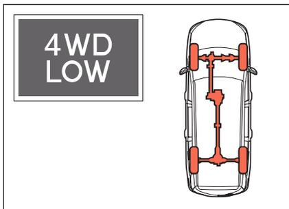
Use the 4WD LOW (4H) mode when the maximum traction power is necessary.
