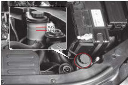
Check the fluid level on a level ground with the engine turned off. The fluid level should be between the MIN and MAX marks on the reservoir cap gauge. If it drops to or below the MIN mark, refill the reservoir with the specified fluid. Only use the specified fluid. The difference between the MIN and MAX marks shows fluctuations of the steering fluid between when it is hot and when it is cold.
