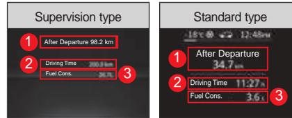
The mileage traveled after the engine is started (km), departure time (hh:mm), driving time (hh:mm) and fuel consumption (L) are displayed.
