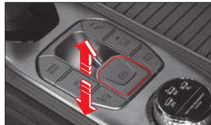
Operate the EPB (Electric Parking Brake) switch and check the operating sound and operation status.
