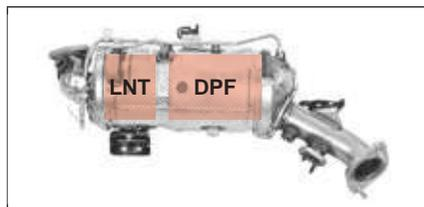
This vehicle is equipped with the Diesel Oxidation Catalyst (DOC) for EU4 emission reduction.
