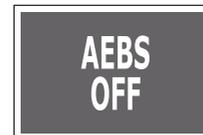
When the AEBS system and the ESP function are deactivated, the AEBS OFF indicator on the instrument cluster turns on.
