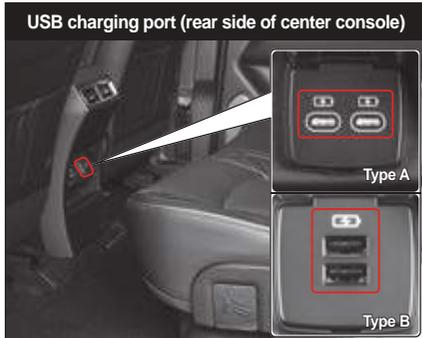
You can charge devices such as a smartphone or tablet PC using the USB charging port.
