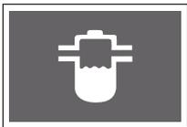
The water separator warning light turns on when the START/STOP switch is in the ON status and it turns off approximately 4 seconds later.
