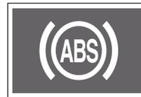
The ABS warning light turns on when the START/STOP switch is in the ON status and turns off approximately 4 seconds later.
