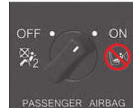
The front passenger air bag is disabled (not inflatable) when placing the passenger air bag ON/OFF switch to "OFF" position. This switch is located on the right side of the instrument panel, and you can see it when opening the front passenger door. Press and turn this switch to operate.
