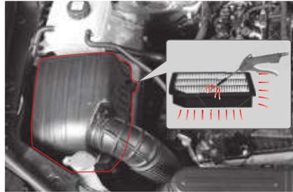
Blow the compressed air through the element in the opposite direction to normal air flow to clean the element as shown above.
