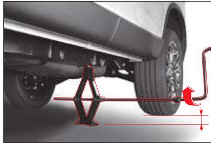
4 Combine the jack, jack extension and the wheel nut wrench as shown in the figure. Raise up the vehicle by rotating the combined wrench clockwise until the tire is off from the ground about 3 cm.
