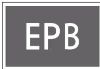
The Electronic Parking Brake (EPB) warning light turns on when the START/STOP switch is in the ON status and turns off approximately 4 seconds later.
