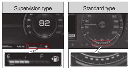
It displays the remaining fuel level when the START/STOP switch is in the ON status or the engine is running.
