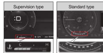
It indicates the temperature of the engine coolant.
