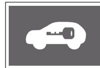
If the smart key system is abnormal or the smart key(transponder) authentication fails, the warning light blinks.
