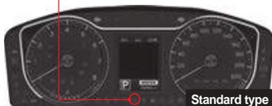
If the tire pressure or the tire pressure monitoring system is abnormal, the global warning light blinks or comes on.
