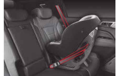
Secure the child restraint with a seat belt as shown in the figure.
