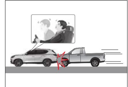
In the event of a rear end collision by another vehicle, the body of the occupants move backwards, so the air bag cannot provide enough protection even if it inflates. In such case, the air bag may not inflate.
