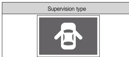
The door open warning light turns on when a door or the tailgate is opened or not closed completely.
