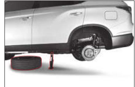
6 Take the wheel off and place the wheel under the vehicle body. This helps to minimize any danger if the jack slip off position.
