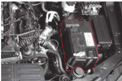
When the battery charge warning light (
