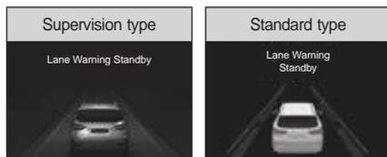
The lanes are shaded when the LDWS is turned ON but the vehicle is driven at a low speed of less than 60 km/h or both lanes are not detected.
