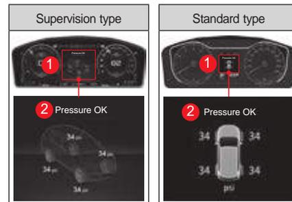
By selecting TPMS status from the main menu (1) of the instrument cluster, you can check all tire pressures from the display (2) of the instrument cluster.
