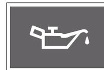
The engine oil pressure warning light turns on when the START/STOP switch is in the ON status and it turns off when the engine is started.
