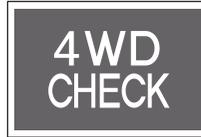
The 4WD CHECK warning indicator turns on when the START/STOP switch is in the ON status and turns off approximately 4 seconds later.
