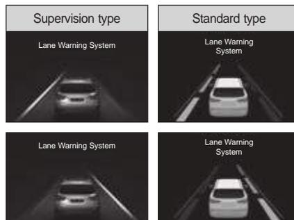
If only one lane is recognized with the vehicle speed of 60 km/h or higher, only the recognized lane is displayed in white.
