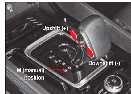
You can shift the gear by pushing or pulling the manual gear shift lever from the M (manual) position.
