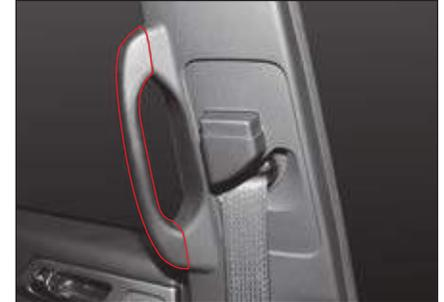
The grip handle is installed at the front of side of rear seats for convenience at the time of getting in and out of the vehicle.
