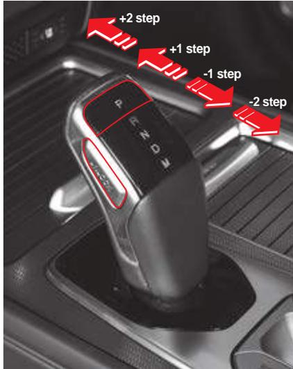
The electronic shift lever can be moved at + 2 step and - 2 step, after which it is always aligned to the central position.
