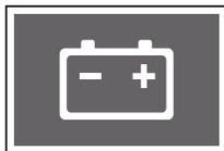
The charge warning light turns on when the vehicle battery is depleted or the charging system is abnormal.
