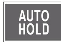
When you press the AUTO HOLD button, the AUTO HOLD system enters the ready mode and the white AUTO HOLD indicator on the instrument cluster turns on.
