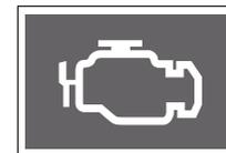
Regeneration may not be performed due to several operating conditions. And in this case, the engine CHECK indicator flashes. This flashing function is to inform the driver to take action for the proper regeneration of the filter.
