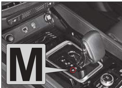
You can shift the gear manually (1st~7th) just as a manual transmission by moving the gear shift lever from the D (driving) position to the M (manual) position.
