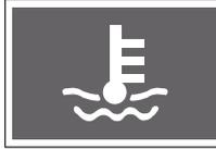
If the temperature of the engine coolant is abnormally high, the engine overheat warning lamp blinks and the warning buzzer sounds.
