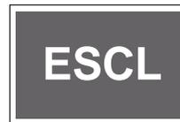
This is the device which has the electronic control of the locking and unlocking of the steering wheel in the vehicle with the smart key. If the ESCL warning lamp comes on, the vehicle may not be started and driven. In this case, have the system checked by a KG Mobility dealer or KG Mobility Authorized Service Center.
