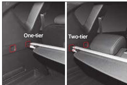
The luggage upper cover can be fixed at the position of one-tier or two-tier according to the angle adjustment level of the rear seat backrest.
