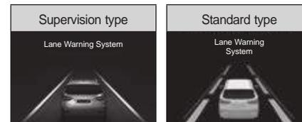
If the vehicle is approaching one of the lanes without the operation of the turn signal while the lane departure warning system is operating normally, the relevant lane blinks.
