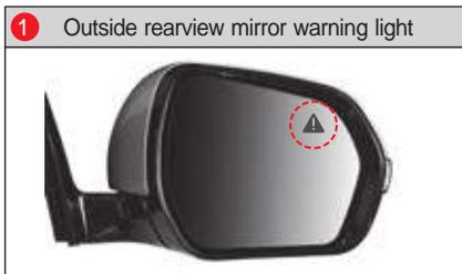
When the outside rearview mirror warning light blinks twice with the START/STOP switch in the ON status or while the engine is running, it indicates that the rear and side warning system is operating normally.
