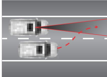
When a vehicle on the next lane changes the lane to the same lane, the vehicle may not be detected until it enters the detection range of the Front Camera Module (FCM).
