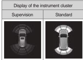
The distance from the obstacle is displayed on the instrument cluster along with the warning buzzer.
