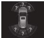
When the obstacle detection sensor is abnormal, “?” is displayed for the relevant sensor. If this message is displayed on the display of the instrument cluster, have your vehicle checked and serviced at a nearby KG Mobility authorized service center.
