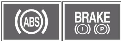
When the ABS warning light and the brake warning light turn on at the same time, it indicates that the EBD system is abnormal. (There is no separate EBD warning light.)
