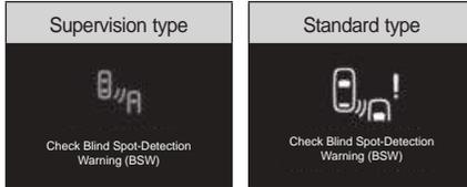
When the rear and side warning system is abnormal, a warning message is displayed on the display of the instrument cluster.
