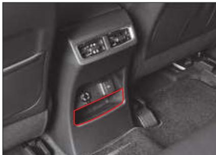
There is a pocket type storage box behind the front seat console storage bin. This is suitable for storing small items.
