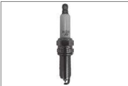
Spark plugs should be inspected periodically for carbon deposits. When carbon accumulates on a spark plug, a strong spark may not be produced. Do not clean the electrodes with a fine wire brush and carefully scrape the carbon off the insulator with a small file. The spark plugs should then be blown clean with compressed air and the upper insulator wiped clean. Do not adjust the spark plug gap.
