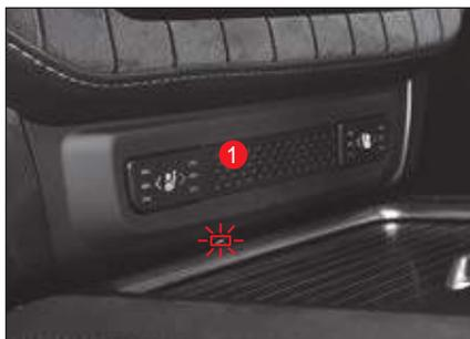
It turns on when the tail light is activated.
