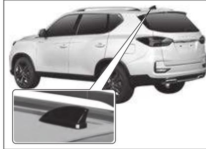
When the audio system is turned on, the antenna receives the following radio waves.
