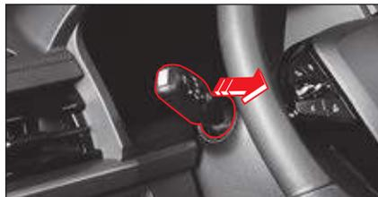
The high beam and the low beam turn on at the same time while pulling the Light switch in the driver's direction.
