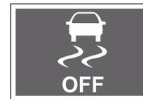
When you deactivate the ESP by pressing and holding down the ESP OFF switch (for 3 seconds or more), the indicator turns on.
