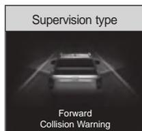
If the distance to the front vehicle is so close that a collision can occur or the front vehicle disappears from the front view due to lane change, etc. while the intelligent cruise control is activated, the message is displayed on the instrument cluster.
