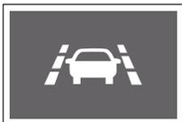
When the lane departure warning system is activated, the indicator on the instrument cluster turns on.
