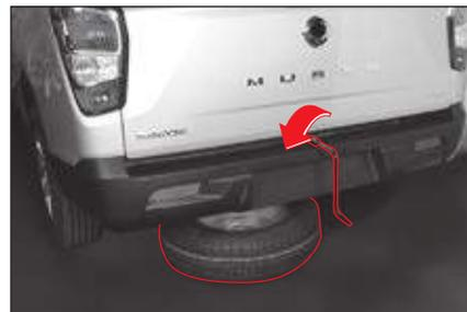
1 Insert the connection rod in the hole located in the upper center of the bumper after opening the tailgate, and then connect the wheel nut wrench to it.
