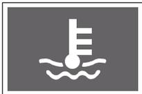
When the engine is overheated, various symptoms appear such as the warning light turns on and steam comes out from the engine.
