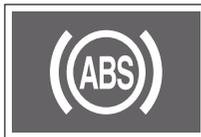
The ABS warning light turns on when the START/STOP switch is in the ON status and turns off approximately 4 seconds later.
