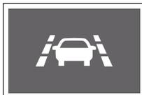
This indicator light up on the instrument cluster when the LKA is activated.
