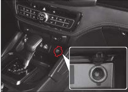
An auxiliary power outlet for extra electrical devices is installed. This power outlet supplies power when the ignition key is in the “ACC” or “ON” position.
