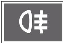
With the headlights turned on, if you rotate the switch in
