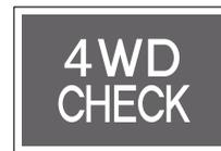
The 4WD CHECK warning indicator turns on if the 4WD switch unit is abnormal.
