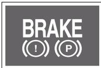
The brake warning light turns on when the START/STOP switch is in the ON status and turns off approximately 4 seconds later. This warning light turns on when the parking brake is applied or the brake fluid is insufficient.
