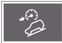
When you press the HDC switch, the system is switched to the HDC operation ready status and the green HDC indicator turns on.
