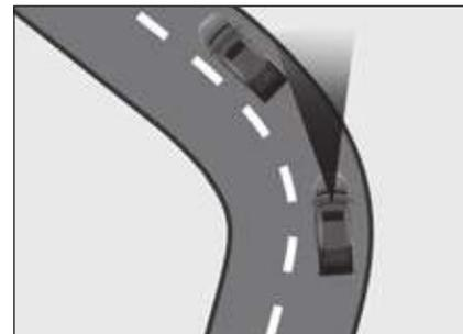
On a curved road, a front vehicle on the same lane cannot be detected and the AEB performance is reduced so that unnecessary warning or braking is applied or the system may not operate.
