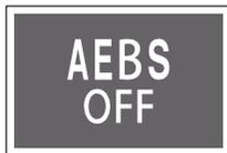
The AEB OFF indicator turns on when the START/STOP switch is in the ON status and it turns off approximately 4 seconds later.
