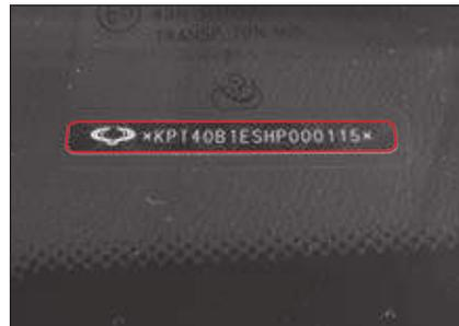
The VIN is stamped on top of the instrument panel.
