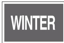
When you press the mode switch "W" next to the gear shift lever, the mode is switched to the winter mode and the winter mode indicator turns on.
