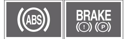
When the ABS warning light and the brake warning light turn on at the same time, it indicates that the EBD system is abnormal. (There is no separate EBD warning light.)
