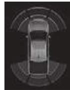
Line No. ③ at the rear right side is deleted and Line No. ④ blinks (Warning buzzer sounds)
