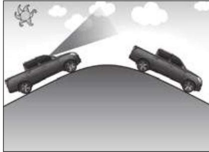
On a uphill road or a downhill road, a vehicle on the same lane cannot be detected and the AEBS performance is lowered so that unnecessary warning or braking is applied or the system may not operate.
