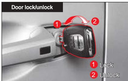
Insert the emergency key into the key hole and turn it clockwise to unlock the door.
