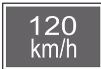
The warning light flashes with repeated (5 times) buzzer sound when the vehicle speed exceeds 120 km/h.
