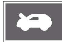
The engine hood open warning light turns on when the engine hood is opened or not closed completely.
