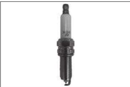
Spark plugs should be inspected periodically for carbon deposits. When carbon accumulates on a spark plug, a strong spark may not be produced.
