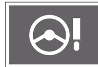
If the Speed Sensing Power Steering (SSPS) device is abnormal, the SSPS warning light turns on and the steering wheel becomes heavier.
