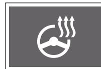
If you press the Steering wheel heater button with the START/STOP switch in the ON status or while the engine is running, the steering wheel heater indicator turns on or turns off.
