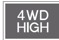
The 4WD HIGH indicator turns on when the START/STOP switch is in the ON status and turns off approximately 4 seconds later.
