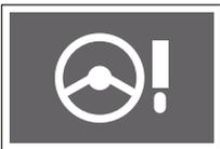
The electric power steering warning light turns on when the ignition switch is turned on and turns off when the ignition is turned on.
