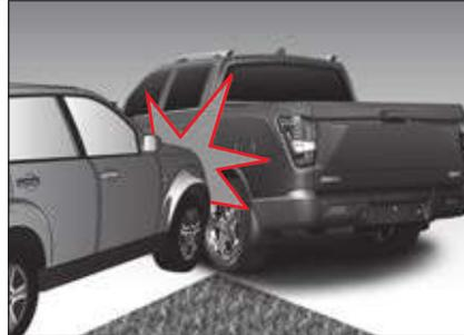
In the event of a side collision, the occupants cannot be protected by the front air bags, so the front air bags may not inflate. However, the curtain air bags and the side air bags operate depending on the degree of impact in the event of a side collision, protecting the front seat occupants.
