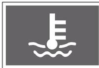
If the temperature of the engine coolant is abnormally high, the engine overheat warning lamp blinks and the warning buzzer sounds.
