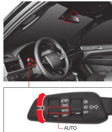
The auto light is the function that detects the amount of sunshine through the sensor and turns on or off the head light and the tail light automatically.
