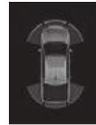
Line No. ① at the front left side is deleted and Line No. ② blinks (Warning buzzer sounds)
