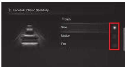
You can change the setting from
