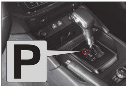
Select this position for parking the vehicle, starting or warming up the engine, or stopping the vehicle for a long period of time.
