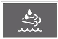
The SCR warning light turns on when the START/STOP switch is in the ON status and it turns off when the engine is started.
