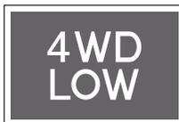
The 4WD LOW indicator turns on when the START/STOP switch is in the ON status and turns off approximately 4 seconds later.
