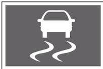
The ESP ON indicator turns on when the START/STOP switch is in the ON status and turns off approximately 4 seconds later.
