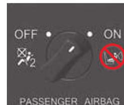
The front passenger air bag is disabled (not inflatable) when placing the passenger air bag ON/OFF switch to "OFF" position. This switch is located on the right side of the instrument panel, and you can see it when opening the front passenger door. Press and turn this switch to operate.
