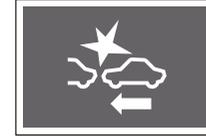
The AEB warning light turns on when the START/STOP switch is in the ON status and turns off approximately 4 seconds later.
