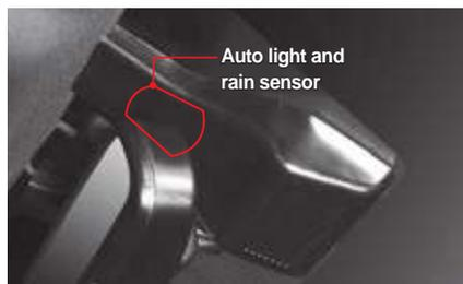
The auto light sensor is integrated with the rain sensor.
