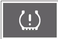
If the tire pressure or the tire pressure monitoring system is abnormal, the global warning light blinks or comes on.
