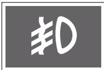
When you place the light switch in
