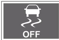
The ESP OFF indicator turns on when the START/STOP switch is in the ON status and turns off approximately 4 seconds later.
