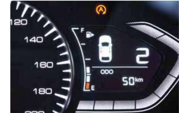
The Intelligent shift reminder in manual transmission indicates the optimum time to shift gears up or down providing greater fuel economy.
