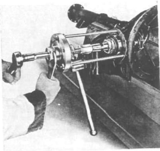
FIG. 273—PINION AND BEARING REMOVER AND REPLACER
