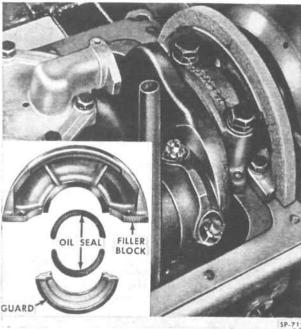
FIG. 71—CRANKSHAFT REAR OIL SEAL AND FILLER BLOCK
