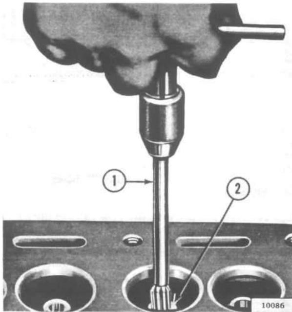
FIG. 68—REAMING VALVE GUIDE
