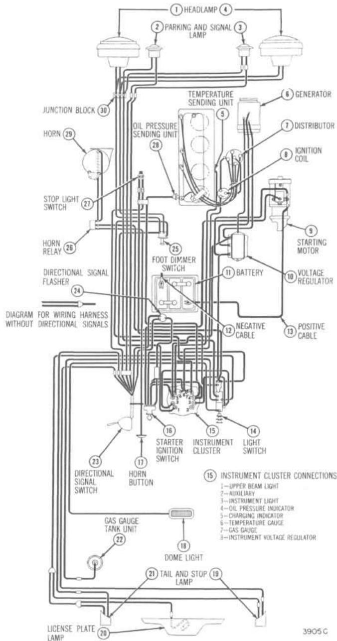
FIG. 158—WIRING DIAGRAM—F4-134 4x4 AND 4x2
