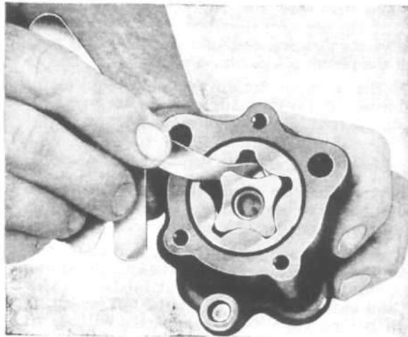
FIG. 121—CHECKING OIL PUMP ROTORS
