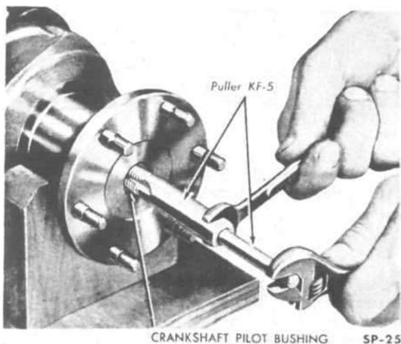
FIG. 45—REMOVING CRANKSHAFT PILOT BUSHING
