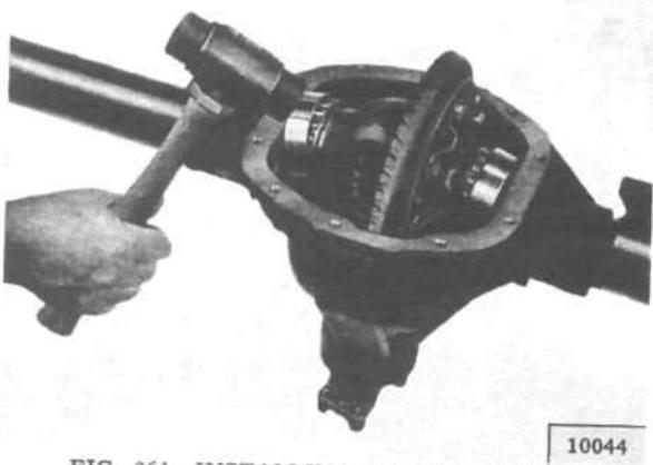
FIG. 264—INSTALLING DIFFERENTIAL
