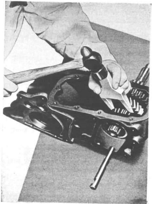
FIG. 209—BEARING CONE REMOVING WEDGE
