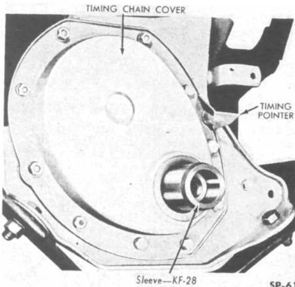
FIG. 86—INSTALLING TIMING CHAIN COVER AND POINTER
