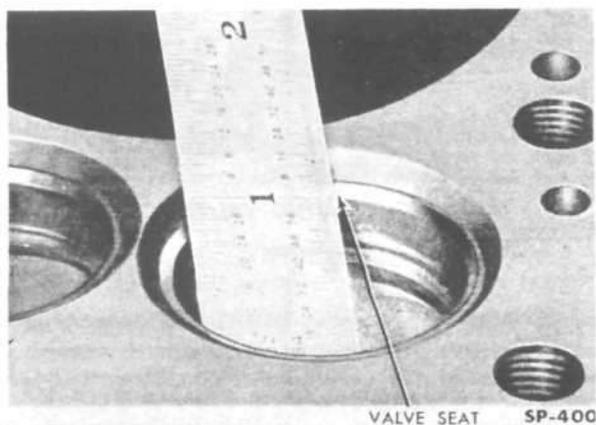
FIG. 61—CHECKING VALVE SEAT WIDTH
