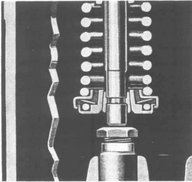
FIG. 11—VALVE WITH BEARING TYPE ROTATOR
