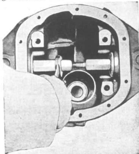
FIG. 263—INNER OIL SEAL INSTALLER
