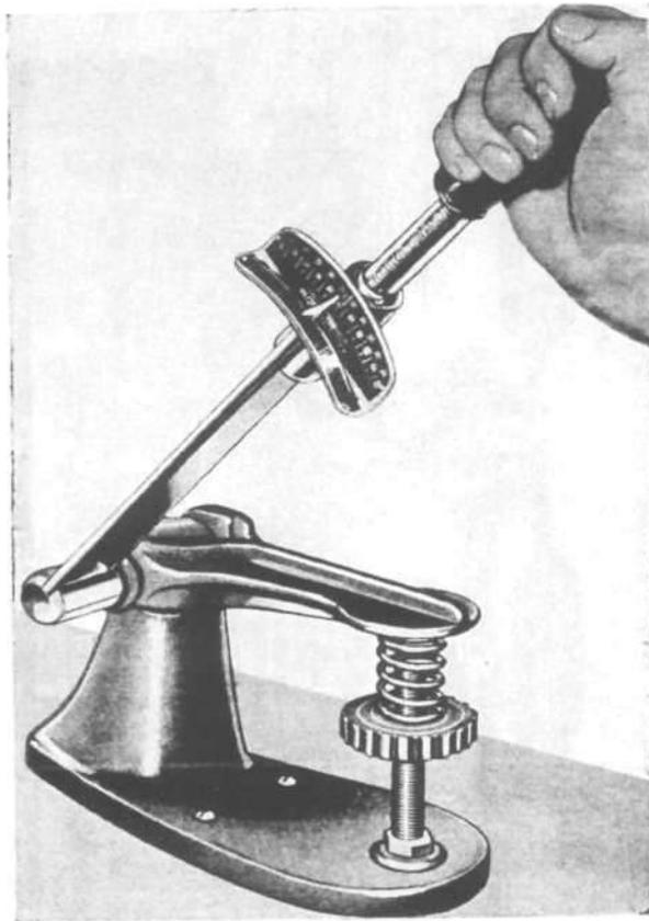
FIG. 99—SPRING TESTING
