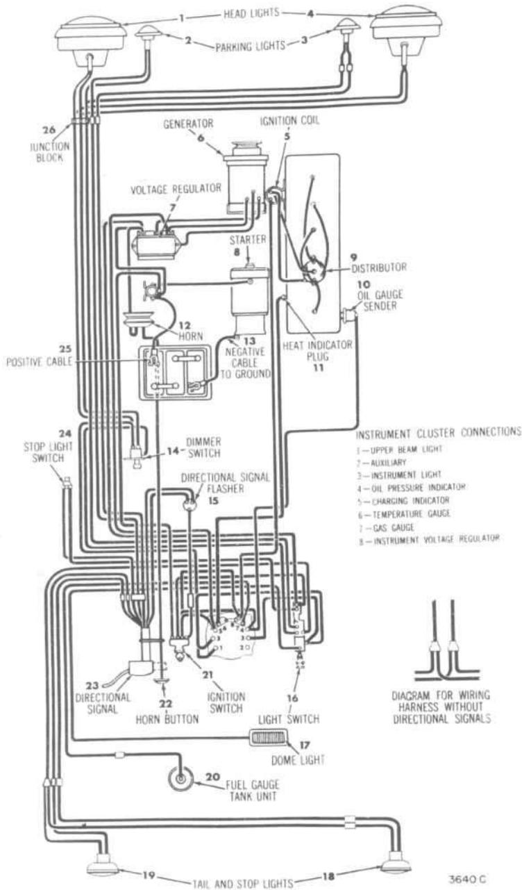
FIG. 155—WIRING DIAGRAM—L6-226 4WD
