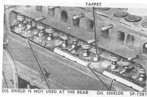
FIG. 22—VALVE TAPPET CHAMBER, TAPPETS AND OIL SHIELDS
