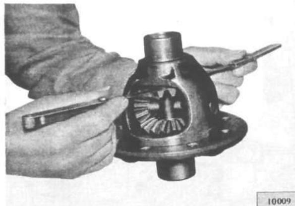
FIG. 259—CHECKING SIDE GEAR CLEARANCE
