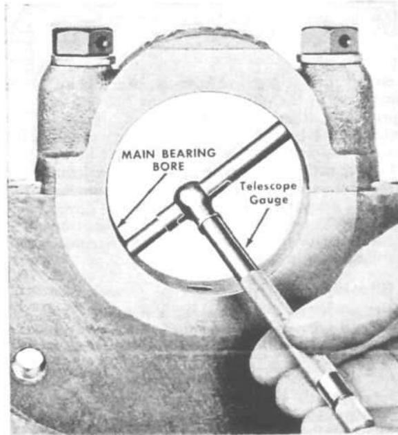
FIG. 48—MEASURING MAIN BEARING BORES
