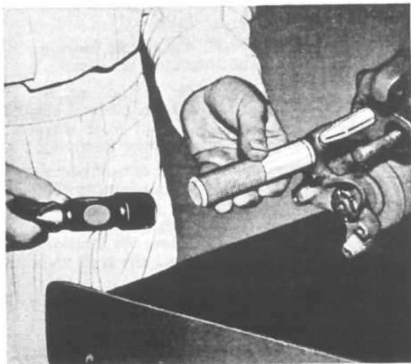
FIG. 214—SHIFT ROD OIL SEAL INSTALLER
