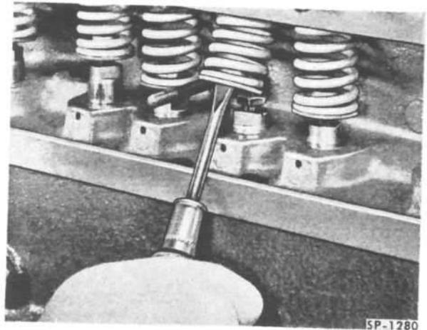
FIG. 24—REMOVING VALVE SPRINGS
