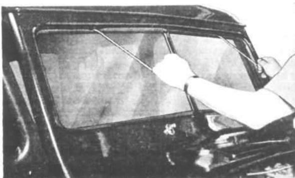
FIG. 309—WINDSHIELD GLASS INSTALLATION
