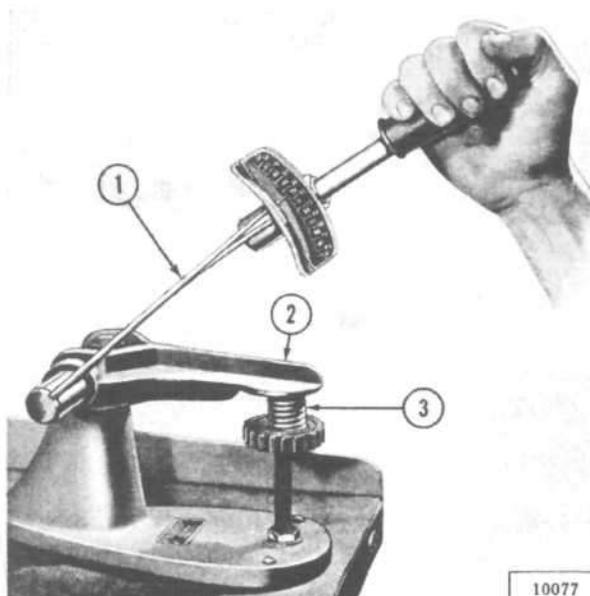
FIG. 58—TESTING VALVE SPRING
