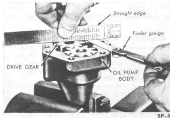
FIG. 76—CHECKING GEAR TO COVER CLEARANCE
