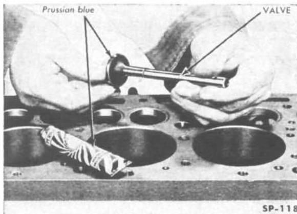
FIG. 65—CHECKING FIT OF VALVE IN VALVE SEAT
