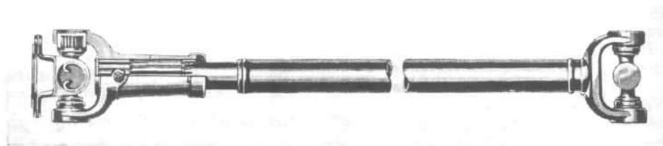
FIG. 221 — PROPELLER SHAFT AND UNIVERSAL JOINTS—NEEDLE BEARING TYPE
