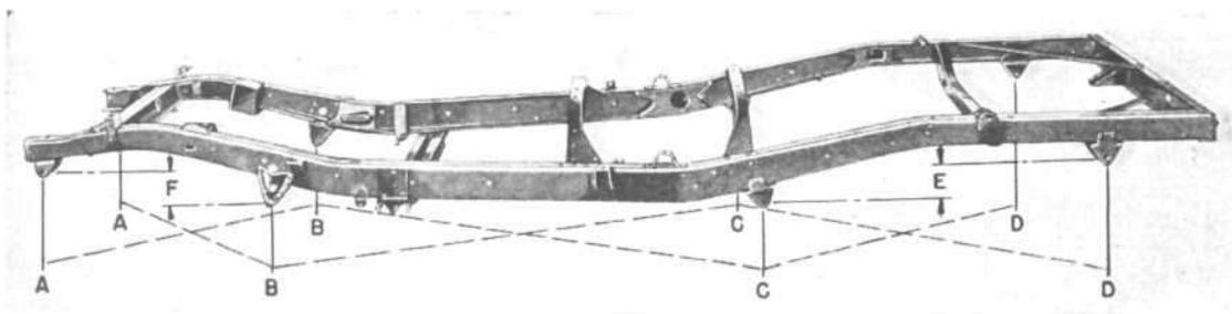
FIG. 296—TYPICAL FRAME SHOWING POINTS FOR MEASURING ALIGNMENT
