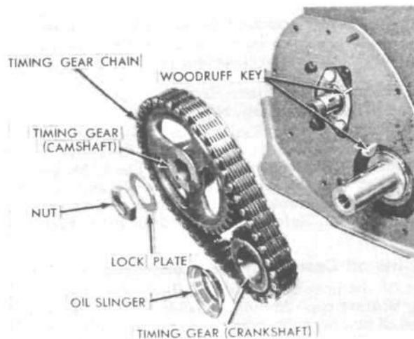
FIG. 84—TIMING GEARS AND CHAIN
