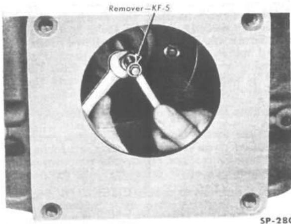
FIG. 186—REMOVING CRANKSHAFT PILOT BUSHING
