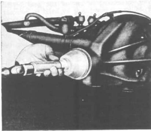
FIG. 267—PINION SHAFT OIL SEAL
