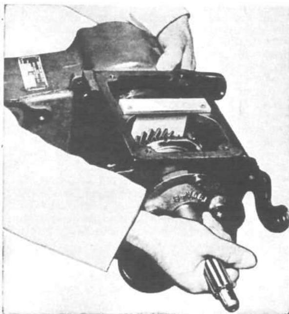
FIG. 189—MAINSHAFT RETAINING PLATE W-194
