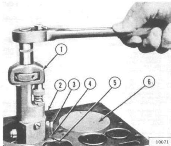
FIG. 20—REMOVING RIDGE FROM CYLINDER BORE
