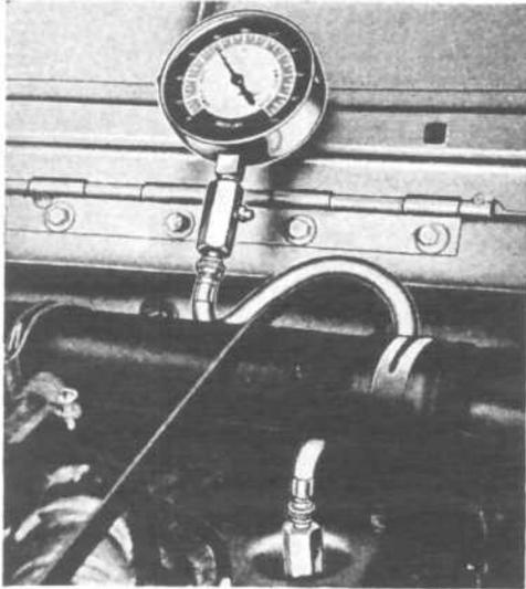
FIG. 18—COMPRESSION AND VACUUM GAUGE
