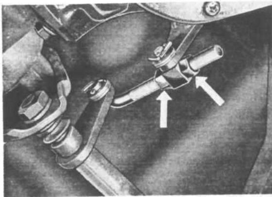
FIG. 173—CLUTCH ADJUSTMENT—L6-226 MODELS
