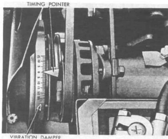
FIG. 14—L6-226 ENGINE TIMING MARKS
