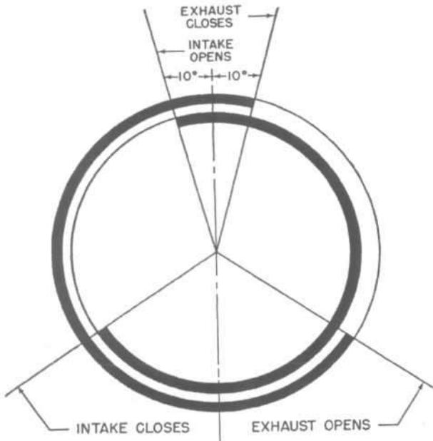
FIG. 88—VALVE TIMING—EARLY L6-226 ENGINES
