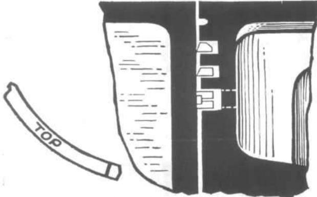
FIG. 115—PISTON RING INSTALLATION
