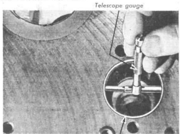
FIG. 53—CHECKING CAMSHAFT BEARING INSIDE DIAMETER
