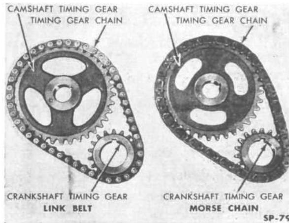
FIG. 56—TWO TYPES OF TIMING CHAINS AND GEARS
