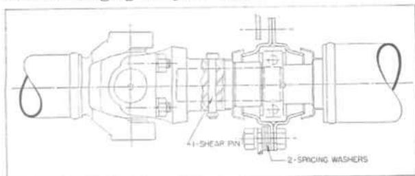
FIG. 315—SPICER PROPELLER SHAFT
