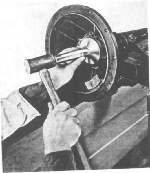
FIG. 272—DIFFERENTIAL BEARING CUP DRIVER
