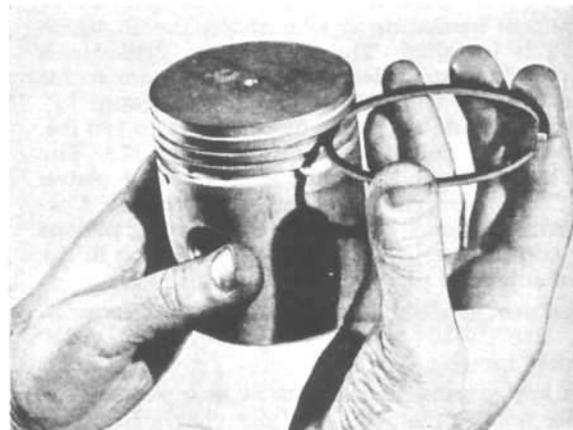
FIG. 117—COMPRESSION RING FITTING
