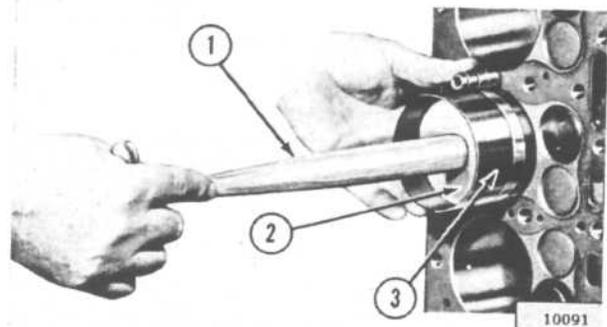
FIG. 87—INSTALLING PISTON AND CONNECTING ROD ASSEMBLY
