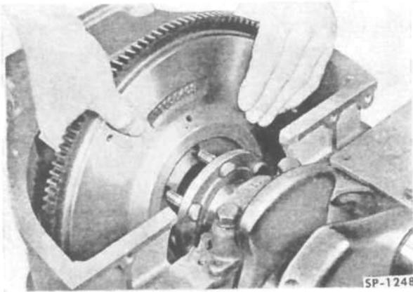
FIG. 82—INSTALLING FLYWHEEL ON CRANKSHAFT
