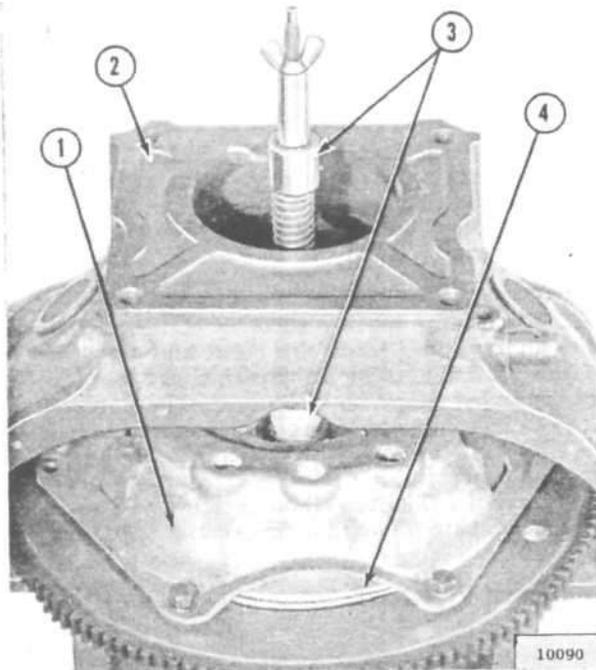
FIG. 83—INSTALLING CLUTCH ON FLYWHEEL
