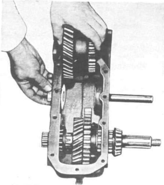
FIG. 215—THRUST WASHER PILOT
