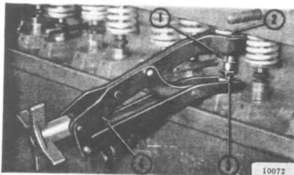
FIG. 23—REMOVING VALVE SPRING LOCKS
