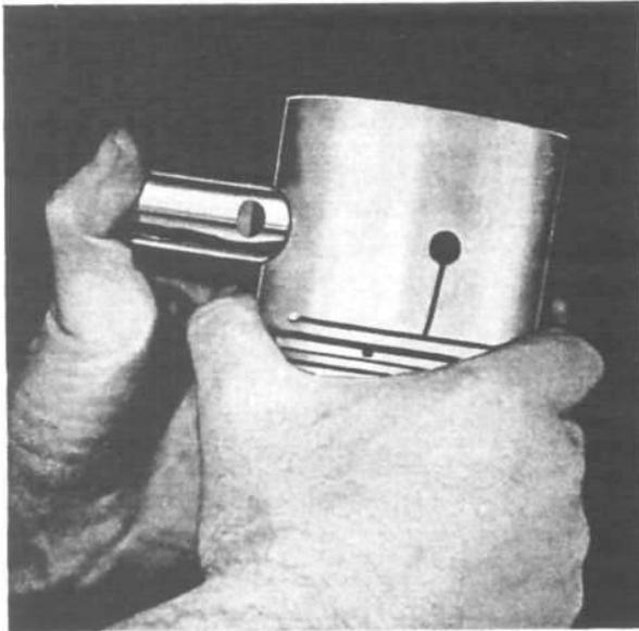
FIG. 118—PISTON PIN FITTING
