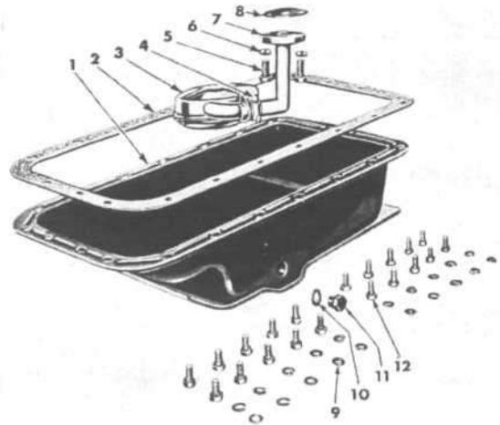
FIG. 124—FLOATING OIL INTAKE AND OIL PAN 124, No. 7, is flat. Clean both the flange and the crankcase surfaces thoroughly before installing a new gasket. Be sure the retaining screws are tight. The oil pan screw torque wrench reading is 9 to 14 lb-ft. [1,24 a 1,94 kg-m.].
