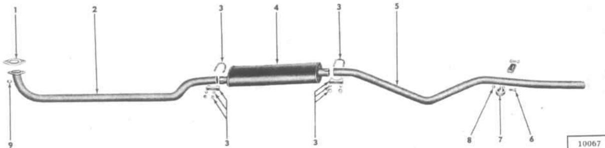
FIG. 145—EXHAUST PIPE AND MUFFLER
