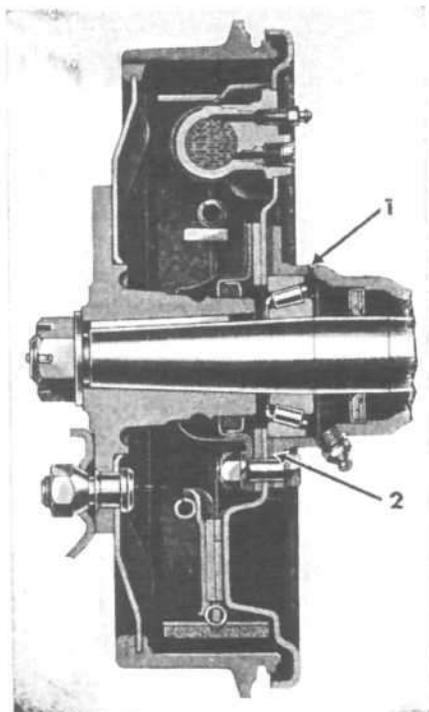
FIG. 294—REAR WHEEL HUB AND BEARING
