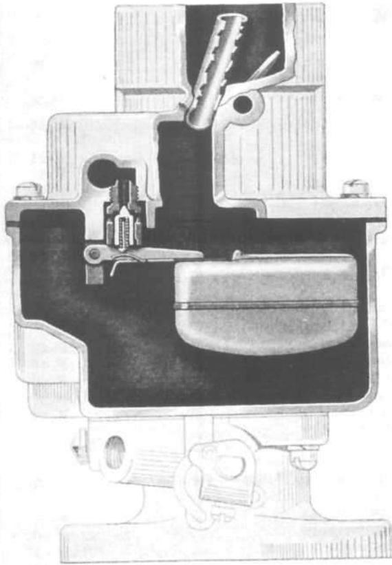
FIG. 127—THE FLOAT CIRCUIT
