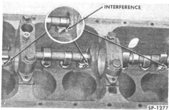
FIG. 85—CAMSHAFT JOURNAL AND TAPPET INTERFERENCE
