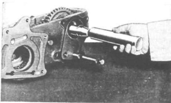
FIG. 216—OUTPUT SHAFT SNAP RING INSTALLER
