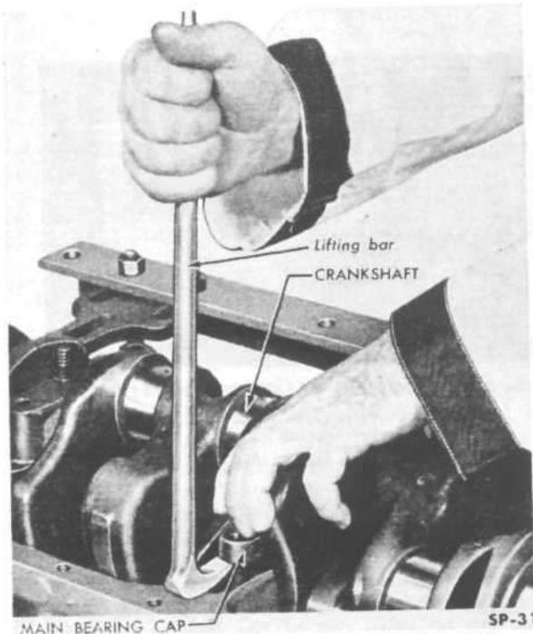
FIG. 28—REMOVING MAIN BEARING CAP
