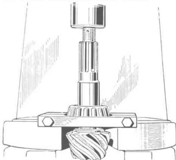
FIG. 252—REMOVING PINION BEARING
