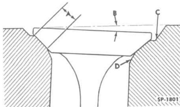
FIG. 64—PROPERLY REFACED VALVE SEAT
