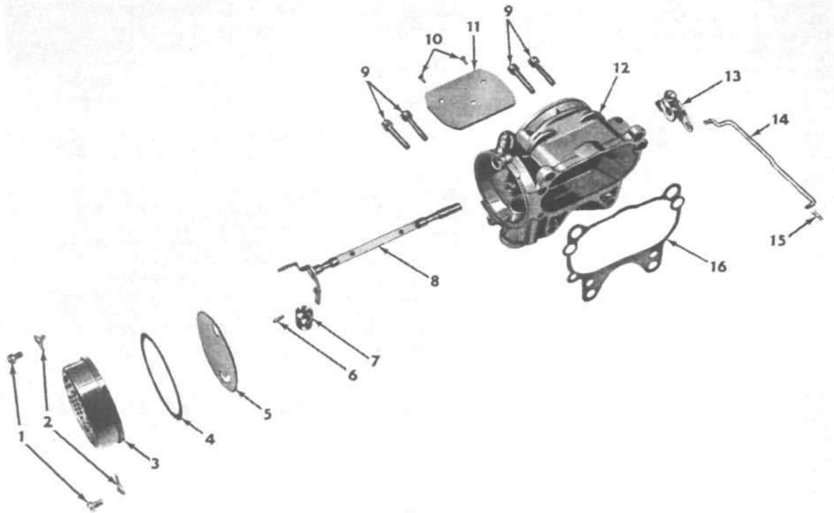
FIG. 138—2204S CARBURETOR AIR HORN AND ATTACHING PARTS
