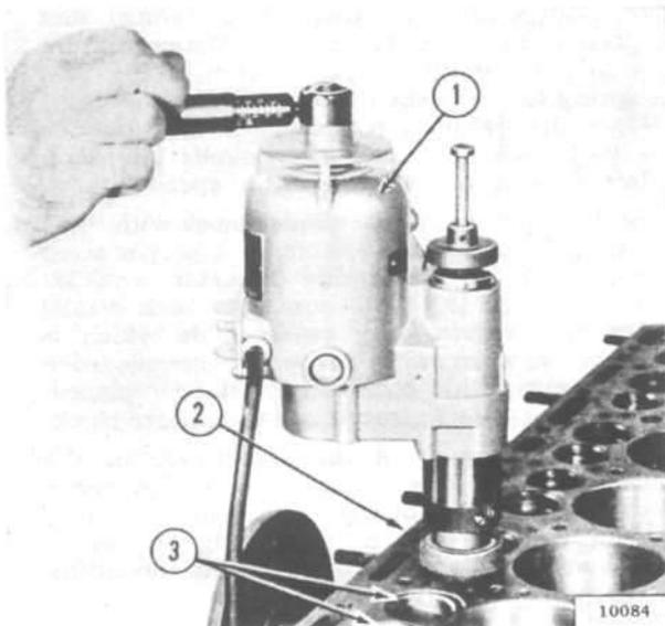
FIG. 60—REFACING VALVE SEATS
