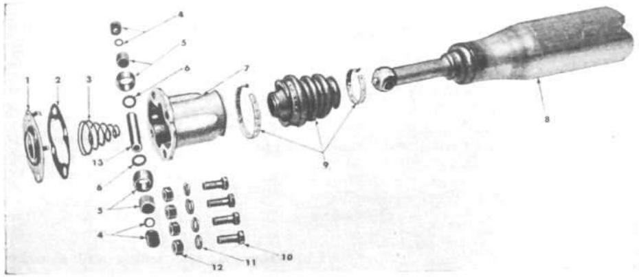
FIG. 220—PROPELLER SHAFT AND UNIVERSAL JOINT—BALL AND TRUNNION TYPE
