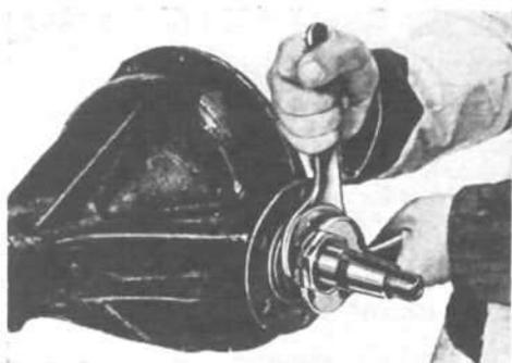
FIG. 276—PINION BEARING ADJUSTING WRENCHES
