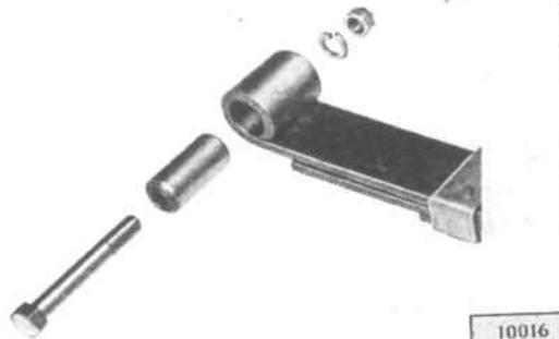
FIG. 299—SPRING PIVOT BOLT
