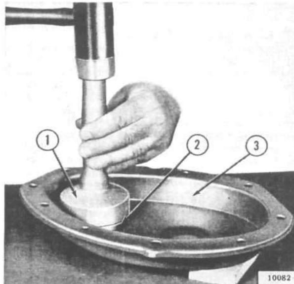
FIG. 57—INSTALLING TIMING CHAIN COVER OIL SEAL
