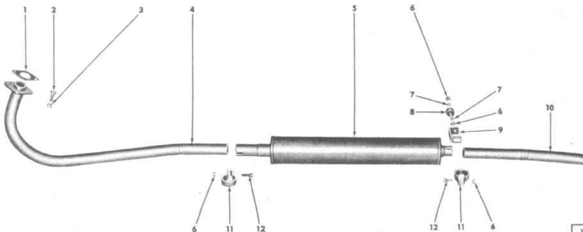
FIG. 146—EXHAUST PIPE AND MUFFLER
