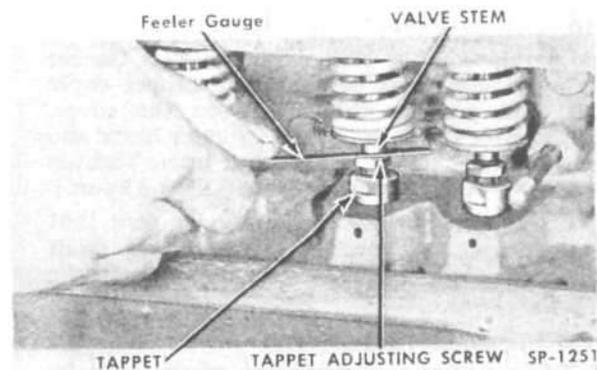
FIG. 95—CHECKING VALVE CLEARANCE
