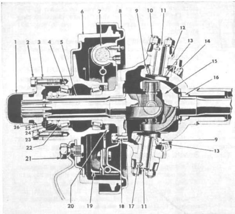
FIG. 236—FRONT STEERING KNUCKLE (With Spicer Universal Joints)
