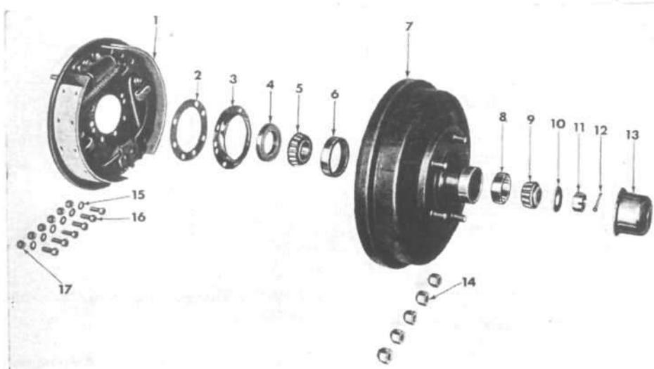
FIG. 292—FRONT WHEEL ATTACHING PARTS — 2-WHEEL-DRIVE VEHICLES
