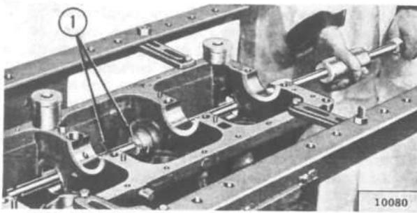
FIG. 54—REMOVING CAMSHAFT BEARINGS
