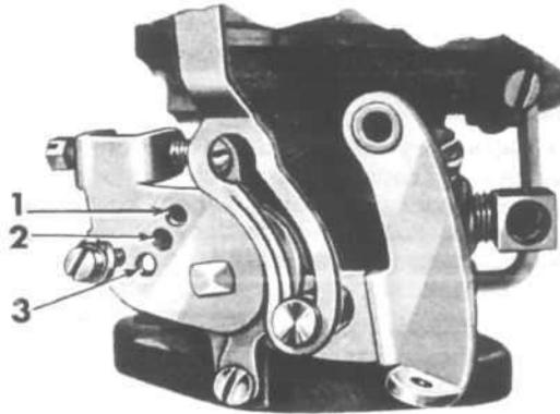
FIG. 317—THROTTLE BELL CRANK
