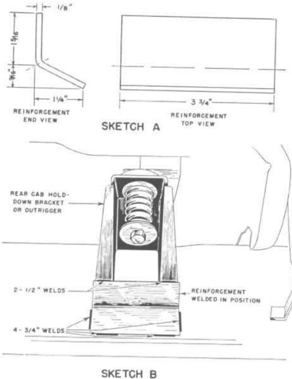
FIG. 311—CAB MOUNTING BRACKET REINFORCEMENT
