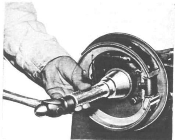
FIG. 218—OUTPUT SHAFT OIL SEAL DRIVER
