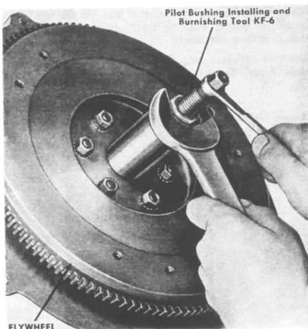
FIG. 181—INSTALLING PILOT BUSHING TO FLYWHEEL
