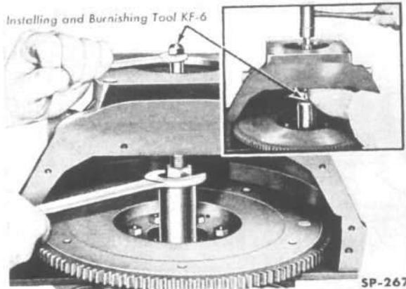
FIG. 187—INSTALLING AND BURNISHING CRANKSHAFT PILOT BUSHING
