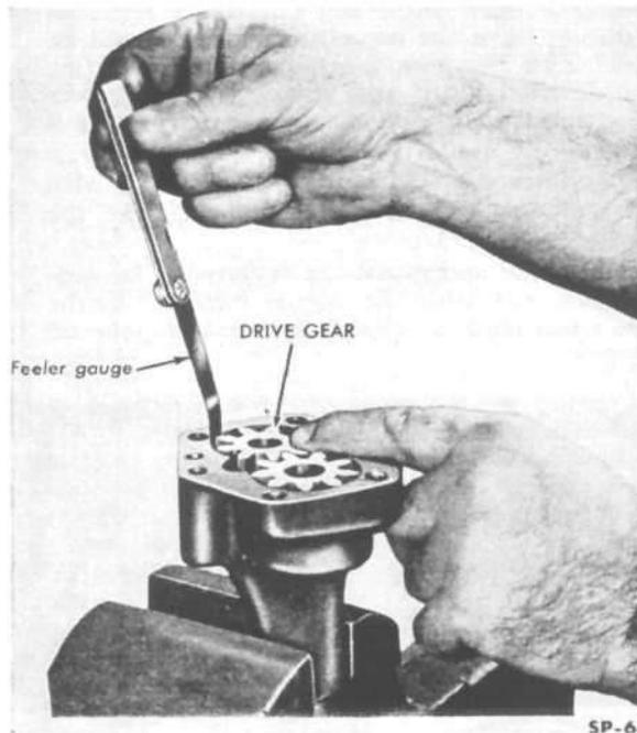
FIG. 75—CHECKING GEAR TOOTH TO BODY CLEARANCE
