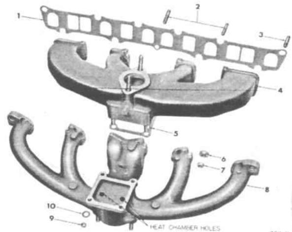
FIG. 143—MODEL L6-226 INTAKE AND EXHAUST MANIFOLD (Single-throat Carburetor)
