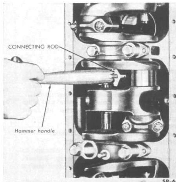
FIG. 21—REMOVING PISTON AND CONNECTING ROD ASSEMBLY
