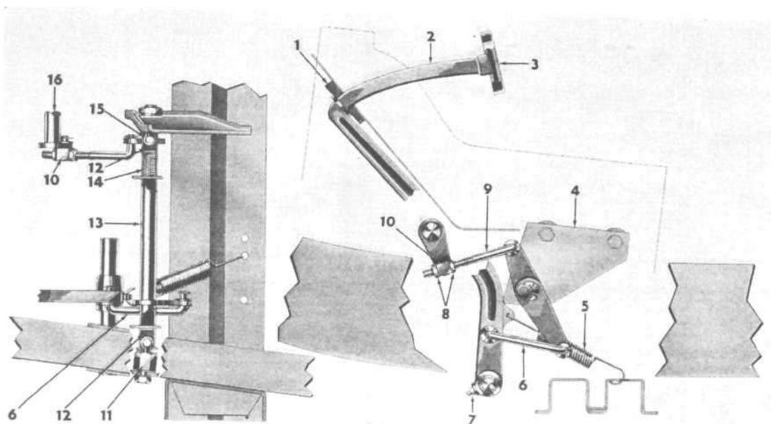
FIG. 172—CLUTCH CONTROL—L6-226 MODELS
