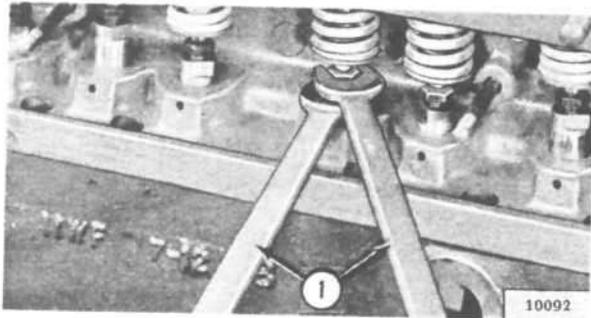
FIG. 96—VALVE TAPPET ADJUSTMENT
