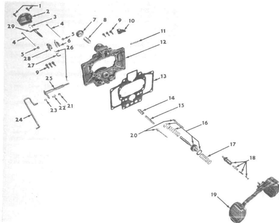
FIG. 135—2204S CARBURETOR BOWL COVER AND ATTACHING PARTS
