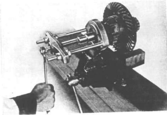
FIG. 268—DIFFERENTIAL BEARING PULLER
