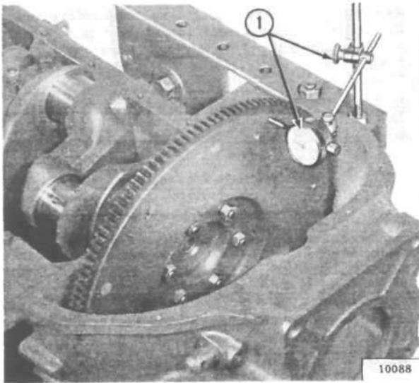
FIG. 79—CHECKING FLYWHEEL RUN-OUT
