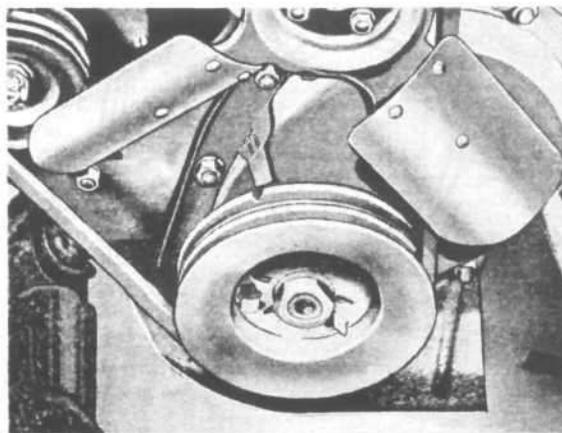
FIG. 13—F4-134 ENGINE TIMING MARKS
