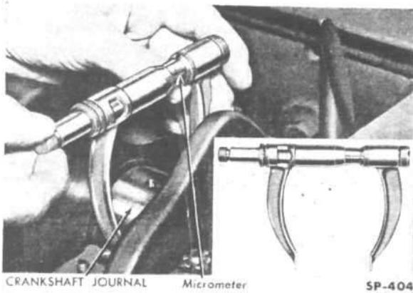
FIG. 44—MEASURING CRANKSHAFT JOURNAL DIAMETER
