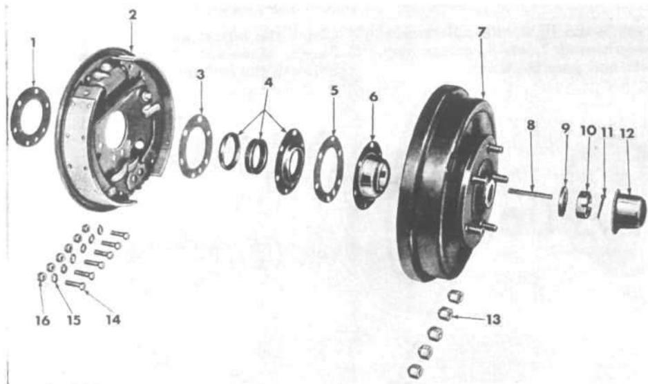
FIG. 293—REAR WHEEL ATTACHING PARTS
