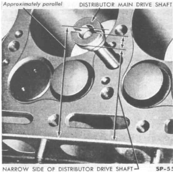
FIG. 93—CORRECT POSITION OF DISTRIBUTOR MAIN DRIVE SHAFT
