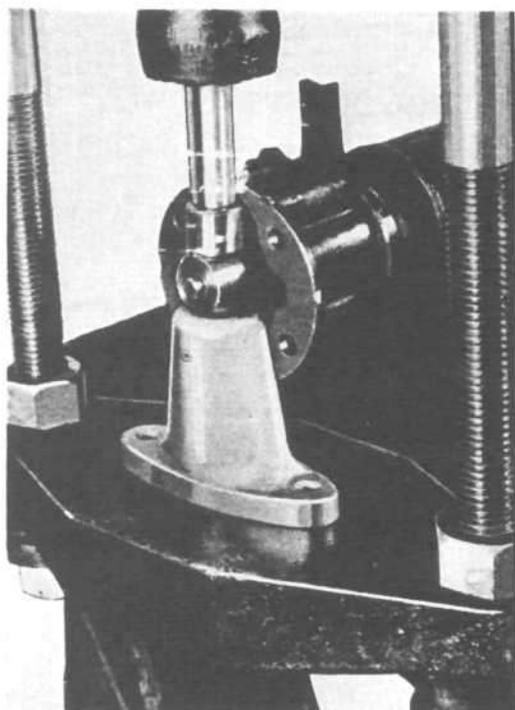
FIG. 223—UNIVERSAL JOINT PIN REMOVER AND REPLACER
