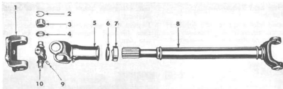
FIG. 222—PROPELLER SHAFT AND UNIVERSAL JOINTS—NEEDLE BEARING TYPE
