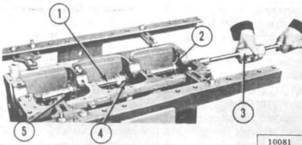
FIG. 55—INSTALLING CAMSHAFT BEARINGS
