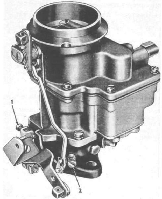
FIG. 16—CARBURETOR ADJUSTMENTS
