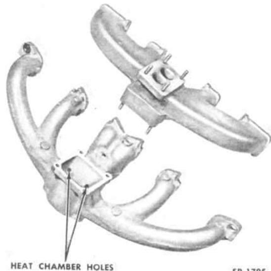
FIG. 144—MODEL L6-226 INTAKE AND EXHAUST MANIFOLD (Double-throat Carburetor)
