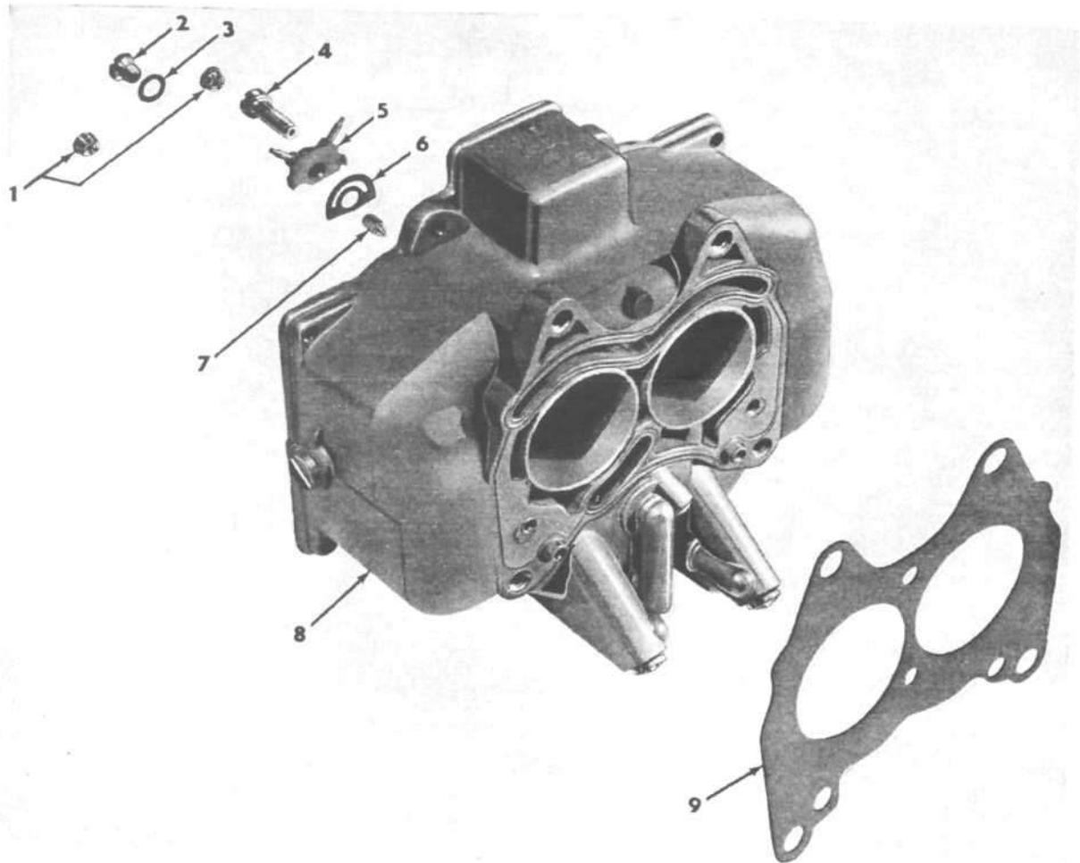
FIG. 136—2204S CARBURETOR BOWL AND ATTACHING PARTS
