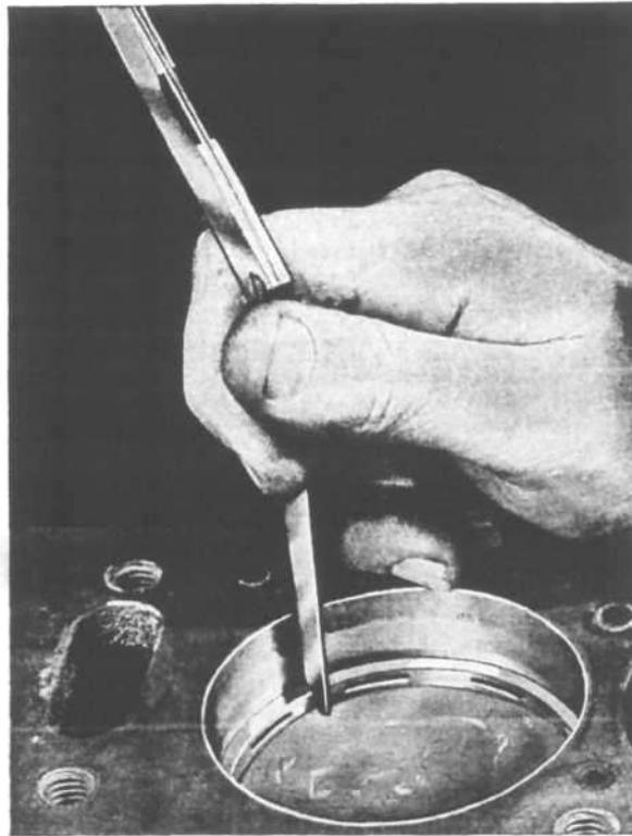
FIG. 116—PISTON RING GAP
