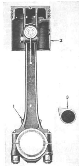
FIG. 119—CONNECTING ROD AND PISTON
