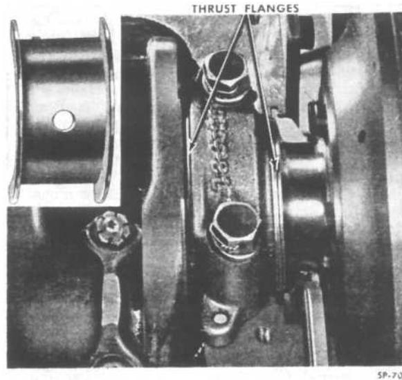
FIG. 51—REAR MAIN BEARING INSTALLATION
