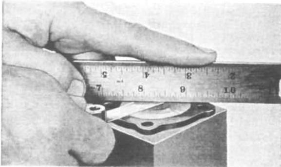
FIG. 123—CHECKING OIL PUMP COVER
