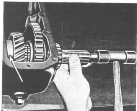
FIG. 210—BEARING CUP REMOVING RING
