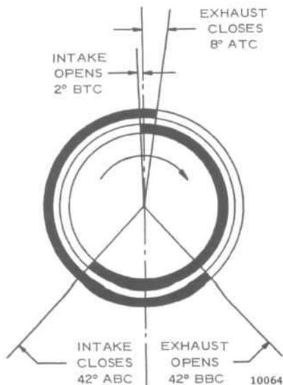
FIG. 89—VALVE TIMING—LATE L6-226 ENGINES
