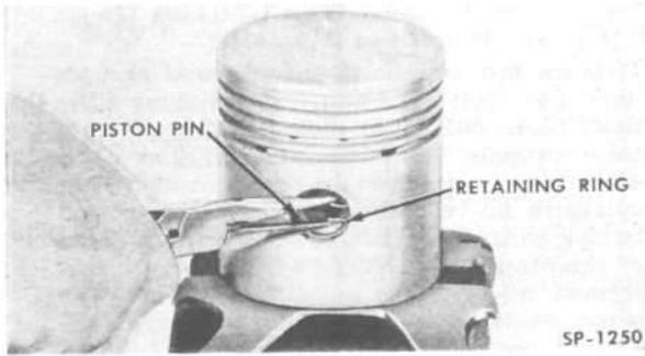
FIG. 36—REMOVING PISTON PIN
