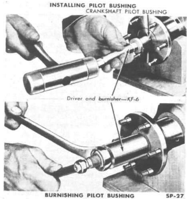
FIG. 46—INSTALLING AND BURNISHING CRANKSHAFT PILOT BUSHING
