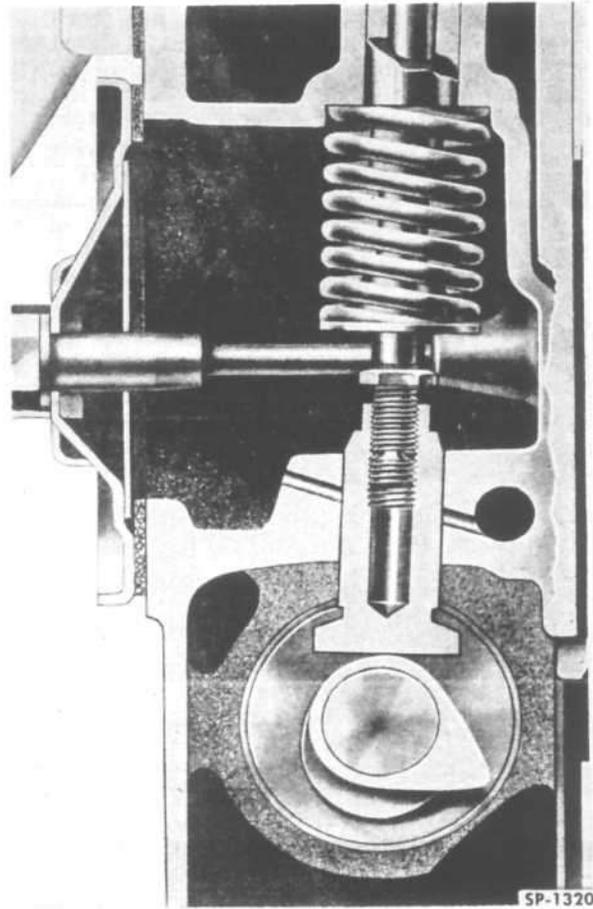
FIG. 94—CAMSHAFT, TAPPET AND VALVE
