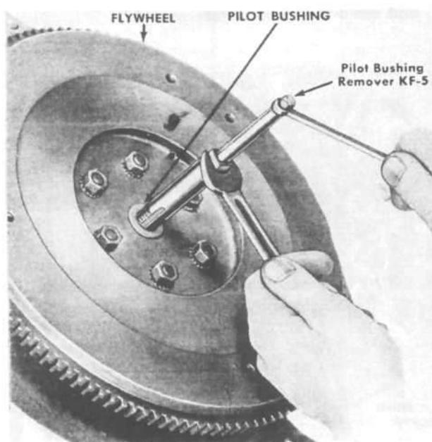
FIG. 180—REMOVING PILOT BUSHING FROM FLYWHEEL
