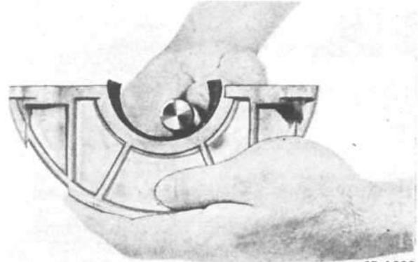
FIG. 72—INSTALLING OIL SEAL IN CRANKSHAFT REAR FILLER BLOCK
