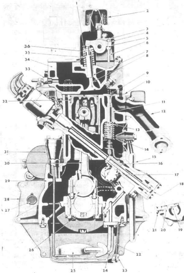
FIG. 97—FOUR-CYLINDER F-HEAD ENGINE — END VIEW
