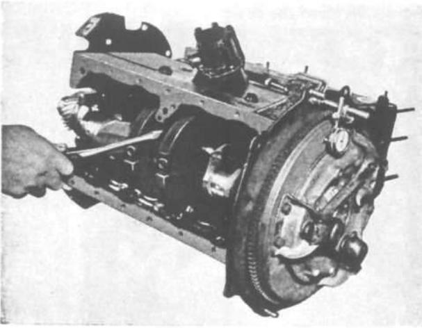
FIG. 107—GAUGING CRANKSHAFT END PLAY
