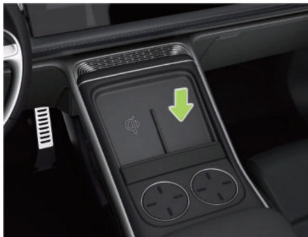
1. Put the smart key in the position of the arrow on the sub IC.
