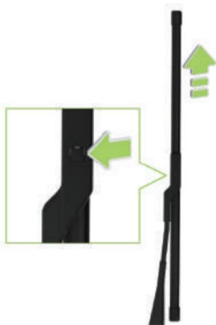
1. Lift the wiper arm, press the lock button, and pull out the wiper blade upward.
