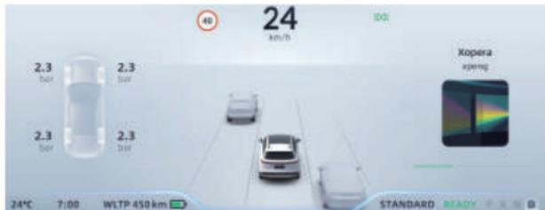
TSR acquires the speed limit information by recognizing the speed limit sign on the road and combining navigation, and displays it on the ICM.
