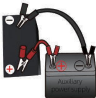
5. Connect one end of the black cable to the negative (-) terminal of the vehicle's 12V battery and the other end to the negative (-) terminal of the auxiliary external power supply.
