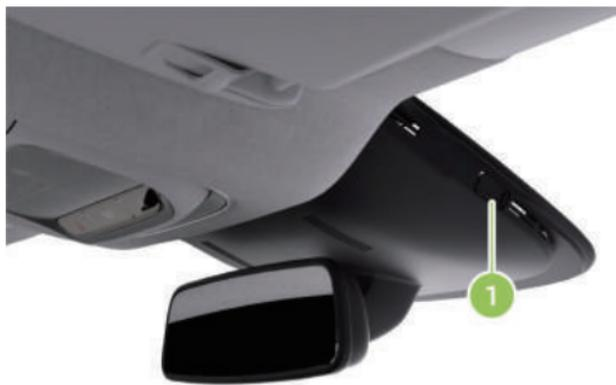
1. USB power port: Can charge the car recorder, with a maximum output current of 2.1A.
