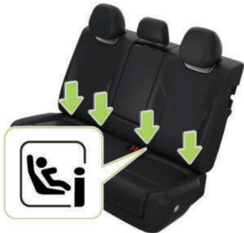
The ISOFIX anchorages are located between the backrests and cushions of the rear left and right seats. The exact location of each anchorage is marked as above (as shown in the figure).
