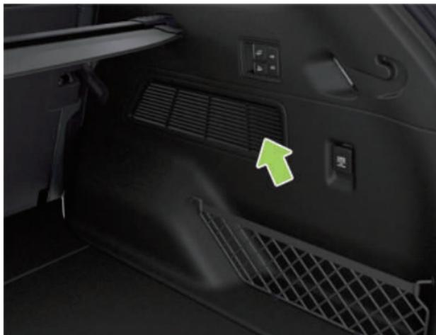
1. Open the trunk and locate the air vent cover located on the right side of the trunk and use the appropriate tool to open the cover at the opening.
