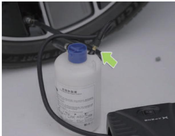
5. Connect the other sealant injection tube to the inflatable pump and tighten it, then insert the electrical source plug of the inflatable pump into the 12V power supply in the vehicle storage box.
