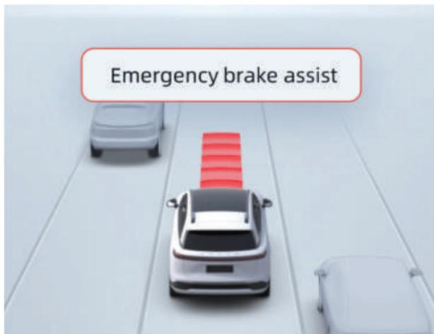
If the driver fails to apply the brakes in time or the braking force is too small, the automatic emergency braking will be started to alleviate or avoid the crash damage.
