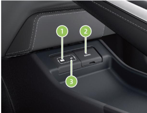
1. USB Media Source Port: Used for data transfer, microphone, game controller, etc.
