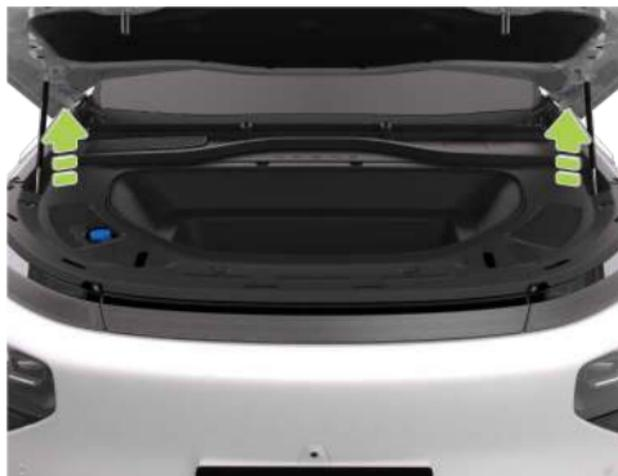
2. Slightly lift the front hood, and it will automatically rise to the limit position with the left and front air springs.
