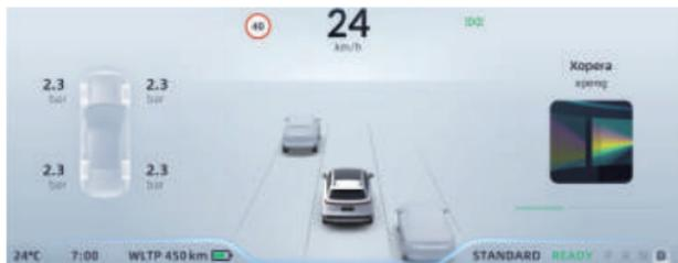
The environment simulation display system is an essential part of the assistive driving system. It simulates and displays the external environment through the ICM, including the lane lines and other traffic participants.
