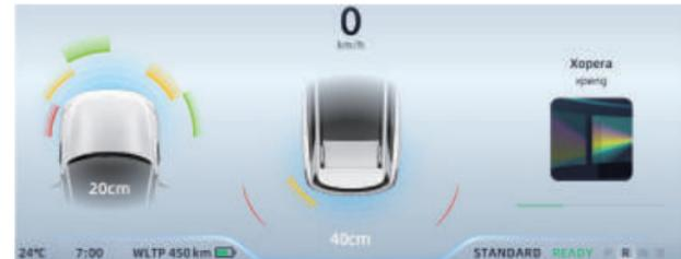
When the vehicle is in R/N gear and the speed is between 2-15 km/h, and there is a vehicle, pedestrian, or two-wheeler approaching at a certain speed within the detection range, with a crash risk, RCTA is activated. It provides reminders through ICM and warning tones.
