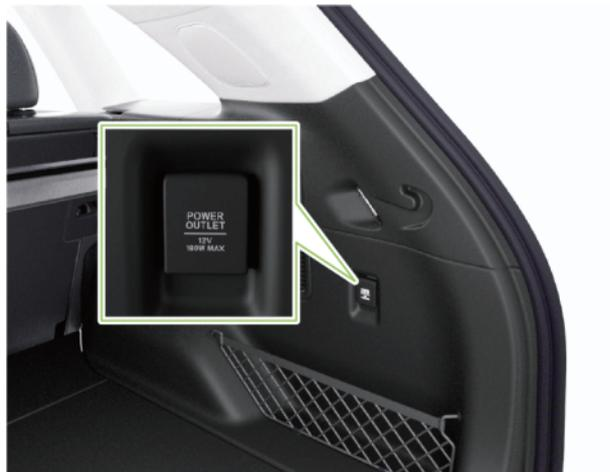
12V Power Supply Port: Maximum supported power is 180W.
