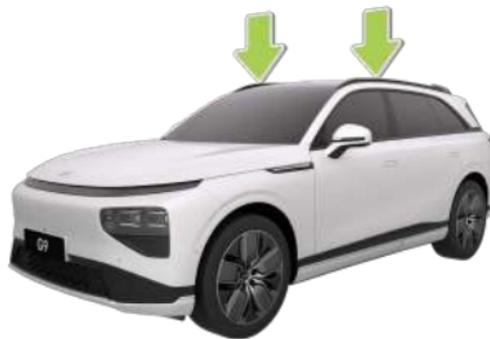
The vehicle features mounting holes for an optional roof rack. When using a roof rack, please follow the instructions and safety warnings provided in this section, as well as the user manual for the roof rack itself.
