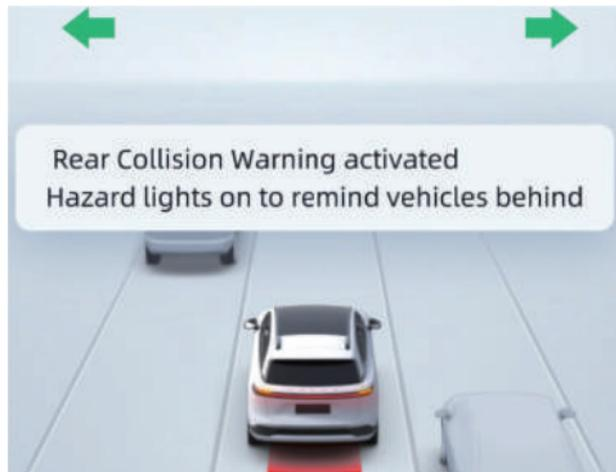
When the vehicle speed is between 0-160 km/h, if there are vehicles, pedestrians, or two-wheelers approaching at a certain speed within the detection range, and there is a crash risk, RCW will be activated. It will provide warnings through ICM, audible alerts, and illuminate the
