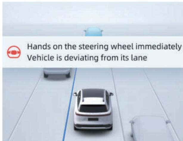
When Lane Departure Assistance is set to the warning mode, LDW enables: if the vehicle deviates from its lane without using the turning lamp with the speed is between 60 km/h-150 km/h, the system provides alerts through ICM, audible warning tones, and steering wheel
