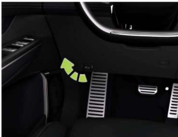
1. The front hood opening handle is located on the left side of the driver's foot space. After continuously pulling the handle twice,
