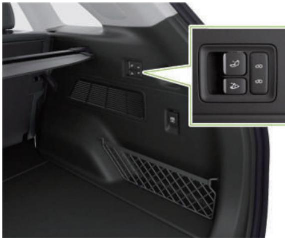
Press the up or down switch of the trunk inner suspension to adjust the height of the trunk, which can facilitate the loading and unloading of items.
