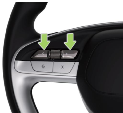
The vehicle-following distance gear can be set by the left/right button at the left of the steering wheel, and there are 5 gears to choose from.
