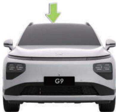
The microwave window is on the front windscreen. Please keep the front windscreen clean so as to ensure the best results and minimize interference with the driving view.
