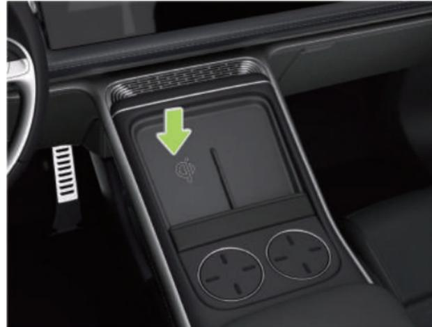
The wireless charging area is located inside the front storage box. When charging, please place the phone with the front side up within the sensing area along the stop bar. The CID will display an icon “” while charging.
