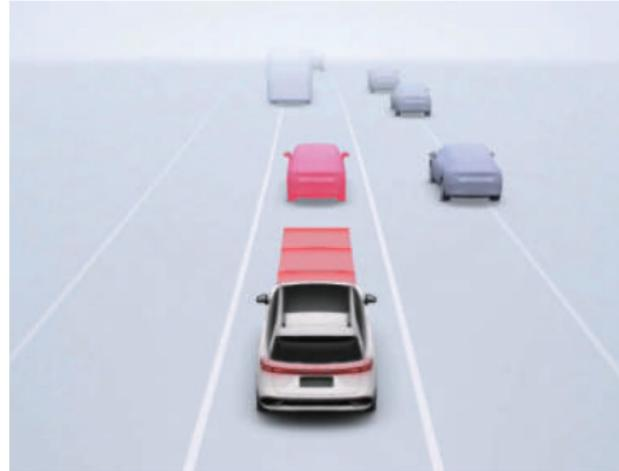
When the function detects that there is a risk of a crash with the preceding vehicle, it will remind the driver via the ICM and alert sound. If the crash risk is greater, the function will remind the driver via stab braking.
