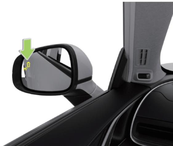
When the vehicle speed is greater than 10km/h, if there is a vehicle in the blind spot or a fast-approaching one behind the blind spot, the corresponding side's exterior rearview mirror warning light will illuminate. If the turning lamp or lane change signal on that side is activated at
