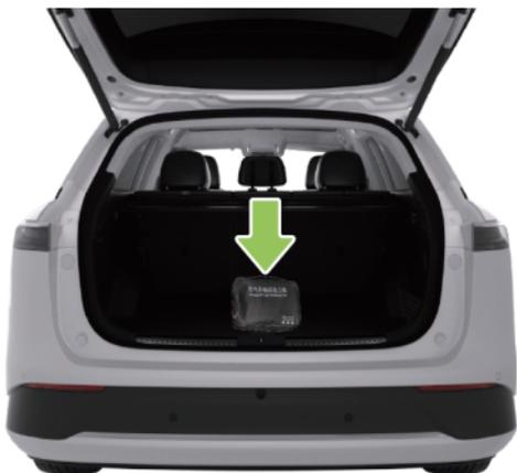
1. Take out the emergency tire-repair kit from the trunk.
