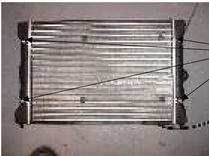
The four plastic bosses on the outside of the radiator need to be tapped M6 to the bottom of the blind hole (Make Sure You Do Not Go To Deep And Break Into The Main Radiator)
