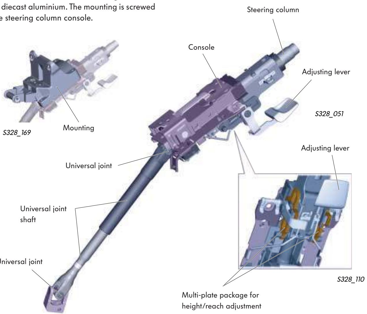
As part of occupant protection, the steering column and universal joint shaft are designed to slide inside each other. This means the steering column and steering wheel cannot be pushed towards the driver when the front section of the car is deformed in a collision.
