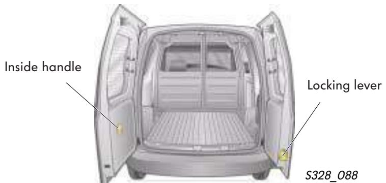
The left-hand wing door needs to be opened first. The outside handle on the left-hand door is integrated in the number plate light fitting. The locking lever built into the bottom of the right-hand door can then be used to open the right-hand wing door. Wing doors lock at a 90° angle when opened. If the door latches are detached, the wing doors will open to approx. 170° due to a stop in the hinge.
