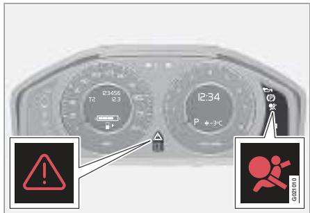
The airbag system is continuously monitored by the system's control module. The warning symbol in the combined instrument panel illuminates when the remote control key is in position **II** or **III**. The symbol goes out after approx. 6 seconds provided the airbag system is fault-free.
