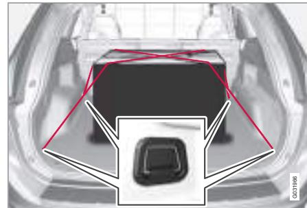
Each corner of the cargo area has attachment points intended for the anchorage of loads.
