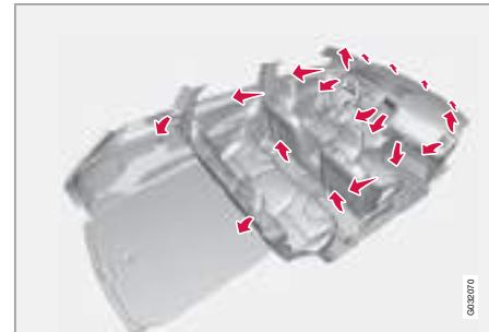
The incoming air is divided between 20 different vents in the passenger compartment.
