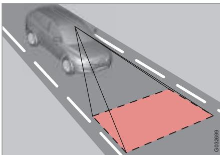
The function is intended to reduce the risk for single-vehicle accidents – accidents where, in certain situations, the vehicle leaves the carriageway and is in danger of driving either into a ditch or into oncoming traffic.
