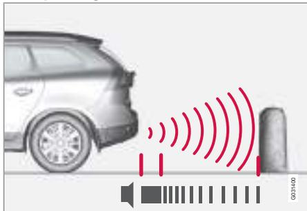
The distance covered to the rear of the car is about 1.5 metres. The acoustic signal for obstacles behind comes from the rear loudspeakers.
