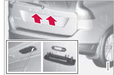
1. Remove the screws with a screwdriver.
