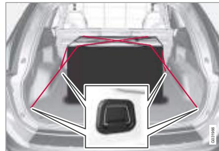
Each corner of the cargo area has attachment points intended for the anchorage of loads.
