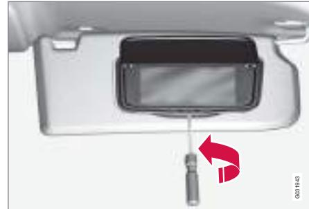
1. Insert a screwdriver underneath the lower edge, in the centre. Carefully prize up the lug on the edge.
