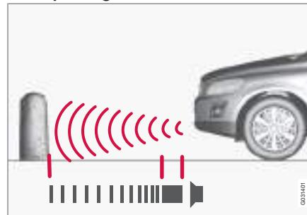
The distance covered to the front of the car is about 0.8 metres. The acoustic signal for obstacles in front comes from the front loudspeaker.
