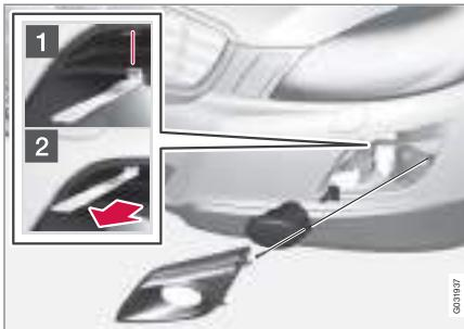
Undo the cover by pulling out the top corner, closest to the grille, see the illustration above.
