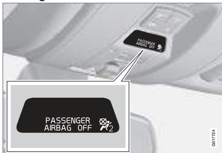
Indicator in the roof console showing that the passenger airbag is deactivated.
