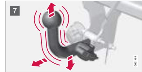
7 Check that the towball section is secure by pulling it up, down and back.
