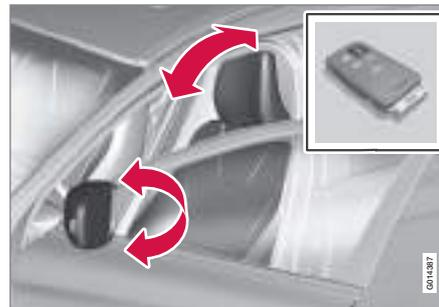
When the car is unlocked with the same remote control key and the driver's door is opened the driver's seat and also the door mirrors auto-
