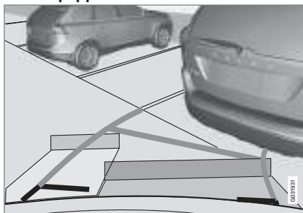
If the car is also equipped with Park Assist\* rear (see page 179), coloured markings indicate the distance to the obstacle, e.g. when reversing into a parking spot.
