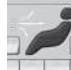
The figure consists of three buttons. When the buttons are pressed a lamp in front of the respective part of the figure illuminates and shows which air distribution is selected, see page 127.
