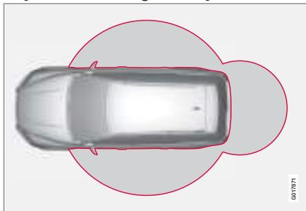
The keyless drive function in the PCC allows the car to be unlocked, driven and locked without the need for a key. You simply have to have the PCC with you. The system makes it easier and more convenient to open the car, for example when your hands are full.
