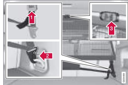
The safety net can be easily removed and folded up.
