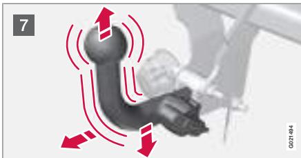
7 Check that the towball section is secure by pulling it up, down and back.
