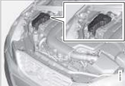
When topping up the coolant, follow the instructions on the packaging. It is important that the mixture of coolant concentrate and water is correct for the prevailing weather conditions. Never top up with water only. The risk of freezing increases with both too little and too much coolant concentrate. For capacities, see page 273.
