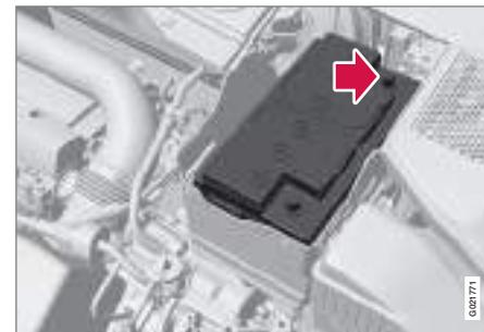
1. Lower the battery into the battery box.
