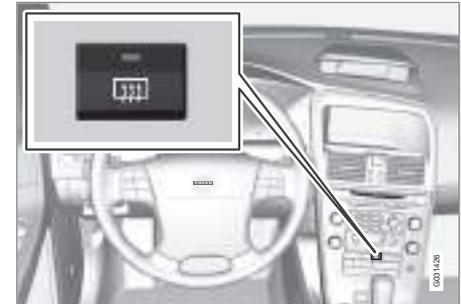
Use the defroster to quickly remove misting and ice from the rear window and the door mirrors.
