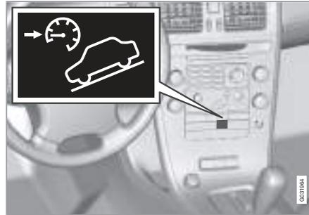
HDC is engaged or disengaged using a switch on the centre console. An indicator lamp in the button illuminates when the function is switched on. When HDC is operating the
