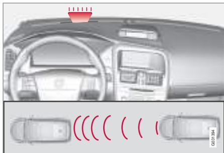
A small section of the red warning lamp in the windscreen illuminates with a constant glow when driving closer than the set time interval to vehicles in front.
