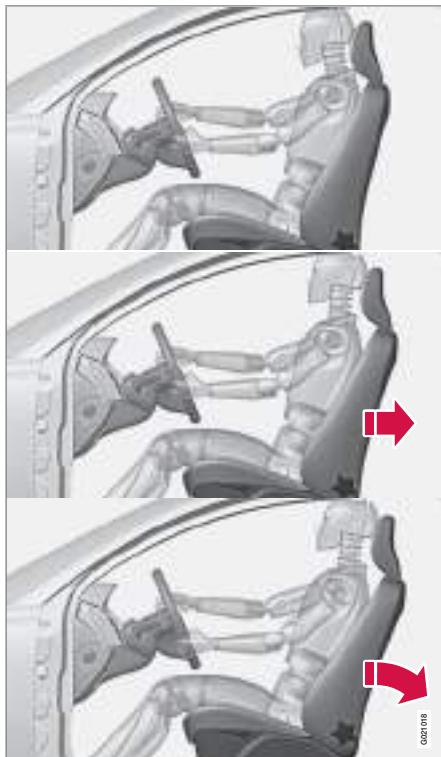
The whiplash protection system (WHIPS) consists of energy absorbing backrests and specially designed head restraints in the front seats. The system is actuated by a rear-end collision, where the angle and speed of the collision, and the nature of the colliding vehicle all have an influence.
