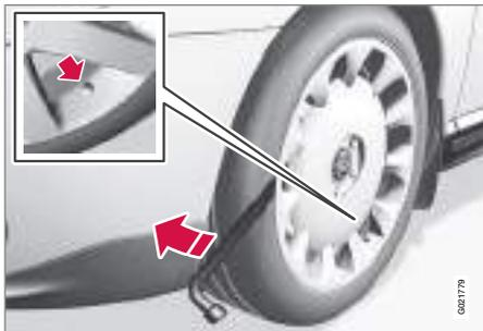
4. Loosen the wheel nuts  $\frac{1}{2}$ -1 turn anticlockwise with the wheel wrench.
