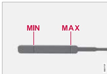
*The oil level must be within the area marked on the dipstick.*
