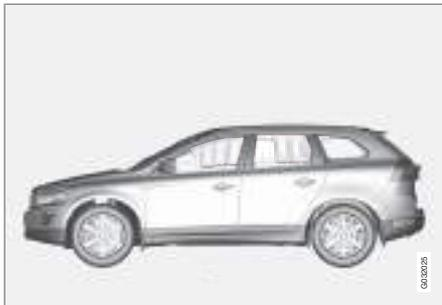
The inflatable curtain (IC) is a supplement to the SIPS and SRS airbags. It is fitted in the headlining along both sides of the roof and protects the car occupants sitting in the outer seats. A sufficiently violent collision trips the sensors and the inflatable curtain is inflated. The inflatable curtain helps to prevent the driver and passengers from striking their heads on the inside of the car during a collision.
