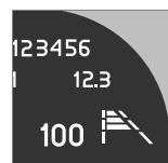
The number of lines for the selected time interval is shown during the setting itself and for several seconds afterwards. Then a smaller scale version of the symbol is shown to the right of the display. The same symbol is also shown when adaptive cruise control is activated.
