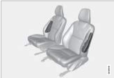
In a side impact collision a large proportion of the collision force is transferred by the SIPS (Side Impact Protection System) to beams, pillars, the floor, the roof and other structural parts of the body. The side airbags at the driver's and front passenger seats protect the chest area and the hip and are an important part of the SIPS.
