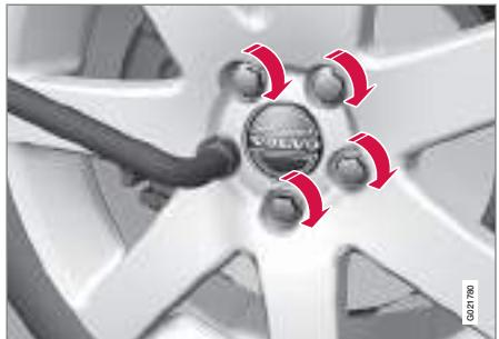
4. Tighten the wheel bolts crosswise. It is important that the wheel bolts are tightened properly. Tighten to 140 Nm. Check the torque with a torque wrench.
