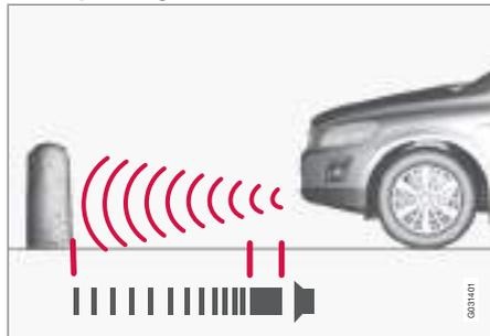
The distance covered to the front of the car is about 0.8 metres. The acoustic signal for obstacles in front comes from the front loudspeaker.
