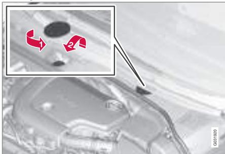
The fluid reservoir is located on the driver's side.
