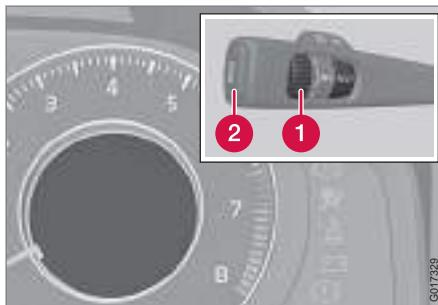
**1** Thumbwheel. Turn the rotary control until the display shows **Driver Alert**. The second row displays the **Off**, **Unavailable** or **Level mark** options.
