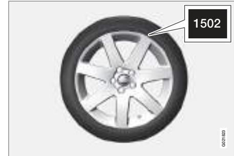
Tyres are perishable. After a few years they begin to harden at the same time as the friction capacity/characteristics gradually deteriorate. For this reason, aim to get as fresh tyres as possible when you replace them. This is especially important with regard to winter tyres. The week and year of manufacture, the tyre's DOT marking (Department of Transportation), are stated with four digits, for example 1502. The tyre in the illustration was manufactured in week 15 of 2002.
