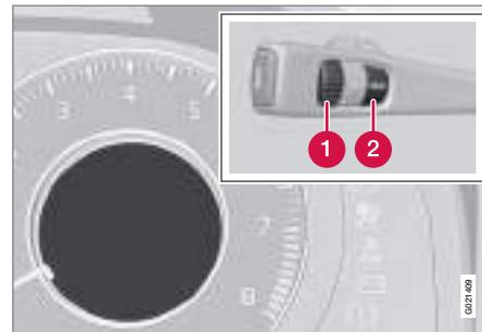
1. Turn the thumbwheel **1** until the **DSTC** menu is shown. **DSTC ON** means that the system function is unchanged.
