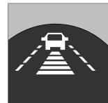
Five different time intervals can be chosen from and shown in the display as 1–5 horizontal lines – the more lines there are the longer the time interval.
