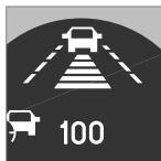
Five different time intervals can be chosen from and shown in the display as 1–5 horizontal lines – the more lines there are the longer the time interval, see page 159 for table.
