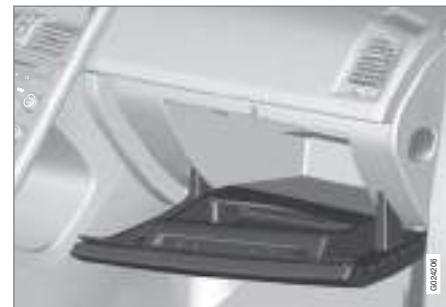
The owner's manual and maps can be kept here for example. There are also holders for pens on the inside of the lid. The glovebox can be locked with the key blade, see page 42.
