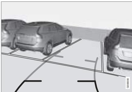
The lines on the screen are projected as if they were at ground level behind the car and are directly related to steering wheel movement, which shows the driver the path the car will take, even when turning.
