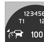
The car symbol is illuminated on the left-hand side of the display when the radar sensor has detected another vehicle. The distance to vehicles in front is only regulated when the symbol is illuminated.
