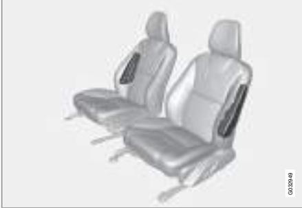
In a side impact collision a large proportion of the collision force is transferred by the SIPS (Side Impact Protection System) to beams, pillars, the floor, the roof and other structural parts of the body. The side airbags at the driver's and front passenger seats protect the chest area and the hip and are an important part of the SIPS.
