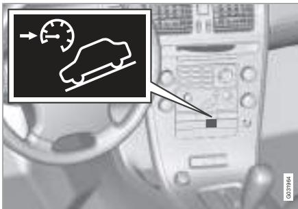
HDC is engaged or disengaged using a switch on the centre console. An indicator lamp in the button illuminates when the function is switched on. When HDC is operating the
