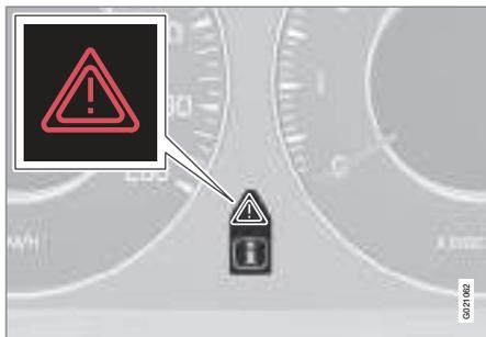
If the car is involved in a collision, the text **Safety mode See manual** may appear on the information display. This means that the car has reduced functionality. Safety mode is a protective state that is enforced when the collision may have damaged any of the car's vital functions, such as the fuel lines, sensors for one of the safety systems, or the brake system.
