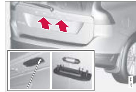
Both the brake light and the reversing lamp bulbs are replaced from inside the cargo area.
