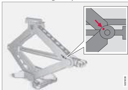
The tools and jack must be returned to their correct places after use. The jack must be cranked to the correct position in order to have space.
