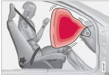
The car has an airbag to supplement the protection afforded by the seatbelt on the passenger side. This airbag is folded up into a compartment above the glovebox. Its cover panel is marked **SRS AIRBAG**.
