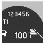
The number of lines for the selected time interval is shown during the setting itself and for several seconds afterwards. Then a smaller scale version of the symbol is shown to the right of the display. The same symbol is also shown when Distance Alert is activated, see page 159.
