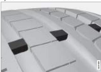
Tread wear indicators are narrow treadless bands across the width of the tread. On the side of the tyre are the letters **TWI** (Tread Wear Indicator). When the tyre's tread depth is down to 1.6 mm, the tread depth will be level in height with the tread wear indicators. Change to new tyres as soon as possible. Remember that tyres with little tread depth provide very poor grip in rain and snow.
