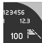
The number of lines for the selected time interval is shown during the setting itself and for several seconds afterwards. Then a smaller scale version of the symbol is shown to the right of the display. The same symbol is also shown when adaptive cruise control is activated.
