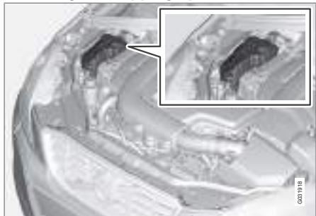
When topping up the coolant, follow the instructions on the packaging. It is important that the mixture of coolant concentrate and water is correct for the prevailing weather conditions. Never top up with water only. The risk of freezing increases with both too little and too much coolant concentrate. For capacities, see page 273.
