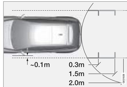
The side lines indicate the path the car will take during reversing. They indicate approx. 10 cm of "free space" between the inside of the line and the outer tip of the door mirrors - even when turning.
