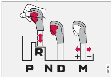
The gear selector can be moved forward and back freely between **N** and **D**. Other positions are locked with a latch that is released with the inhibitor button on the gear selector.
