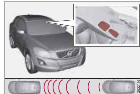
Laser sensor transmitter and receiver window.
