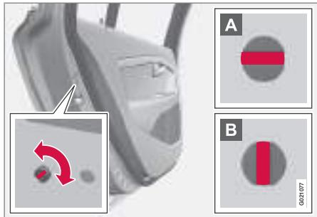
The child safety locks are located on the trailing edge of the rear doors and are only accessible when the doors are open.
