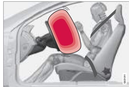
The car has an SRS airbag (Supplemental Restraint System) on the driver's side to supplement the protection afforded by the seatbelt. This airbag is fitted into the centre of the steering wheel. The steering wheel is marked **SRS AIRBAG**.
