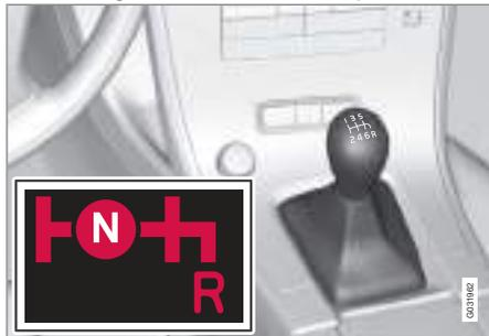
The reverse gear inhibitor prevents the possibility of mistakenly attempting to engage reverse gear during normal forward travel. Only engage reverse gear when the car is stationary.
