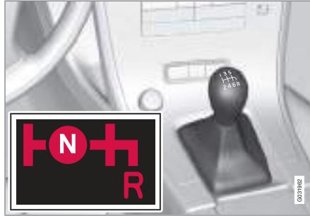
The reverse gear inhibitor prevents the possibility of mistakenly attempting to engage reverse gear during normal forward travel.
