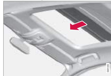
One long press on the lock button, see pages 43 (remote control key) and 50 (central locking button), closes the panorama roof and all the windows. The door mirrors are retracted\* and the doors and tailgate are locked. To interrupt closing, press the lock button again.
