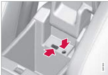
An iPod® or MP3 player can be connected to the car's infotainment system via the AUX socket or the USB connection in the centre console.
