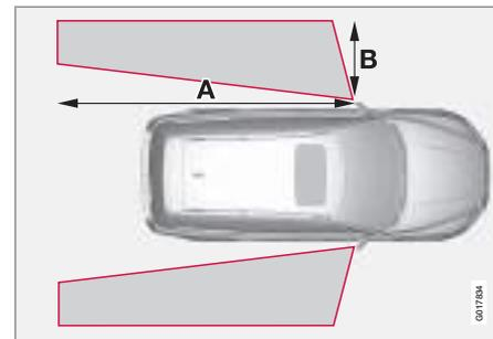
$A = \text{approx. } 9.5 \text{ m}$  and  $B = \text{approx. } 3 \text{ m}$
