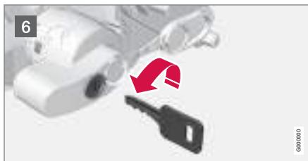
6 Turn the key anticlockwise to locked position. Remove the key from the lock.
