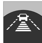
Five different time intervals can be chosen from and shown in the display as 1–5 horizontal lines – the more lines there are the longer the time interval.
