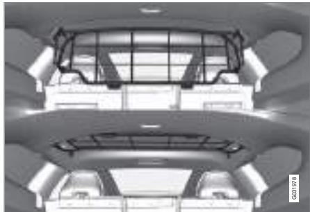
A safety grille prevents loads or pets from being thrown forward in the passenger compartment in the event of sudden braking. For safety reasons, the grille must always be mounted and secured correctly.
