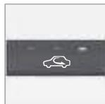
ETC - The right-hand orange light in the button illuminates when recirculation is engaged. The function is selected to shut out bad air, exhaust gases etc. from the passenger compartment. The air in the passenger compartment is recirculated, i.e. no outside air is taken into the car when this function is activated.
