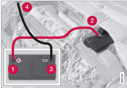
If the battery is flat then the car can be started with current from another battery.
