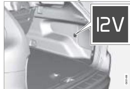
Fold down the cover to access the electrical socket. It works irrespective of whether or not the ignition is switched on.
