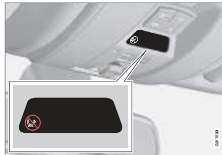
Indicator in the roof console showing that the passenger airbag is activated.
