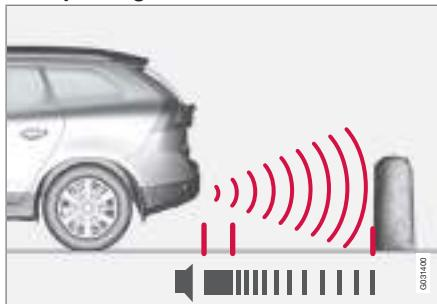
The distance covered to the rear of the car is about 1.5 metres. The acoustic signal for obstacles behind comes from the rear loudspeakers.
