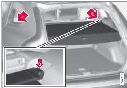
Pull the cargo cover over the load and hook it into the holes by the rear pillars in the cargo area.
