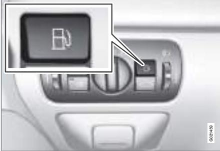
Open the fuel filler flap using the button on the lighting panel. The filler flap is located on the right-hand rear wing, as indicated by the symbol's
