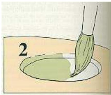
When the primer surface is dry, the paint can be applied using a brush.
