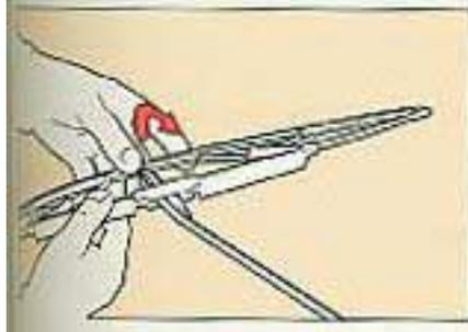
Install new blade, installation is the reverse of removal, and make sure that it is properly attached to the wiper arm.
