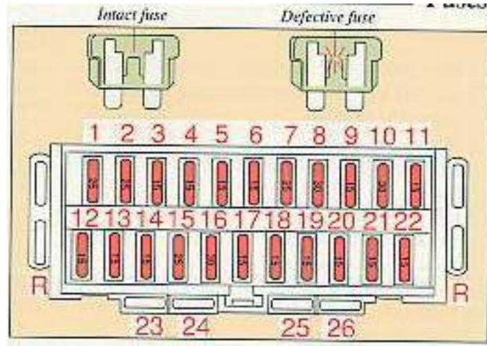
The fuses are removed by pulling them straight out. If they are defective, the metal wire is broken. When fitting a new fuse, be certain to use one with **the same amperage and color** as the one removed (see top of fuse)! Spare fuses are located on each side of the fusebox (1x15A, 1x25A, 1x30A).
