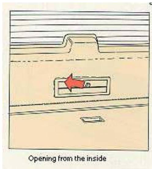
To open the tailgate from the inside of the vehicle, move the handle to the left and push outwards.
