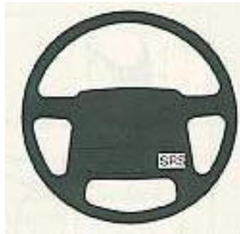
As an enhancement to the three-point seatbelt system, certain models are equipped with a Supplemental Restraint System (SRS). The Volvo SRS consists of a driver's side airbag with a driver's side knee bolster. The system is designed to supplement the protection provided by the three-point seatbelt system.
