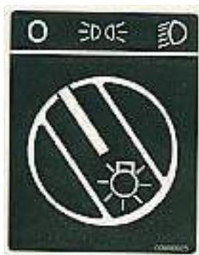
With the headlight switch in position ☐ the parking lights will stay on. Switch from high to low beams, and vice versa, by moving the turn signal switch lever on the left side of the steering column towards the steering wheel.
