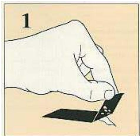
Remove loose flakes of paint with masking tape
