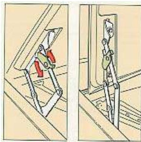
The normal opening angle for the hood is approximately 55°. By turning the catches or the hinges as illustrated, the hood can be opened to the vertical position. The catches will return to their normal positions when the hood is closed.
