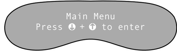
To return to the Main Menu press both function switches simultaneously.
