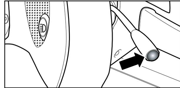
Should the vehicle become immobile or present a hazard to other road users, indicators may be operated in unison as a hazard warning. Depress button on the end of the indicator stalk to activate the hazard warning lights. Depress the button once again to deactivate the hazard warning lights.
