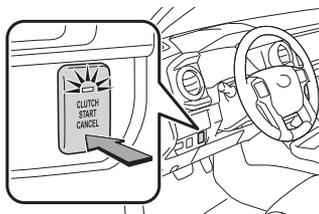
The engine switch must be in the "ON" position.
