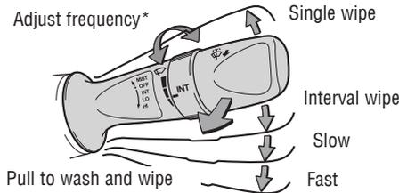
\* **Intermittent windshield wiper frequency adjustment** Rotate to increase/decrease wipe frequency.
