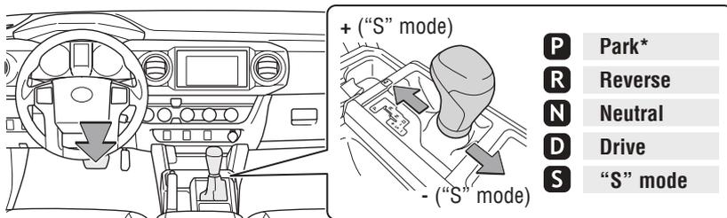
\* The engine switch must be in the "ON" position (without Smart Key) / "IGNITION ON" mode (with Smart Key) and the brake pedal depressed to shift from Park.
