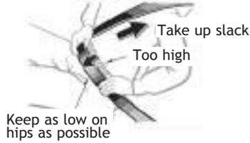
**NOTE:** If a passenger's seat belt is fully extended, then retracted even slightly, the Automatic locking retractor (ALR) will prevent it from being re-extended beyond that point, unless fully retracted again. This feature is used to help hold child restraint systems securely.
