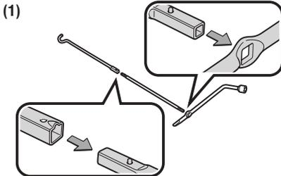
Insert the jack handle end into the lowering screw.
