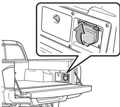
The power outlet can be used when the engine is running.
