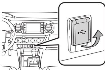
Connecting a compatible device and cable into the USB media port will support charging and music playback through the audio multimedia system.
