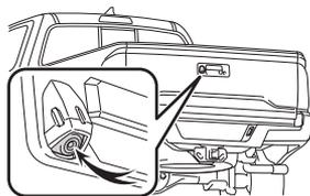
The rear view monitor system displays an image of the view from the bumper of the rear area of the vehicle. The camera for the rear view monitor system is integrated in the tailgate handle.
