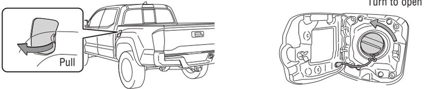
**NOTE:** Tighten until one click is heard. If the cap is not tightened enough, Check Engine “
