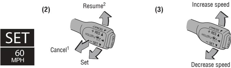
Vehicle will cruise at a set speed, decelerate to maintain selected distance from a slower vehicle traveling in front and accelerate back up to the selected speed if the vehicle in front changes lanes or speeds up.
