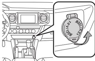
The engine switch must be in the “ACC” or “ON” position (without Smart Key) / “ACCESSORY” or “IGNITION ON” mode (with Smart Key) for use.
