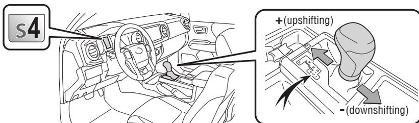
The initial shift range in "S" mode is set automatically to 5 or 4 according to vehicle speed.
