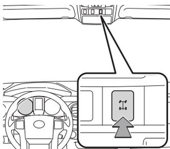
Use **ONLY** when wheel spinning occurs in a ditch, or on slippery or unpaved surfaces. **DO NOT USE THE REAR DIFFERENTIAL LOCK IN CONDITIONS OTHER THAN THOSE SPECIFIED IN THE OWNER'S MANUAL. UNLOCK THE DIFFERENTIAL ONCE THE VEHICLE MOVES OUT OF THE TROUBLE SPOT.**
