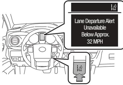
Press the LDA switch to turn the LDA system on. Depress again to turn it off.
