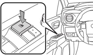
**Automatic down (type A)/up or down (type B) operation** Push the switch completely down or pull it completely up and release to fully open or close. To stop the window partway, operate the switch in the opposite direction.
