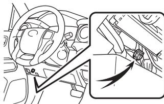
Use service connector for the trailer brake controller.
