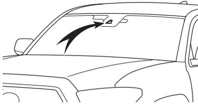
LDA in TSS-P uses an in-vehicle camera designed to detect visible white and yellow lane markers in front of the vehicle and the vehicle’s position on the road. If the system determines that the vehicle is starting to unintentionally deviate from its lane, the system alerts the driver with an audio and visual alert. When the alerts occur, the driver must check the surrounding road situation and carefully operate the steering wheel to move the vehicle back to the center part of their lane.
