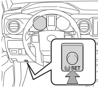
After adjusting tire pressures, or after tires have been rotated or replaced, turn the ignition switch to “ON” and press and hold the “
