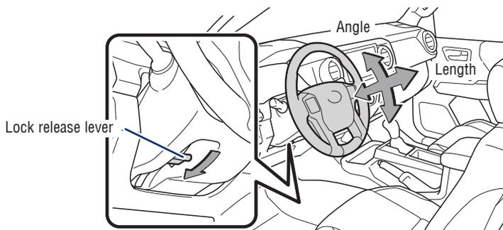
Hold wheel, push lever down, set angle and length, and return lever.
