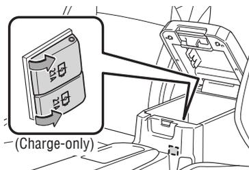
The engine switch must be in the "ACC" or "ON" position (without Smart Key) / "ACCESSORY" or "IGNITION ON" mode (with Smart Key) for use.
