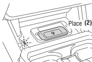
Place device nearest the center of charging area for best results. Moving device may result in stopping or restarting the charging process.
