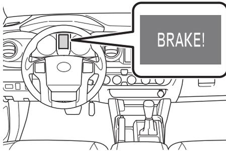
The Pre-Collision System uses a radar sensor and camera sensor to help detect a vehicle or pedestrian in front of your vehicle.
