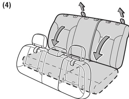
Pull lock release strap and fold down the seatback.
