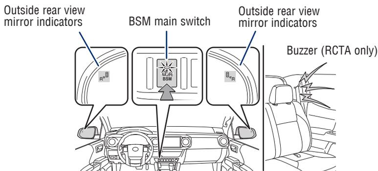
**The Blind Spot Monitor is a system that has two functions:**
