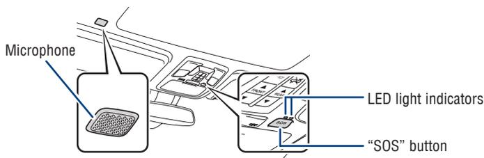
Safety Connect is a subscription-based telematics service that uses Global Positioning System (GPS) data and embedded cellular technology to provide safety and security features to subscribers. Safety Connect is supported by Toyota's designated response center, which operates 24 hours per day, 7 days per week.
