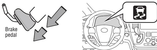
HAC helps prevent rolling backwards on an incline. To engage, push the brake pedal farther down while at a complete stop until a beep sounds and slip indicator illuminates. HAC holds for approximately 2 seconds after releasing brake pedal.
