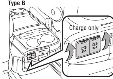
The ignition/"ENGINE START STOP" switch must be in "ACC" or "ON"/ACCESSORY or IGNITION ON position for use.
