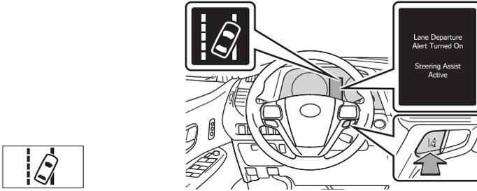
Press the LDA switch to turn the LDA system on. Depress again to turn it off.
