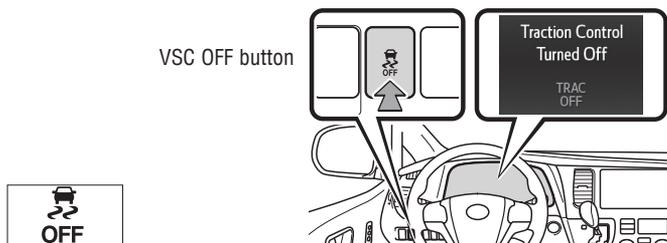
The VSC OFF switch can be used to help free a stuck vehicle in surroundings like mud, dirt or snow. While the vehicle is stopped, press switch to disable the TRAC system.
