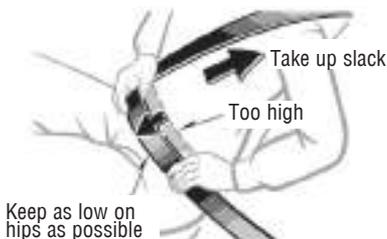
**NOTE:** If a passenger's seat belt is fully extended, then retracted even slightly, the Automatic locking retractor (ALR) will prevent it from being re-extended beyond that point, unless fully retracted again. This feature is used to help hold child restraint systems securely.
