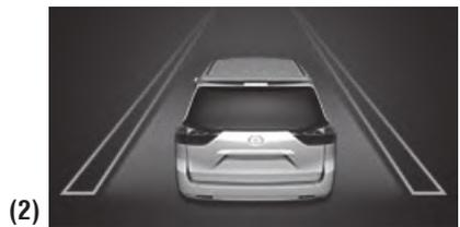
The LDA function
