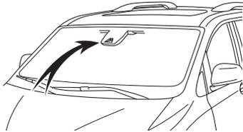
LDA in TSS-P uses an in-vehicle camera designed to detect visible white and yellow lane markers in front of the vehicle and the vehicle's position on the road. If the system determines that the vehicle is starting to unintentionally deviate from its lane, the system alerts the driver with an audio and visual alert. When the alerts occur, the driver must check the surrounding road situation and carefully operate the steering wheel to move the vehicle back to the center part of their lane.
