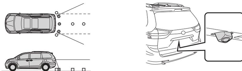
The rear view monitor system displays an image of the view from the bumper of the rear area of the vehicle. The camera for the rear view monitor system is located above the license plate.
