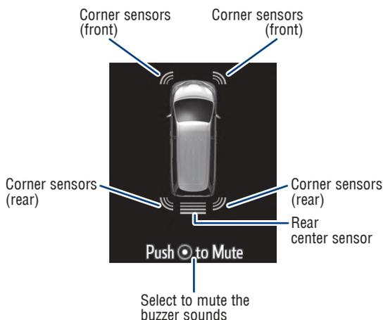
The parking assist sonar system operates when the vehicle approaches an obstacle. The distance from your vehicle to nearby obstacles when parallel parking or maneuvering into a garage is measured by sensors and communicated via the Multi-Information Display (MID), the navigation system screen and audible beeps.
