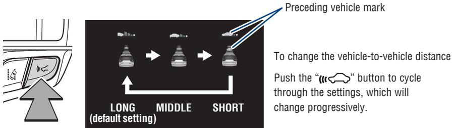
This mode employs a radar sensor to detect the presence of vehicles up to approximately 328 ft (100 m) ahead, determines the current vehicle-to-vehicle following distance and operates to maintain a preset following distance from the vehicle ahead. These distances vary based on vehicle speed.
