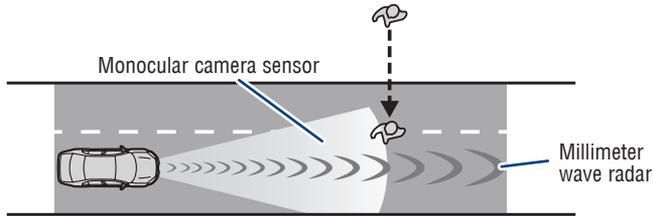
As part of the Pre-Collision System, this function is also designed to first provide an alert and then automatic braking if needed.
