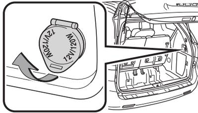
The ignition/"ENGINE START STOP" switch must be in "ACC" or "ON"/ACCESSORY or IGNITION ON position for use.
