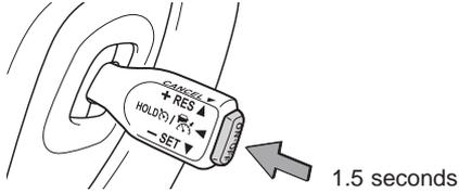
If you are already using DRCC “
