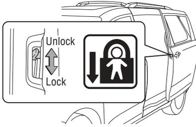
Moving the lever downward will allow the door to be opened only from the outside.
