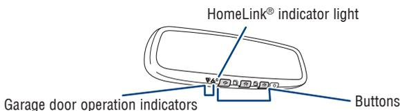
Garage door openers manufactured under license from HomeLink®\* can be programmed to operate garage doors, estate gates, security lighting, etc.
