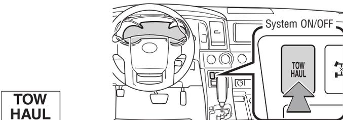
"TOW/HAUL" mode can be used when carrying or towing heavy loads. As fuel economy is reduced while in "TOW/HAUL" mode, deactivating when driving without a load is recommended.
