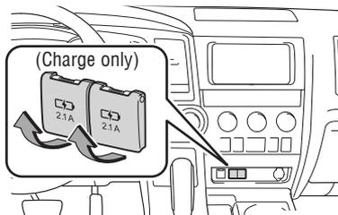
The engine switch must be in the "ACCESSORY" or IGNITION ON mode for use.
