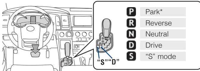
\* The engine switch must be in the "IGNITION ON" mode and the brake pedal depressed to shift from Park.
