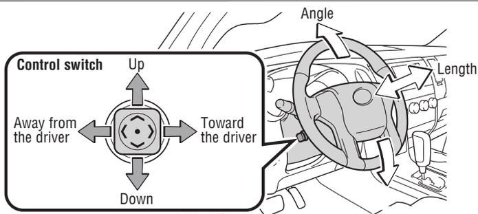
Toggle the control switch to set angle and length.
