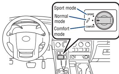
AVS controls the suspension according to the road and driving conditions. Selecting an optimum driving mode allows good vehicle posture and steering wheel operation.
