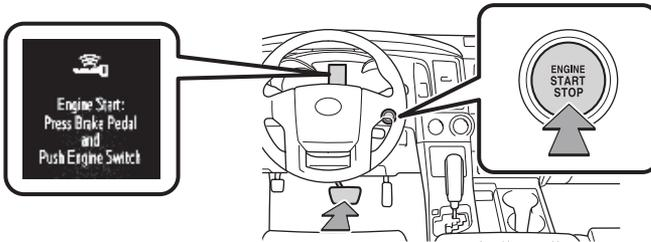
**NOTE:** The Smart Key must be carried to enable the start function. With the gear shift lever in Park and the brake pedal depressed, push the “ENGINE START STOP” switch.
