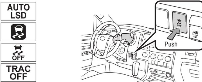
The VSC OFF switch is used to switch between modes related to the TRAC, VSC and AUTO LSD functions.
