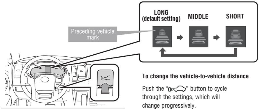
This mode employs a radar sensor to detect the presence of a preceding vehicle up to approximately 328 ft (100 m) ahead, determines the current vehicle-to-vehicle following distance and operates to maintain a preset following distance from the vehicle ahead. These distances vary based on vehicle speed.
