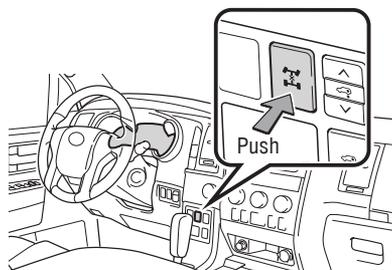
Lock the center differential if the vehicle's wheels get stuck in a ditch or when driving on a slippery or bumpy surface.
