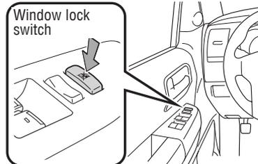
**Automatic operation (front windows only)** Push the switch completely down or pull it completely up and release to fully open or close. To stop window partway, lightly push the switch in the opposite direction.
