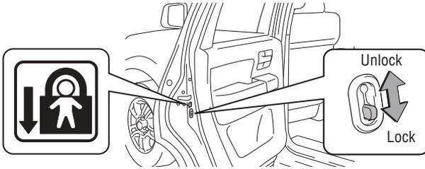
Moving the lever downward will allow the door to be opened only from the outside.
