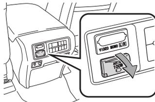
The engine switch must be in the “IGNITION ON” mode for use.
