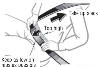
**NOTE:** If a passenger’s seat belt is fully extended, then retracted even slightly, the Automatic locking retractor (ALR) will prevent it from being re-extended beyond that point, unless fully retracted again. This feature is used to help hold child restraint systems securely.
