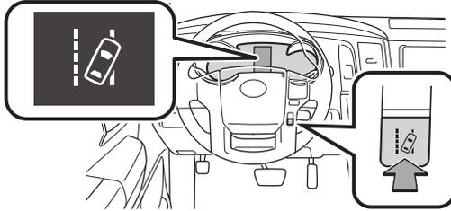
Press the LDA switch to turn the LDA system on. Depress again to turn it off.
