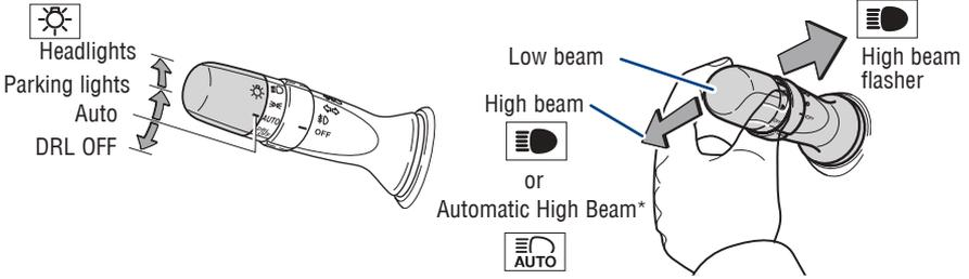
**Daytime Running Light system (DRL)** Automatically turns on under certain conditions to make vehicle more visible to other drivers. Not for use at night.
