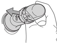
\* **Intermittent windshield wiper frequency adjustment** Rotate to increase/decrease wipe frequency.
