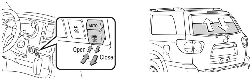
**Automatic operation** Push the switch completely in or pull it completely out and release to fully open or close. To stop window midway, lightly push the switch in the opposite direction.
