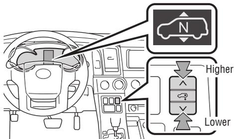
Vehicle height can be adjusted only when the engine is running.
