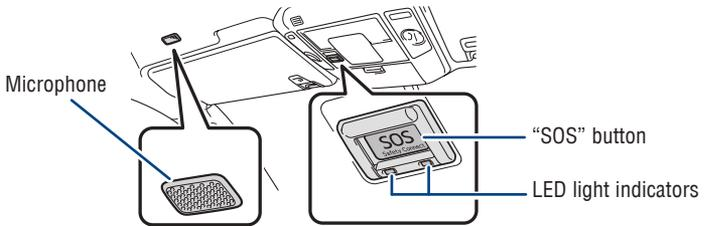
Safety Connect is a subscription-based telematics service that uses Global Positioning System (GPS) data and embedded cellular technology to provide safety and security features to subscribers. Safety Connect is staffed with live agents at the Toyota response center, which operates 24 hours per day, 7 days per week.
