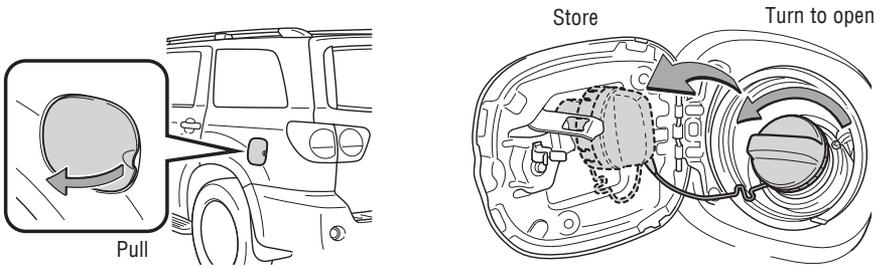
**NOTE:** To close, tighten until one click is heard. If the cap is not locked or tightened, Check Engine “
