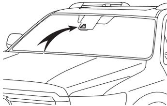
LDA in TSS-P uses an in-vehicle camera designed to detect visible white and yellow lane markers in front of the vehicle and the vehicle's position on the road. If the system determines that the vehicle is starting to unintentionally deviate from its lane, the system alerts the driver with an audio and visual alert. When the alerts occur, the driver must check the surrounding road situation and carefully operate the steering wheel to move the vehicle back to the center part of their lane.
