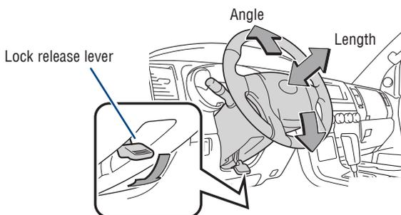
Hold wheel, push lever down, set angle and length and return lever.
