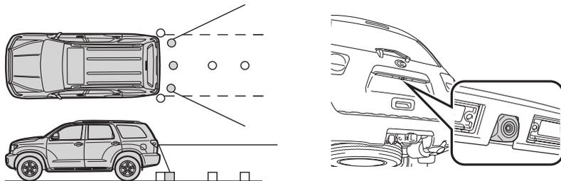
The rear view monitor system displays an image of the view from the bumper of the rear area of the vehicle. The camera for the rear view monitor system is located above the license plate.
