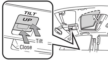
Lightly press either side of the moonroof switch while opening/tilting is in progress, the moonroof stops partway.
