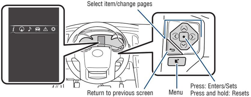
Use the meter control switches on the steering wheel to scroll through the following information screens:
