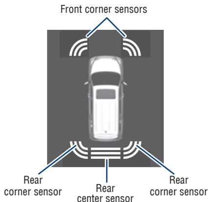
The parking assist sonar system operates when the vehicle approaches an obstacle. The distance from your vehicle to nearby obstacles when parallel parking or maneuvering into a garage is measured by sensors and communicated via the Multi-Information Display (MID) and audible beeps.
