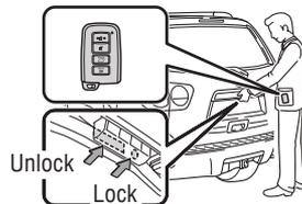
\* Driver door unlocking function can be programmed to unlock driver door only, or all doors. Grasping passenger door handle will unlock all doors.
