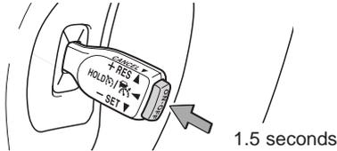
If you are already using DRCC
