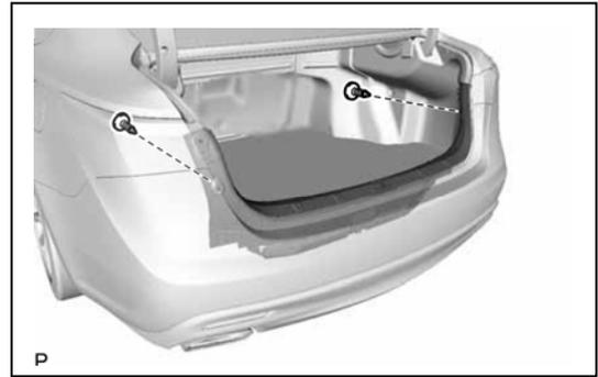
(2) Disengage the 4 clips and 3 guides to remove the rear floor finish plate as shown in the illustration.
