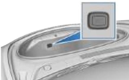
Press the interior release button to open the front trunk, then push up on the hood.
