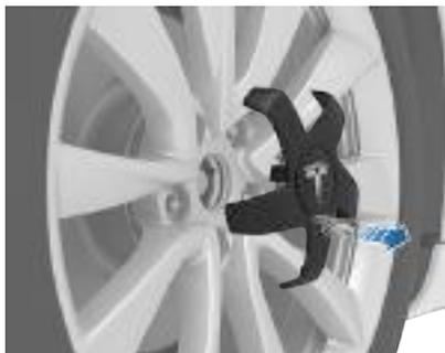
To install the lug nut cover, align it into position and push firmly until it fully snaps into place.
