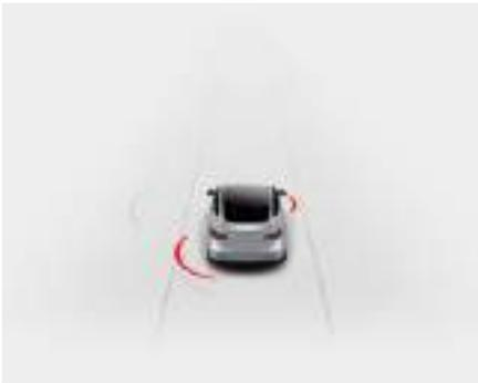
Lane Assist also warns you of undesired lane departures by vibrating the steering wheel slightly if a front wheel passes over a lane marking and the associated turn signal is off. This warning is active only when driving between approximately 36 and 90 mph (59 and 150 km/h). To turn this warning on or off, touch **Controls > Autopilot > Settings > Lane Departure Warning**. Your chosen setting is retained until you manually change it.
