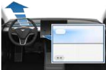
You can toggle between having the air flow from the vent in a single direction (represented on the control grid by an oblong shape) or in two mirrored directions (represented on the control grid by two circles). To do so, touch the combine/split icon. The icon changes based on whether air flow is combined or split.
