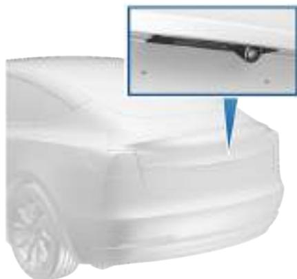
Whenever you shift into Reverse, the touchscreen displays the view from the camera. Lines show your driving path based on the position of the steering wheel. These lines adjust appropriately as you move the steering wheel.
