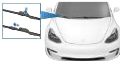
4. If necessary, temporarily place a towel between the wiper arm and windshield to avoid scratching the windshield.
