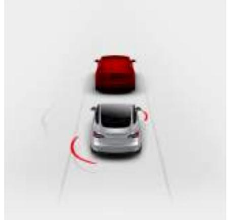
Warnings cancel automatically when the risk of a collision has been reduced (for example, you have decelerated or stopped Model 3, or the object in front of your vehicle has moved out of your driving path).
