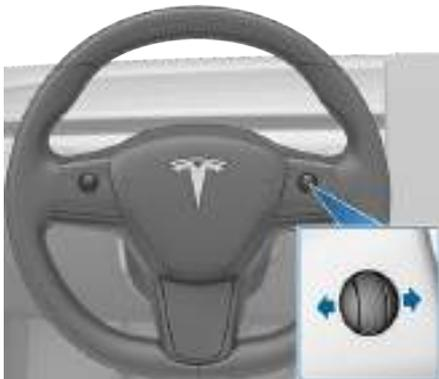
To display and adjust the setting for the following distance on the touchscreen at any time, touch **Controls** > **Autopilot** > **Cruise Follow Distance**. Adjust the following distance by touching plus (+) or minus (-) buttons.
