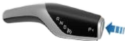
**Note:** The parking brake operates on the rear wheels only, and is independent of the pedal-operated brake system.
