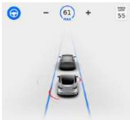
**Note:** To initiate Autosteer when there is no vehicle in front of you, you must be driving at least 18 mph (30 km/h) on a roadway with visible lane markings. If a vehicle is detected ahead of you, you can initiate Autosteer at any speed, even when stationary (if you are at least 5 feet (150 cm) away from the vehicle).
