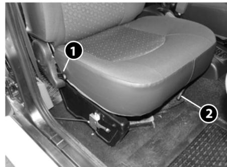
1. Seat backrest inclination adjustment lever
