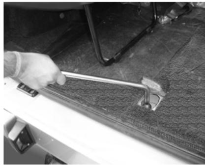
*Loosening/Tightening of wheel winch screw*
