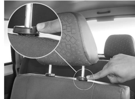
*Release Button for Head rest height adjustment*
