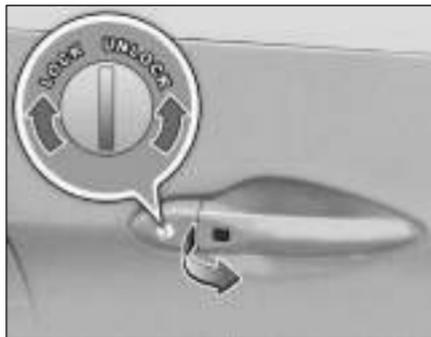
Insert the key and turn it clockwise to lock and anticlockwise to unlock the door.
