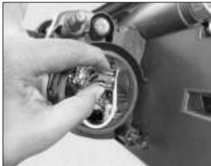
3. Unlock high beam bulb holder clip, by pulling it backward.
