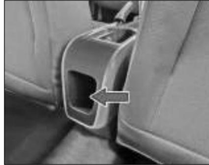
Stowage for Rear passenger is provided on rear side of floor console between the front passenger seats. It can be used to keep mobile charger and small items.
