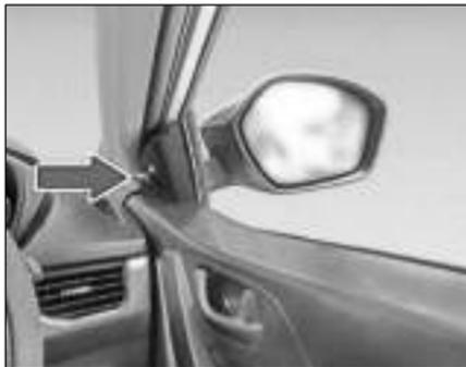
You can adjust the outer rear view mirrors manually by joy stick knob located in the driver's and front passenger's door panel.
