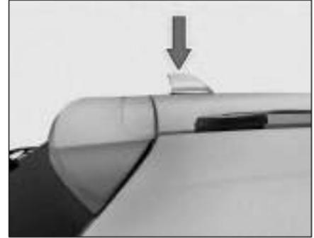
Shark FIN antenna is provided on the roof at rear end.
