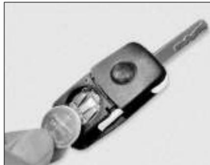
5. Ensure that the “+” symbol on the battery is facing upwards. The correct polarity is shown on the battery cover.
