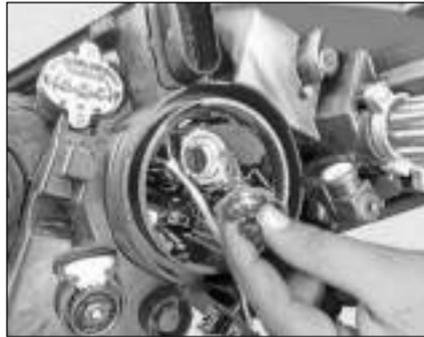
6. Insert the new bulb (without touching the glass) into the socket.
