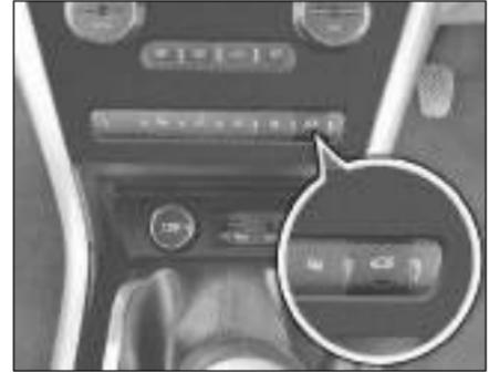
To open the Tail gate, press the switch located on fascia switch.
