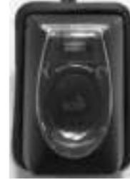
The emergency switches are provided inside the vehicles. It shall be pressed by the driver or any occupant in emergency like accidents, medical emergencies & or Law & order situations. If the occupant feels threatened or unsafe, then also this can be used
