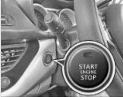
Start/Stop switch is provided on the dashboard towards the left side of steering wheel.
