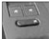
When switch is pressed, red light turns 'ON'. The individual switches provided on rear and front passenger door can be operated. It can also be operated from the switches on driver's arm rest.
