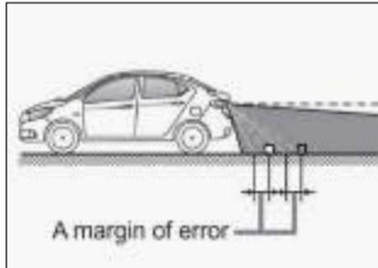
When any part of the vehicle sags due to the number of passengers or the distribution of the load, there is a margin of error between the fixed guide lines on
