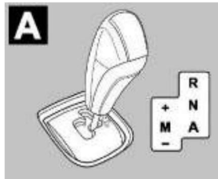
Auto mode will be engaged only when vehicle is stationary and brake pedal pressed. An audio signal indicates when Automatic gear is engaged.
