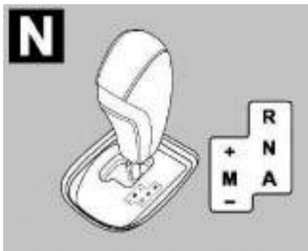
Vehicle is in neutral gear position. This will be indicated
