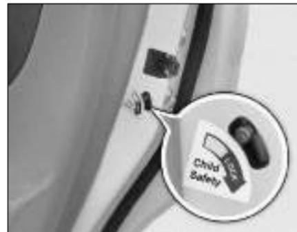
Both the rear doors of the vehicle are provided with a child proof lock. Push the lock lever located on vertical face of the door downward before closing the door. The door which has been locked by activating the child lock cannot be opened from inside, it can be opened only from the outside.
