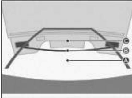
Visually check the surroundings and the area behind the vehicle. On the screen, it appears that a truck is parked at point B. However, in reality if you back up to point A, you will hit the truck. On the screen, it appears that A is closest and C is furthest away. However, in reality, the distance to A and C is the same, and B is farther than A and C.
