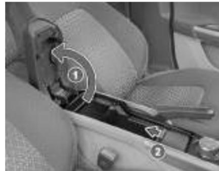
Tambour door is provided on center console. To access Tambour door, lift arm rest (1). Slide the shutter (2) to open and close the stowage area.
