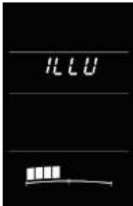
For Instrument Cluster illumination level settings, it is necessary to turn the Park Lamp 'ON' and then Press the 'SET' knob on Instrument Cluster.
