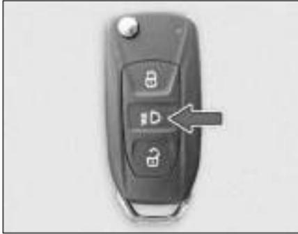
Remote operated Tail gate unlatching can be done through long press (2 sec) approach light button on remote key.
