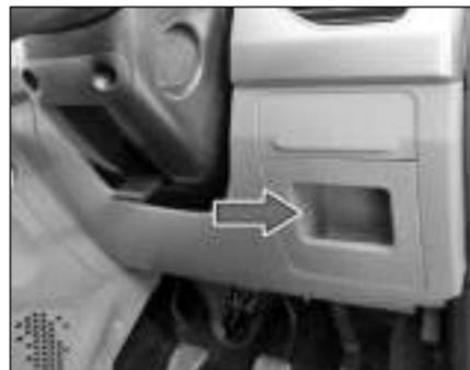
2. To remove the cover, gently pull the cover from bottom side such that the lugs get disengaged.
