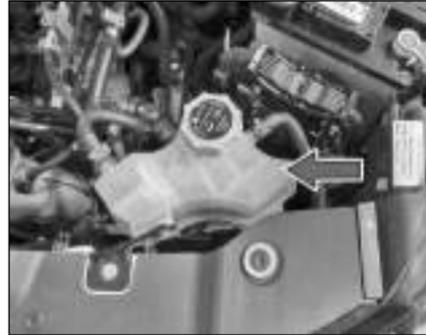
Check whether the coolant level is between the 'MIN' and 'MAX' marks provided on the coolant reservoir.
