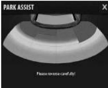
There are 4/3 ultrasonic sensors placed on the rear bumper of the vehicle. Once
