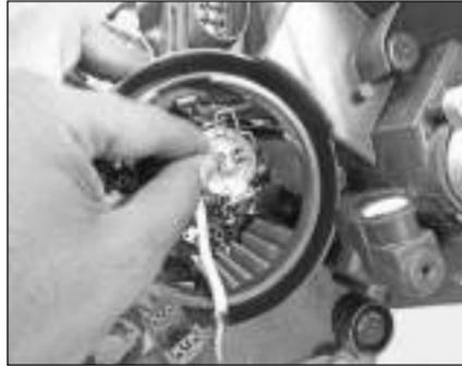
5. Pull out the bulb from the socket.
