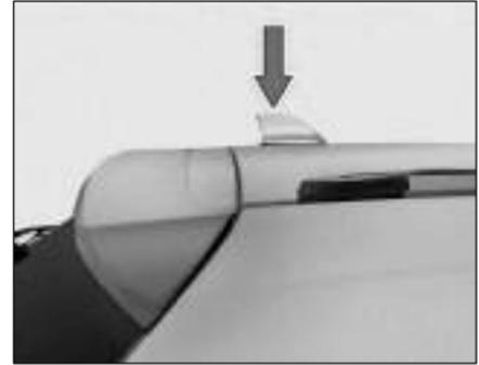
Shark FIN antenna is provided on the roof at rear end.
