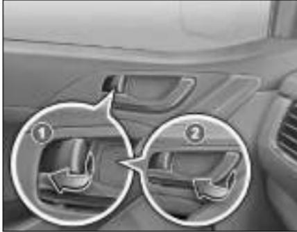
All doors can be opened from inside. To open, pull the door opening knob (1) and then lever (2).
