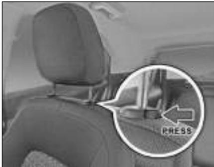
Adjust the head restraint so that it is as close to the head as possible and the center of the head restraint supports the back of the head at eye level. This will reduce the potential for injury to the head and neck in the event of an accident or similar situation.
