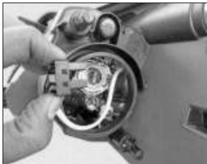
4. Remove high beam bulb.
