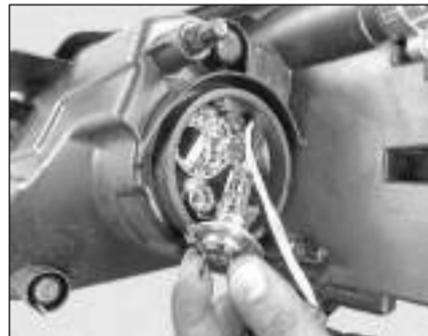
5. Refit high beam bulb by locking high beam bulb holder clip.
