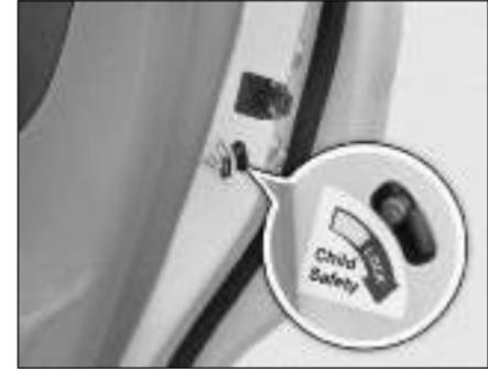
Both the rear doors of the vehicle are provided with a child proof lock. Push the lock lever located on vertical face of the door downward before closing the door. The door which has been locked by activating the child lock cannot be opened from inside, it can be opened only from the outside.
