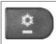
Press the switch to activate / deactivate the AC. The indicator lamp in the button will light up when climate control is activated.
