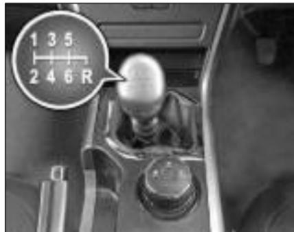
The gearshift pattern is as shown on the gear lever knob. Gear shifting should always be done with clutch pedal pressed
