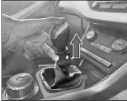
For engaging reverse gear, lift the latch and keeping latch lifted, shift to reverse position.
