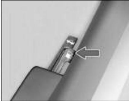
To unlatch the fuel flap, pull the lever located at the right hand side below the driver seat.
