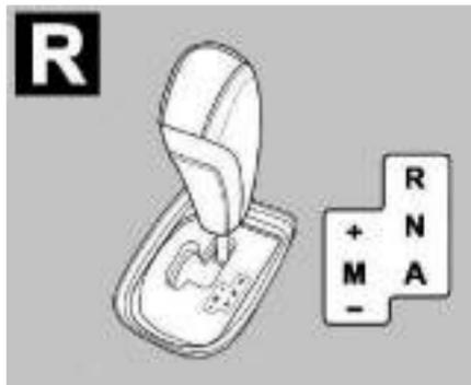
Reverse gear will be engaged only when vehicle is stationary and brake pedal pressed. An audio signal indicates when reverse gear is engaged.
