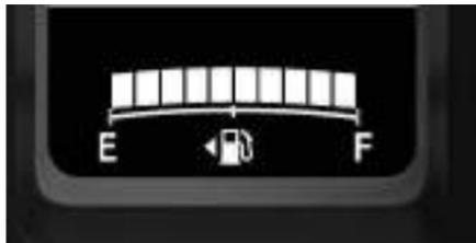
When fuel in the tank is near to empty position, low fuel warning Tell tale turns ‘ON’. Refill the tank as soon as possible.
