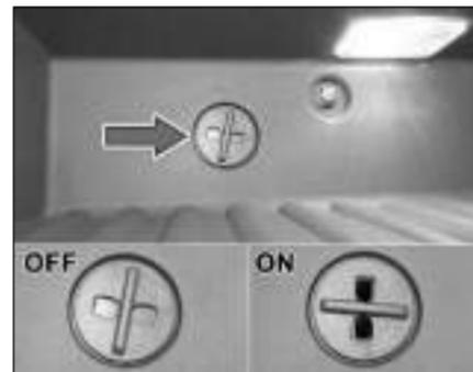
On selected models glove box is provided with a cooling facility. It cools the glove box only when the front A/C is ON. Shut OFF the vent by rotating the knob, whenever cooling is not required.
