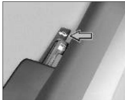
To open the Tail gate, pull the lever located at the right hand side below the driver's seat and lift the Tail gate.
