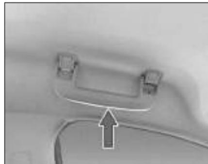
Roof grab handles are provided on all seats except driver's seat. This helps in comfortable positioning of passengers during a journey.
