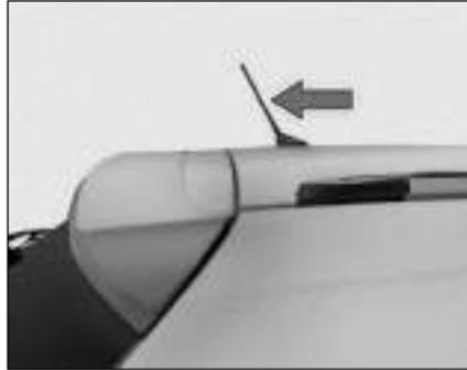
Antenna is located on the roof. Turn antenna anticlockwise to remove from vehicle, if required.
