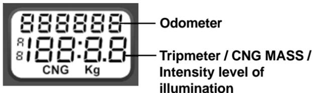
The speedometer indicates the car speed in km/hr. The odometer records the total distance the car have been driven. The tripmeter can be used to measure the distance travelled on each trip or between fuel fillings.
