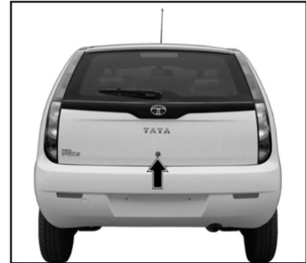
It can also be opened by using door key. The lock is located on the trunk lid.
