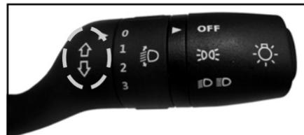
**A. Right turn signal :** Right indicator lamps and instrument cluster tell tale will come 'ON' if ignition is 'ON' and
