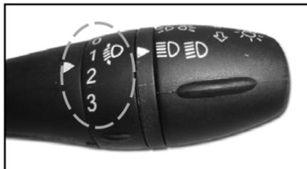
Inner rotary switch on right hand stalk is provided for head lamp leveling. Setting is done by rotating the knob to select one of the 3 level positions depending upon the loading of the car. Head lamp leveling can be done with head lamp in Low Beam and in ON position.
