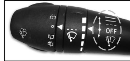
Pull the stalk upwards to operate intermittent wipe (- - -), Slow wipe (—) or fast wipe (—). Pull the stalk down for wipe and wash. Pull towards driver for Flick Wipe (spring return).
