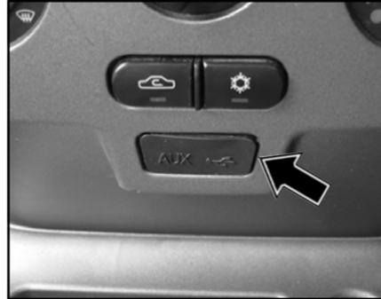
**USB** and **AUX** Ports are provided just below the HVAC controls on the centre console.
