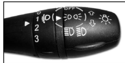
Position (Parking) lamp and tail lamp will be ON in this position.
