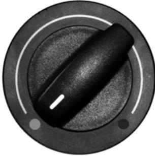
The air temperature in the car can be controlled by operating the temperature control knob (B) on the control panel. The temperature can be increased by rotating the knob towards the red segment and decreased by rotating it towards the blue segment.
