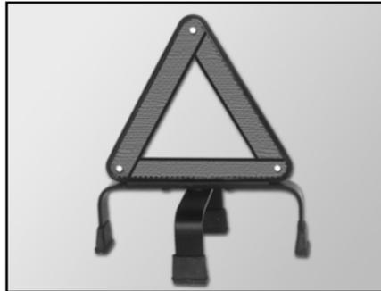
An advance warning triangle is kept inside the pocket provided behind the rear seat back rest.
