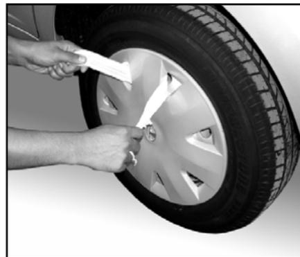
Insert a piece of cloth between the spokes of the wheel cover and pull cover outward.
