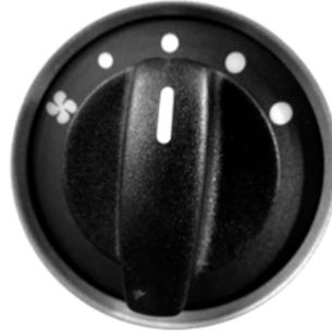
The HVAC system has a four speed blower. The blower speeds can be regulated by operating the blower knob (C) at the centre of the control panel.
