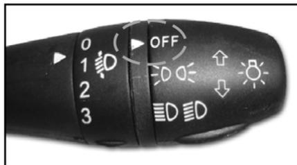
Head lamp, position (Parking) lamp and tail lamp will be OFF in this position.
