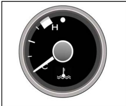
The engine coolant temperature gauge indicates the approximate coolant temperature. If the coolant temperature reading is very high or if the high coolant temperature indicator comes ON, reduce the car's speed and switch OFF the AC.
