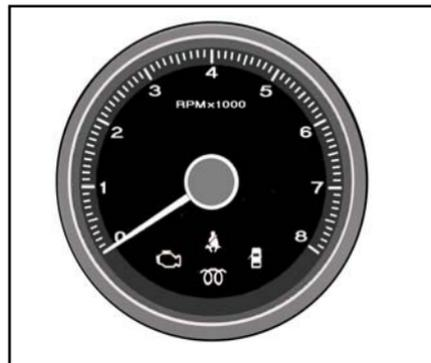
This meter indicates the engine rpm. Change the gears at appropriate engine rpm and speed to get good fuel economy and driving pleasure. Do not increase the engine rpm unnecessarily.
