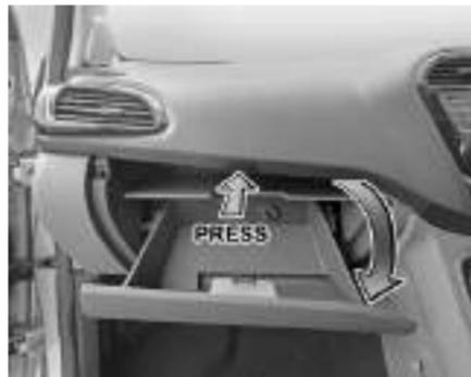
**To open** - Press the knob and open the glove box flap.
