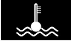
When the ignition switch is in the “ON” position, this gauge indicates the engine coolant temperature. The indicator should stay within the normal, acceptable temperature range between “H” and “C”. If the indicator approaches “H”, overheating is indicated by red LED bar.
