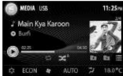
Also, when the display is not in climate mode then climate information will be displayed on the all-time display provide on the bottom bar.
