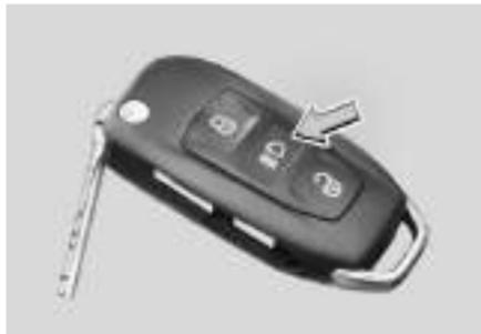
trunk lid opening can be done through long press (4 sec) approach light button on remote key.
