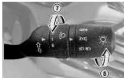
Inner rotary switch on right hand stalk is provided for head lamp leveling. With the inner rotary switch, Head lamp leveling can be done with head lamp in Low Beam and in 'ON' position. Select correct position before start of trip and vehicle is stationary. Depending upon the number of passengers and luggage in the vehicle headlamp focus may change. This can be adjusted by rotating the knob to one of the 3 level positions.
