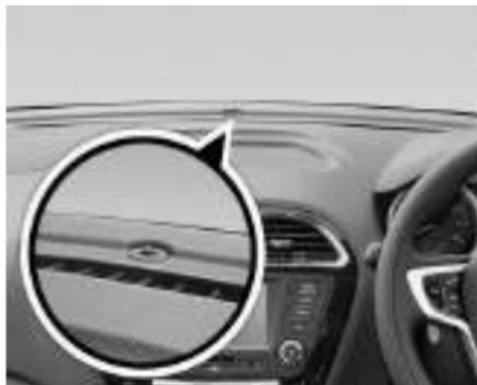
2. In-car sensor on control panel.
