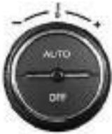
Turning the temperature control knob clockwise increases the temperature of the air. The desired temperature will be increased by steps of 0.5°C. User can select temperature range from 18°C to 30°C. Whereas the anticlockwise direction decreases the temperature.
