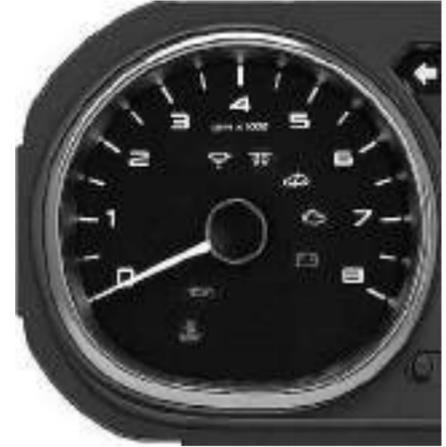
Tachometer indicates engine speed in revolutions per min (rpm).
