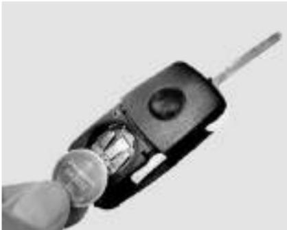
5. Ensure that the “+” symbol on the battery is facing upwards. The correct polarity is shown on the battery cover.
