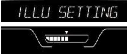
For Instrument Cluster illumination level settings, it is necessary to turn the Park Lamp 'ON' and then Press the 'SET' knob on Instrument Cluster.
