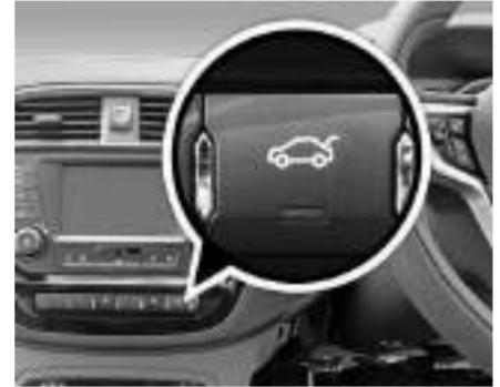
To open the trunk lid, press the switch located on fascia switch.
