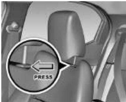
Adjust the head restraint so that it is as close to the head as possible and the center of the head restraint supports the back of the head at eye level. This will reduce the potential for injury to the head and neck in the event of an accident or similar situation.
