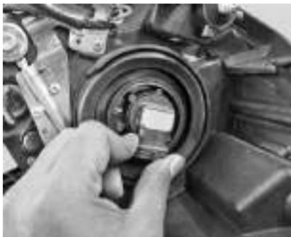
10. Remove position high beam bulb
