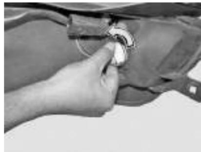
Replace with the new bulb (refer bulb specification table) and refit it by pressing and turning it in clockwise direction firmly into the socket.
