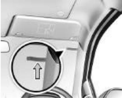
Tag holder is provided near the front windshield for ease of displaying toll, parking tickets, ID's, passes, labels etc.
