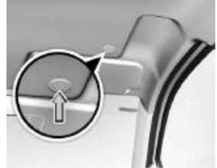
A mic is provided on roof interior above driver seat position.
