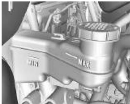
The level of the brake fluid should be between the 'MIN' and 'MAX' marks on the side of the brake fluid container. If the level falls below the 'MIN' mark, add recommended brake fluid.
