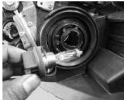
11. Refit position high beam bulb.
