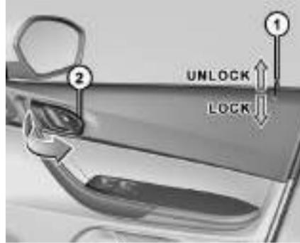
All the doors can also be locked from inside by pressing knob (1) on driver door and independently on other doors respectively.
