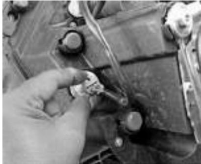
15. Unlock side indicator lock in anti-clockwise direction & remove front direction indicator bulb.
