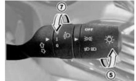
Inner rotary switch on right hand stalk is provided for head lamp leveling. With the inner rotary switch, Head lamp leveling can be done with head lamp in Low Beam and in 'ON' position. Select correct position before start of trip and vehicle is stationary. Depending upon the number of passengers and luggage in the vehicle headlamp focus may change. This can be adjusted by rotating the knob to one of the 3 level positions.
