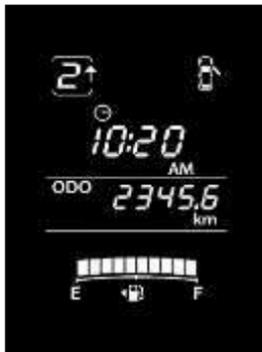
Digital clock appears on the DIS screen. To adjust the values in Hrs. Min. and AM/PM mode, Press 'SET' knob on Instrument Cluster. A delayed press on the 'SET' knob for selected value will confirm it and move towards next respective value.
