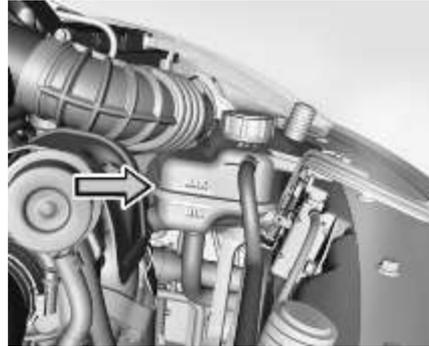
Check whether the coolant level is between the 'MIN' and 'MAX' marks on the coolant reservoir.
