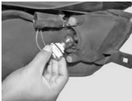
Replace with the new bulb (refer bulb specification table) and refit it by pressing and turning it in clockwise direction firmly into the socket.
