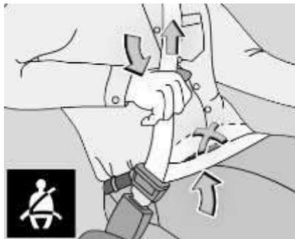
6. To unlatch the belt, press the red button on the buckle. Guide the belt to the pillar as it retracts.
