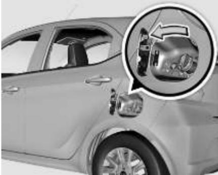
To open the fuel flap, pull the lever (2) located at the right hand side of the driver on floor. Open the fuel cap by turning it in counter clockwise direction for fuel filling.
