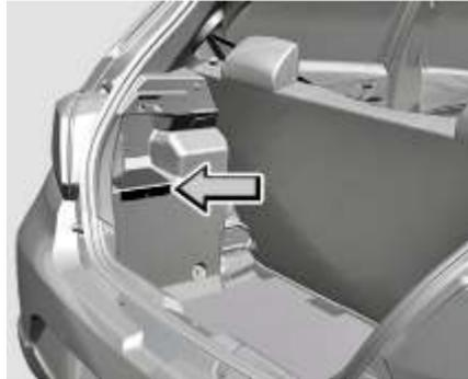
Tool kit & tow hook are provided in bag. This bag is stowed inside LH side pocket of luggage compartment.
