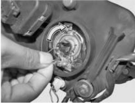
7. Refit the connector into the bulb and press the rubber cover on headlamp housing to fit it properly.
