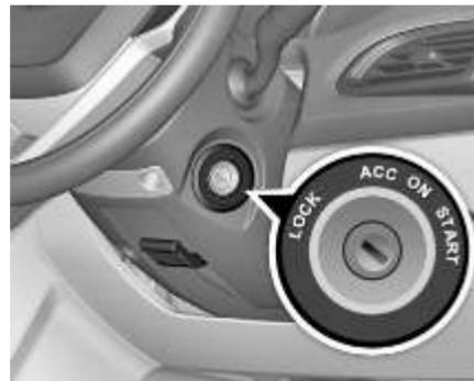
The ignition switch has the following four positions:
