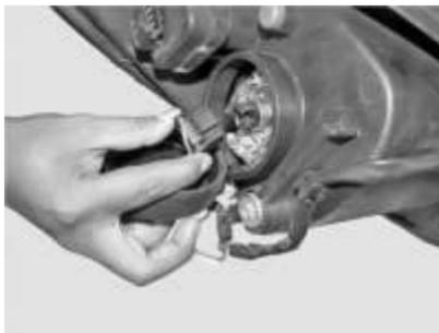
3. To free the headlamp bulb from the socket, press and swing the retaining spring and pull it straight back.
