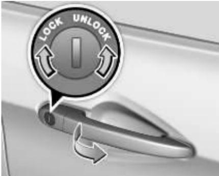
Insert the key and turn it clockwise to lock and counter clockwise to open the door.
