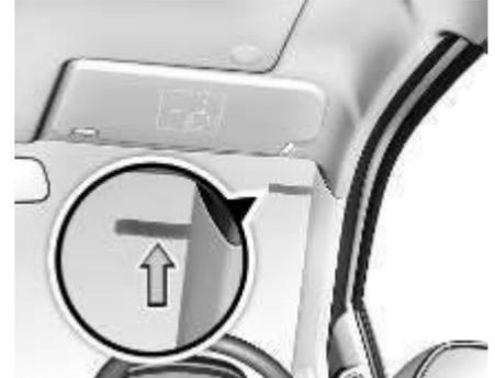
Tag holder is provided near the front windshield for ease of displaying toll, parking tickets, ID's, passes, labels etc.
