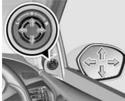
The switch to adjust the motorized mirrors is located on the driver's door. You can adjust the mirrors when the ignition switch is in the "ACC" or "ON" position.
