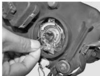
4. Pull out the bulb from the socket.
