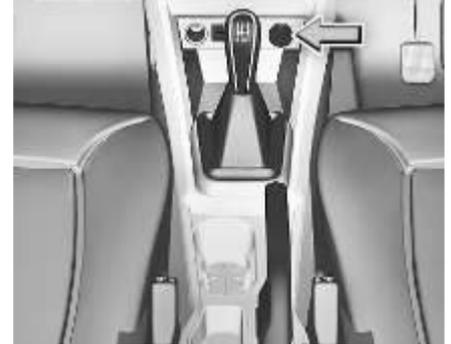
The power socket will work when the ignition switch is in the "ACC" or "ON" position. This socket can be used to provide 12V (10A) power for electrical accessories.
