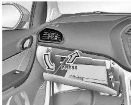
**To open** - Press the knob and open the glove box flap.
