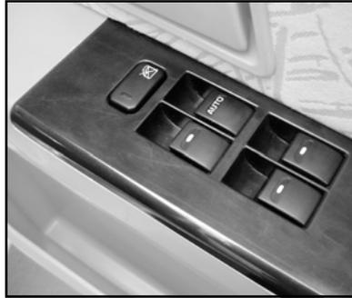
still be operated by using the switches on the console. Illumination on the rear window switch goes off when the switch is in locked condition. Press down the lock button to unlock. Individual window winding switches have been provided only on other doors.
