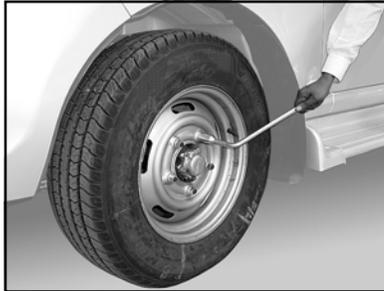
Set the jack properly at correct jack point as shown for front or rear wheel and slowly lift the vehicle with the help of jack handle.
