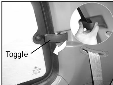
Butterfly windows are provided on both rear sides of vehicle to provide ventilation for 3rd row occupants when required. Pull the toggle to unlock and open the window. For
