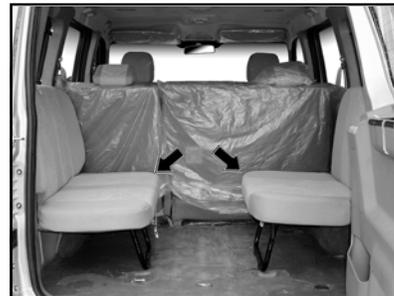
In this there are two options, 7-Seater and 9-seater. In the 7-seater option, two occupants can be accommodated and in 9-seater option, four occupants can be accommodated in the rear most part of the vehicle.
