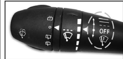
Pull the stalk upwards to operate intermittent wipe (---), Slow wipe (—) or fast wipe (—). Pull the
