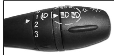
Head lamp, position (Parking) lamp and tail lamp will be ON in this position. Toggling the lever (Stalk)
