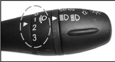
Inner rotary switch on right hand stalk is provided for head lamp leveling. Setting is done by rotating the knob to select one of the 3 level positions depending upon the loading of the vehicle. Head lamp leveling can be done with head lamp in Low Beam and in ON position.
