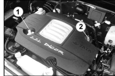
1. Engine oil filling cap 2. Dip Stick
