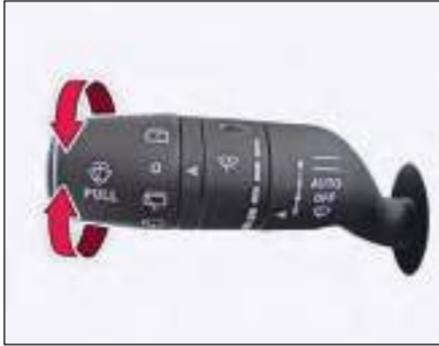
Turn the outer rotary knob such that it aligns its position
