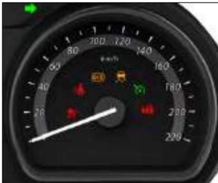
Speedometer indicates the actual vehicle speed in km/h.
