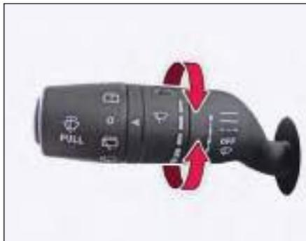
Inner rotary switch on left hand stalk is provided for intermittent front wiper delay. The switch has 5 delay timers.
