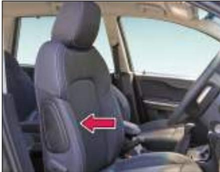
Front side impact air bags deploy next to the outer bolster of the seat backrest.
