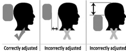
Adjust the head restraint so that it is as close to the head as possible and the center of the head restraint supports the back of the head at eye level. This will reduce the potential for injury to the head and neck in the event of an accident or similar situation.
