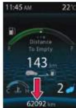
Odometer indicates total distance traveled by vehicle up to 999999 km with the resolution of 1 km.
