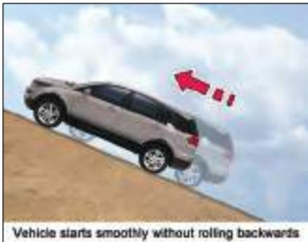
Hill Hold Control allows easy starting up the hill without the risk of unwanted rolling backwards. It is activated automatically when driving off up-hill on an inclined surface after the driver has released the brake pedal.
