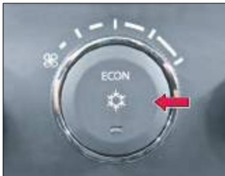
During ECON A.C. operation the system automatically cuts off at a higher temperature than normal A.C. The operation can be used during mild weather conditions for better fuel efficiency. Comfort level may be compromised during this operation.
