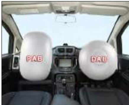
Driver's air bag (DAB) deploys in front of the steering wheel. Front-passenger air bag (PAB) deploys in front of and above the glove box.
