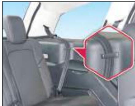
When second or third row seat is not occupied, hook the seat belts at its respective belt hanger to avoid rattling. Make sure the belt webbing is not twisted.
