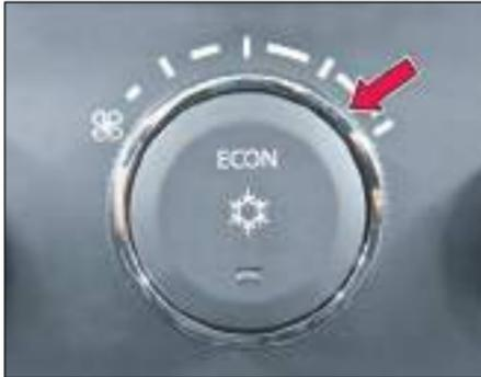
To switch OFF, turn the blower speed control knob in extreme counter clockwise direction
