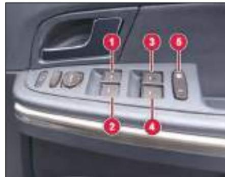
1. Front Window Winding Switch (Right)
