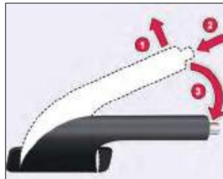
To release it, pull the lever up slightly (1), press the release button (2) and push the lever down (3). Parking brakes tell-tale on the instrument cluster will turn 'OFF' when the lever is fully released.
