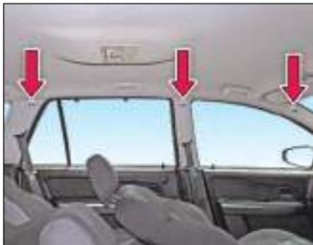
Curtain air bags are integrated into the side of the roof frame and deployed in the area from the 1<sup>st</sup> row seat to the 2<sup>nd</sup> row seat.
