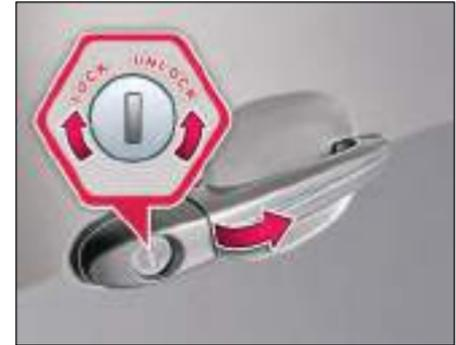
All doors can be locked / unlocked manually from outside using driver door key slot. Insert the mechanical key and turn it clockwise to lock and counter clockwise to open the doors.
