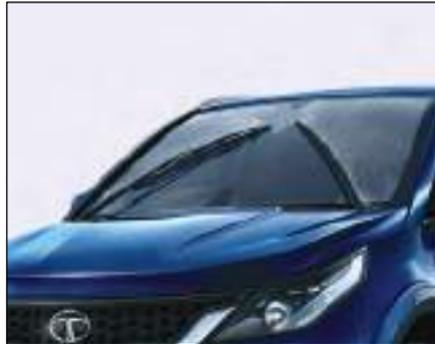
The rain sensor automatically operates your vehicle's wipers when it detects raindrops falling on the windscreen. The Auto front wipe gets enabled only when you keep the left wiper stalk in 'AUTO' position and ignition is 'ON'.
