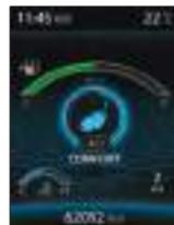
Cyan in color and 4x2 indicates the vehicle is in two-wheel drive mode.
