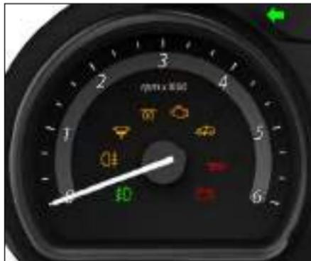
Tachometer indicates engine speed in revolutions per min (rpm).
