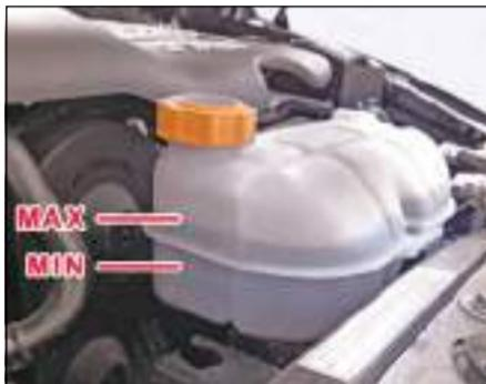
Check the coolant level when the vehicle is on a level surface and the engine has cooled down.
