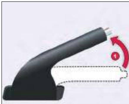
To apply the parking brake, pull the lever (1) up fully. The parking brakes tell-tale illuminates on the instrument cluster.
