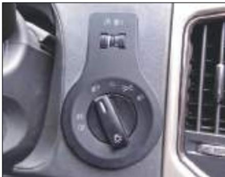
Automatic Headlamp mode is activated if Master Light switch is in auto mode.
