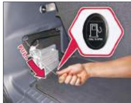
Alternatively, you can also open the fuel flap manually by following the below steps:
