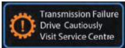
In the event that transmission develops a fault, a warning message will be displayed on instrument cluster.
