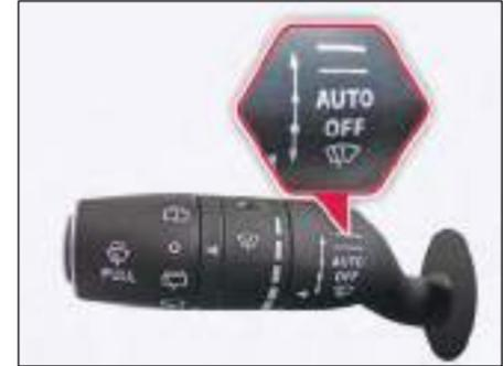
The wiper stalk will also provide five rain sensitivity/frequency settings to allow you to select the sensitivity of the auto wipe system,
