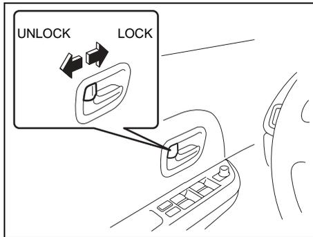
To lock a door from inside the vehicle, turn the lock knob forward. Turn the lock knob rearward to unlock the door.
