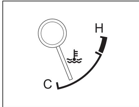
When the ignition switch is in the "ON" position, this gauge indicates the engine coolant temperature. Under normal driving conditions, the indicator should stay within the normal, acceptable temperature range between "H" and "C". If the indicator approaches "H", overheating is indicated. Follow the instructions in the "If the Engine Overheats" or "EMERGENCY SERVICE" section.
