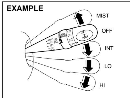
To turn the windshield wipers on, move the lever up and down to one of the four operating positions. In the "INT" position (if equipped), the wipers operate intermittently. The "INT" position is very convenient for driving in mist or light rain. In the "LO" position, the wipers operate at a steady low speed. In the "HI" position, the wipers operate at a steady high speed. To turn off the wipers, move the lever back to the "OFF" position.
