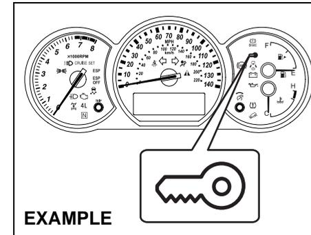
If the keyless start system blue indicator light illuminates on the instrument cluster, you can turn the ignition switch. If the red indicator light illuminates, you cannot turn the ignition switch.
