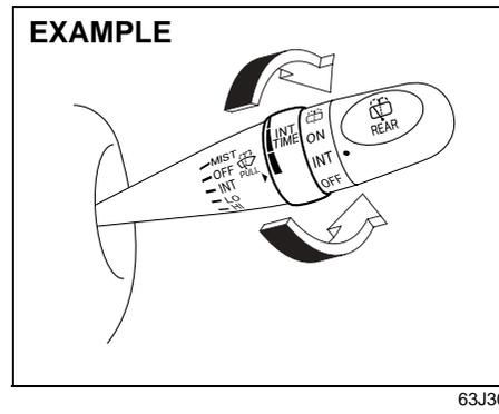
If the lever is equipped with the "INT TIME" control, turn the control forward or rearward to adjust the intermittent wiper operation to the desired interval.
