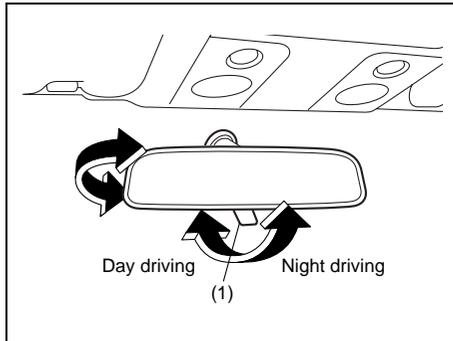
You can adjust the inside rearview mirror by hand so as to see the rear of your vehicle in the mirror. To adjust the mirror, set the selector tab (1) to the day position, then move the mirror up, down or sideways by hand to obtain the best view.
