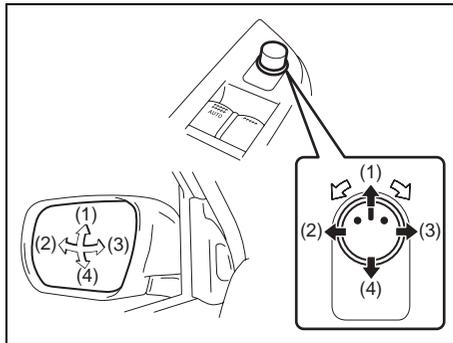
The switch to control the power rearview mirrors is located on the driver's door panel. You can adjust the mirrors when the ignition switch is in the "ACC" or "ON" position. To adjust the mirrors:
