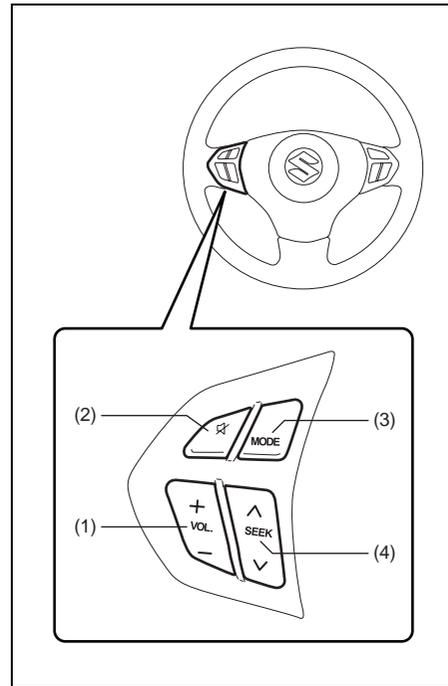
You can control basic functions of the audio system with the switches on the steering wheel.
