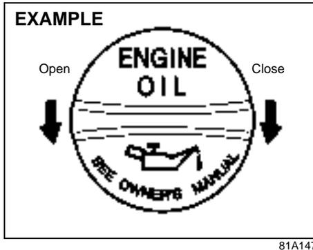
Remove the oil filler cap and pour oil slowly through the filler hole to bring the oil level to the upper limit on the dipstick. Be careful not to overfill. Too much oil is almost as bad as too little oil. After refilling, start the engine and allow it to idle for about a minute. Stop the engine, wait about 5 minutes and check the oil level again.
