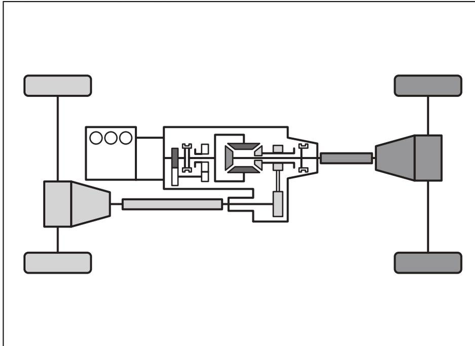
In this position, engine power is supplied to the front and rear axles. Use this position for normal driving.
