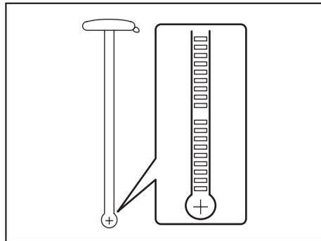
Check that there is washer fluid in the tank by looking at the washer fluid level gauge which is attached to the cap of the washer
