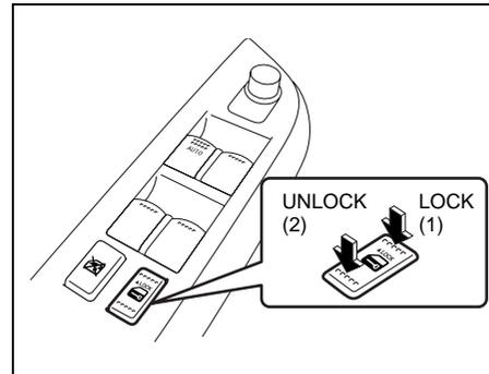
1. Push the power door locking switch of the driver's door to the lock position and then push it to the unlock position.
