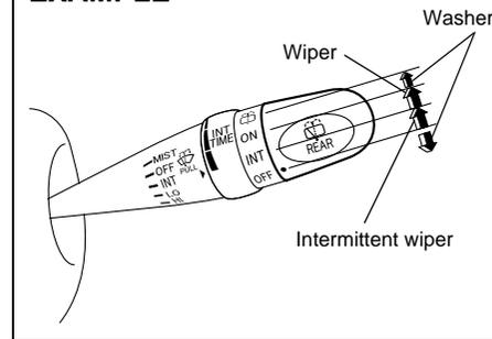
To turn the rear wiper on, twist the rear wiper switch on the end of the lever forward to the "ON" position. If your vehicle is equipped with the "INT" position, the rear wiper operates intermittently when you twist the switch forward to the "INT" position. To turn the rear wiper off, twist the switch rearward to the "OFF" position.
