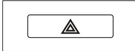
Push in the hazard warning switch to activate the hazard warning lights. All turn signal lights and both turn signal indicators will flash simultaneously. To turn off the lights, push the switch again.
