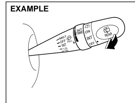
To spray windshield washer fluid, pull the lever toward you. The windshield wipers will automatically turn on at low speed if they are not already on and if the "INT" position is equipped.
