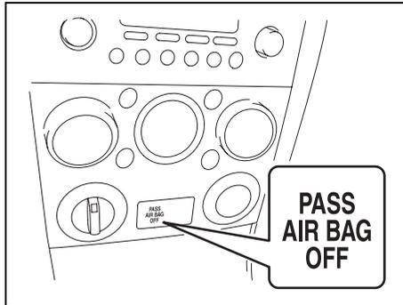
The “PASS AIR BAG OFF” indicator is located on the center of the instrument panel.
