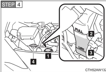
The coolant level is satisfactory if it is between the “FULL” and “LOW” lines on the reservoir.
