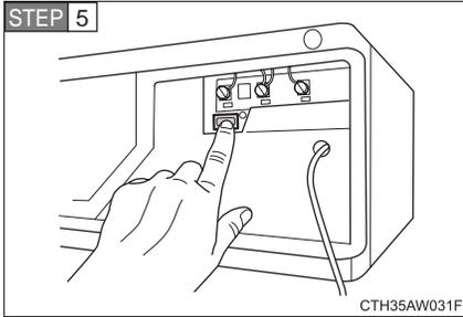
At the garage door opener motor, (security gate motor, etc...) locate the “Learn”, “Smart”, or “Program” button. This can usually be found where the hanging antenna wire is attached to the motor-head unit (see the device’s manual to identify this button). The name and color of the button may vary by manufacturer.
