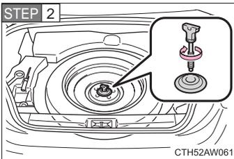
Install the center fastener as shown in the illustration.
