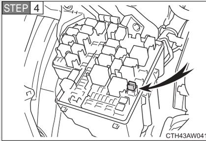
Remove the fuse with the pull-out tool.
