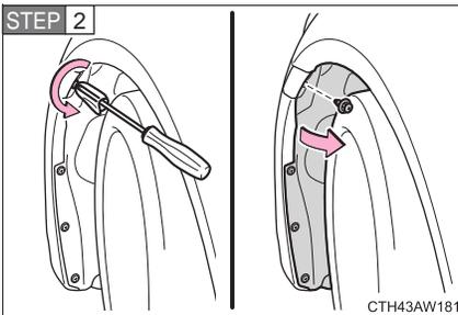
Remove the clips and partly remove the fender liner.
