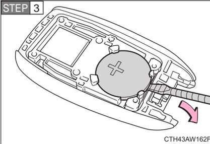
Remove the depleted battery.
