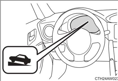
When the system is enabled, the hill start assist ON indicator will be illuminated.
