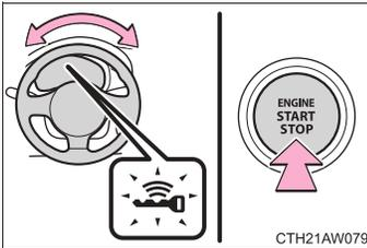
The keyless access with push button start system indicator light (green) will flash quickly and a message will be shown on the multi-information display. (→P. 442)
