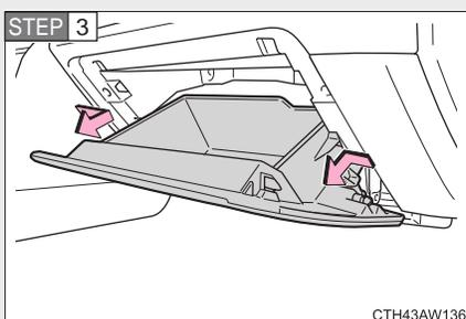
Push in each side of the glove box and pull the glove box toward you to disconnect the claws.
