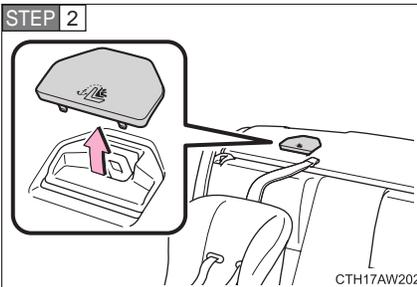
Remove the anchor bracket cover.
