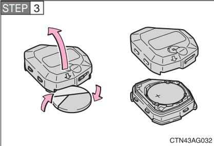
Open the case cover using a coin protected with tape and remove the depleted battery.
