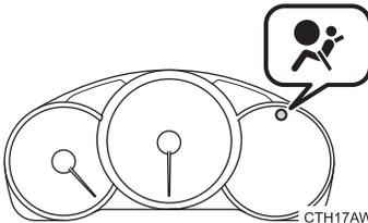
A diagnostic system continually monitors the readiness of the SRS airbag system (including front seatbelt pretensioners) while the vehicle is being driven. The SRS airbag system warning light will show normal system operation by illuminating for approximately 6 seconds when the ignition switch is turned to the “ON” position.
