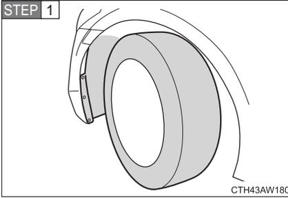
Turn the steering wheel in the opposite direction of the light to be replaced.
