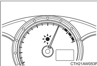
When the set engine speed is reached the REV indicator comes on and a buzzer sounds to inform the driver. (→P. 215, 228)
