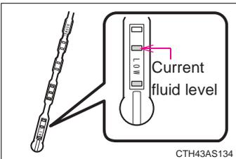
The washer fluid level can be checked by observing the position of the level on the liquid-covered holes in the gauge.
