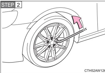
Slightly loosen the wheel nuts (one turn).
