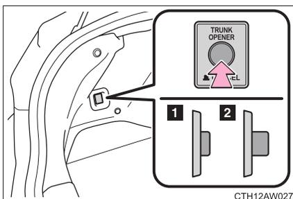
Turn the main switch in the trunk lid off to disable the trunk lid opener.
