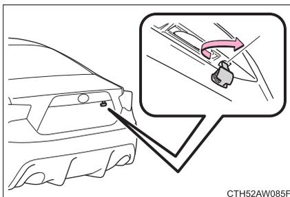
Turn the mechanical key clockwise to open.
