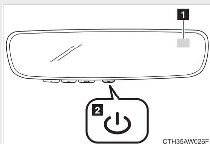
To turn the compass feature on/off, press and hold the
