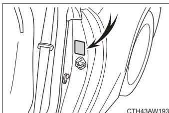
For the GAWR, see the Certification Label. For the maximum load of the tire, see the load limit at maximum cold tire inflation pressure mentioned on the sidewall of the tire. (→P. 505)
