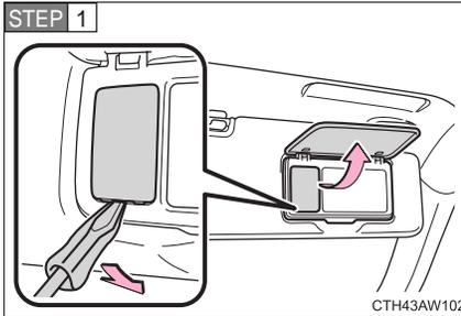
Open the cover and remove the lens.
