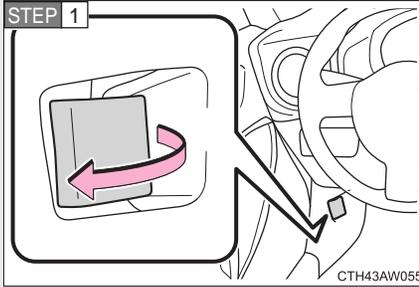
Pull the engine hood release lever.
