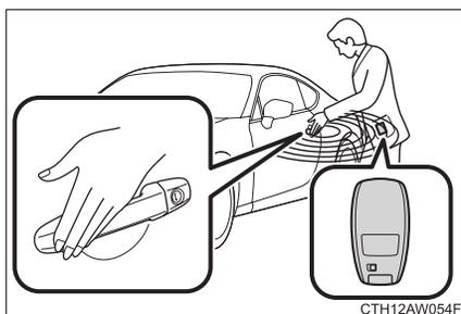
Touch the lock sensor (the indentation on the side of the door handle) to lock the doors.
