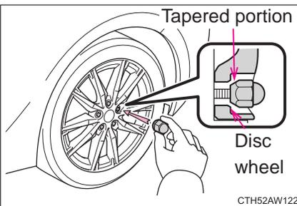
Vehicles with a spare tire of the same wheel type as the installed tires: Tighten the wheel nuts until the tapered portion comes into loose contact with the disc wheel.
