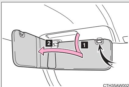
**1** To set the visor in the forward position, flip it down.
