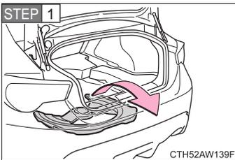
Vehicles with a T145/70D17 compact spare tire only: Before stowing the flat tire, remove the spare tire spacer.
