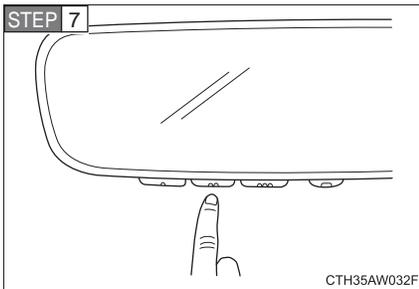
Return to the vehicle and firmly press, hold for two seconds and release the HomeLink button up to three times. At this point programming is complete and your device should operate when the HomeLink button is pressed and released.
