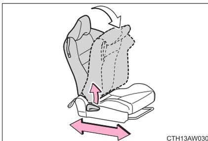
Lift the seatback angle adjustment lever.
