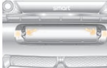
Parking assist uses two ultrasound sensors (A) mounted on the rear licence plate holder to monitor the rear section of your car when slowly reversing (walking pace). Parking assist is automatically activated when you start the engine and engage the reverse gear. An acoustic signal notifies you that the system is activated.
