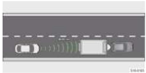
ACC detects a narrow or staggered vehicle only when it is in the area covered by the radar.
