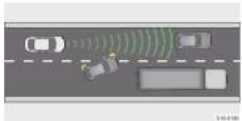
A vehicle that changes to the lane a short distance away may not be recognized by the ACC in time.
