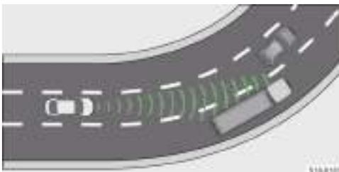
When cornering, a vehicle in the next lane may enter the detected area. Your vehicle will be controlled according to this vehicle.
