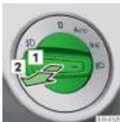
Positions for pulling out the light switch
