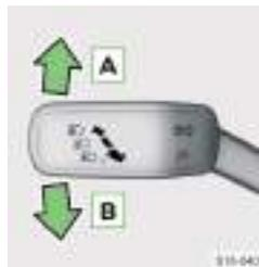
**A** Switching on the indicator light on the right - the warning light flashes in the instrument cluster
