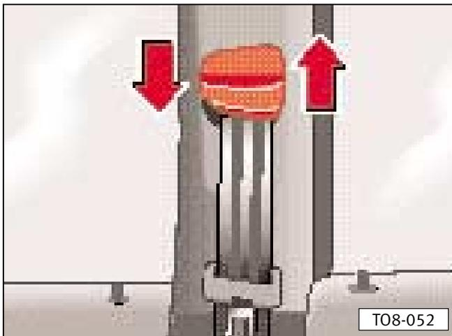
With the aid of the **belt height adjustment** the routing of the shoulder belt for the front and rear seats can be set to fit the body properly.
