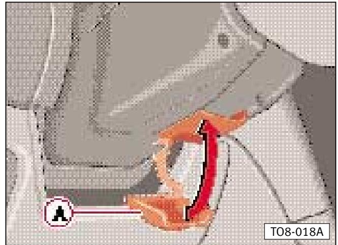
The steering column can be adjusted at will both for reach and for height. Press the lever **A** beneath the steering column down and move the steering wheel to the desired position. Then press the lever firmly up again.
