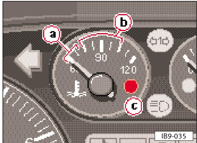
If the needle is in the right half of the indicator, the coolant temperature is too high. **In this case, pull over, switch the engine off, wait until it cools** and then look for the cause of the problem. See the chapter on “Cooling system”.
