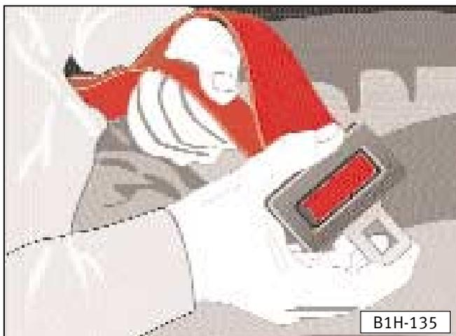
**To lengthen** belt hold the tongue at right angles to belt and pull belt through to the required length – see illustrations.
