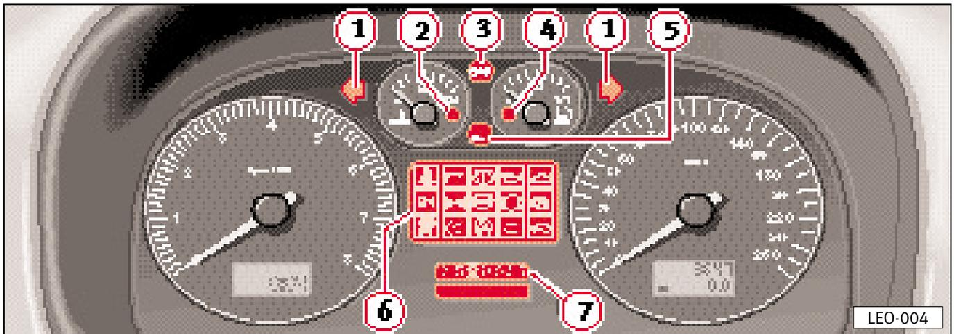
The layout of the warning lamps depends on the model version and engine fitted. The symbols shown here are also on the actual warning lamps.
