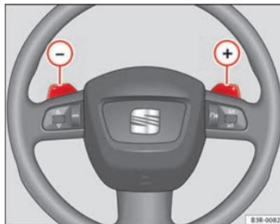
Fig. 152 Steering wheel: tiptronic controls
