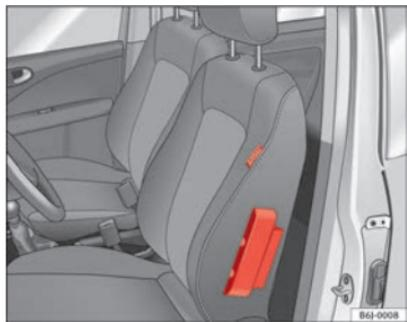
**Fig. 24 Side airbag in driver seat**
