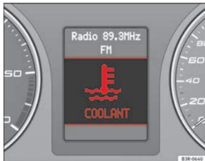
Fig. 55 Display: Coolant level warning
