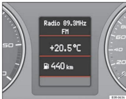
Fig. 48 Cockpit: Digital instrument panel display
