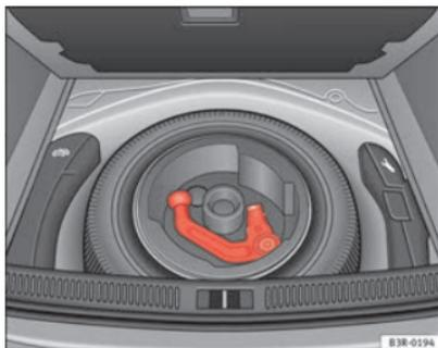
**Fig. 155** Luggage compartment: Spare wheel with towing bracket
