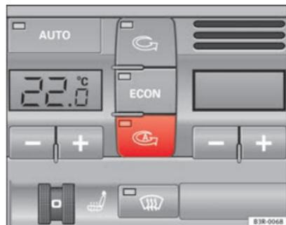
Fig. 130 Button for automatic air recirculation
