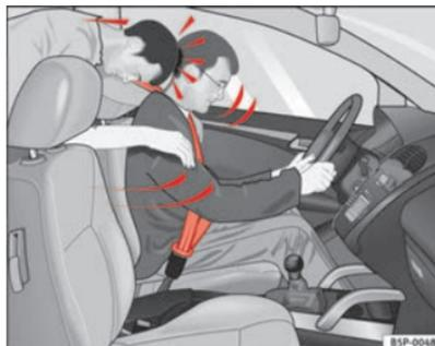
**Fig. 10** The unbelted passenger in the rear seat is thrown forward violently, hitting the driver wearing a seat belt
