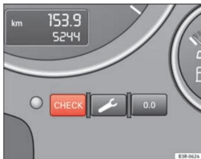
Fig. 54 Instrument panel: CHECK button
