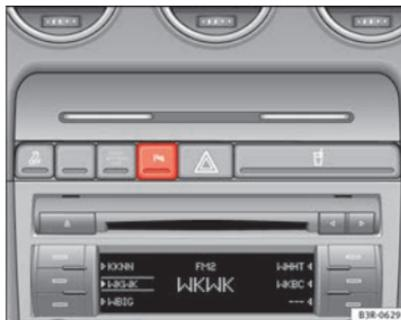
Fig. 143 Centre console: switch for parking aid
