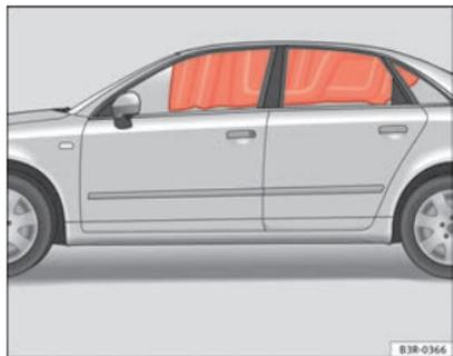
Fig. 27 Deployed curtain airbags
