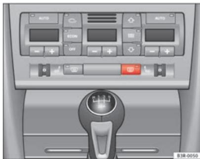
**Fig. 96** Switch for heated rear window
