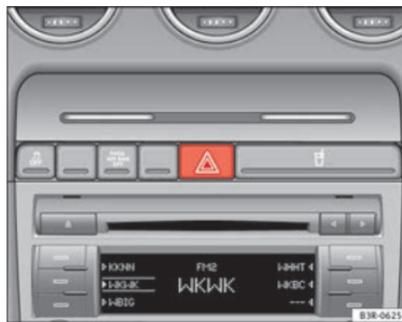
Fig. 90 Centre console: Switch for hazard warning lights
