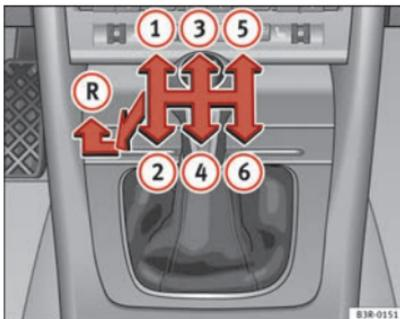
Fig. 146 Detailed view of the centre console: gear shift pattern of a 6-speed manual gearbox
