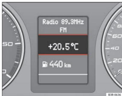
Fig. 50 Display: Outside temperature indicator
