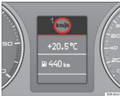
Fig. 57 Display: Speed warning function
