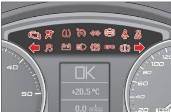
Fig. 45 Instrument panel with warning and indicator lamps
