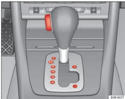
Fig. 147 Detailed view of the centre console: Selector lever with lock button
