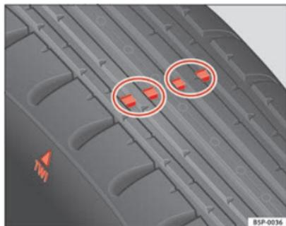
Fig. 178 Tyre tread wear indicators
