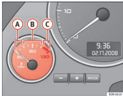
Fig. 39 Engine coolant temperature gauge
