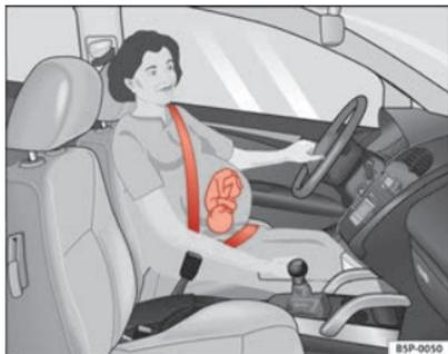
Fig. 15 Positioning seat belts during pregnancy
