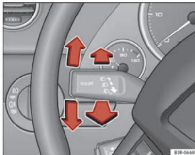
Fig. 91 Turn signal and main beam headlight lever
