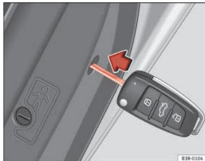
**Fig. 74** Activating manual locking
