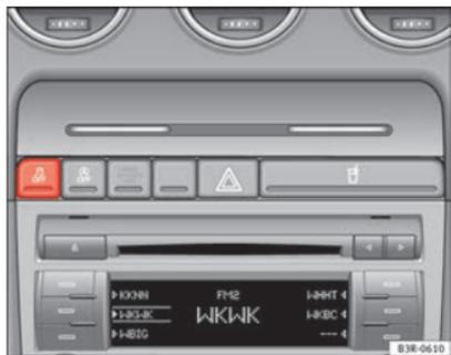
**Fig. 153** Centre console with ESC switch
