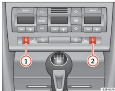
Fig. 132 Detailed view of the dash panel: Thumbwheel controls for seat heating
