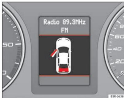
Fig. 52 Display: Door and rear lid warning
