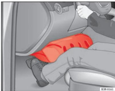
**Fig. 23** Inflated airbags protect in a frontal collision.
