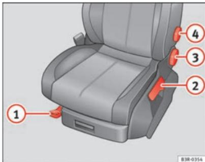
Fig. 104 Adjuster controls on driver seat
