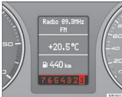
Fig. 151 Display: Manual gear selection (tiptronic mode)
