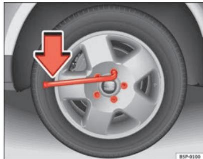
Fig. 183 Changing a wheel: Loosen the wheel bolts
