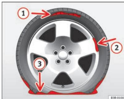
**Fig. 187** The Tyre Mobility System is not suitable for repairing this type of damage to tyres.
