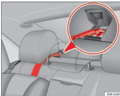
Fig. 36 Retainer strap: correct adjustment and fitting
