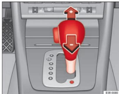
Fig. 150 Centre console: Manual gear selection (tiptronic mode)
