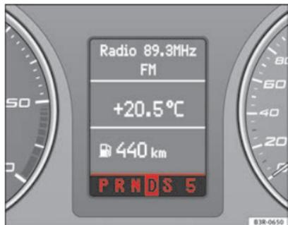
Fig. 148 Display: Selector lever positions
