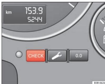
Fig. 58 Detailed view of the instrument panel: **CHECK** button
