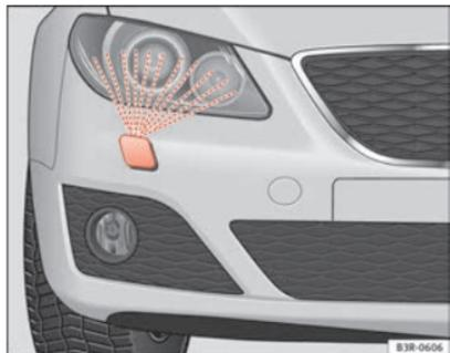
Fig. 101 Headlight with extended washer jet
