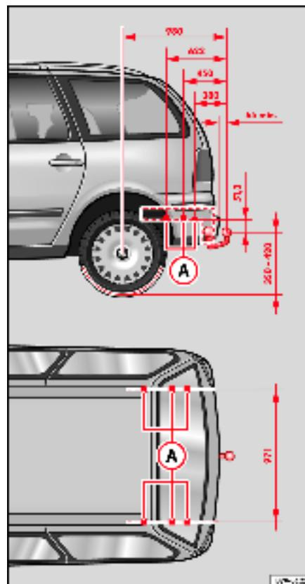
Fig. 135 Attachment points for towing bracket ►
