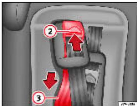
Fig. 39 Integrated child seats. adjusting harness belt
