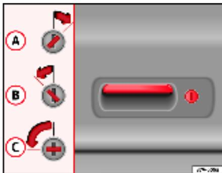
Fig. 63 Key slot positions of tailgate lock
