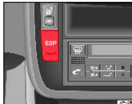
**Fig. 124** Detailed view of dash panel ESP button
