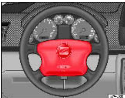
**Fig. 22** Driver airbag located in steering wheel
