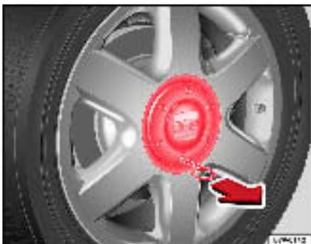
Fig. 155 Removing the hubcaps
