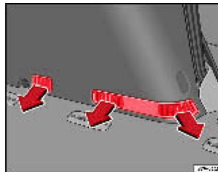
Fig. 120 Air outlets for heating the passenger compartment
