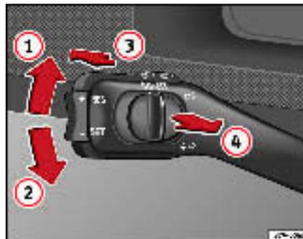
**Fig. 73** Turn signal and main beam headlight lever
