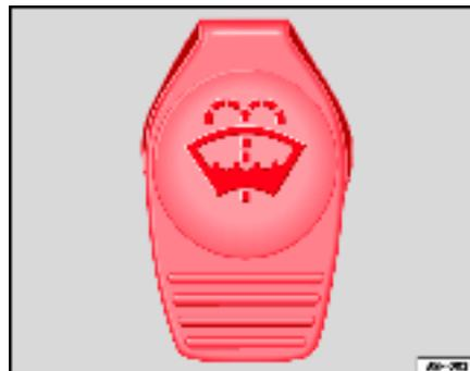
**Fig. 143** In the engine compartment: Cap of windscreen washer fluid reservoir.
