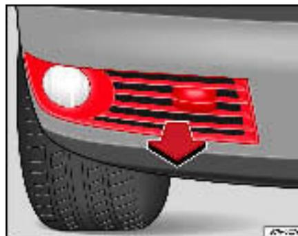
**Fig. 172 Towing eye at the front of the vehicle**
