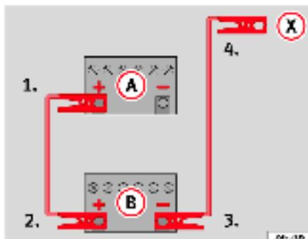
Fig. 171 How to connect the jump leads
