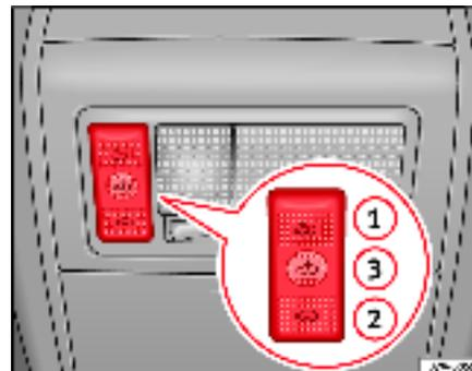
Fig. 66 Interior roof trim: control of sliding/tilting roof
