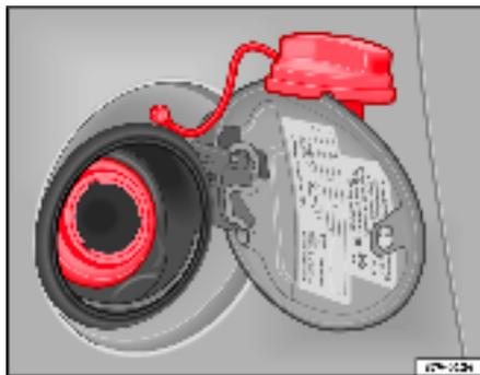
**Fig. 136** Tank filler neck and tank flap
