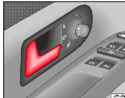
**Fig. 58 Driver's door release lever in normal position**
