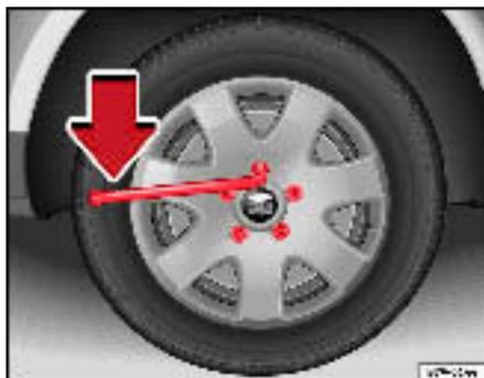
Fig. 157 Changing the wheel: loosen the wheel bolts
