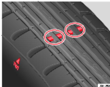
Fig. 148 Tyre tread wear indicators
