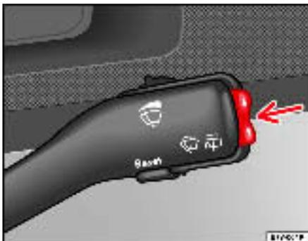
Fig. 51 Button on the windscreen washer lever:
