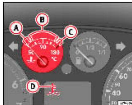
Fig. 45 Instrument panel: engine coolant temperature gauge
