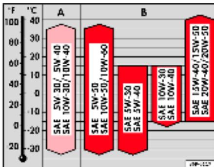
Fig. 139 Types of oil according to temperature
