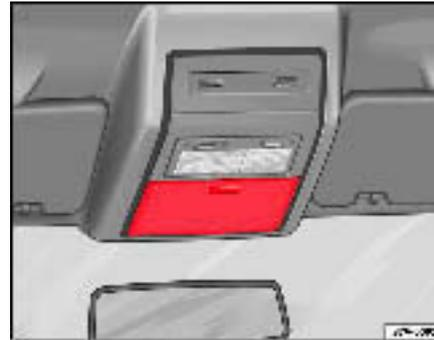
Fig. 103 Stowage area in the roof
