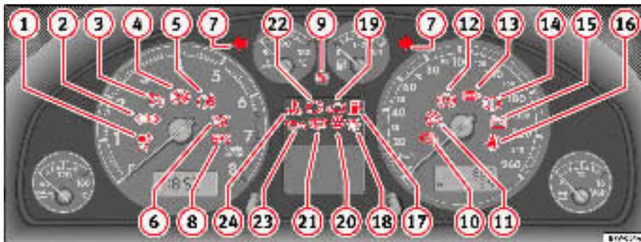
Fig. 48 Instrument panel with warning lamps. Some of the items of equipment listed here are fitted only on certain models/model years or are optional extras.
