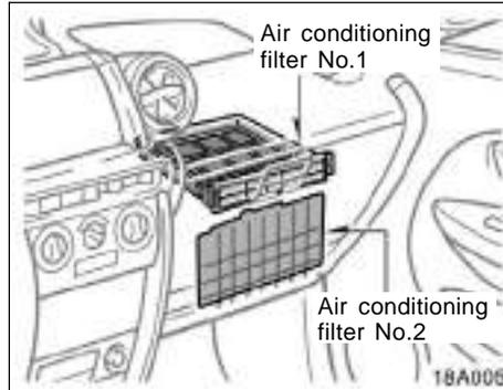
**The air conditioning filters are behind the glove box.**
