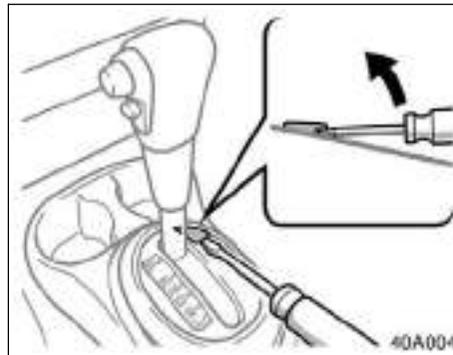
If you cannot move the selector lever out of “P” position to other positions even though the brake pedal is depressed, use the shift lock override button as follows:
