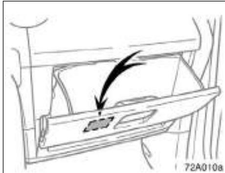
**The air conditioning filter information label is placed on the inside of the glove box as shown and indicates that the filters have been installed.**
