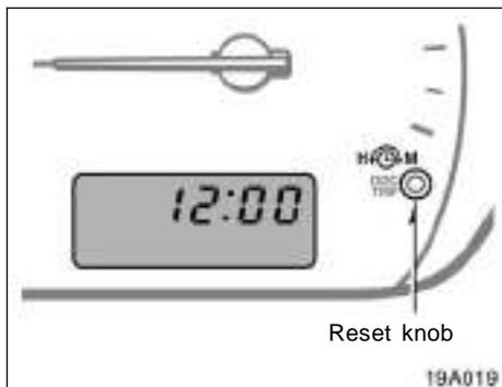
To reset the hour: Turn the knob counter-clockwise.
