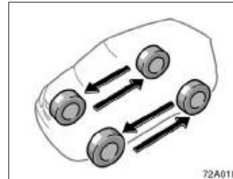
To equalize the wear and help extend tire life, Scion recommends that you rotate your tires according to the maintenance schedule. (For scheduled maintenance information, please refer to the "Scheduled Maintenance Guide" or "Owner's Manual Supplement".) However, the most appropriate timing for tire rotation may vary according to your driving habits and road surface conditions.
