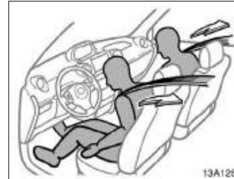
Both front seats are equipped with seat belt pretensioners and are designed to be activated in response to a severe frontal impact.
