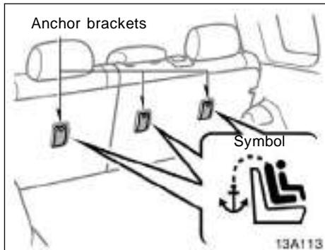
Use the anchor brackets on the back of the rear seatback to attach the strap.
