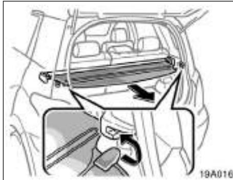
To use the luggage cover, pull it out of the retractor and hook it on the anchors.
