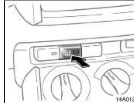
**To defog or defrost the rear window and outside rear view mirror, push the switch.**
