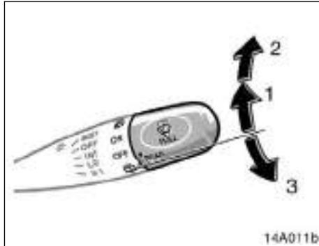
**To turn on the rear window wiper, twist the lever knob upward. (Position 1)**
