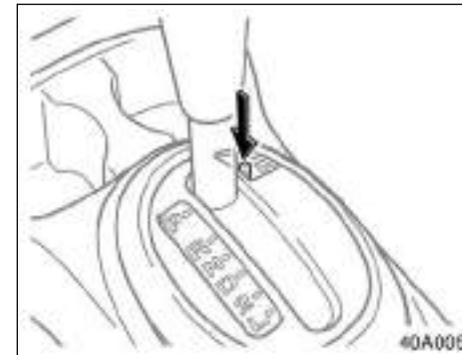
3. Insert your finger into the hole to push down the shift lock override button. You can move out of “P” position only while pushing the button.
