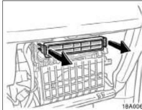
**2. Pull out the air conditioning filter case as shown in the illustration.**
