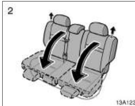
2. Pull up the lock release button and fold the seatback down.
