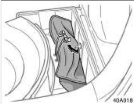
To remove the tool bag, unlock the tightening strap.
