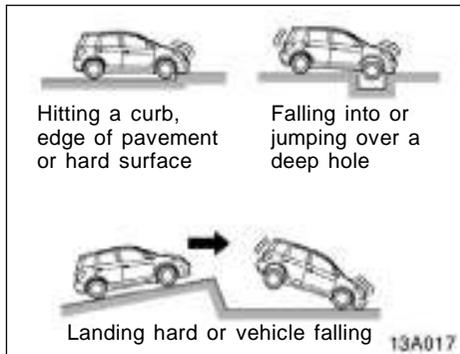
**The SRS front airbags may also deploy if a serious impact occurs to the underside of your vehicle. Some examples are shown in the illustration.**
