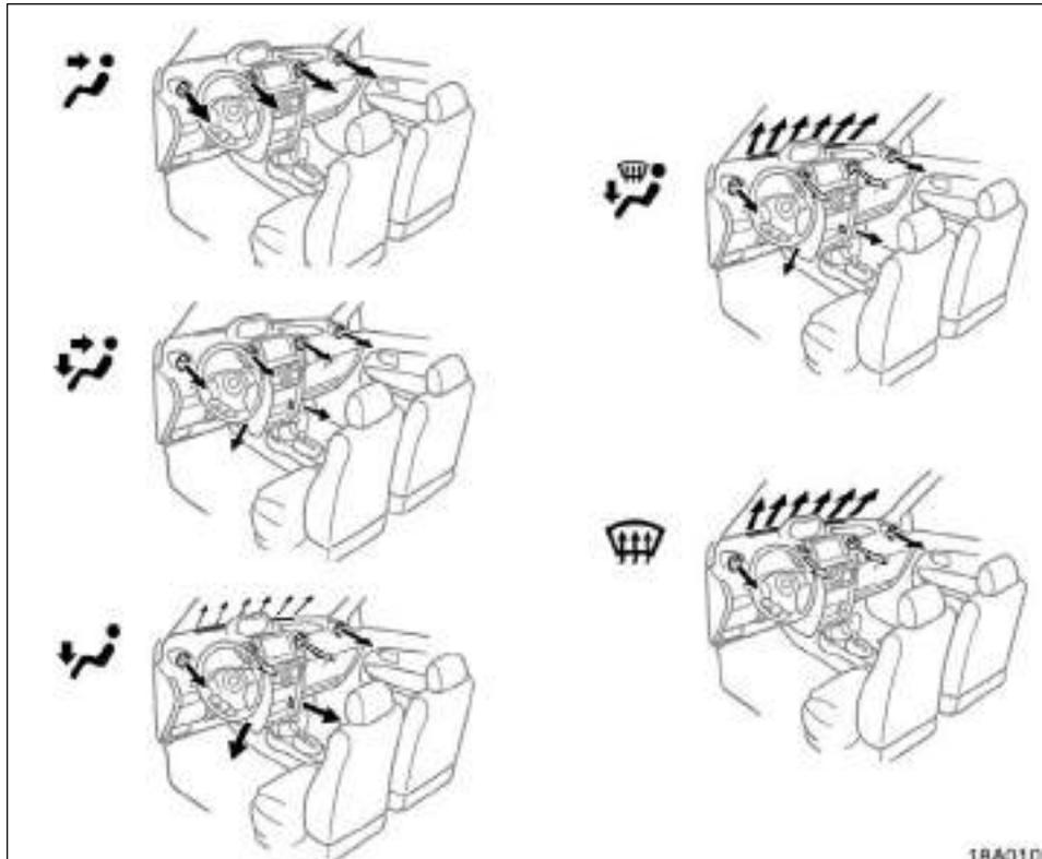
⇒ : When turning the temperature selector fully to the left position, cold air comes out from the center vents regardless of the position of the air flow selector.
