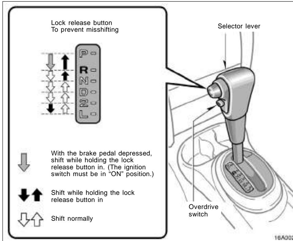
Your automatic transmission has a shift lock system to minimize the possibility of incorrect operation. This means you can only move out of "P" position when the brake pedal is depressed (with the ignition switch in "ON" position and the lock release button depressed).
