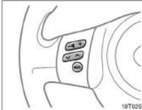
Steering switches are installed on the left side of the steering wheel.
