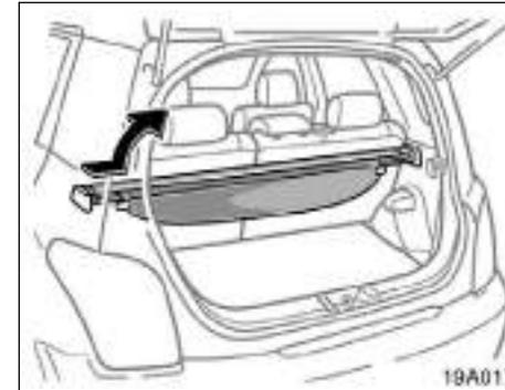
To remove the luggage cover, fold down the rear seat on the right side, retract and release the left end, and lift the luggage cover out.
