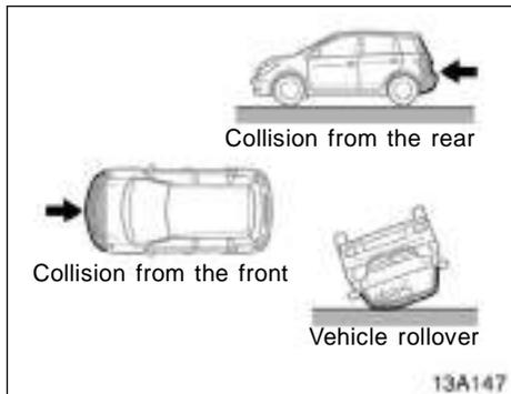
**The SRS side airbag and curtain shield airbags are not generally designed to inflate if the vehicle is involved in a front or rear collision, if it rolls over, or if it is involved in a low-speed side collision.**
