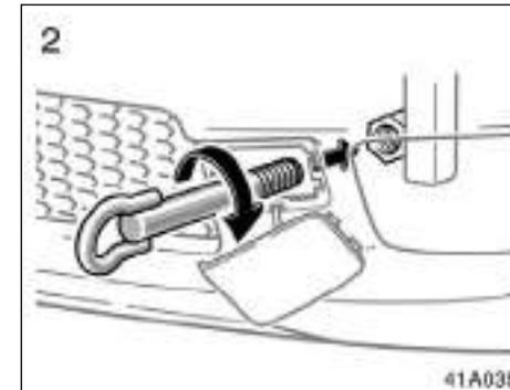
2. Use the towing eyelet in the tool bag. Secure it to the hole on the bumper by turning clockwise. (For the tool bag storage location, see "—Required tools and spare tire" on page 161.)
