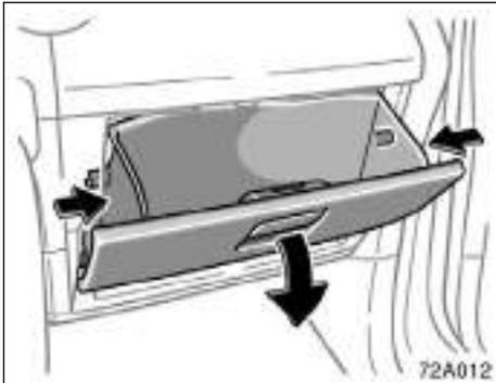
**1. Remove the glove box from the instrument panel.**
