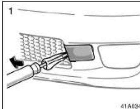
1. Remove the towing eyelet cover on the bumper, using a flathead screwdriver which is wrapped with a cloth.
