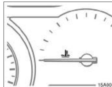
The indicator and warning light indicates the engine coolant temperature when the ignition switch is on. The engine operating temperature will vary with changes in weather and engine load.
