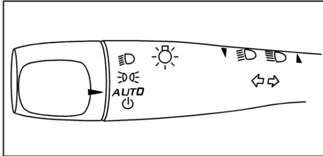
The lever on the left side of the steering column operates the exterior lamps.
