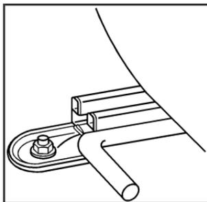
Lift the lever located under the front of the seat to unlock it.
