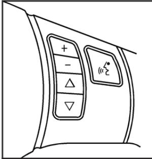
Radio controls are located on the inboard side of the steering wheel. If your vehicle has this feature, some audio controls can be adjusted at this location. They include the following:
