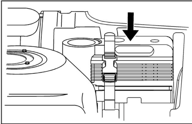
3. Locate the tire sealant and compressor kit on the driver side of the vehicle, near the back corner of the trunk.
