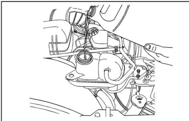
The coolant surge tank is located in the engine compartment on the driver's side of the vehicle.
