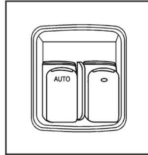
On vehicles with power windows, the switches on the driver's door armrest control both windows.
