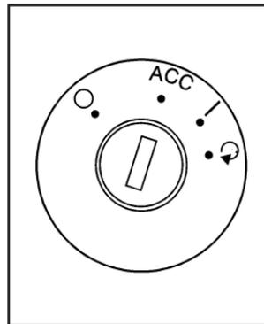
With the key in the ignition switch, you can turn it to four different positions.
