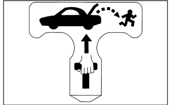
**Notice:** Do not use the emergency trunk release handle as a tie-down or anchor point when securing items in the trunk as it could damage the handle. The emergency trunk release handle is only intended to aid a person trapped in a latched trunk, enabling them to open the trunk from the inside.
