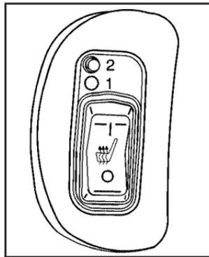
On vehicles with heated front seats, the buttons are located on the outboard side of the driver's and front passenger seats.
