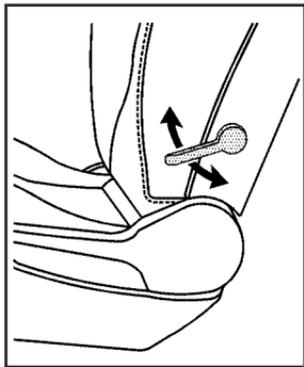
On vehicles with this feature, the handle is located on the outboard side of the seat.
