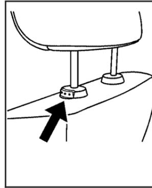
Pull the restraint up to raise it. To lower the head restraint, press the button, located on the top of the seatback, and push the restraint down.
