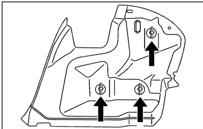
4. Turn the three wing nuts counterclockwise that hold the taillamp assembly counterclockwise.
