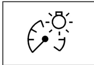
The knob with this symbol is located on the instrument panel to the left of the steering column.
