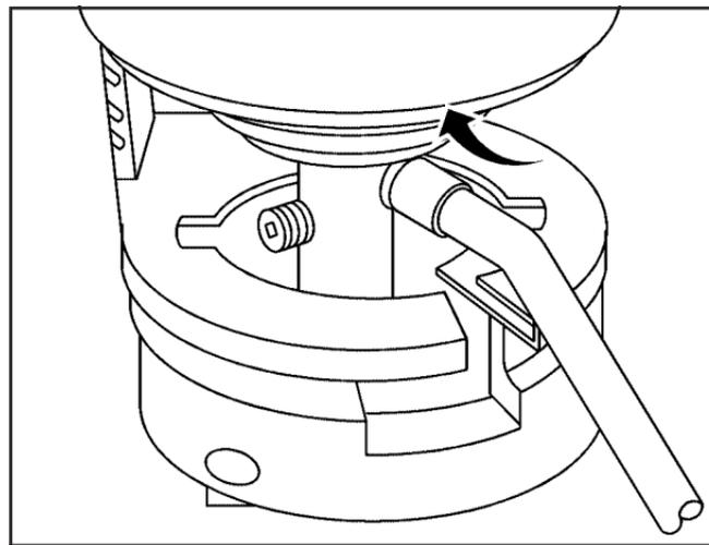
1. Unlock the air only hose (F) from the sealant canister (B) by pulling up on the lever.
