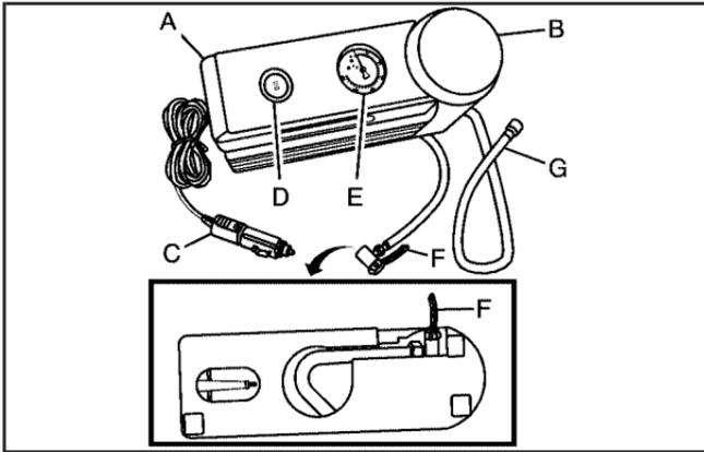
2. Unlock the air only hose (F) from the sealant canister (B) by pulling up on the lever.
