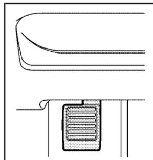
To set the parking brake, push down the parking brake pedal with your left foot. If the ignition is on, the brake system warning light will come on. See *Brake System Warning Light* on page 3-30.
