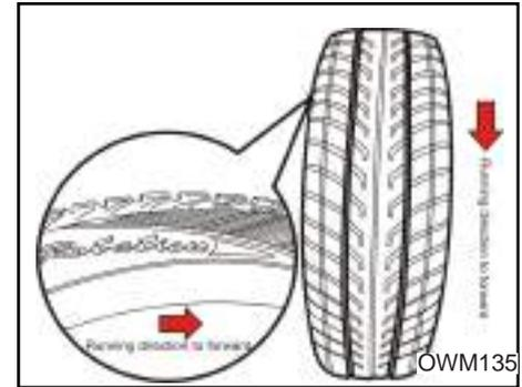
In the vehicles with directional tread tires, the tires should be installed such that the direction of tread stays at the same direction of vehicle motion toward the front. In this condition when you look at the vehicle from the front, you will see tread as V or Y shape.
