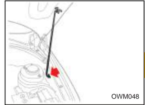
3- Raise the engine hood and insert the retainer rod free end into the corresponding slot in the hood.
