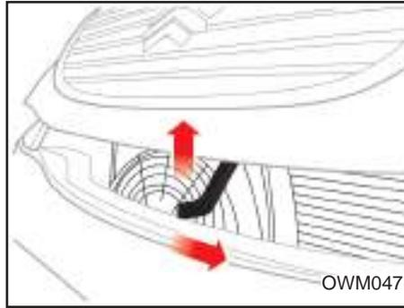
2- Go to the front of vehicle and pull the engine hood up. Then release the secondary lever located at the middle bottom part of the engine hood as shown in the figure.
