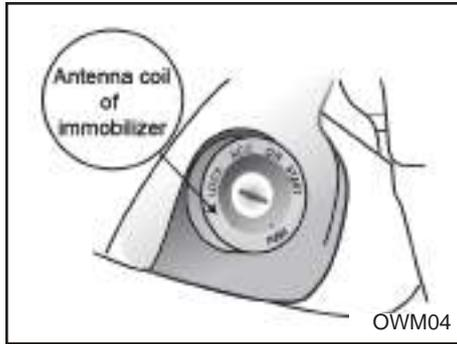
When starting the engine, first turn the key into ON position and then try to start.
