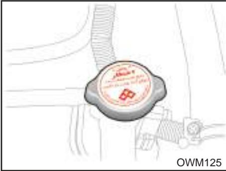
1- Remove the radiator cap by turning it counter-clockwise.
