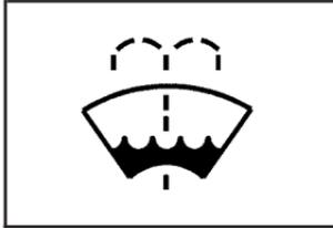
Open the cap with the washer symbol on it. Add washer fluid until the tank is full. See *Engine Compartment Overview on page 330* for reservoir location.
