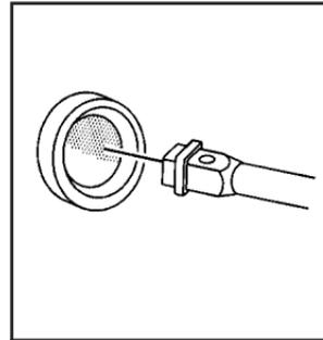
11. If the spare tire is hanging from the cable, insert the socket end of the extension into the hoist shaft hole on a 45 degree angle downward.
