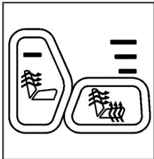
Your vehicle has heated front seats. The buttons used to control this feature are located on the front door armrests. The engine must be running for the heated seat feature to work.
