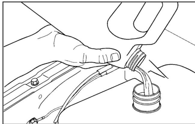
3. Fill the radiator with the proper DEX-COOL<sup>®</sup> coolant mixture, up to the base of the filler neck. See *Engine Coolant on page 344* for more information about the proper coolant mixture.
