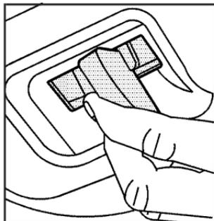
The tilt lever is located to the left of the steering column, under the turn signal lever.
