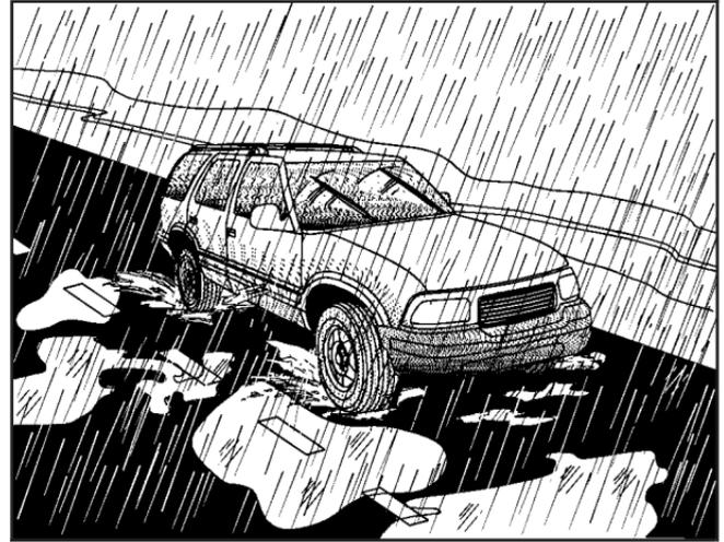
Rain and wet roads can mean driving trouble. On a wet road, you cannot stop, accelerate, or turn as well because your tire-to-road traction is not as good as on dry roads. And, if your tires do not have much tread left, you will get even less traction. It is always wise to go slower and be cautious if rain starts to fall while you are driving. The surface may get wet suddenly when your reflexes are tuned for driving on dry pavement.
