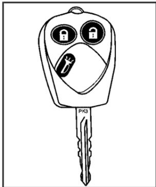
**U (Unlock):** Press the unlock button to automatically unlock the driver's door. The parking lamps may flash and the interior lights will go on. Press the unlock button again and all remaining doors will unlock.
