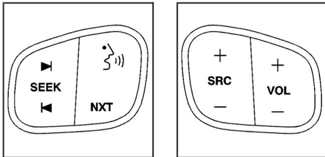
Some audio controls can be adjusted at the steering wheel. They include the following:
