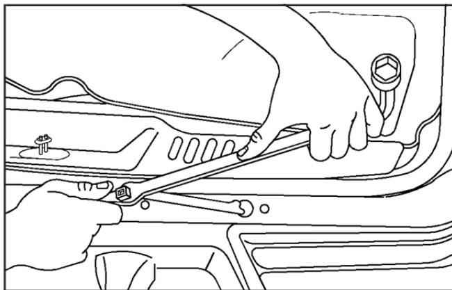
Turn the wheel wrench counterclockwise to lower the spare the rest of the way.
