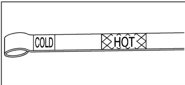
3. Check both sides of the dipstick, and read the lower level. The fluid level must be in the COLD area, below the cross-hatched area, for a cold check or in the HOT or cross-hatched area for a hot check. Be sure to keep the dipstick pointed down to get an accurate reading.
