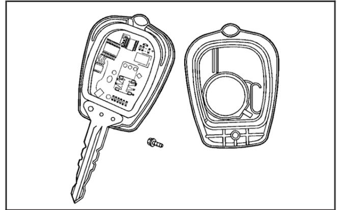
1. Remove the screw from the back of the remote keyless entry cover and gently pry the transmitter apart.
