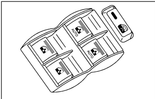
The controls for the power windows are located on the armrest on each of the side doors. With power windows, the switches operate the windows when the ignition is in RUN, ACC or when Retained Accessory Power (RAP) is active. See *Retained Accessory Power (RAP)* on page 108. The driver's door also has a switch for each of the passenger's windows.
