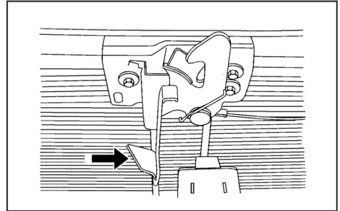
2. Then go to the front of the vehicle and push the secondary hood latch up and to the right to release it, then lift the hood.
