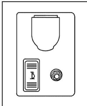
The accessory inflator is located in the rear compartment on the driver's side of the vehicle, behind an access cover, and near the liftgate opening.
