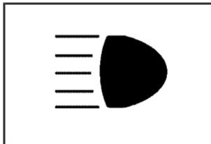
This light comes on when the high-beam headlamps are in use.
