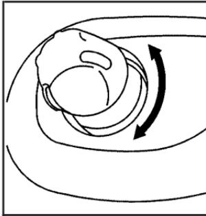
The outside power mirror control is located on the driver's door.
