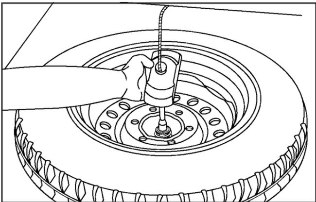
5. Tilt the retainer at the end of the cable when the tire has been completely lowered, and pull it through the wheel opening.
