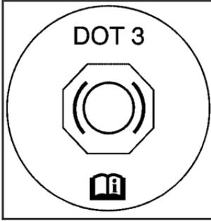
Your brake master cylinder reservoir is filled with DOT-3 brake fluid. See *Engine Compartment Overview* on page 330 for the location of the reservoir.
