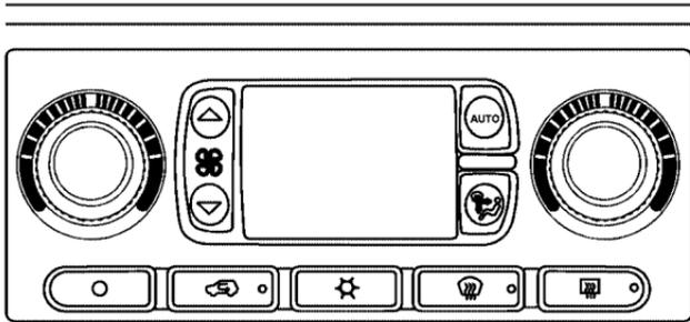
With this system you can control the heating, cooling and ventilation for your vehicle. When your vehicle is first started and the climate control system is on, or if the climate control system has been turned on, the display will show the driver's temperature setting for five seconds. Then it will show the outside temperature.
