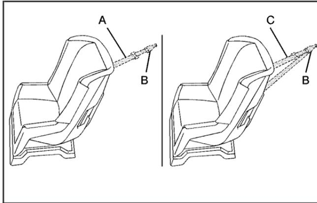
A top tether (A, C) anchors the top of the child restraint to the vehicle. A top tether anchor is built into the vehicle. The top tether attachment (B) on the child restraint connects to the top tether anchor in the vehicle in order to reduce the forward movement and rotation of the child restraint during driving or in a crash.
