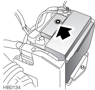
The battery is designed to be maintenance free, so topping-up is unnecessary. On the top of the battery there is a battery condition indicator (arrowed in illustration). Examine the indicator periodically to check the battery's condition. When the indicator shows:
