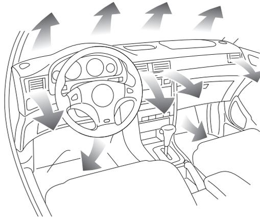
The heating and ventilation system provides fresh or heated air to the interior of the car from the air intake grille in front of the windscreen.
