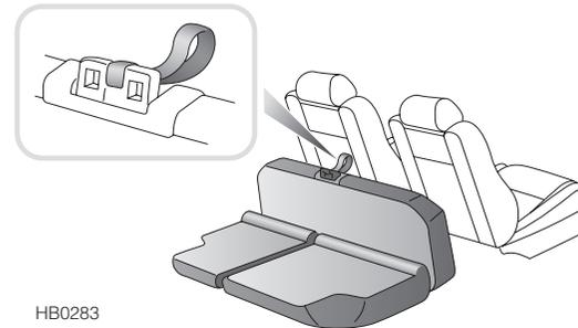
To create an extra large luggage area; pull the lifting strap (highlighted in illustration) and tip the rear seat cushion forwards. Remove both rear head restraints, then release both parts of the backrest and fold them forwards as shown.
