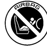
The above symbol affixed to the fascia panel of your car, warns against the use of a REAR FACING child seat in the front passenger seat. This type of child seat could cause serious injury to your child in the event of an airbag deployment.
