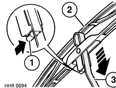
Lift the wiper arm away from the windscreen. With the blade at 90° to the arm as shown, disconnect the blade by pushing in the locking tab (1) and sliding the blade (2) down the arm (3).
