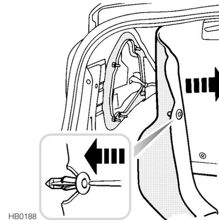
From inside the luggage compartment, remove the fastener (illustrated in inset) and pull back the moulded lining as shown.
