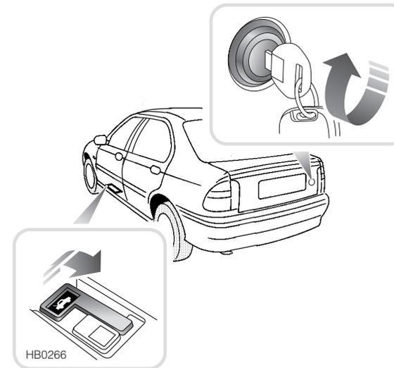
To open, use the key in the lock or, from inside the car, lift the release lever adjacent to the driver's seat. The luggage compartment light switches on automatically when the taildoor (or boot lid) is opened.
