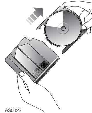
Holding the magazine as shown (arrow on magazine casing uppermost), remove each CD tray in turn.
