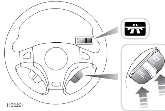
1. Press the master switch (the warning light in the instrument panel illuminates).
