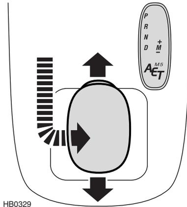
There are five predetermined gear ratios, all of which can be selected sequentially by a single forward or rearward movement of the gear selector lever, as follows:
