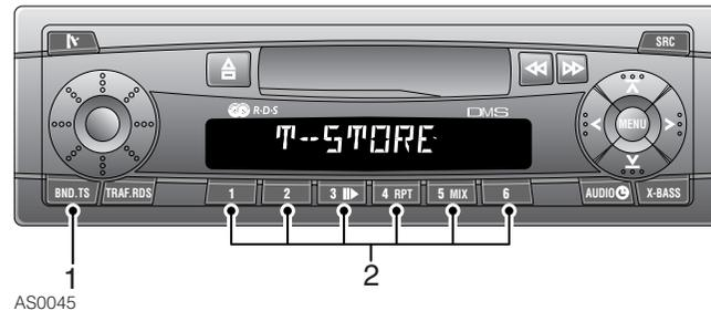
Travelstore operates on the FM waveband only and enables you to rapidly tune and store the six strongest FM radio signals in a single operation. This facility is particularly useful if you are in an unfamiliar area and have little knowledge of local transmitter frequencies.
