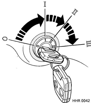
The starter switch uses the following sequence of key positions to operate the steering lock, electrical circuits and starter motor:
