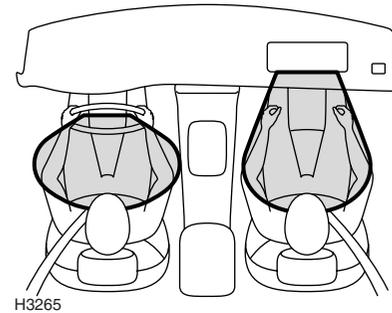
Airbag inflation is virtually instantaneous and occurs with considerable force, accompanied by a loud noise. The inflated bag, together with the seat belt restraint system, limit the movement of a front seat occupant, thereby reducing the risk of injury to the head and upper torso.
