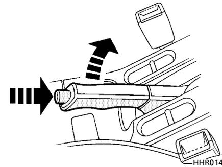
The handbrake operates on the rear wheels only. To apply the handbrake, pull the lever up. Always apply the handbrake FULLY whenever you park the car.
