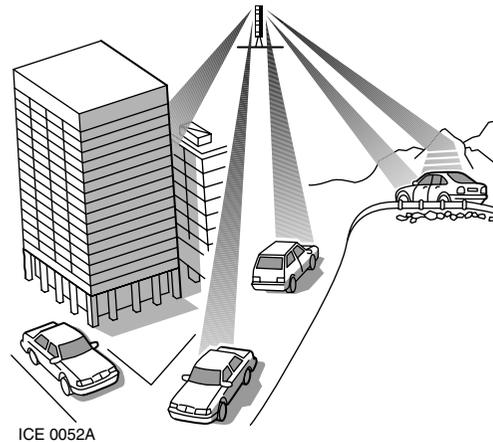
Distortion, interference and lack of signal clarity, are often attributed to a fault in the radio - this is rarely the case.
