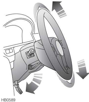
The angle of the steering column can be adjusted to suit your driving position:
