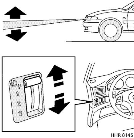
The angle of the dipped beams is affected by the distribution of passenger and luggage weight within the car. It is important that the headlights are adjusted to ensure that the point at which they meet the road surface provides adequate illumination ahead of the vehicle, without dazzling other road users.
