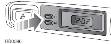
The digital clock display illuminates when the starter switch is turned on and dims for night viewing when the sidelights are switched on.
