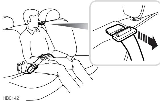
The central rear seating position is fitted with a lap belt only. It is essential that all slack is removed from the webbing and that the belt fits snugly **AS LOW ON THE HIPS AS POSSIBLE**. Fit the tongue plate into the buckle (marked 'CENTRE') nearest the centre of the seat.
