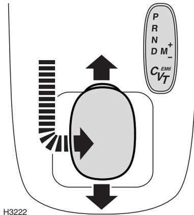
There are six predetermined gear ratios, all of which can be selected sequentially by a single forward or rearward movement of the gear selector lever, as follows:
