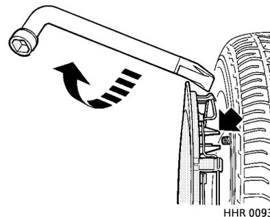
Slide the flat, wedge end of the wheel nut spanner behind the edge of the wheel trim. Working carefully around the wheel, apply a twisting action to the tool, to prise the trim from the wheel.
