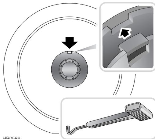
Insert the hooked end of the removal tool into the small rectangular aperture in the wheel nut cover (arrowed in illustration). Pull the wheel nut cover from the wheel to access the wheel nuts.
