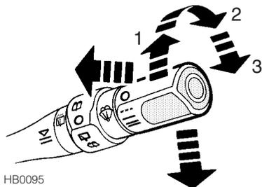
The wipers and washers will only operate when the starter switch is turned to position 'II'.
