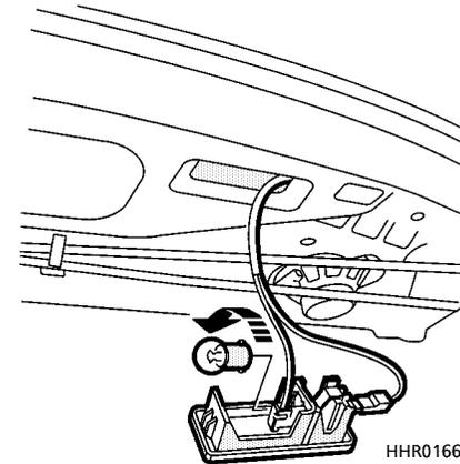
Use a small screwdriver to prise the lens from the light housing. Twist the bulb to remove.
