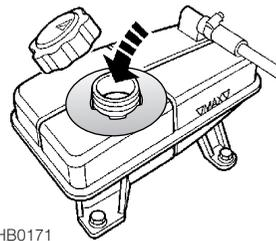
Remove the filler cap, and top-up to the MAX' mark with a 50% mixture of water and anti-freeze (see 'Coolant specification'). Ensure the cap is tightened fully after top-up is completed.
