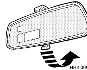
The interior mirror can be dipped to reduce glare from following vehicles. At night, move the lever at the base of the mirror forward to 'dip' the mirror. Normal visibility is restored, by pulling the lever back to its original position.
