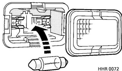
Use a small screwdriver to prise the lens from the light housing.
