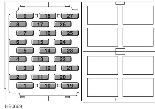
Always turn off the starter switch and the appropriate electrical circuit before removing a fuse. To remove a fuse, press the removal tweezers onto the head of the fuse and pull. Always replace a fuse with another of the same (or lower) rating. If a replacement fuse blows almost immediately, this indicates a serious electrical problem and the circuit **MUST** be checked by an MG Rover dealer.
