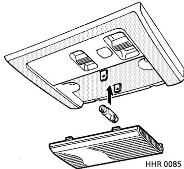
Pull down on the front edge of the lens to remove it from the light housing. Spring the bulb connectors apart to release the bulb.
