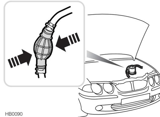
In the event of the fuel tank running dry, it will be necessary to hand-prime the fuel system (after refuelling) by squeezing the priming bulb in the engine compartment (where shown in illustration), until the bulb feels solid.
