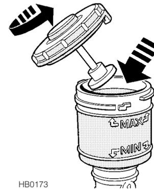
Wipe the filler cap clean before removing, to prevent dirt from entering the reservoir. Unscrew the cap 1/4 turn anti-clockwise and lift to remove. Top-up the reservoir to the 'MAX' mark using a recommended fluid.
