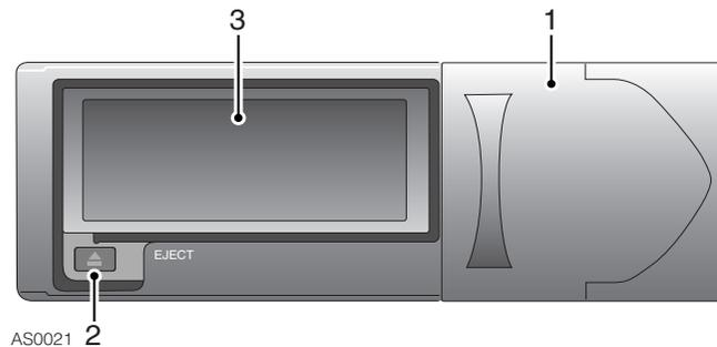
Fully open the sliding cover (1) to insert or remove the magazine. Keep the cover closed at all other times to prevent dust and dirt from entering. Press the button (2) to eject the magazine.
