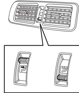
Air will flow from the centre vents when face level, or foot and face level air distribution is selected. With the air flow lever set at the lower position (white arrow showing), air temperature will vary according to the position of the air temperature control.
