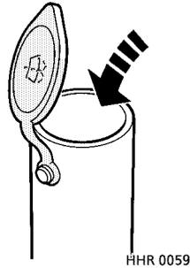
Check the reservoir level every week. To ensure proper cleaning of the windscreen and to prevent freezing in cold weather, top-up with a mixture of water and a proprietary brand of screenwash. Preferably mix the recommended quantities of water and screenwash in a separate container before topping-up the system, and always follow the instructions on the container.
