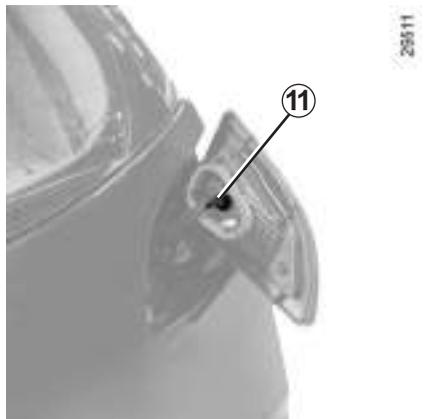
From the outside of the vehicle, pull on the light unit to remove it then unscrew bulb holder **11** a quarter of a turn.
