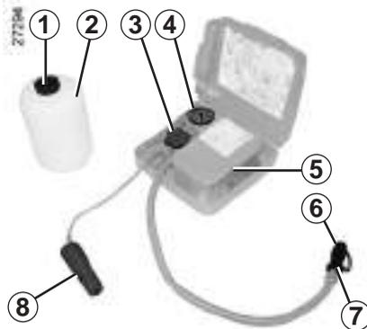
Open the kit, remove caps **1** and **3** (it is **essential** not to remove the cap from the bottle) then screw bottle **2** to its base **3**.
