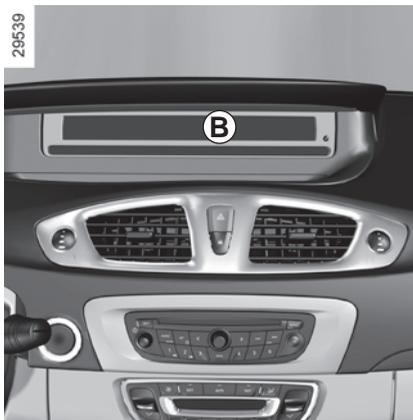
**Dashboard A or B:** lights up when the ignition is switched on.
