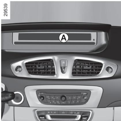
vehicles without “TFT display” instrument panels **A** Display **1** on the instrument panel informs you of any tyre pressure faults (flat tyre, punctured tyre, etc.).
