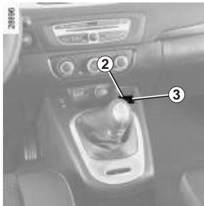
To confirm that the electronic parking brake is applied, the message “Parking brake on” and warning light
