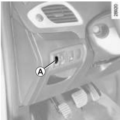
On vehicles fitted with this function, control **A** allows you to adjust the height of the beams according to the load. Turn control **A** downwards to lower the headlights and upwards to raise them. For vehicles not fitted with control **A**, adjustment is automatic.
