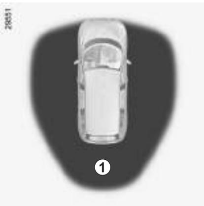
The hazard warning lights **flash twice** and a beep sounds to indicate that the doors have locked.
