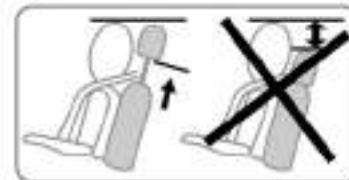
The three upper positions can be manipulated without pressing button **2**. However, it is preferable to press this button to lower the headrest.
