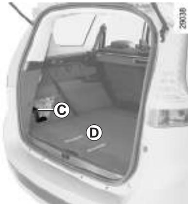
Depending on the vehicle, in the event of a puncture, use the kit located in storage compartment **C** or underneath luggage compartment carpet **D**.
