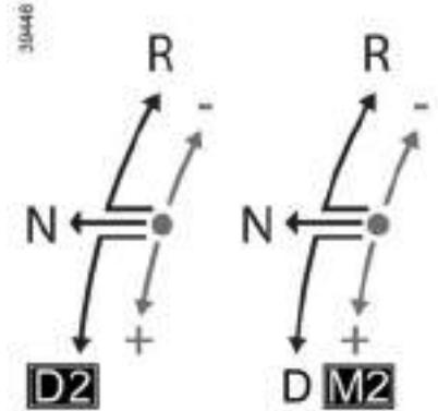
The gear engaged is first displayed to the right of **D** on the instrument panel, then **M** followed by the gear engaged appear under **+** once permanent manual mode is activated.
