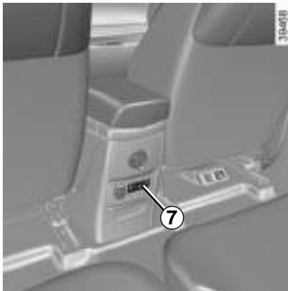
The sockets USB can also recharge accessories with a maximum power rating of 12 Watts (voltage: 5V) per socket, which have been approved by our Technical Department.
