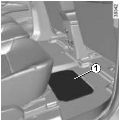
In the event of a puncture, use the kit situated under the second row rear passenger footwell flap **1**.
