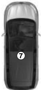
If, **while the engine is running**, a door is opened and closed, and the card is no longer in the zone **7**, the message Keycard not detected indicates that the card is not inside the vehicle. This will, for example, prevent you from driving away after dropping off a passenger who has kept the card on them.
