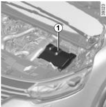
The battery **1** does not require any maintenance.
