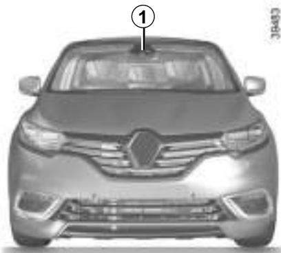
The overspeed alert with signage panel recognition notifies the driver that they are exceeding the speed limit for the section of road on which they are currently travelling.
