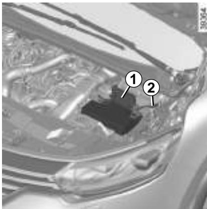
Lift the red cover on box **1** located behind the battery.
