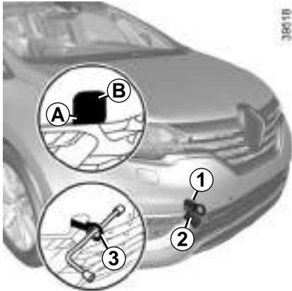
Only use the front **1** and rear **4** towing points (never use the driveshafts or any other part of the vehicle). These towing points may only be used for towing: never use them for lifting the vehicle directly or indirectly.
