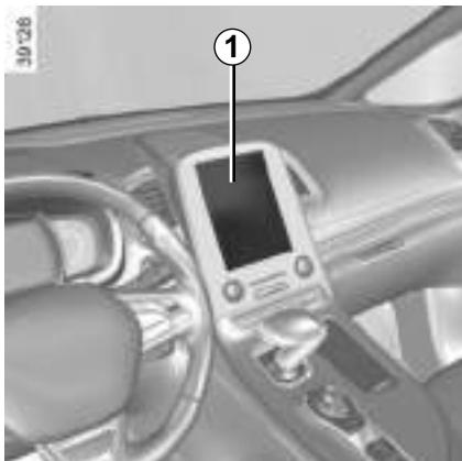
Depending on the vehicle, this function, which is integrated in the multifunction screen **1**, allows you to activate/deactivate and adjust some of the vehicle's functions.
