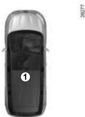
The RENAULT card must be inserted in detection zone **1**.
