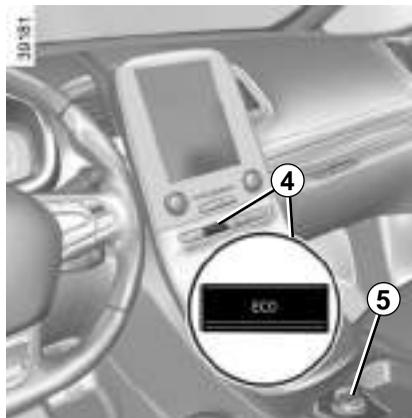
While driving, it is possible to leave the ECO mode temporarily in order to improve engine performance.
