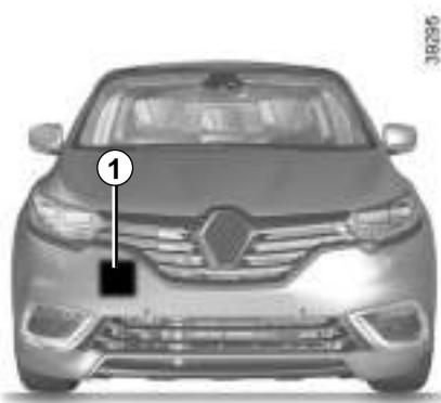
Using the sensor **1**, this function notifies the driver about the time interval separating them from the vehicle in front, so they can respect a safe distance between the two vehicles.
