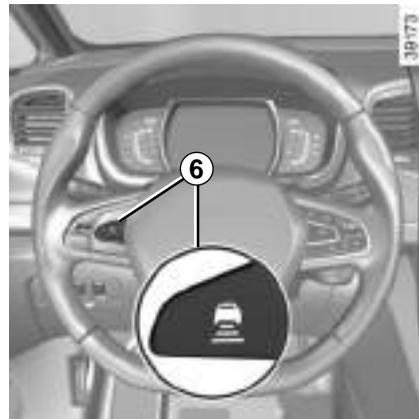
The cruising speed replaces the dashes and cruise control is confirmed by the appearance of the message “Adaptive cruise ctrl” and the warning light
