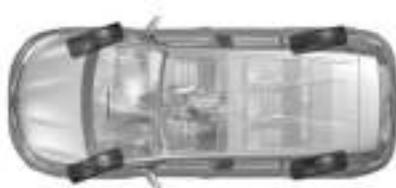
When driving at higher speeds, the rear wheels steer in the same direction as the front wheels (figure **B**) to optimise the vehicle's stability. This is useful when changing lanes or when cornering etc.
