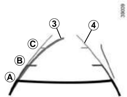
This gauge remains fixed and indicates the vehicle trajectory if the wheels are in line with the vehicle.
