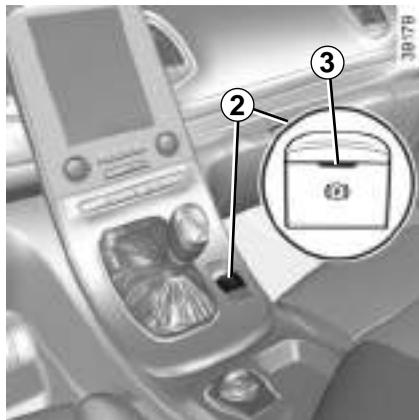
To confirm that the electronic parking brake is applied, the message “Parking brake on” and warning light
