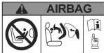
The markings on the dashboard and labels **A** on each side of the passenger sun visor **3** (example: label shown above) remind you of these instructions.
