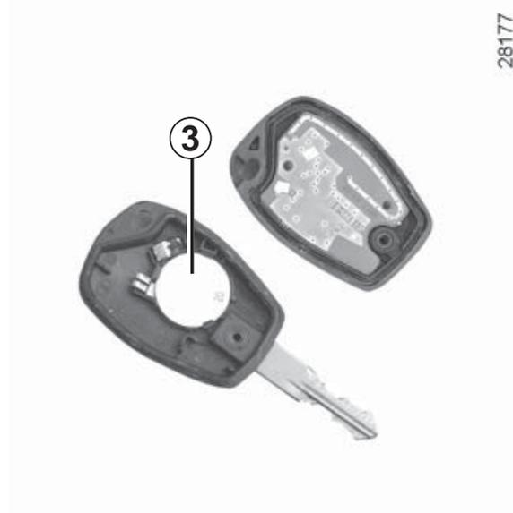
Replace battery **3** according to the direction marked on the cover.
