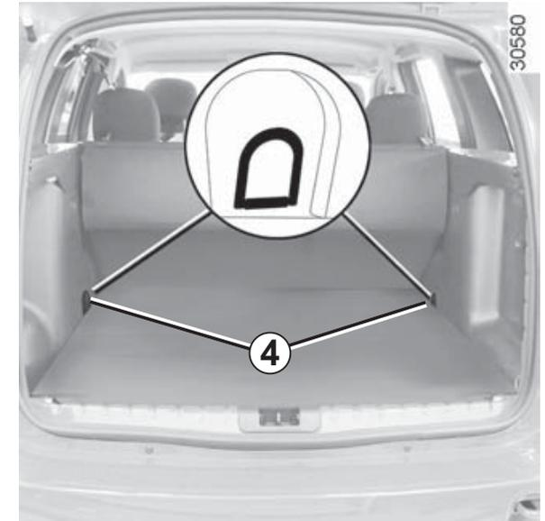
Attach the hook on the belt to one of the rings **3** (4x2 version) or **4** (4x4 version).
