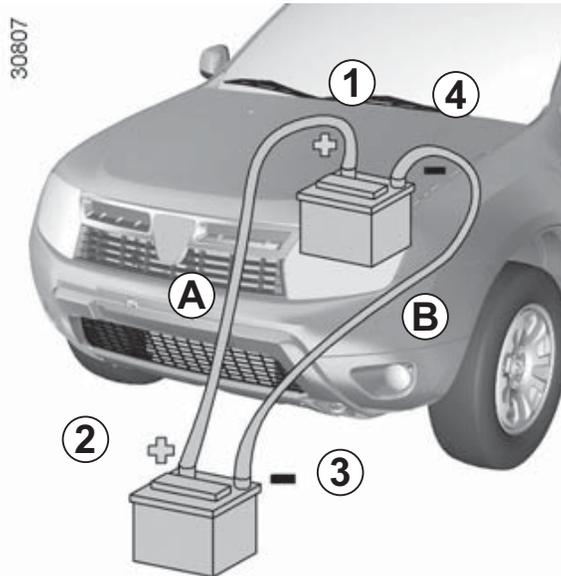
Connect the positive (+) lead **A** to (+) terminal **1** of the discharged battery, then to (+) terminal **2** of the battery supplying the current.
