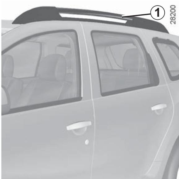
When these are fitted to the vehicle, you can transport luggage or additional accessories (bike rack, ski rack, etc.) on a roof rack or on transverse roof bars attached to the longitudinal roof bars **1** or directly on these bars.
