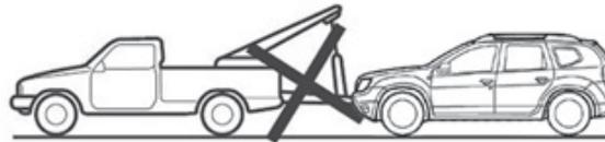
You must never tow a 4-wheel drive vehicle, irrespective of the mode selected, if one of the 4 wheels is in contact with the ground (except for off-road recovery). Risk of mechanical damage.
