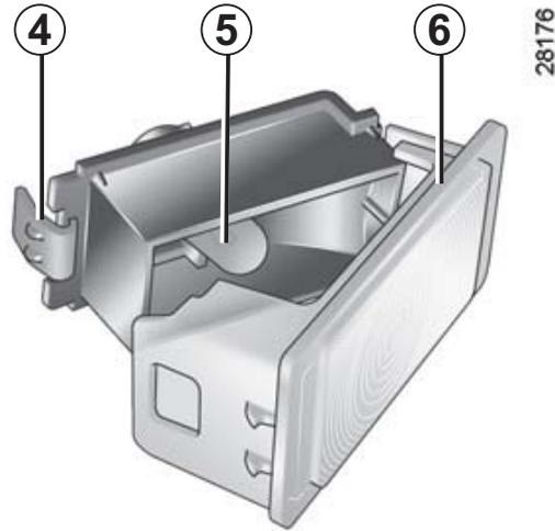
Press tab **4** to release lens **6** and access bulb **5**.
