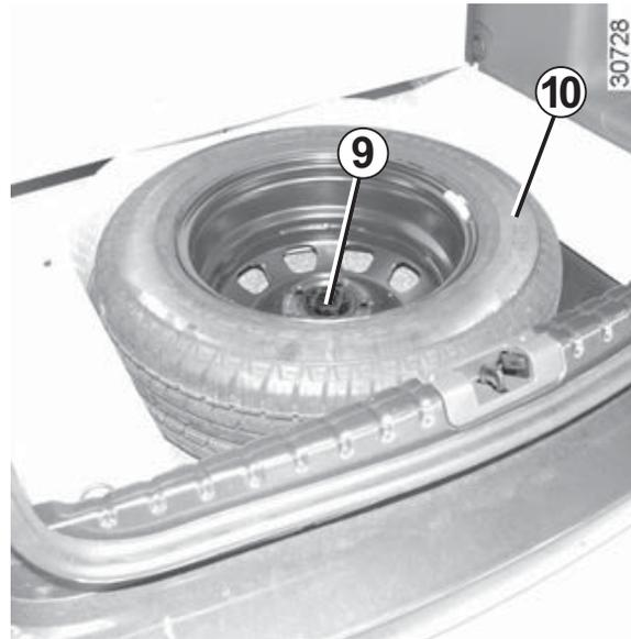
**Note:** ensure that the emergency spare wheel or punctured wheel and the wheel tray are correctly positioned so that the luggage compartment carpet can be properly fitted.
