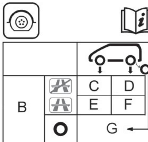
**F:** tyre pressures for the rear wheels (motorway).
