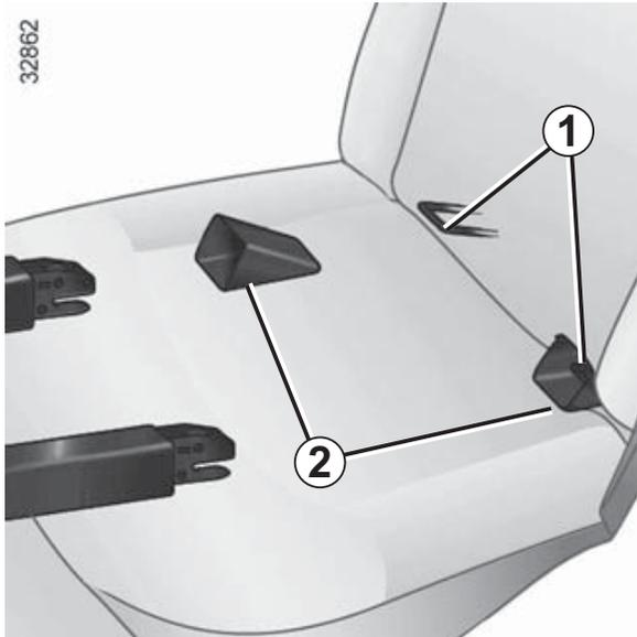
The rings ISOFIX **1** are located between the seatback and the seat base and are clearly visible.
