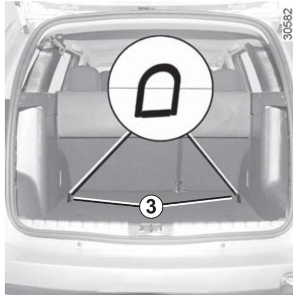
The third ring of each side seat is used to attach the upper strap on some child seats.
