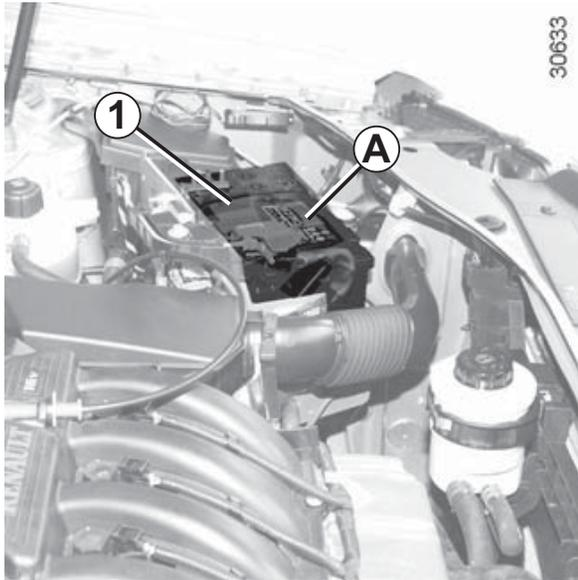
Battery **1** does not require any maintenance.
