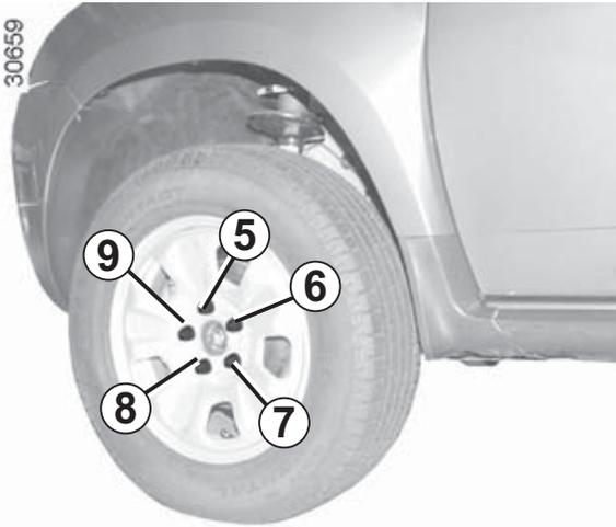
Tighten the bolts, checking that the wheel is correctly positioned on its hub and lower the jack.
