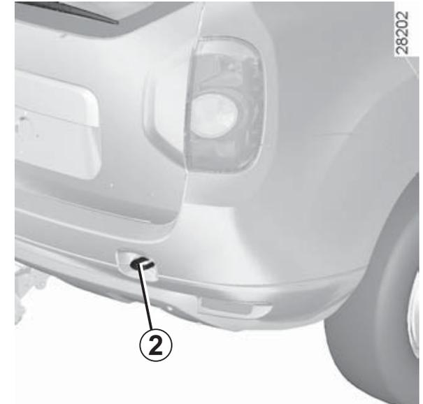
These towing points may only be used for towing: never use them for lifting the vehicle directly or indirectly.
