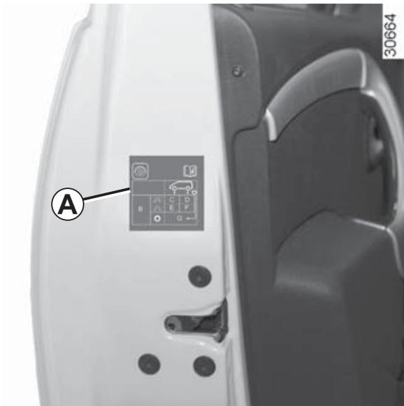
The tyre pressure is indicated on label **A** affixed to the edge of the driver's door. Open the door to read it.
