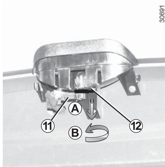
Unclip tab **12** carefully (movement **A**) and turn it an eighth of a turn (movement **B**) to release the bulb holder **11**.
