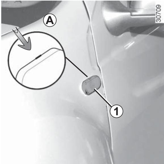
Unclip indicator light **1** (using a flat-blade screwdriver or similar positioned at **A** to move the indicator light towards the outside of the vehicle).
