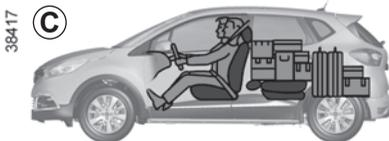
If you have to place objects on the folded seatback, it is necessary that you lower the headrests before folding the seatback so that it can be folded as flat as possible against the seat.
