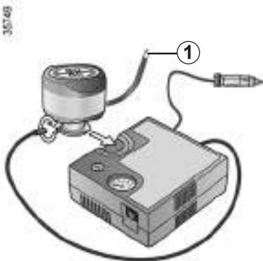
Once the tyre is correctly inflated, remove the kit: slowly unscrew the inflation adapter **1** to prevent any repair product from escaping and store the container in plastic packaging to prevent the product from escaping.
