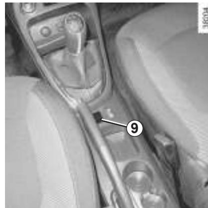
**Vehicles fitted with the ECO mode (button 9):** once activated, the ECO mode may reduce the effective performance of the air conditioning. Please refer to the information on “Eco-driving” in Section 2.
