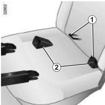
The two rings **1** are located between the seatback and the seat base and are identified by a marking. Use the access guides **2** of the child seat to ease it into place and lock it into the rings **1**. The third ring **4** or **5** is used to attach the upper strap on some child seats.
