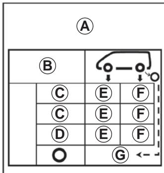
**B:** dimension of the tyres fitted to the vehicle.
