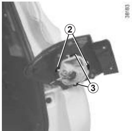
Pull on the outside **A** of the light and remove the rear light unit.
