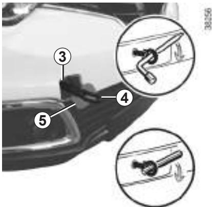
Only use the front **3** and rear **6** towing points (never use the drive shafts or any other part of the vehicle)
