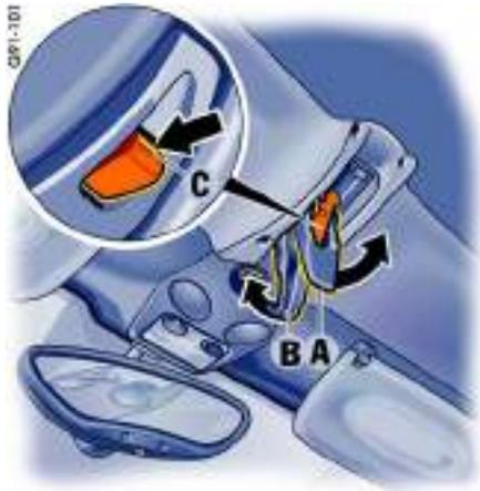
12. Swing locking lever of front latch to the rear (arrow **A**).
