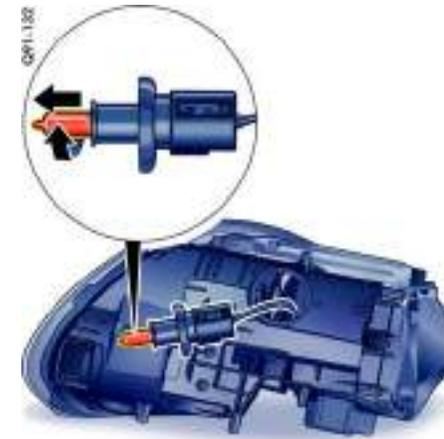
3. Replace the defective bulb (bayonet lock).
