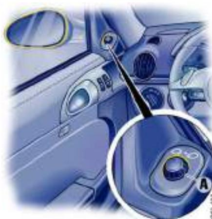
**A** - Control switch for door mirror adjustment
