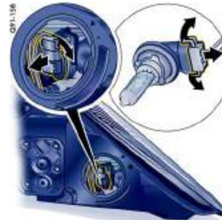
2. Turn bulb holder clockwise and remove it (bayonet lock).
