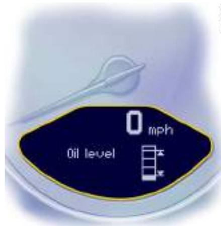
7. If the bottom segment is filled in, the oil level has reached the minimum mark.
