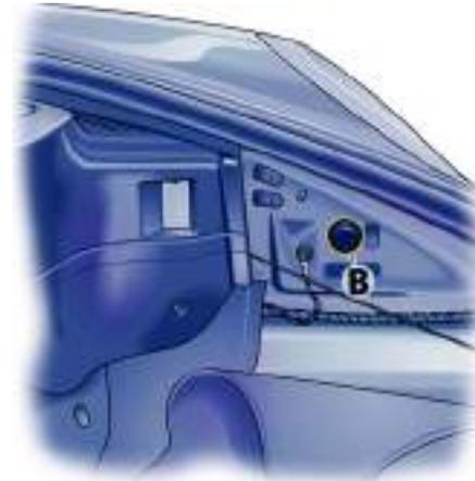
2. Remove rubber plug **B** from the unlocking opening.
