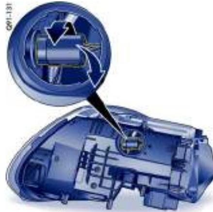
2. Turn bulb holder counter-clockwise and remove it (bayonet lock).
