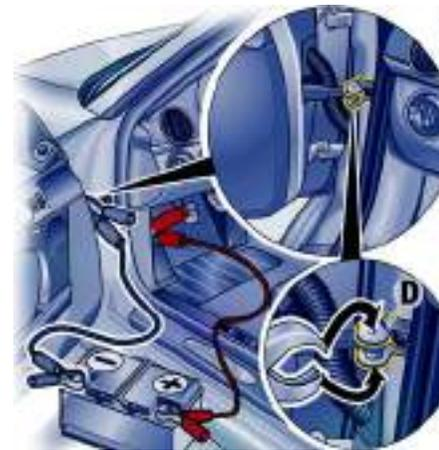
5. Use the black jumper cable to connect the negative terminal of the donor battery to the door arrester **D**.
