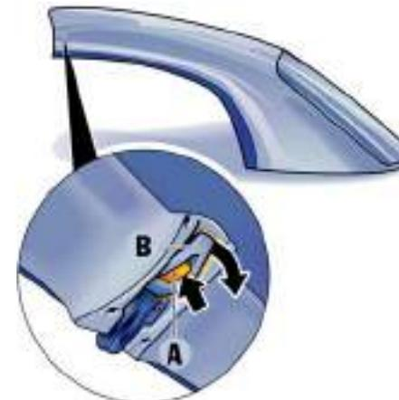
6. Press red locking button of the front locking lever (**arrow A**).
