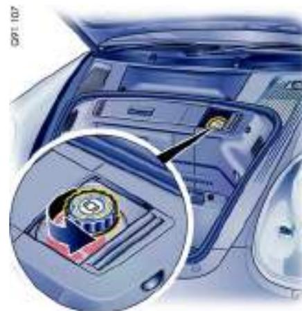
A slight decrease in the fluid level due to wear and automatic readjustment of the disc brakes is normal.
