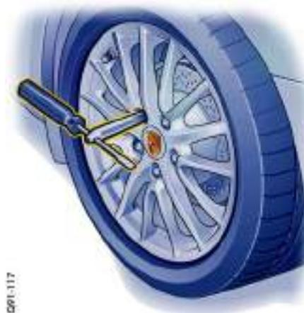
Screw in assembly aid for cars **without** Porsche Ceramic Composite Brake
