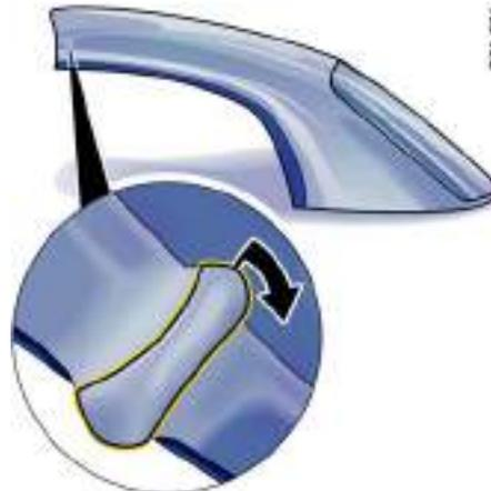
5. Remove cover from front locking lever (**arrow**).
