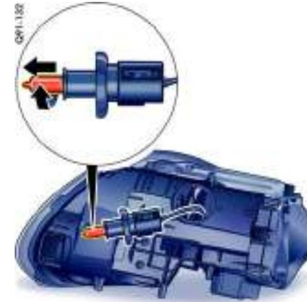
3. Replace the defective bulb (bayonet lock).
