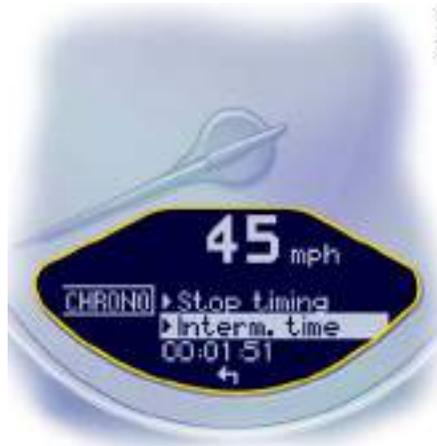
After timing has been started, the on-board computer display changes to the "Stop timing/Intermediate time" selection.
