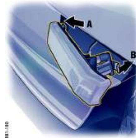
3. Remove side marker and undo bulb holder (bayonet lock).
