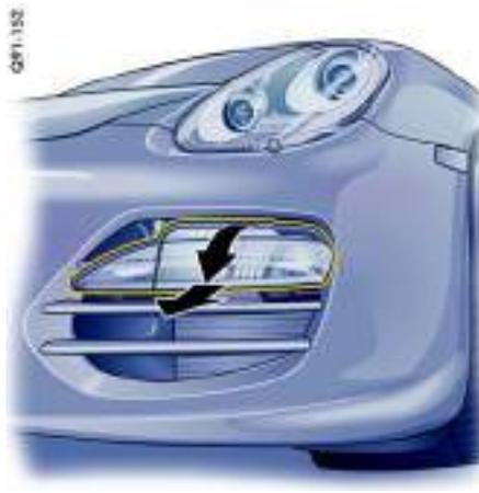
2. Lower headlight slightly and lift it forward and out.
