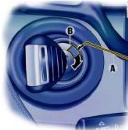
3. Use metal hook **A** to remove the plastic lid **B** from the ignition lock. Make sure that plastic lid **B** is not lost.
