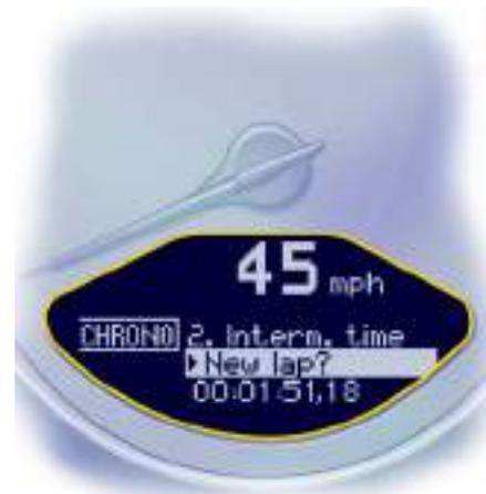
▷ Select "Intermediate time" with the operating lever and push the operating lever forwards. The intermediate time will be displayed for approx. 5 seconds.
