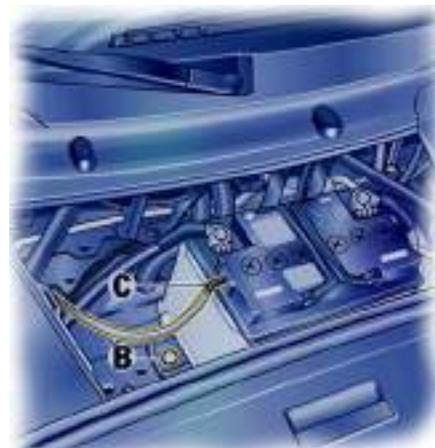
4. Important: disconnect the negative (-) ground wire first, and then the positive (+) cable - danger of short circuit!
