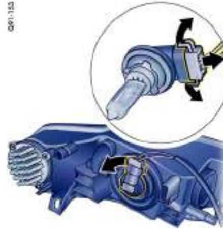
3. Turn bulb holder counter-clockwise and remove it.
