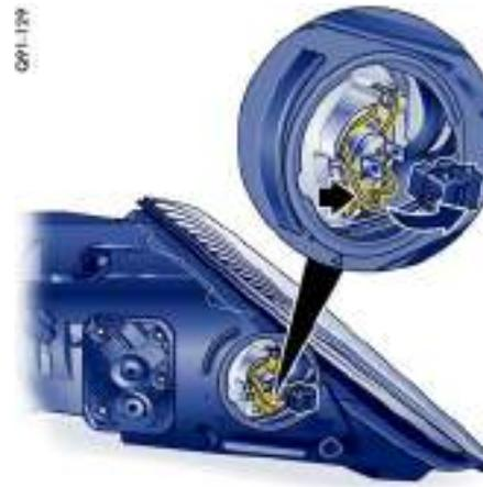
3. Disengage fixing clip.
