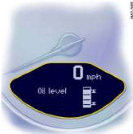
6. If the segments are filled in up to the top line, the oil level has reached the maximum mark. Under no circumstances add engine oil.
