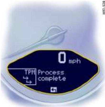
The tire selection has only been successfully completed when the message “Process complete” is displayed by the on-board computer.
