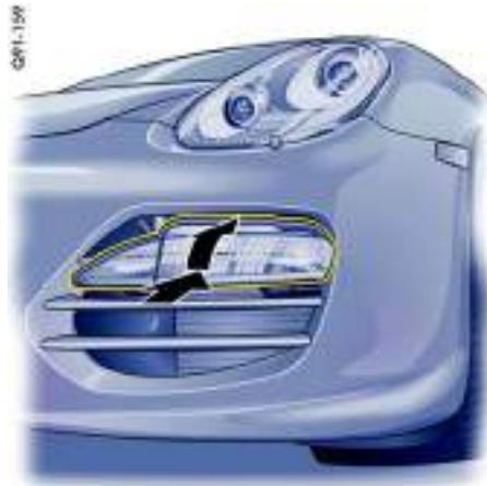
7. Fit headlight housing from underneath at an angle and then swivel it upward.
