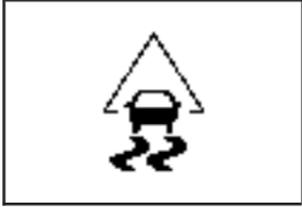
Your vehicle has a Traction Control System (TCS) and StabiliTrak<sup>®</sup> warning light.
