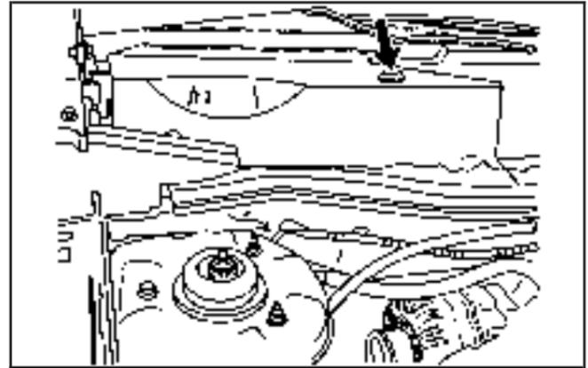
1. The passenger's side air inlet panel is located below the center of the passenger's side wiper blade. Remove the push pin retaining the air inlet panel. Pry the center of the push pin out 0.5 in (13 mm) for removal.
