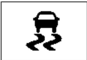
TCS can be turned off by pressing the StabiliTrak/TCS button, located next to the gear shift lever.
