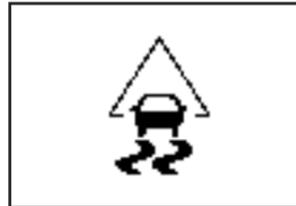
The StabiliTrak/TCS warning light on the instrument panel cluster will flash when the system is operating.
