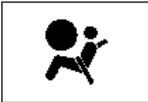
If the airbag readiness light stays on after you start the vehicle or comes on when you are driving, your airbag system may not work properly. Have your vehicle serviced right away.
