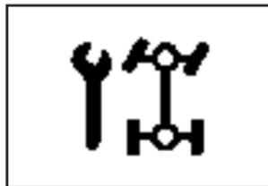
The Service All-Wheel Drive Light is located on the instrument panel cluster.
