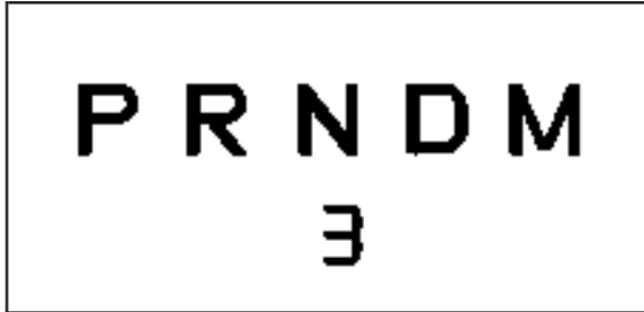
There are several different positions for the shift lever. When using the MSM (Manual Shift Mode), a number indicating the gear selected will appear on the instrument cluster below the shift position display. For more information on the manual shift option see “Manual Shift Mode” in this section.
