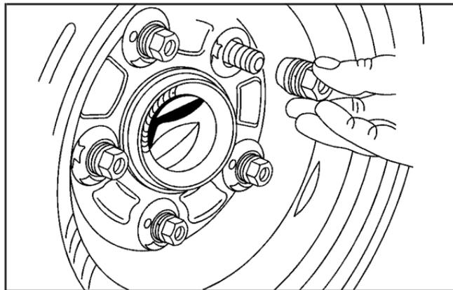
9. Put the wheel nuts back on with the rounded end of the nuts toward the wheel. Tighten each nut by hand until the wheel is held against the hub.
