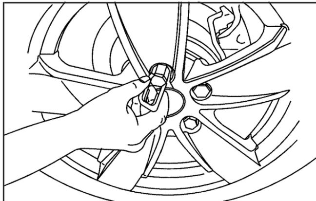
1. Remove each wheel nut cap individually with the wheel nut cap tool provided. Insert the nut cap tool into the nut cavity, squeeze the tool to grasp the nut cap, and pull out to remove it. Store the nut caps in a clean area to avoid dirt getting into them.
