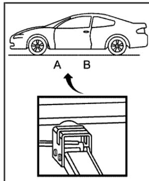
3. Fit the jack handle onto the jack by sliding the open end of the handle over the nut end of the jack. Position the jack and raise the jack head until it fits firmly into notches A and B in the vehicle's frame closest to the tire being changed.
