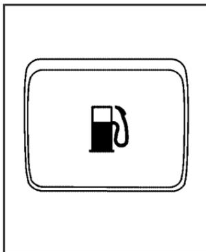
The fuel release button is located on the instrument panel to the left of the steering wheel. Push the button to release the fuel door.
