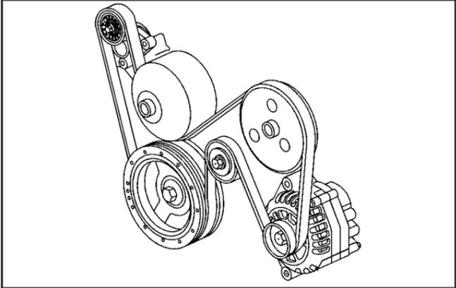
Power Steering/Generator Belt Routing
