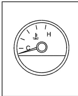
The temperature gage shows the engine coolant temperature when the ignition is on.
