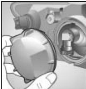
2. Turn the dust caps counterclockwise and remove from the rear of the headlamp assembly to gain access to the bulb.
