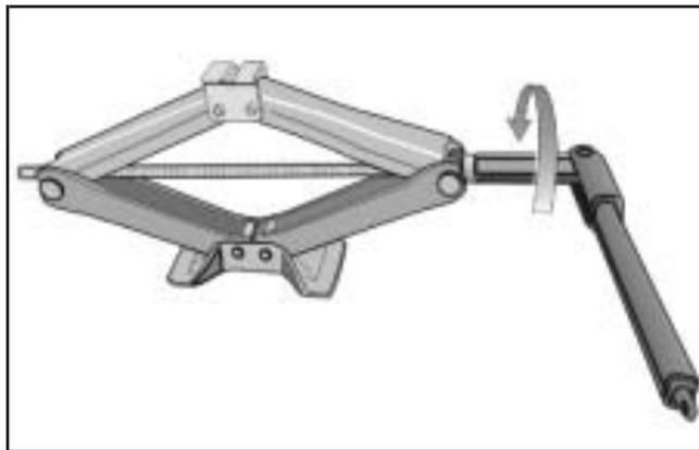
4. Raise the vehicle by turning the wheel wrench clockwise. Raise the vehicle far enough off the ground so there is enough room for the compact spare tire to fit underneath the wheel well.
