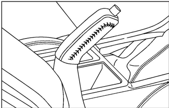
To set the parking brake, pull up on the parking brake handle without pressing the release button. If the ignition is on, the brake system warning light will come on. See *Brake System Warning Light* on page 3-27.
