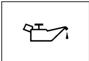
If you have a low engine oil pressure problem, a Check Oil message in the trip computer display along with this symbol will stay on after you start your engine, or come on when you are driving.
