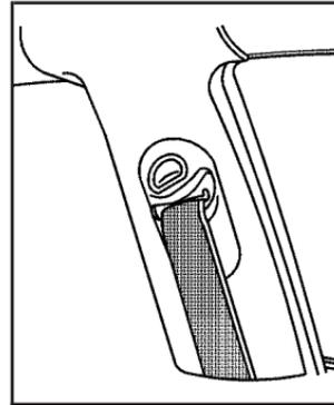
To move it up or down, squeeze the adjuster as shown and move it to the desired position. After you move the adjuster to where you want it, try to move it without squeezing it, to make sure it has locked into position.
