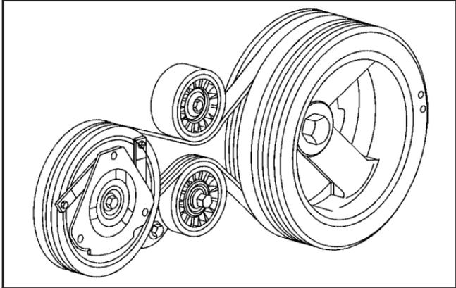
Air Conditioning Compressor Belt Routing
