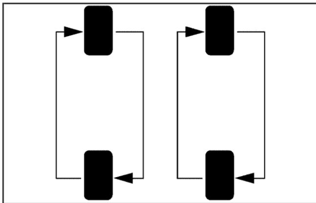
If your vehicle has 235/40ZR18 tires, they must roll in a certain direction for the best overall performance. The direction is shown by an arrow on the tire sidewall. Because these tires are uni-directional, they should be rotated as shown here. These tires should only be moved from front to rear and rear to front on the same side of the vehicle.
