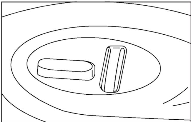
The power front seat controls are located on the outboard side of the driver's and passenger's seat.
