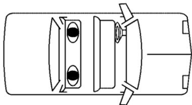
Your vehicle has the LATCH system. You will find anchors (A) for the two rear seat positions.
