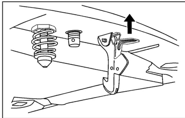
2. Then go to the front of the vehicle and pull up on the secondary hood release.
