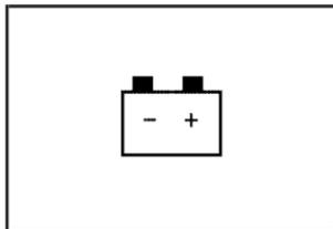
The charging system light will come on when you turn on the ignition, until the engine is started, as a check to show you it is working.
