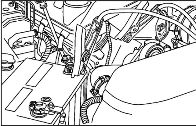
Don't let the other end touch anything until the next step. The other end of the negative (-) cable does not go to the dead battery. It goes to a heavy, unpainted metal engine part or to a remote negative (-) terminal on the vehicle with the dead battery.
