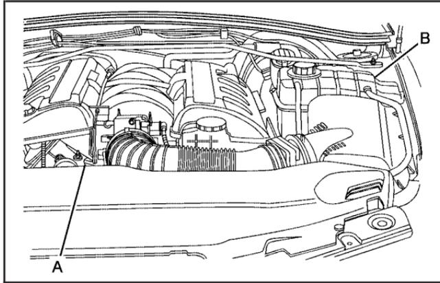
When you decide it's safe to lift the hood, you'll see the electric engine cooling fan (A) and the engine coolant reservoir (B).
