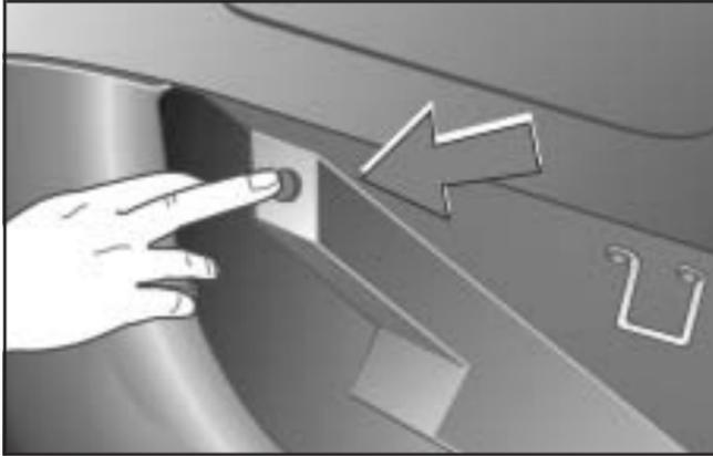
Push the button in the glovebox to unlock the trunk, provided you are not traveling over 12 mph (20 km/h) or the alarm system is on. Then from the outside, lift up the trunk. For added vehicle security, the glovebox button is disabled when all the doors are locked with the LOCK button on the key or through the door lock.
