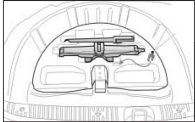
3. Remove the jack, wheel wrench, and nut cap removal tool from storage. Your vehicle's jack, wheel wrench, and nut cap removal tool are stored in a container in the floor, under the spare tire.
