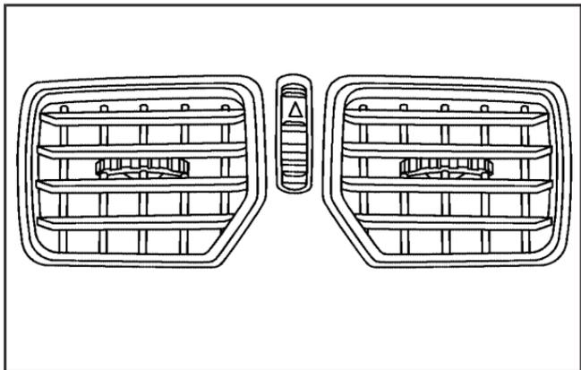
Move the thumbwheel on the vents to change the direction of the airflow. The center thumbwheel adjusts the volume of the airflow.
