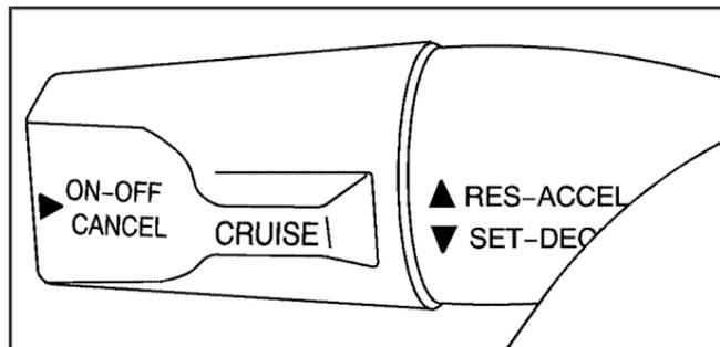
With cruise control, you can maintain a speed without keeping your foot on the accelerator. This can really help on long trips. Cruise control does not work unless the vehicle speed is at least 25 mph (40 km/h).
