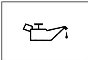
If the Service Engine Oil message in the trip computer is displayed along with this symbol after you start the engine, it means that service is required for your vehicle.
