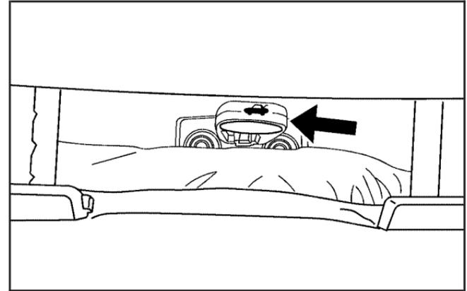
There is also a secondary trunk release handle located under the passenger's side rear seat head restraint. To access this handle, when the vehicle is not moving, lift the head restraint and pull the yellow ring towards the front of the vehicle.
