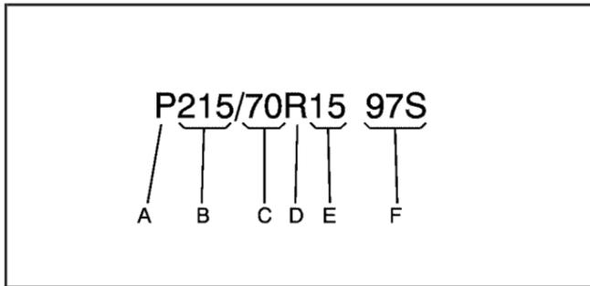
**(A) Passenger (P-Metric) Tire:** The United States metric tire sizing system uses the letter "P" to designate a passenger vehicle tire. The European metric tire sizing system does not use the letter "P" to designate a passenger vehicle tire.
