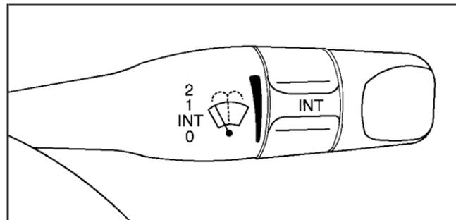
The lever on the right side of the steering column operates the windshield wipers and washer.
