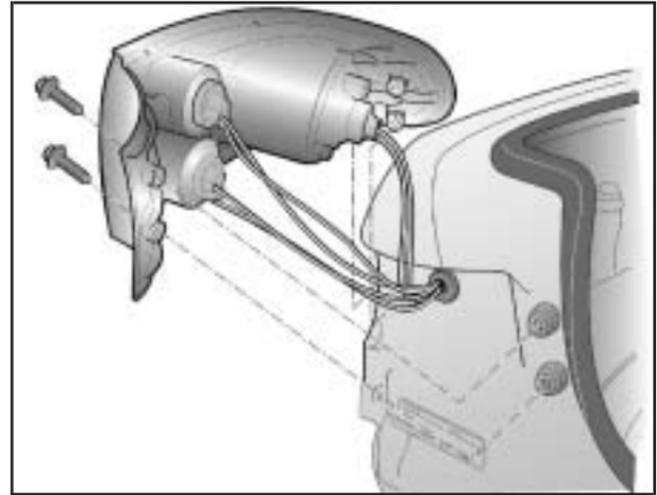
2. Remove the two screws that attach the taillamp assembly to the vehicle.
