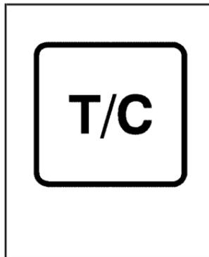
To turn the system off, press the T/C button. On manual transmission vehicles the button is located on the driver's side of the center console. On automatic transmission vehicles the button is located on the passenger's side of the shift lever.
