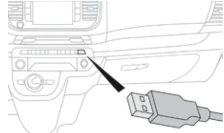
It allows the connection of a portable device, such as a digital audio player of the iPod® type or a USB memory stick.
