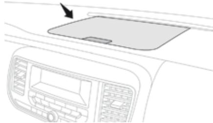
Press the control to open the lid (depending on version) then guide it to its fully open position. To close, guide the lid then press the centre gently. Any liquid which could spill risks causing an electrical short circuit and therefore a potential fire.
