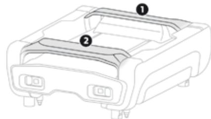
**i** As a safety measure, the bars 1 and 2 prevent the box escaping from its housing, if it is not correctly secured.
