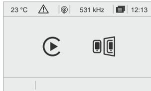
Operate certain applications on a smartphone connected via MirrorLink™ or CarPlay®. Check the state of Bluetooth and Wi-Fi connections.
