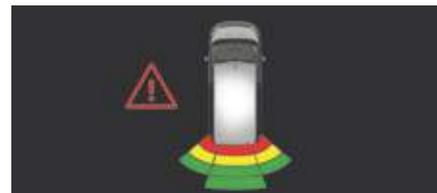
This supplements the audible signal by displaying bars in the screen or the instrument panel which move progressively nearer to the vehicle. When the obstacle is near, the "Danger" symbol is displayed.
