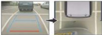
This mode is activated by default. Using sensors in the rear bumper, the automatic view allows a change from the rear view to the view from above as an obstacle is approached during a manoeuvre.
