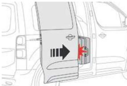
The obstacle detection system is triggered when the moving door encounters an obstacle with a certain level of physical resistance.
