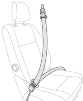
The front seat belts are fitted with a pretensioning and force limiting system. This system improves safety in the front seats in the event of a front or side impact. Depending on the severity of the impact, the pretensioning system instantly tightens the seat belts against the body of the occupants.
