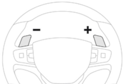
You can temporarily take control of gear changes using the "+" and "-" steering mounted control paddles. The gear change instruction is acted on if the engine speed permits. This function allows you to anticipate certain situations, such as overtaking another vehicle or approaching a bend in the road. Following a few moments with no action on the control paddles, the gearbox returns to automatic operation.
