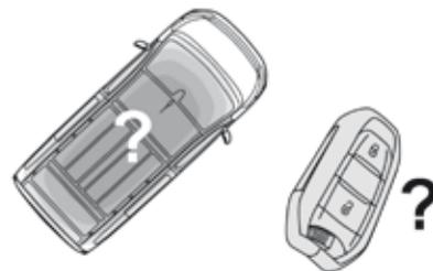
If the remote control is no longer in the recognition zone when you close a door or when you (later) request switching off the engine, a message appears in the instrument panel.
