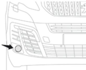
With dipped or main beams, this function makes use of the beam from a front foglamp to illuminate the inside of a bend, when the vehicle speed is below 25 mph (40 km/h) (urban driving, winding road, intersections, parking manoeuvres...).
