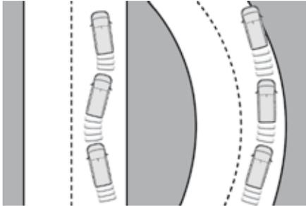
Using a camera placed at the top of the windscreen, the system assesses the driver's level of vigilance by identifying variations in trajectory compared to the lane markings. This system is particularly suited to fast roads (speed higher than 40 mph (65 km/h)).
