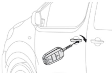
☞ To unlock the vehicle **totally**, turn the key to the rear of the vehicle.
