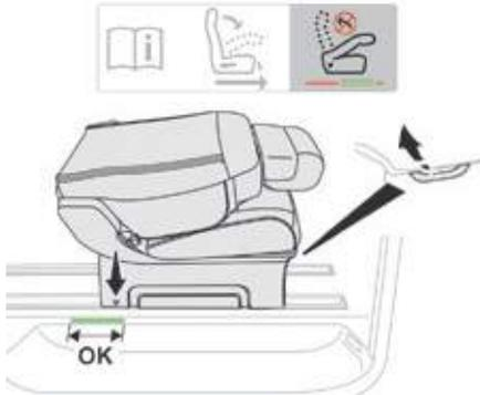
To return the backrest to the normal position, the seat must be positioned between the markings.
