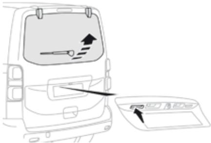
After unlocking the vehicle using the key, remote control or Keyless entry and Starting (depending on equipment) press this control and raise the rear screen to open it.
