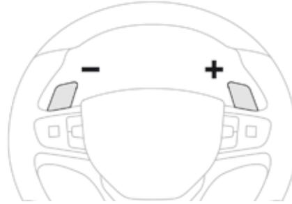
You can temporarily take control of gear changes using the "+" and "-" steering mounted control paddles. The gear change instruction is acted on if the engine speed permits. This function allows you to anticipate certain situations, such as overtaking another vehicle or approaching a bend in the road. Following a few moments with no action on the control paddles, the gearbox returns to automatic operation.
