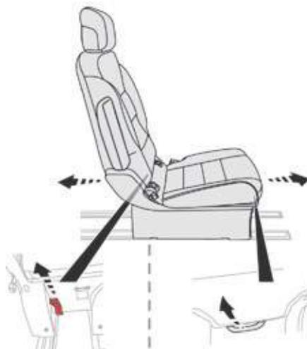
Two controls are provided for moving the seat forward and backward:
