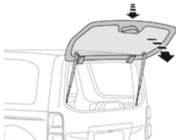
Close the rear screen by pressing the centre of the glass until it is fully closed.
