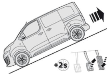
**On a descending slope, with the vehicle stationary and reverse gear engaged, the vehicle is held momentarily when you release the brake pedal.**
