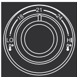
☞ Turn the knob from "**LO**" (cold) to "**HI**" (hot) to adjust the temperature to your requirements.
