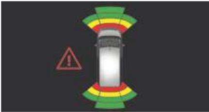
As an addition to the rear parking sensors, the front parking sensors are triggered when an obstacle is detected in front and the speed of the vehicle is still below 6 mph (10 km/h).
