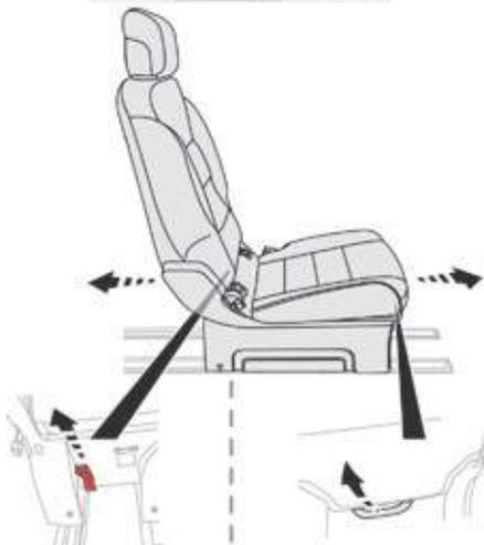
Two controls are provided for moving the seat forwards and backwards:
