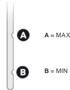
If you find that the level is above the **A** mark or below the **B** mark, **do not start the engine.**
