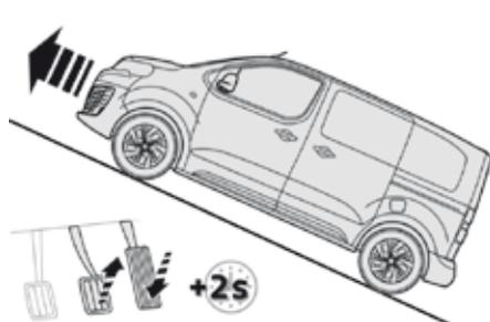
**On an ascending slope, with the vehicle stationary, the vehicle is held for a momentarily when you release the brake pedal.**
