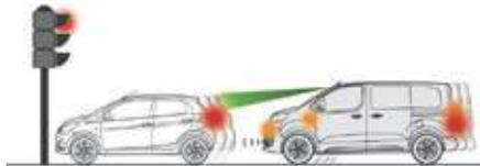
This system, also called automatic emergency braking, aims to reduce the speed of impact or avoid a frontal collision by your vehicle (between 3 and 87 mph (5 and 140 km/h) where the driver fails to react. Using a radar and a camera, this system acts on the vehicle's braking system.
