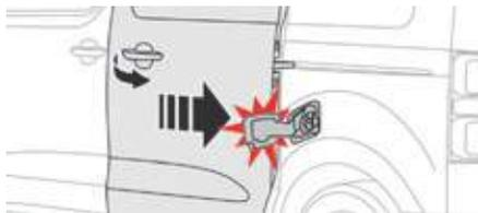
**!** If your vehicle has sliding side doors, do not open the left hand sliding door as there is a risk of damaging the fuel filler flap when refuelling.
