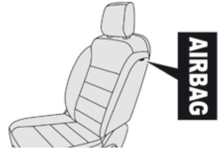
If fitted to your vehicle, this is a system which protects the driver and front passenger in the event of a serious side impact in order to limit the risk of injury to the chest, between the abdomen and head.
