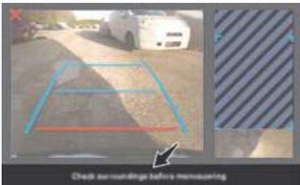
This mode displays, as quickly as possible, the contextual view (left-hand part) and the view from above the vehicle.
