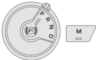
Before switching off the engine, select position **P** then apply the parking brake to immobilise the vehicle.
