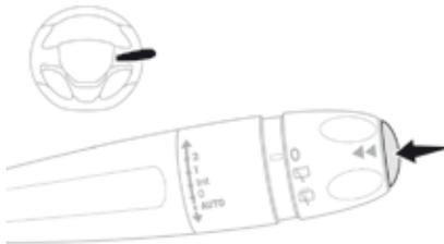
☞ Press the button on the end of the **wiper control stalk** to display the different trip computer tabs in turn.
