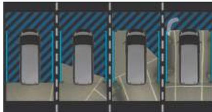
Using the rear camera, the system records the vehicle's surroundings during a manoeuvre. An image from above your vehicle in its close surroundings is reconstructed (represented between the blue brackets) in real time and as the manoeuvre progresses.
