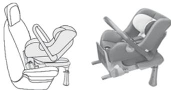
Installed rearward facing using an ISo FIX base which is attached to the rings **A**. The base has a support leg, adjustable for height, which sits on the vehicle's floor. This seat can also be secured with a seat belt. In this case only the seat shell is used and is attached to the vehicle's seat by the three-point seat belt.
