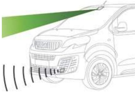
These systems use a radar located in the front bumper and a camera at the top of the windscreen.
