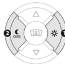
☞ With the engine running, press button **1** to activate the system and deploy the blade.
