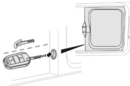
**ⓘ** Lock/unlock the system using the remote control or the back-up key of the Keyless entry and Starting system.
