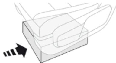
The tool box is located under the left-hand front seat.
