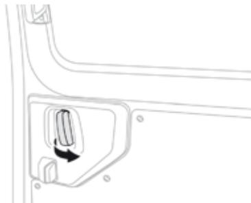
To hold the sliding side door in the open position, open the door fully to engage the latch (located at the bottom of the door).
