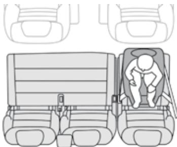
When a rearward facing child seat is installed **on a rear passenger seat**, move the vehicle's front seat forward and straighten the backrest so that the rearward facing child seat does not touch the vehicle's front seat.
