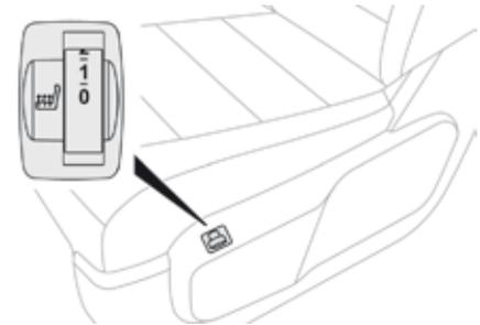
☞ Use the adjustment wheel to switch on and select the level of heating required:
