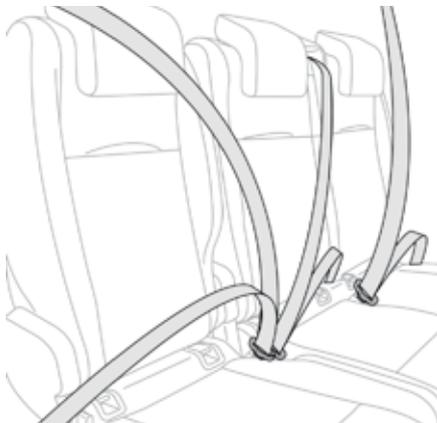
If your vehicle is fitted with a 3-seat bench seat (one piece or 1/3 - 2/3 split), these are fitted with three-point seat belts and inertia reels on the outer seats.
