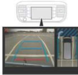
The system displays the contextual view (left-hand part) as well as the view from above the vehicle in its close surroundings. By default, automatic mode is activated. In this mode, the system chooses the best view to display (standard or zoom) according to the information received from the parking sensors. The 180° view is only available through the menus.
