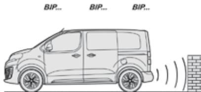
The proximity information is given by an intermittent audible signal, the frequency of which increases as the vehicle approaches the obstacle.
