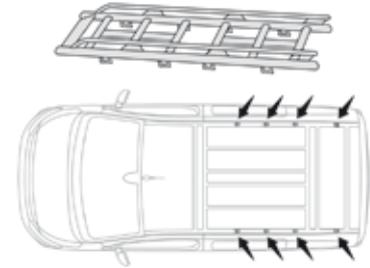
To fit a roof rack, use the fixing points provided for this purpose:
