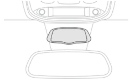
This mirror, placed on top of the central mirror, enables the driver or front passenger to observe all the rear seats. Fitted on its own ball joint, its manual adjustment is simple and provides a view of the rear interior of the vehicle. It can also be adjusted for improved visibility during manoeuvres or when overtaking.
