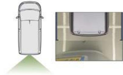
The camera records the surroundings during a manoeuvre in order to create a reconstruction of the view from above the rear of the vehicle in its close surroundings, allowing the vehicle to be manoeuvred among the obstacles nearby. This view is available with Au To view or by selecting of the view in the change view menu.
