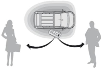
This allows the unlocking, locking and starting the vehicle while keeping the remote control on your person.
