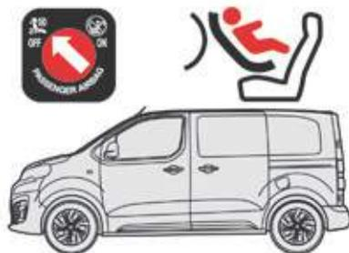
When a rearward facing child seat is installed on the **front passenger seat**, adjust the seat to the fully back and highest position, with the backrest straightened. The passenger's front airbag must be deactivated. **Otherwise, the child risks being seriously injured or killed if the airbag is deployed.**
