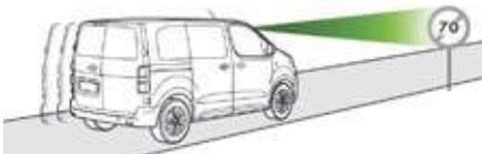
Depending on equipment, using a camera at the top of the windscreen, this system detects and reads speed limit and end of speed limit signs.
