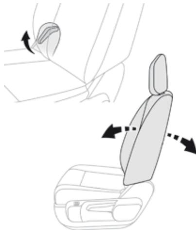
☞ Pull the control fully up and move the backrest forward or backward.
