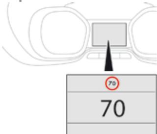
This system allows the speed limit detected by the camera to be displayed in the instrument panel.
