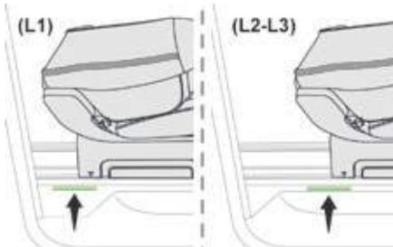
☞ Use the front control to move the seat so that it is between the markings.
