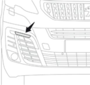
If fitted to your vehicle, contact a Peugeot T dealer or a qualified workshop for the replacement of this type of LeD lamp and light guide.
