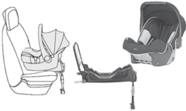
Installed rearward facing using an ISofix base which is attached to the rings **A**. The base has a support leg, adjustable for height, which sits on the vehicle's floor. This child seat can also be secured with a seat belt. In this case, only the shell is used and attached to the vehicle's seat by the three-point seat belt.
