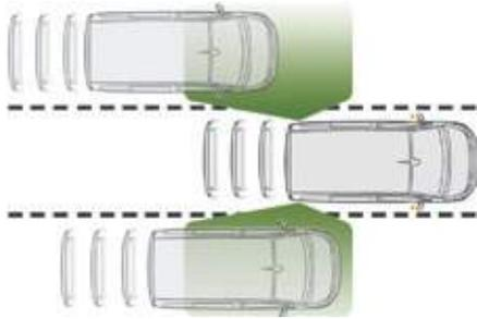
This driving assistance system warns the driver of the presence of another vehicle in the blind spot angle of their vehicle (areas masked from the driver's field of vision), as soon as this presents a potential danger.
