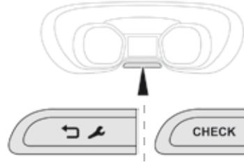
After each service, the service indicator must be reset to zero. If you have carried out the service on your vehicle yourself, switch off the ignition:
