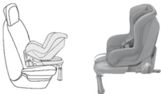
Installed rearward facing using an ISO FIX base which is attached to the rings **A**. The base has a support leg, adjustable for height, which sits on the vehicle's floor. This child seat can also be used forward facing.
