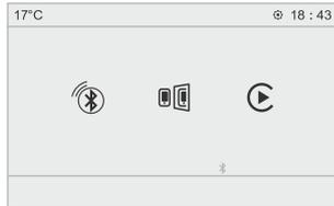
Connect a telephone by Bluetooth®. operate certain applications on a smartphone connected via MirrorLink™ or CarPlay®.
