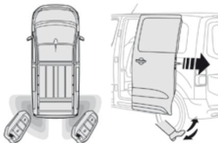
By keeping the remote control on your person and with a movement of your foot, the system unlocks and opens the sliding side door or closes and locks it.
