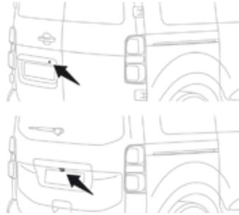
This system allows the near surroundings of the vehicle to be viewed in the display screen using cameras located at the rear of the vehicle. The parking sensors in the rear and/or front bumper complete the information on the view from above the vehicle (right-hand part).
