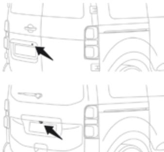
The visual aid reversing camera is activated automatically when reverse gear is engaged.
