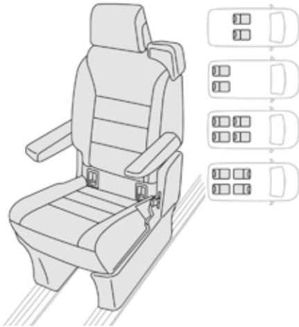
The individual seat is fitted with a three-point inertia reel seat belt.
