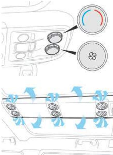
If your vehicle is fitted with a rear air conditioning unit, located in the roof, this system allows the distribution of air conditioned and heated air via ducting and individual outlets.
