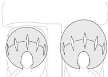
System which protects the driver and passenger(s) in the event of a serious front impact in order to limit the risk of injury to the head and thorax.
