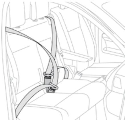
If your vehicle is fitted with a front bench seat, ensure that each belt is used with its correct buckle.
