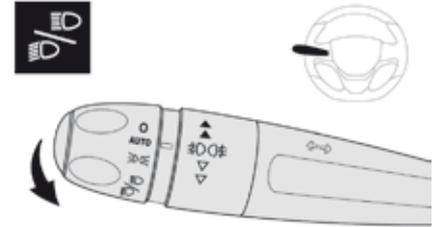
Pull the stalk to switch between dipped and main beam headlamps.
