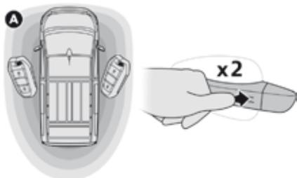
**!** Deadlocking renders the exterior and interior door controls inoperative. It also deactivates the manual central locking button. Therefore, never leave anyone inside the vehicle when it is deadlocked.
