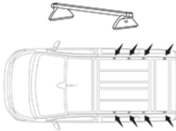
To fit the transverse roof bars, use the fixing points provided for this purpose:
