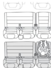
If fitted to your vehicle, when a child seat is installed on a passenger seat in the 3<sup>rd</sup> row, move the seats in the 2<sup>nd</sup> row forward and straighten the backrests so that the child seat and the child's legs do not touch the seats in the 2<sup>nd</sup> row.
