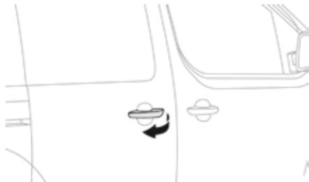
☞ After unlocking the vehicle (using the key, remote control or Keyless entry and Starting, depending on equipment) pull the door handle.
