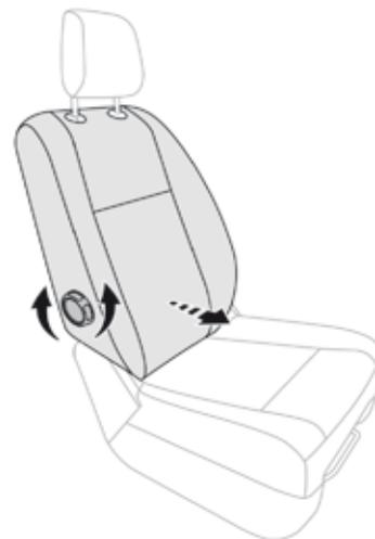
☞ Turn the knob manually to obtain the desired level of lumbar support.
