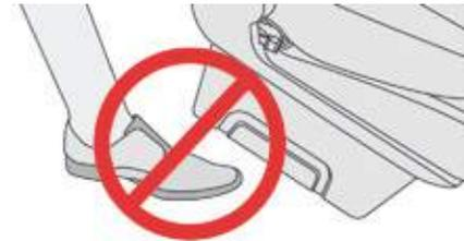
**!** ensure that no object, or the feet of a passenger seated at the rear, could obstruct the anchorage points or prevent the correct latching of the assembly.
