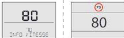
On detection of speed limit information, the system displays the figure.
