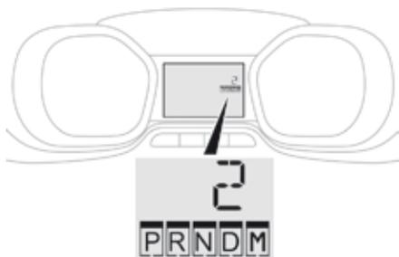
When you move the gear selector or press the **M** button, the corresponding symbol appears in the instrument panel.
