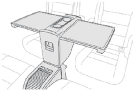
It comprises a central storage space closed with a lid. Unfolded, it offers a table with two tops on which objects can be placed. The central area includes two cup holders and can also be used to place small objects (credit card, pen, ...).
