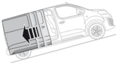
It is possible to open and close the doors electrically on slopes of up to 20%.
