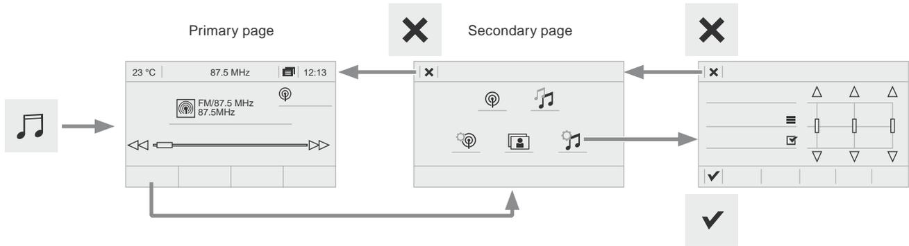
Short-cuts: using the virtual buttons in the upper band of touch screen, it is possible to go directly to the selection of audio source, the list of stations (or titles, depending on the source), message notifications, emails, mapping updates and, depending on services, navigation notifications.
