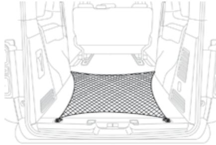
Attached to the stowing rings on the rear floor, it allows objects to be held down.
