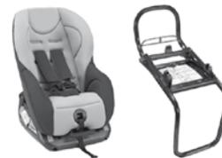
Can be installed forward facing or rearward facing using an ISo FIX base which is attached to the rings **A**. The base includes a support leg which extends down to the floor of the vehicle. 6 seat body angle positions. This child seat can also be used in a forward facing position on seats not fitted with ISo FIX mountings. In this case, it must be secured to the vehicle seat by the three-point seat belt. Adjust the front seat of the vehicle so that the child's feet do not touch the backrest.
