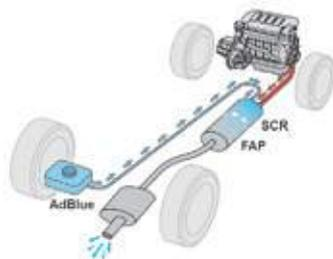
To assure respect for the environment and conformity with the new euro 6 emissions standard, without adversely affecting the performance or fuel consumption of Diesel engines, Peugeot T has taken the decision to equip its vehicles with an effective system that associates SCR (Selective Catalytic Reduction) with a particle filter (FAP) for the treatment of exhaust gases.
