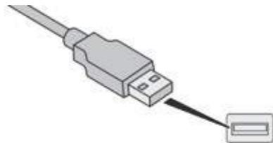
Insert the uSB memory stick in the uSB port or connect the uSB device to the uSB port using a suitable cable (not supplied).
