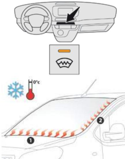
In area 1, the heating frees the wiper blades when they are stuck by snow or ice.
