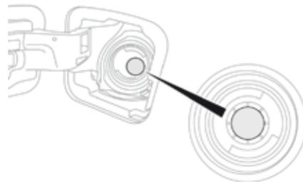
When a petrol filler nozzle is introduced into the fuel filler neck of your Diesel vehicle, it comes into contact with the flap. The system remains closed and prevents filling.
