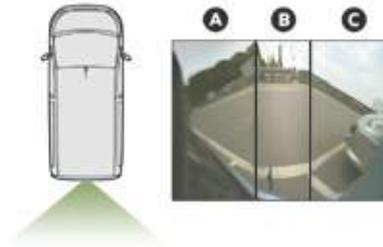
180° view makes it possible to reverse out of a parking space while being able to see the arrival of vehicles, pedestrians or cyclists. This view is not recommended for carrying out a complete manoeuvre. It is made up of the following:
