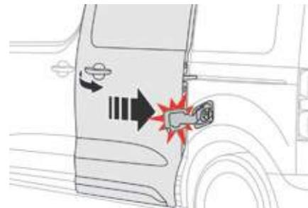
**!** If fitted to your vehicle, never open the left-hand sliding side door when the fuel filler flap is open. Otherwise you risk damaging the fuel filler flap and the sliding door and causing injury to the person filling the vehicle.
