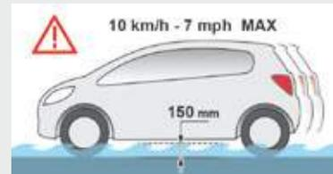
Before driving through a flooded road, it is strongly recommended that you deactivate the Stop & Start system. For more information on **Driving advice**, particularly on flooded roads, refer to the corresponding section.
