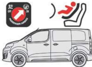
When a forward facing child seat is installed on the **front passenger seat**, adjust the vehicle's seat to the fully back and highest position with the seat backrest straightened and leave the passenger's front airbag activated.
