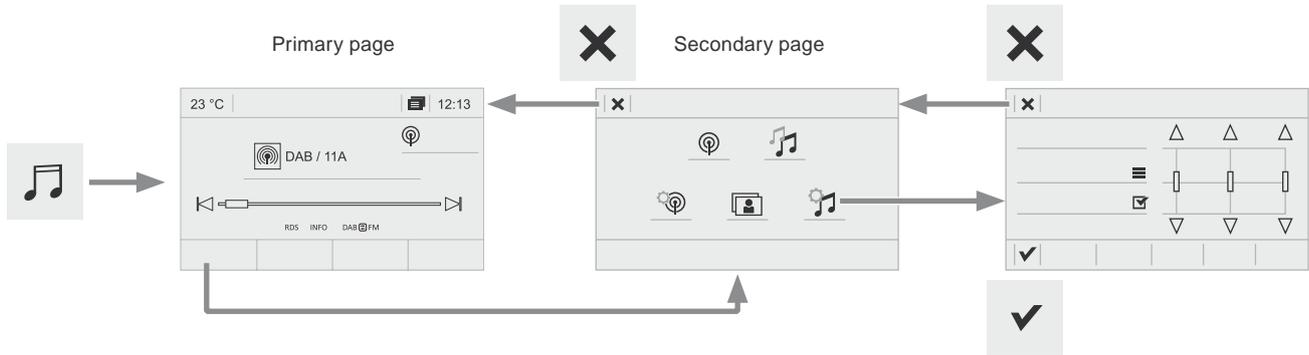
Short-cuts: using the virtual buttons in the upper band of touch screen, it is possible to go directly to the selection of audio source, the list of stations (or titles, depending on the source), message notifications and emails.
