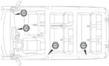
☞ To connect a 12 V accessory (maximum power: 120 Watts), lift the cover and connect a suitable adaptor.
