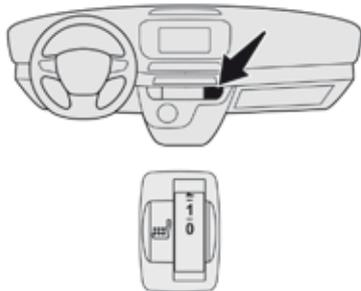
With the engine running, the bench seat cushions can be heated.
