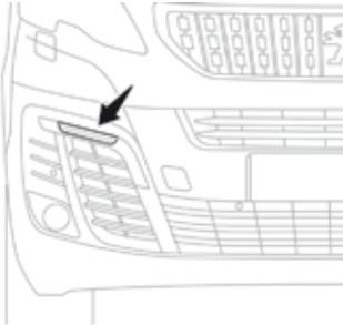
If fitted to your vehicle, they come on automatically when the engine is started, when the lighting control stalk is in position "0" or "AUTO".
