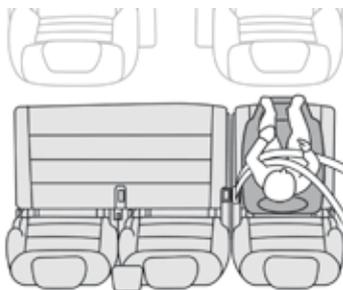
When a forward facing child seat is installed **on a rear passenger seat**, move the vehicle's front seat forward and straighten the backrest so that the legs of the child in the forward facing child seat do not touch the vehicle's front seat.
