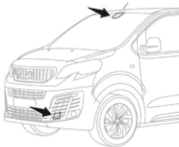
**i** If one of the two sensors (camera or radar) is masked or its visibility is reduced, while the other sensor is able to work normally, the system still operates, but at a lower level of performance. This is not indicated by a message or a warning lamp. To ensure correct operation of the radar radar, do not paint over the paintwork on the vehicle's bumper.
