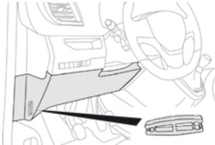
The extraction tweezers are located behind the fusebox cover, on the dashboard pillar.
