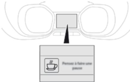
This alert takes the form of the display of a message encouraging you to take a break, accompanied by an audible signal. If the driver does not follow this advice, the alert is repeated hourly until the vehicle is stopped.
