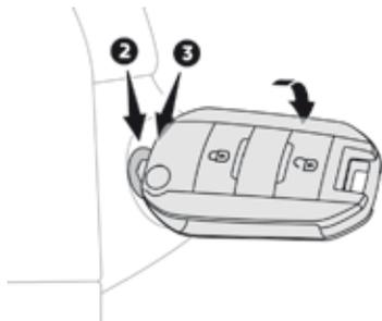
☞ Turn the key to position **2**, ignition on, to operate the engine pre-heating.
