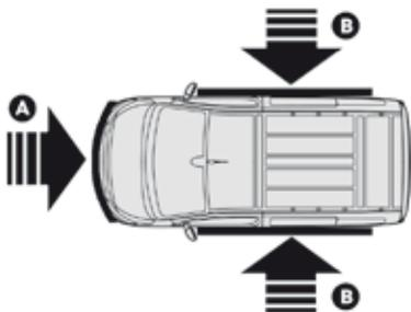
The curtain airbag is deployed in the event of a serious side impact applied to all or part of the side impact zone **B**, perpendicular to the longitudinal centreline of the vehicle on a horizontal plane and directed from the outside towards the inside of the vehicle.
