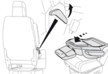
☞ Pull the control fully up and tip the backrest forward.
