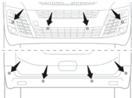
This system indicates the proximity of an obstacle (examples: pedestrian, vehicle, tree, gate) which comes within the field of detection of sensors located in the bumper. Certain types of obstacle (examples: stake, roadworks cone) detected initially will no longer be detected at the end of the manoeuvre, if they are located in blind spots in the sensors' field of detection.
