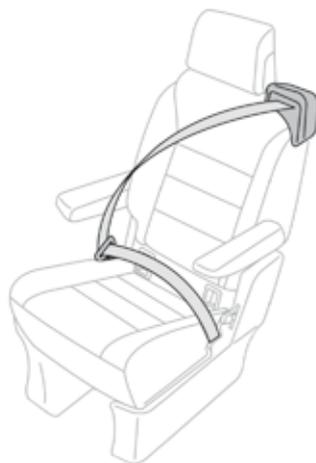
If your vehicle is fitted with individual seats, they have three-point seat belts with their guides and belt reels built into the backrests.
