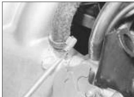
18.3 Disconnecting the brake servo vacuum hose
