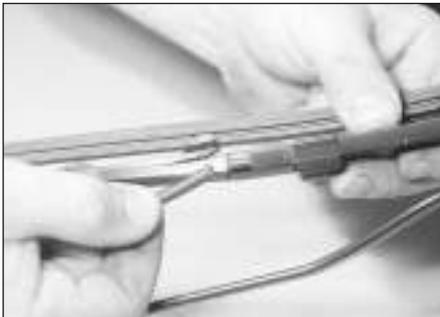
**1** Check the condition of the wiper blades; if they are cracked or show any signs of deterioration, or if the glass swept area is smeared, renew them. For maximum clarity of vision, wiper blades should be renewed annually, as a matter of course. To remove a front wiper blade, first prise off the securing clips, and disconnect the washer tube from the arm.
