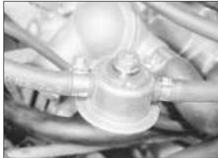
14.40 Fuel pump damper showing fuel hose connections
