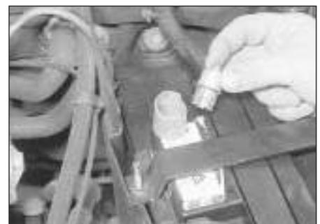
**4** Note that the battery negative terminal stud can be removed for cleaning or renewal. Unscrew the lead clamp, then pull off the plastic insulator, and lever off the stud and cover.
