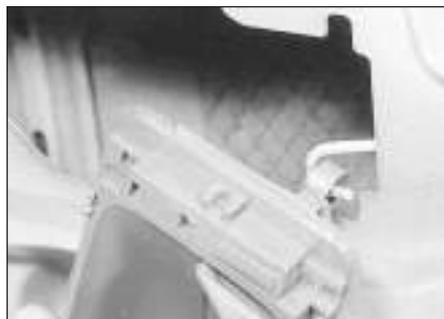
14.3 Unhooking the link rod from the interior door handle
