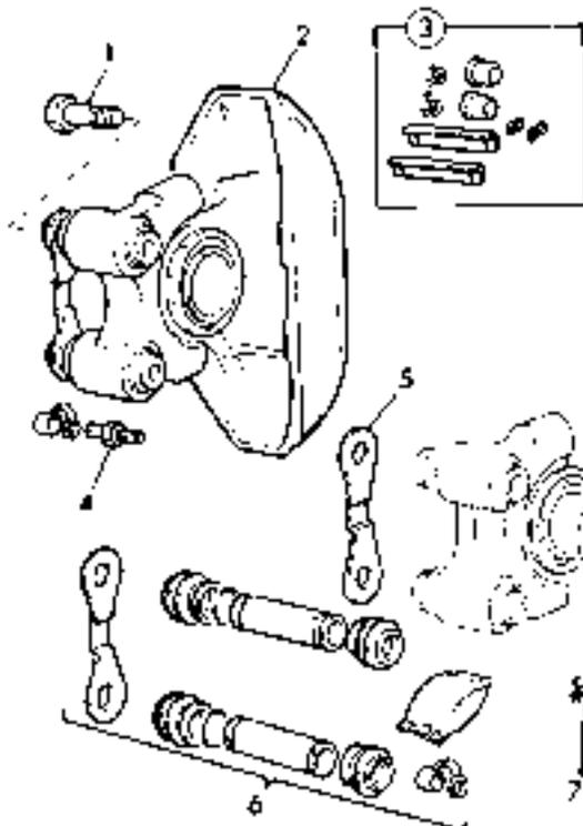
**10.6 Components of Bendix front caliper**
