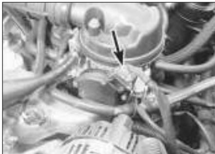
16.14 Throttle potentiometer wiring connector (arrowed)
