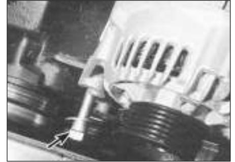
7.4b . . . and lower bolt (arrowed)
