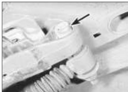
**13.3 Rear shock absorber upper mounting bolt (arrowed)**
