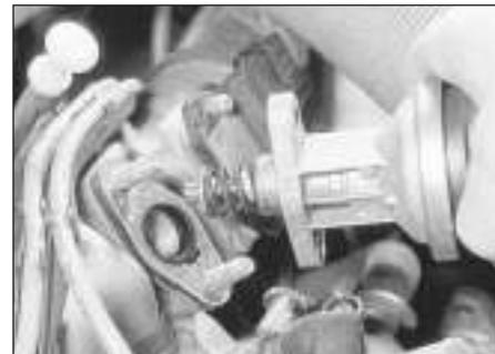
4.5 Removing the fuel pump (XU engine)
