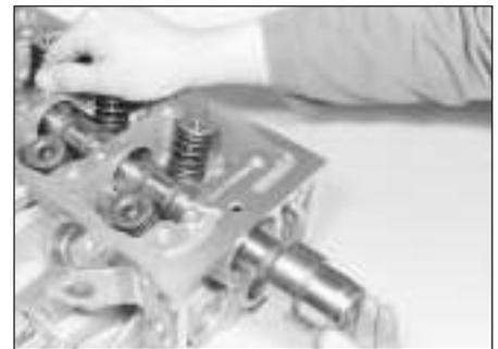
**10.9b** . . . and slide out the camshaft
