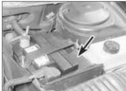
**1** The battery is located on the left-hand side of the engine compartment. The exterior of the battery should be inspected periodically for damage such as a cracked case or cover.
