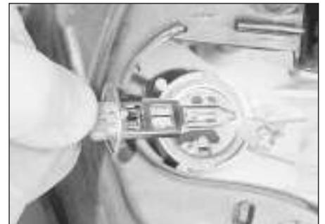
5.23b Removing a headlight-mounted driving light bulb
