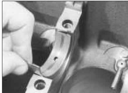
11.21 Remove the upper main bearing shells from the cylinder block/crankcase, and store them with their lower shells
