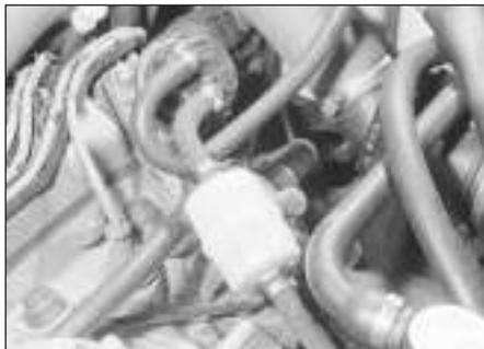
**8.1 Fuel filter location on carburettor models**
