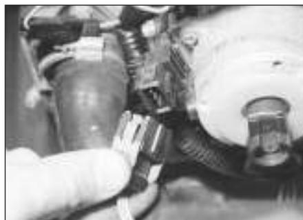
4.3a Disconnect the distributor wiring connector . . .
