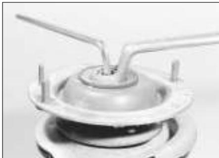
5.3 Counterhold the piston rod and unscrew the top mounting nut
