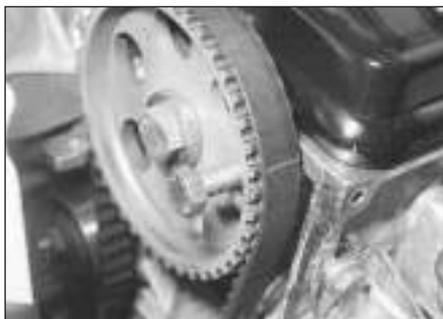
3.5 . . . then insert a 10 mm bolt through the cam sprocket timing hole, and locate it in the cylinder head
