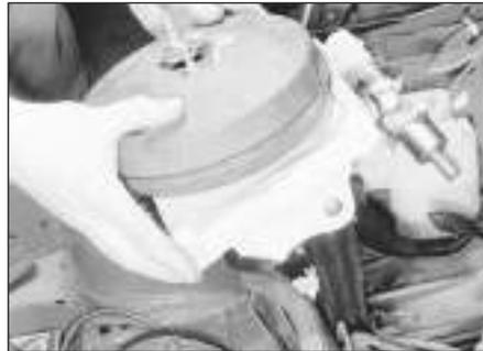
**15.15** Removing the vacuum servo/pedal bracket assembly
