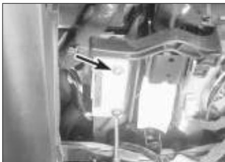
**3.14b** Unscrewing a relay bracket securing screw from under the steering column - models from 1993 (viewed with steering column shrouds removed)
