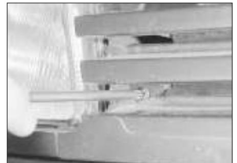
25.2 Remove the grille front securing screws . . .
