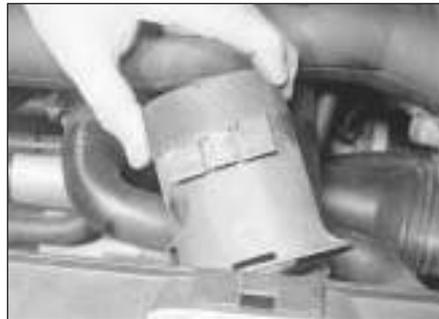
3.5b . . . and withdraw the air intake tube
