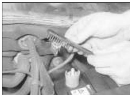
**3** If corrosion (white fluffy deposits) is evident, remove the cables from the battery terminals, clean them with a small wire brush, then refit them. Tools for cleaning the battery post and terminals are available.
