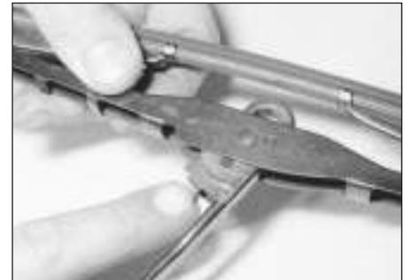
**3** On Estate models, to remove a tailgate wiper blade, pull the arm fully away from the glass until it locks. Swivel the blade through 90°, then press the locking tab, and slide the blade out of the arm's hooked end.
