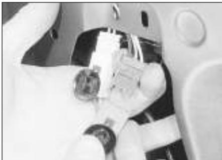
22.3 Disconnecting the door mirror wiring connectors
