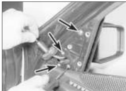
22.6a Remove the four securing screws . . .
