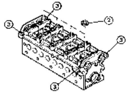
4.40a Spark plug hole oil seal (2). Apply silicon sealant to the areas arrowed (3) - XU9J4 engine
