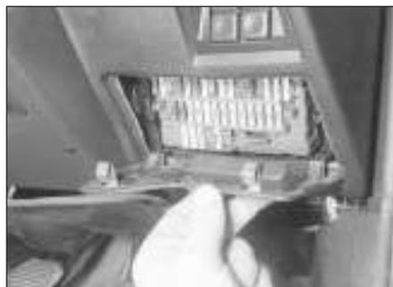
**2** If more than one indicator light or tail light has failed it is likely that either a fuse has blown or that there is a fault in the circuit (see Chapter 12). The fuses are located behind a panel on the bottom of the driver's side lower fascia panel.
