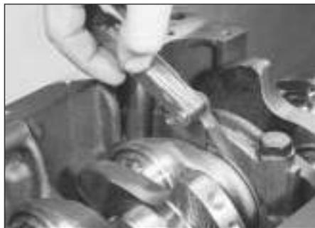
14.3 Checking crankshaft endfloat using feeler gauges
