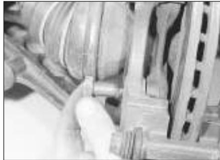
7.7 Removing a Girling caliper mounting bracket bolt
