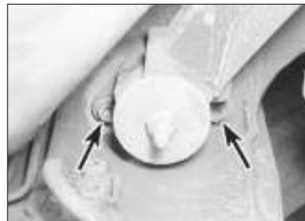
**14.16 Unscrew the two bolts (arrowed) on each side securing the suspension mountings to the body**
