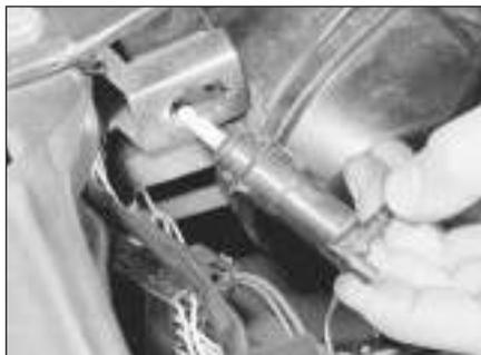
7.4 Removing a cable-operated headlight adjuster
