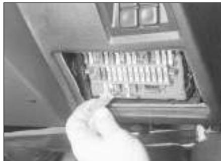
3.7 Removing a fuse using the plastic tool
