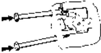
14.10b Using the improvised tools to release the lock cylinder securing clip
