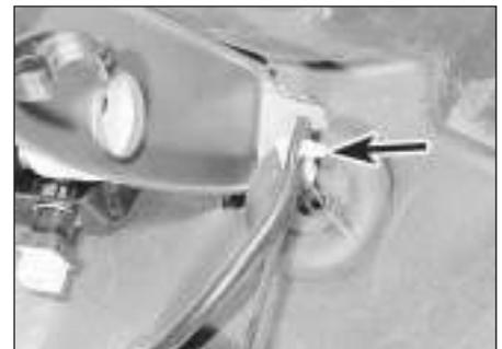
7.4 Accelerator cable connection to accelerator pedal (arrowed)
