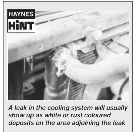
4 Inspect the cooling system (hoses, joint faces, etc.) for leaks (see Haynes Hint).
