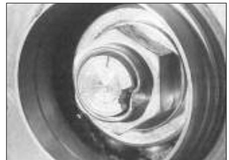
**11** Ensure that the bearing is packed with grease, then slide the hub assembly onto the stub axle. Fit the new outer bearing race, and tap it into position using a tubular drift until the hub nut can be fitted to finally draw the hub into position (see illustrations).
