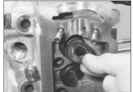
7.4c Remove the spring retainer . . .
