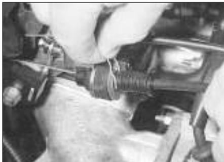
7.9 Adjusting the accelerator cable
