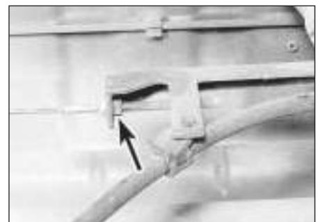
**17.7** Handbrake cable adjuster (arrowed)
