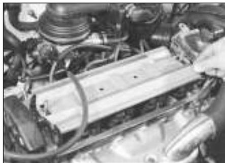
4.6b . . . and remove the oil baffle plate
