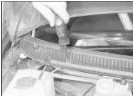
25.9 Unscrew the grille panel securing screws
