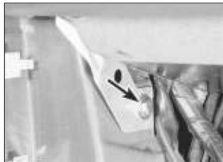
30.21 Lower facia mounting bracket-to-footwell bolt (arrowed)
