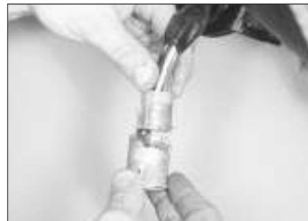
18.8c . . . and slide out the ignition switch
