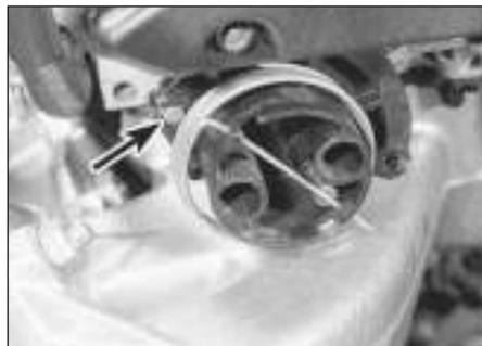
7.1a Accelerator cable connection on the throttle quadrant (arrowed)
