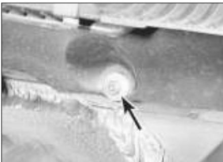
30.20 Facia securing nut (arrowed) in scuttle
