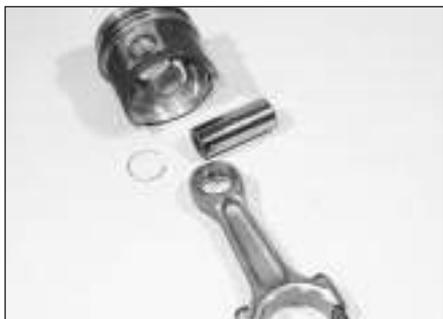
13.15c Piston and connecting rod components
