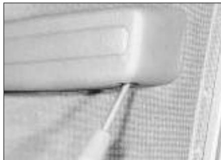
13.9 Remove the securing screws and withdraw the armrest
