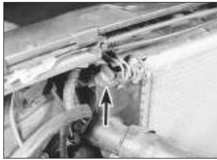
20.4c Radiator bleed screw (arrowed)
