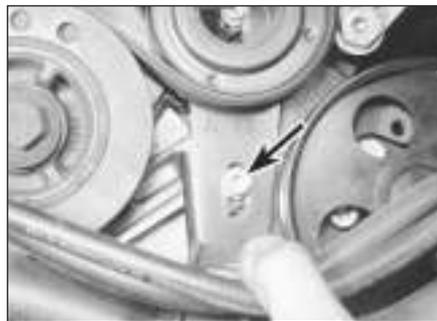
5.14 Tensioner pulley bracket lower mounting bolt (arrowed)
