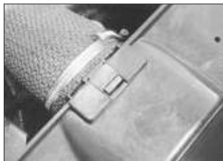
4.4 Inlet air duct connection to the front crossmember
