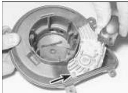
9.68a . . . then remove the securing screws . . .
