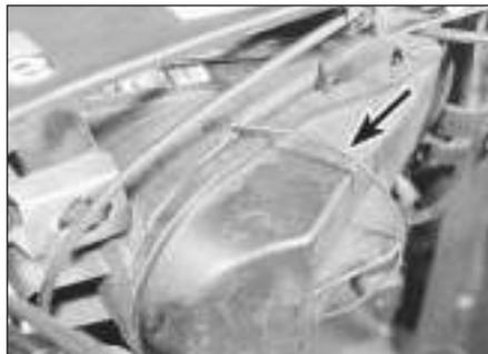
5.2 Headlight rear cover securing clip (arrowed)
