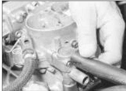
12.5 Disconnecting the float chamber breather pipe
