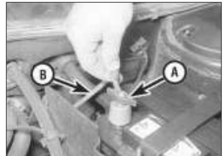
**2** Check the tightness of the battery cable clamps (A) to ensure good electrical connections. You should not be able to move them. Also check each cable (B) for cracks and frayed conductors.
