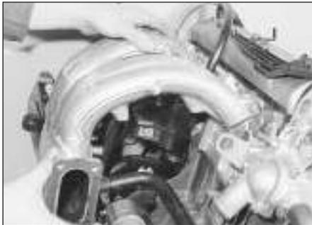
18.12c Fitting the inlet manifold
