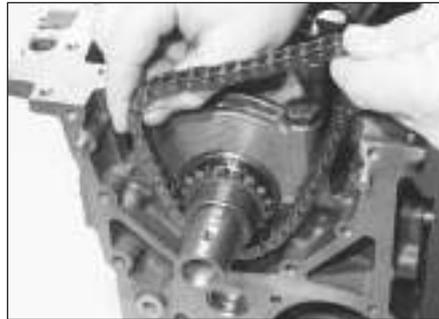
11.16a Remove the oil pump drive chain . . .
