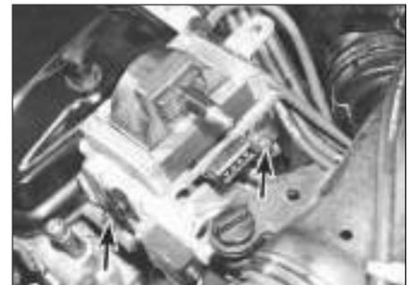
3.5a Undo the two retaining bolts (arrowed) . . .
