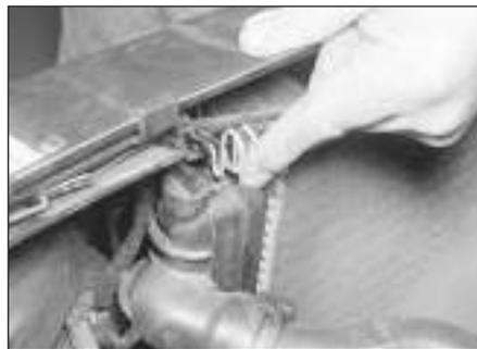
3.10 Releasing a radiator upper securing clip
