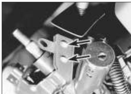
**4.3** Steering column combination switch screws (arrowed) - models up to 1992
