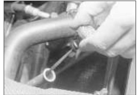
4.2a Withdrawing the automatic transmission dipstick
