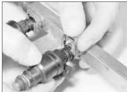
14.29 Removing an injector from the fuel rail
