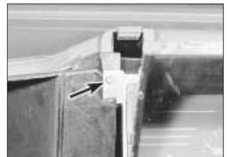
9.8 Instrument panel securing screw (arrowed)
