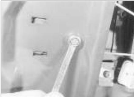
20.8 Unscrewing the tailgate lock motor securing bolt
