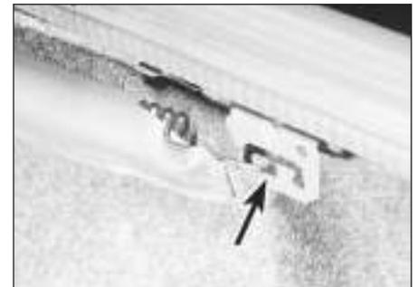
16.2 Note which slots (arrowed) the ends of the boot lid assister springs are positioned in before disconnecting them
