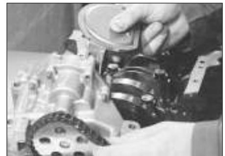
**14.3** Removing the oil pump
