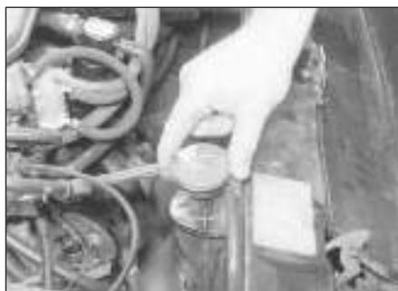
2 If topping up is necessary, **wait until the engine is cold**. Unscrew the expansion tank cap to the first stop, to release any pressure present in the system. Push the cap down, turn to the second stop, and remove it.
