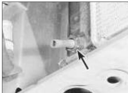
20.3 Radiator drain outlet (arrowed)
