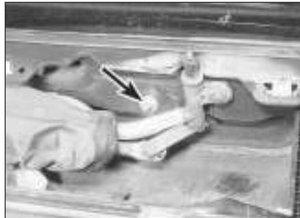
**30.70** Fascia securing nut (arrowed) in scuttle
