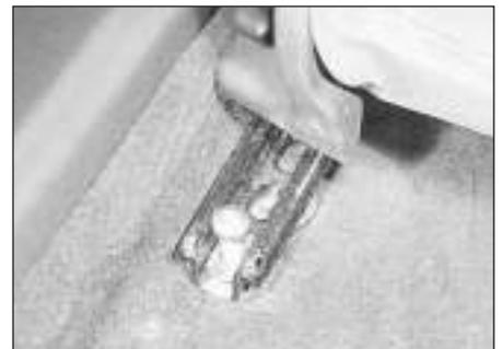
26.3 Front seat rear securing bolt partially removed
