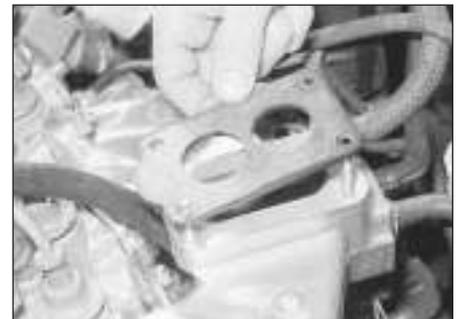
12.11 Removing the insulating spacer
