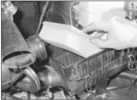
21.9 Removing the air filter element
