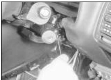
18.5 Unscrewing the lock securing screw
