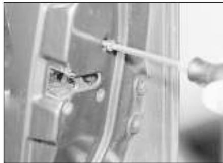
14.16 Remove the door lock securing screws
