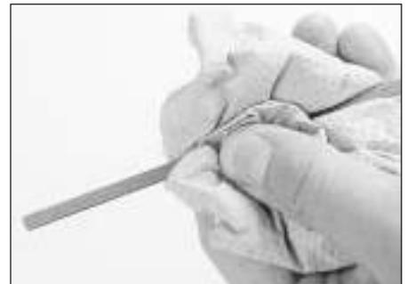
2 Using a clean rag or paper towel remove all oil from the dipstick. Insert the clean dipstick into the tube as far as it will go, then withdraw it again.
