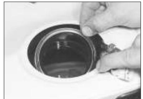
9.12b . . . and recover the rubber sealing ring
