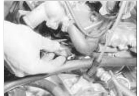
14.45 Disconnecting the supplementary air device plug
