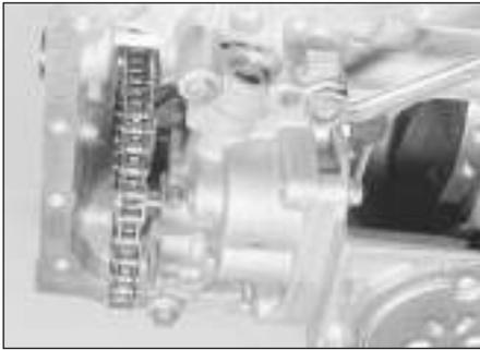
13.2 Oil pump is retained by three bolts
