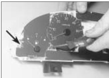
10.10 Remove the gauge securing screws . . .
