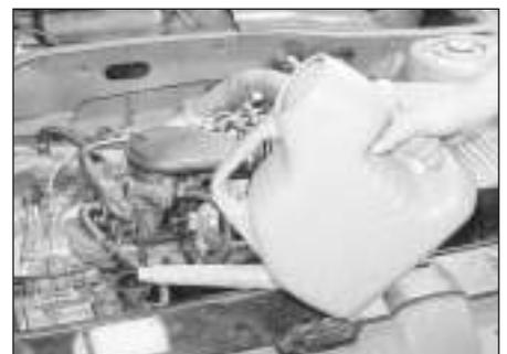
3 Add a mixture of water and antifreeze through the expansion tank filler neck, until the coolant level is up to the “MAXI” level mark. Refit the cap, turning it clockwise as far as it will go to secure.
