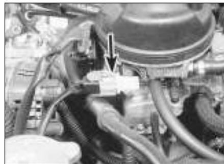
**16.3** Injector wiring connector (arrowed)
