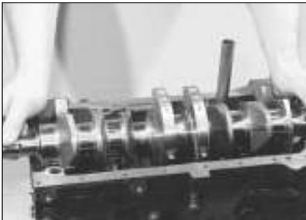
11.20 Lifting out the crankshaft - XU series engine
