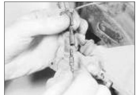
4.2 Disconnecting the pad wear sensor wiring connector
