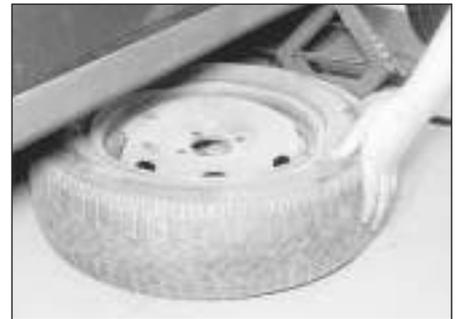
**6** Temporarily place the spare wheel under the sill as a precaution should the jack topple.
