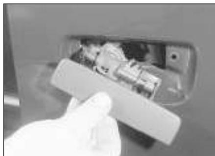
14.8 Withdrawing the exterior door handle
