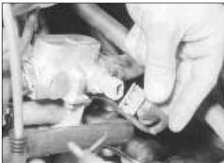
14.48 Disconnecting the injection thermistor wiring
