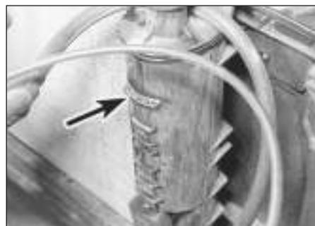
1 The coolant level varies with engine temperature. When cold, the coolant level should be on the “MAXI” mark (arrowed). When the engine is hot, the level may rise slightly above the “MAXI” mark.
