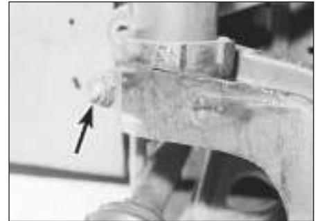
2.12 Hub carrier-to-suspension strut clamp nut (arrowed)
