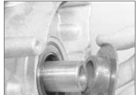
7.12 Remove the flanged spacer if necessary
