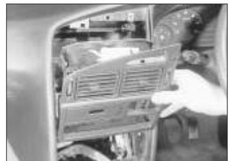
30.40 Withdrawing the ventilation nozzle housing
