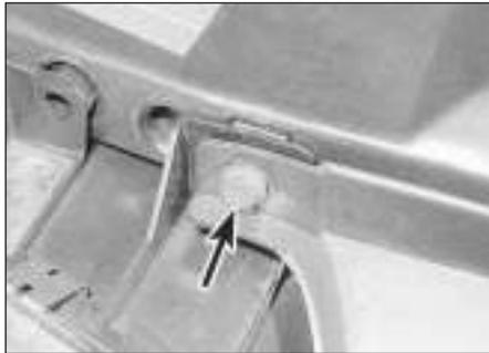
25.3 . . . and the upper securing bolts (arrowed)
