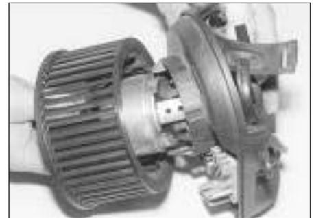
9.66 . . . then withdraw motor from casing
