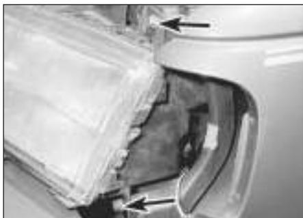
7.8 Outer headlight securing bolts (arrowed)
