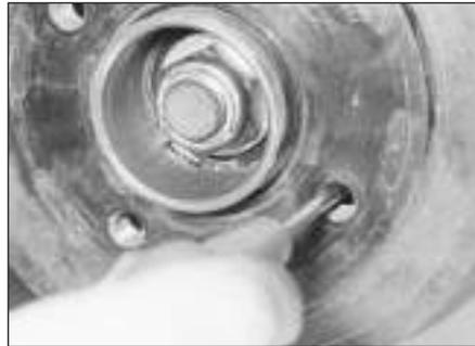
9.3b Releasing the handbrake operating lever
