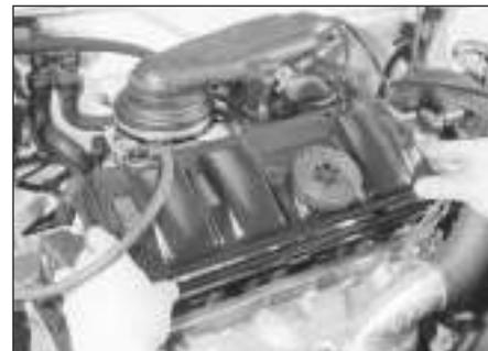
4.5 . . . and lift off the cylinder head cover
