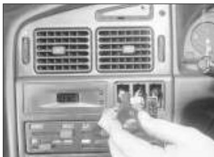
30.39b . . . then remove the remaining housing securing screw
