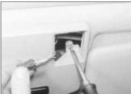
20.31 Removing a roof console securing screw
