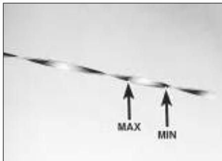
3 Note the oil level on the end of the dipstick, which should be between the upper (“MAX”) mark and lower (“MIN”) mark. Approximately 1.0 litre of oil will raise the level from the lower mark to the upper mark.
