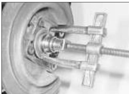
10.6b Removing the inner bearing race . . .
