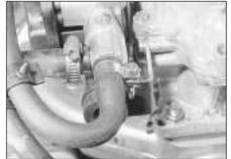
12.6a Automatic choke coolant pipe connection . . .
