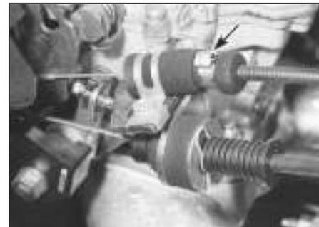
9.10 Choke cable-to-rubber collar retaining clip (arrowed)
