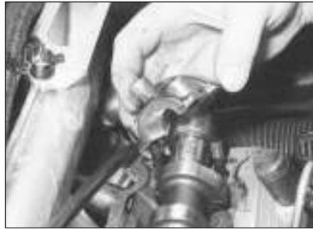
10.32 . . . and remove the camshaft bearing caps . . .
