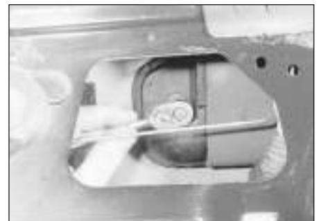
14.7b Unscrew the securing nut . . .
