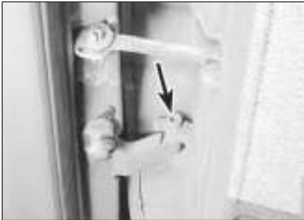
12.6 Door pivot pin (arrowed)
