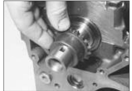
11.16b . . . then slide off the drive sprocket . . .
