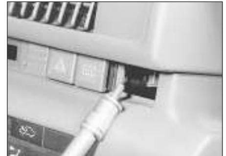
9.3a . . . and remove the visor securing screws
