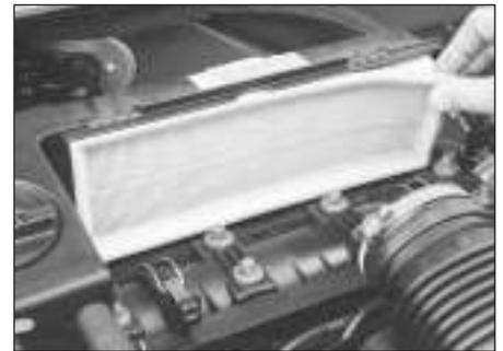
21.14d . . . and withdraw the filter element
