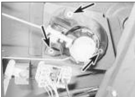
19.4 Tailgate lock cylinder securing rivets (arrowed)
