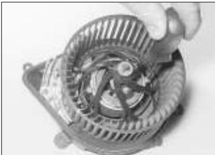
9.65a Remove the securing screws . . .
