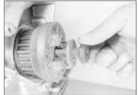
7.11a Remove the crankshaft sprocket retaining bolt . . .
