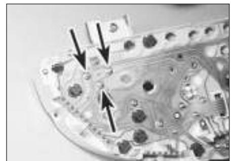
10.9 Fuel gauge securing nuts (arrowed)
