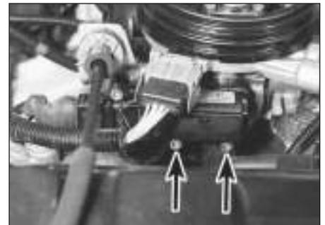
15.11 Idle control stepper motor retaining screws (arrowed)
