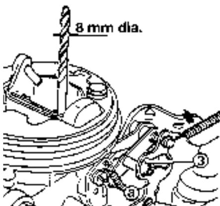
13.34 Checking the choke mechanical opening (Weber carburettor)
