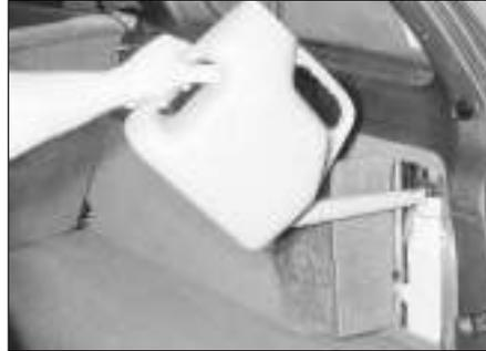
**2** On Estate models, the tailgate washer fluid reservoir is located behind a hinged cover on the right-hand side of the luggage compartment.
