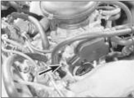
**10.7 Idle mixture adjustment screw (arrowed)**
