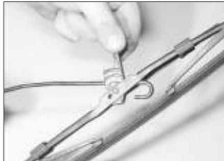
**2** Pull the arm fully away from the glass until it locks. Swivel the blade through 90°, then pull up the blade securing clip, and slide the blade out of the arm's hooked end.
