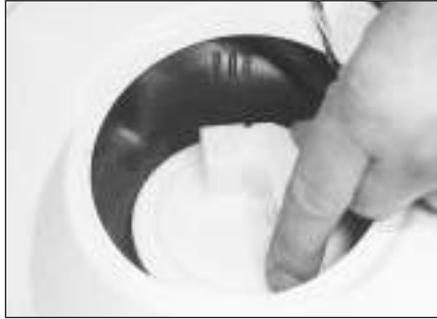
10.1 Removing the fuel gauge sender unit
