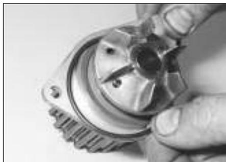
7.6b . . . and recover the O-ring - 1.4 litre engine shown
