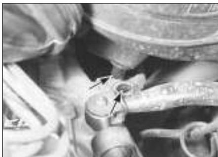
2.10 Air cleaner housing peg and mounting rubber (arrowed)
