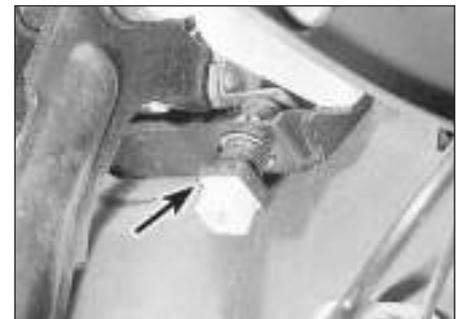
**22.1 Stop-light switch (arrowed) on brake pedal bracket**
