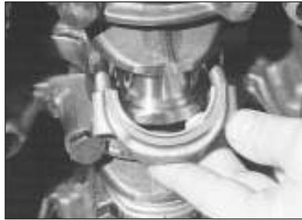
10.5 Removing a big-end bearing cap and shell
