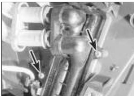
9.36a Remove the two securing screws . . .
