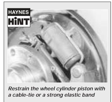
Restrain the wheel cylinder piston with a cable-tie or a strong elastic band
