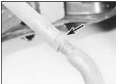
22.3 Track rod end locknut (arrowed)
