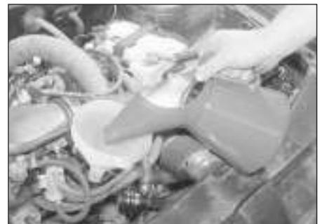
4 Oil is added through the filler cap. Unscrew the cap and top-up the level; a funnel may help to reduce spillage. Add the oil slowly, checking the level on the dipstick often. Don't overfill (see “Car Care” left).
