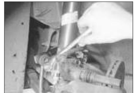
4.5 Unscrewing the hub carrier-to-suspension strut clamp bolt
