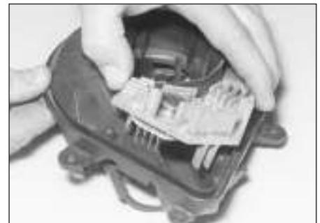
9.68b . . . and withdraw the control module
