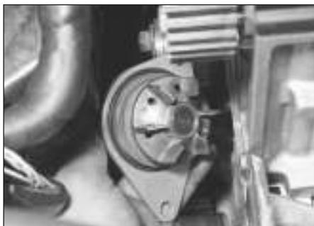
7.6a Withdraw the coolant pump . . .
