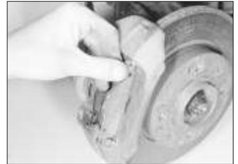
4.6 Withdrawing the outer brake pad - Bendix caliper
