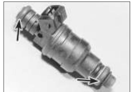
14.30 Injector O-ring seals (arrowed)
