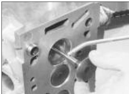
**9.1 Lubricate the valve stems prior to refitting**
