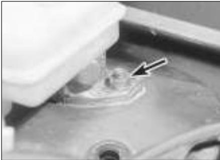
13.5 Master cylinder securing nut (arrowed)
