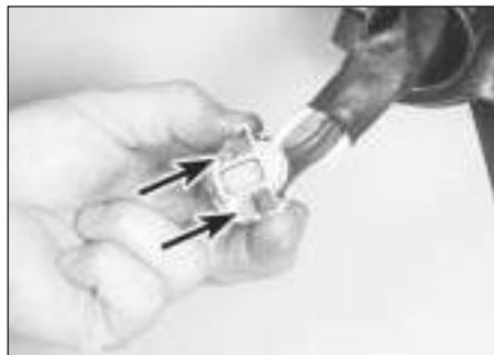
18.8a Remove the two lock securing screws . . .
