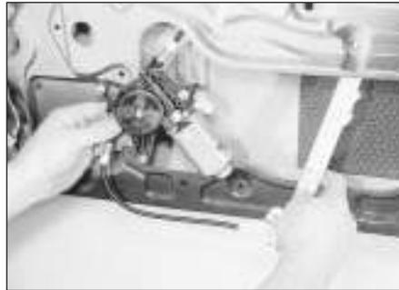
15.16 Removing the front door window regulator assembly
