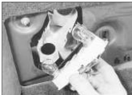
5.36b Removing a tailgate-mounted light bulbholder - Estate model
