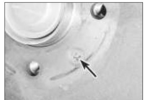
9.2 Rear brake drum retaining screw (arrowed)
