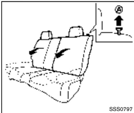
To fold down the seatback of each rear seat, pull the adjusting knob (A) .
