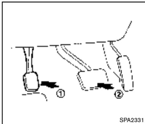
**To apply:** Fully depress the parking brake pedal ①.
