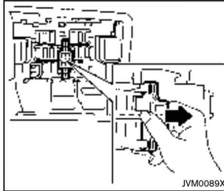
4. If the fuse is open (A) , replace it with a new fuse (B) .
