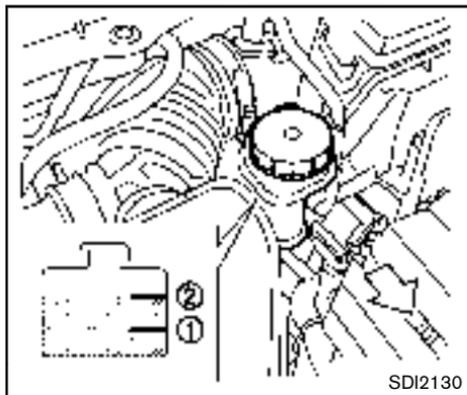
Check the fluid level in the reservoir. If the fluid is below the MIN line ① or the brake warning light comes on, add Genuine NISSAN Super Heavy Duty Brake Fluid or equivalent **DOT 3** fluid up to the MAX line ②. If fluid must be added frequently, the system should be checked by a NISSAN dealer.
