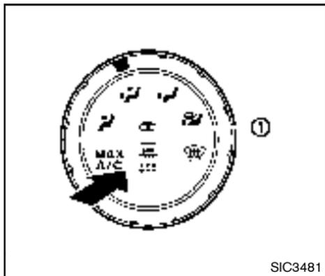
To defog/defrost the rear window glass and outside mirrors (if so equipped), start the engine and push the switch on. The indicator light ① will illuminate. Push the switch again to turn the defroster off.
