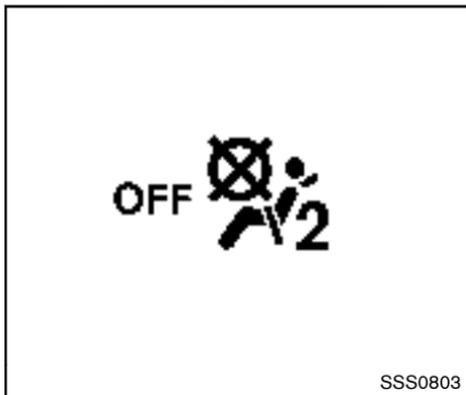
7. If the booster seat is installed in the front passenger seat, turn the ignition switch to the ON position. The front passenger air bag status light
