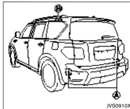
The BSI system uses radar sensors (A) installed near the rear bumper to detect other vehicles in an adjacent lane. In addition to the radar sensors, the BSI system uses a camera (B) installed behind the windshield to monitor the lane markers of your traveling lane.
