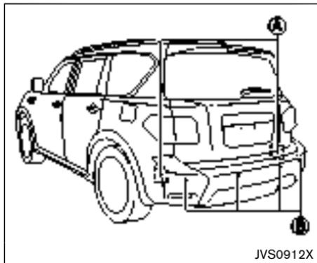
The BCI system uses radar sensors (A) installed on both sides near the rear bumper to detect an approaching vehicle and sonar sensors (B) to detect objects in the rear.
