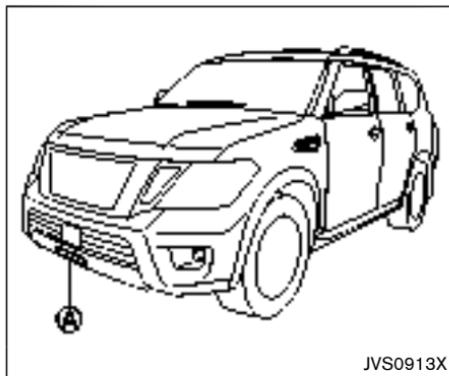
The FEB system uses a sensor (A) located below the front bumper to measure the distance to the vehicle ahead in the traveling lane.
