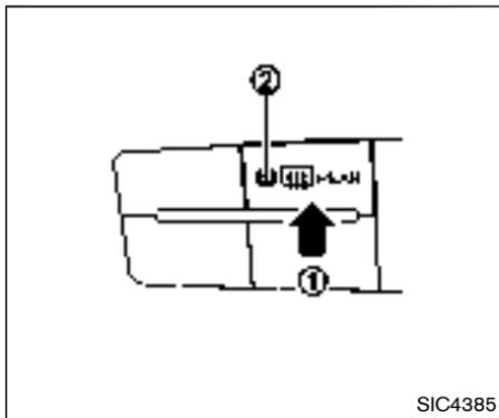
The windshield deicer switch (defroster switch) operates when the ignition switch is in the ON position.
