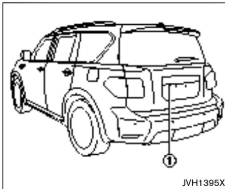
To display the rear view, the RearView Monitor system uses a camera (1) located just above the vehicle's license plate.
