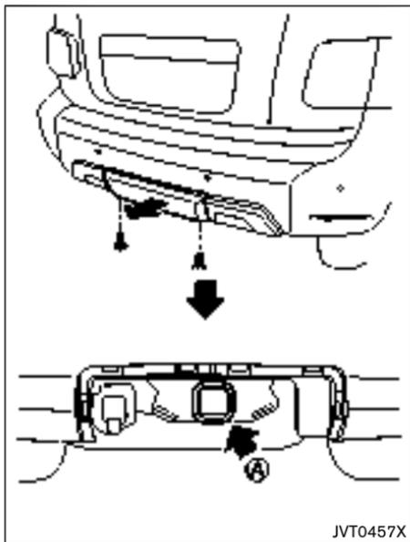
To access the trailer hitch (A), remove the trailer hitch cover located on the lower part of the rear bumper.
