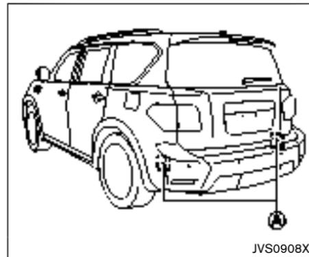
The BSW system uses radar sensors **A** installed near the rear bumper to detect other vehicles in an adjacent lane.
