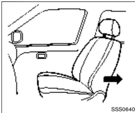
1. **If you must install a booster seat in the front seat, move the seat to the rear-most position.**
