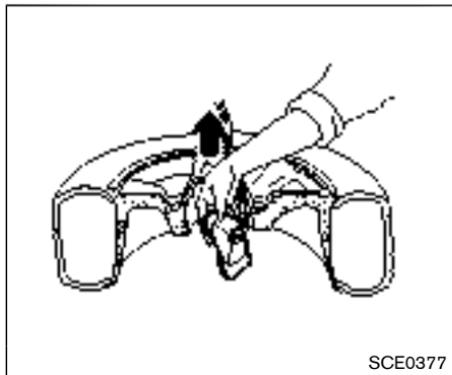
10. Once the spare wheel is completely lowered, remove the jack rod and reach under the vehicle to remove the hanging plate.
