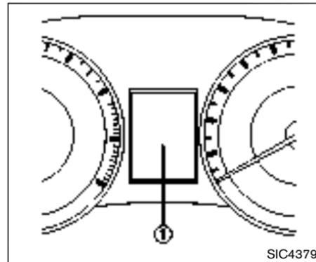
The vehicle information display
