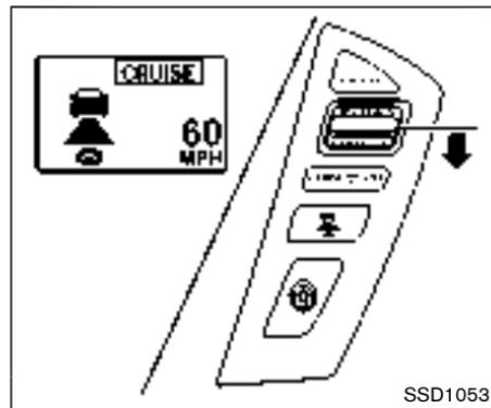
**To set cruising speed**, accelerate your vehicle to the desired speed, push the COAST/SET switch and release it. (Vehicle ahead detection indicator, set distance indicator and set vehicle speed indicator come on.) Take your foot off the accelerator pedal. Your vehicle will maintain the set speed.
