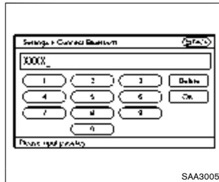
4. When a passkey appears on the screen, operate the compatible Bluetooth® audio device to enter the passkey. The pairing procedure of the audio device varies according to each audio device. See the Bluetooth® audio Owner’s Manual for details.
