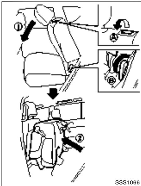
To enter the 3rd row seat, pull the lever (A) or (B) located on the 2nd row seat and fold the seatback forward (1) at an angle over the seat base. Then lift up the seat base and tip the 2nd row seat forward (2). This will release the back of the seat so it may be tipped forward.
