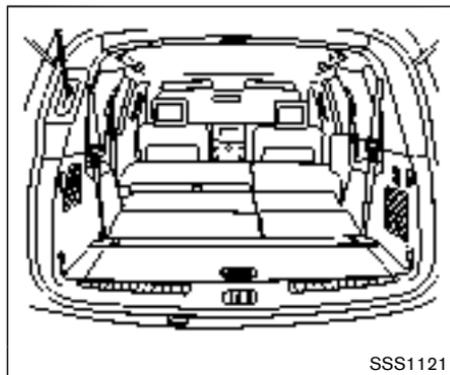
3. Power operation (if so equipped): Fold the 3rd row seat flat using the switches located in the cargo area. See "Power seat adjustment" (P.1-8).
