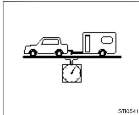
The GCWR equals the combined weight of the towing vehicle (including passengers and cargo) plus the total trailer load. Towing loads greater than these or using improper towing equipment could adversely affect vehicle handling, braking and performance.
