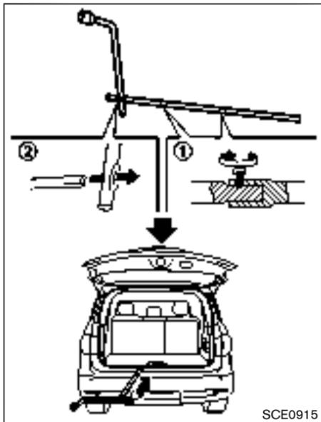
5. Securely screw to connect the T-shaped end of the jack rod and two extension bars ① as illustrated.
