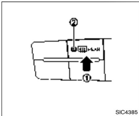
To defog/defrost the rear window glass and outside mirrors (if so equipped), start the engine and push the switch ① on. The indicator light ② will come on. Push the switch again to turn the defroster off.
