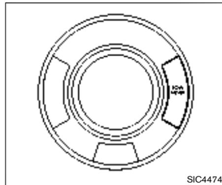
TOW MODE should be used when pulling a heavy trailer or hauling a heavy load. Driving the vehicle in TOW MODE with no trailer/load or light trailer/light load will not cause any damage. However, fuel economy may be reduced, and the transmission/engine driving characteristics may feel unusual.
