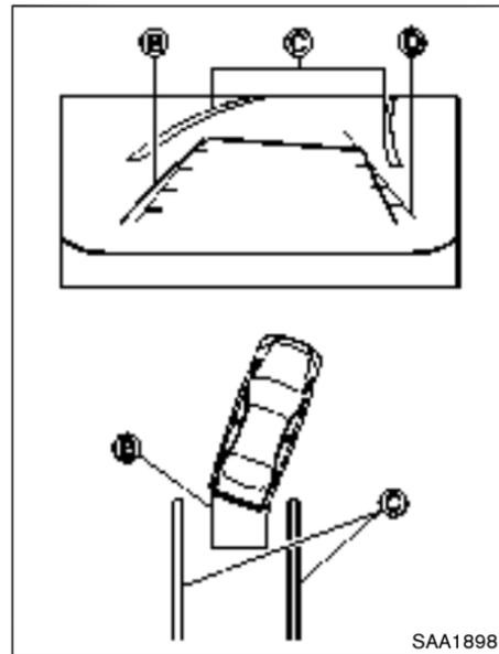
3. Slowly back up the vehicle adjusting the steering wheel so that the predictive course lines (B) enter the parking space (C) .
