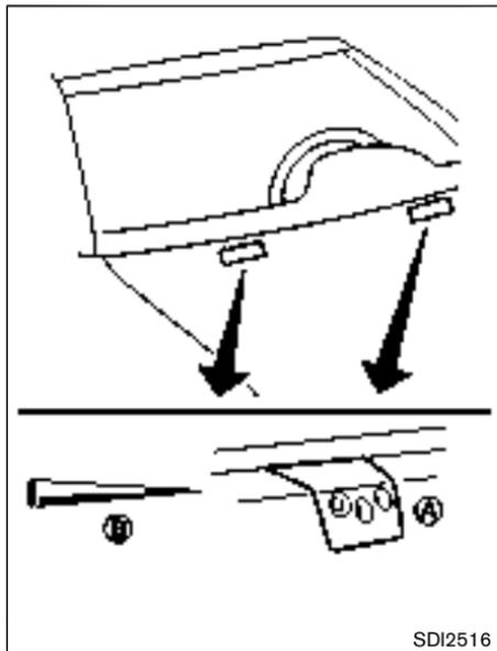
Be careful not to clog the washer nozzle (A) . This may cause improper windshield washer operation. If the nozzle is clogged, remove any objects with a needle or small pin (B) . Be careful not to damage the nozzle.
