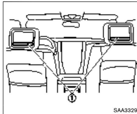
The rear displays are located on the back of the front head restraints.
