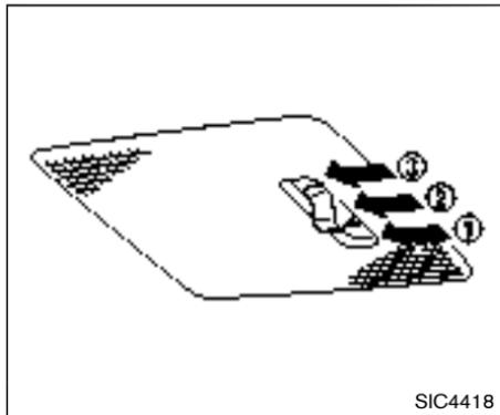
The cargo light switch has three positions: ON ①, center ② and OFF ③.
