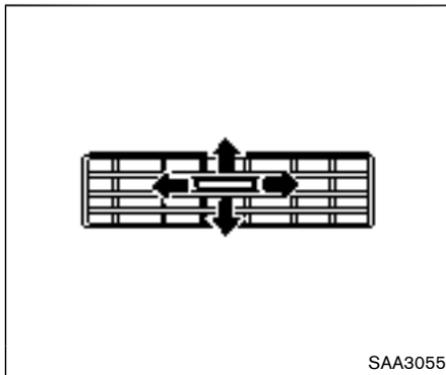
Adjust the air flow direction of the ventilators by moving the center knob (up/down, left/right) until the desired position is achieved.
