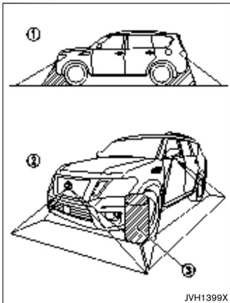
There are some areas where the system will not show objects and the system does not warn of moving objects. When in the front or the rear view display, an object below the bumper or on the ground may not be viewed ①. When in the bird's-eye view, a tall object near the seam ③ of the camera viewing areas will not appear in
