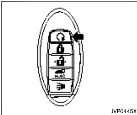
The remote engine start
