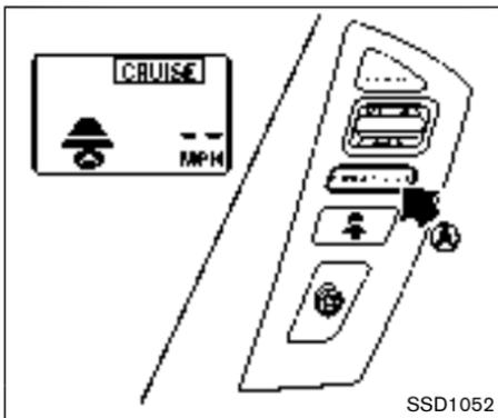
Operating vehicle-to-vehicle distance control mode
