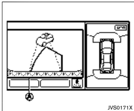
If an approaching vehicle or object behind the vehicle is detected when your vehicle is backing up, a red frame (A) will appear on the display and the system will chime three times. Then, the brakes will be applied momentarily. After the automatic brake application, the driver must depress the brake pedal to maintain brake pressure.
