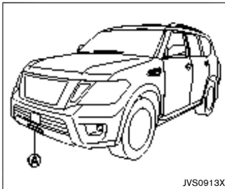
The system is intended to assist the driver to keep a following distance from the vehicle ahead traveling in the same lane and direction.
