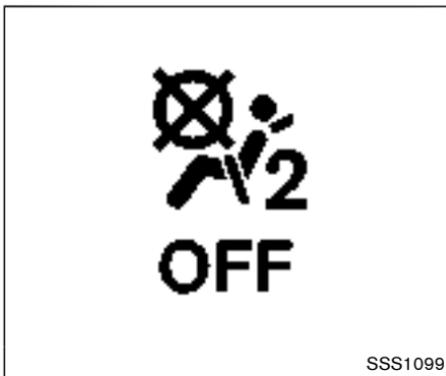
7. If the booster seat is installed in the front passenger seat, place the ignition switch in the ON position. The front passenger air bag status light
