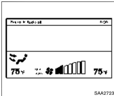
When the STATUS button is pushed, the heater and air conditioner status screen will appear. (See "How to use STATUS button" (P.4-8).)
