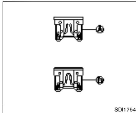
4. If the fuse is open, replace it with a new fuse.
