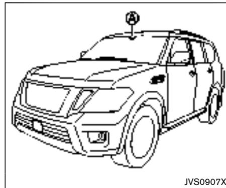
The LDW and LDP systems use a camera
