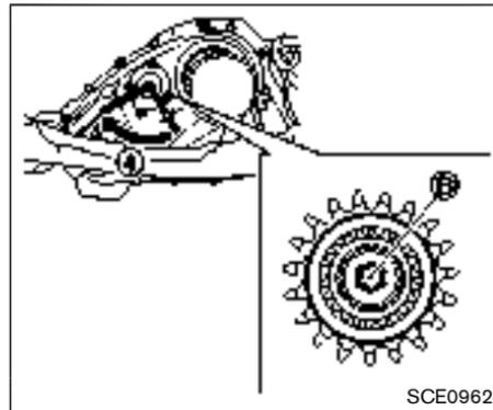
6. Completely insert the wrench into the internal gear (B) of the transfer.
