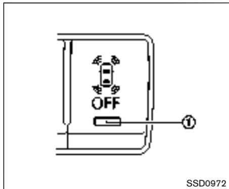
The sonar system OFF switch on the lower side of the instrument panel allows the driver to turn the sonar system on and off. To turn the sonar system on and off, the ignition switch must be in the ON position. The indicator light ① on the switch will illuminate when the system is turned off. If the indicator light flashes when the sonar system is not turned off, it may indicate a malfunction in the sonar system.
