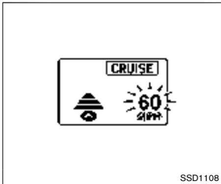
**When passing another vehicle,** the set speed indicator will flash when the vehicle speed exceeds the set speed. The vehicle detect indicator will turn off when the area ahead of the vehicle is open. When the pedal is released, the vehicle will return to the previously set speed.
