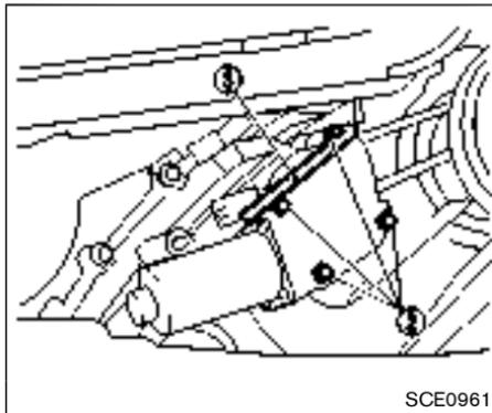
4. Remove the 4 bolts (2) that secure the 4WD shift motor using the wrench (3) that is equipped in the vehicle.
