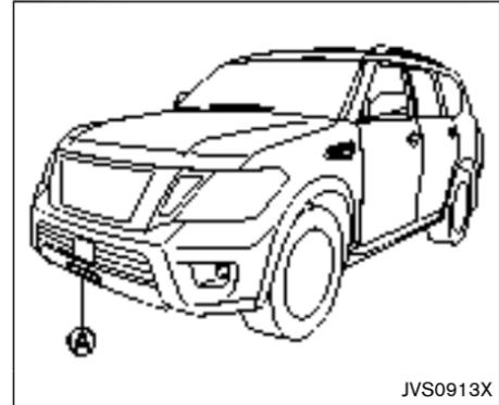
The PFCW system uses a radar sensor (A) located below the front bumper to measure the distance to a second vehicle ahead in the same lane.
