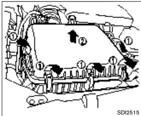
To remove the filter, release the lock pins ① and pull the unit upward ②.
