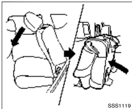
1. Push and hold the corresponding switch located on the instrument panel below the audio system. The seatback will fold down and tip forward. See "Entry to 3rd row seat" (P.1-5).
