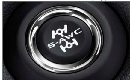
The drive mode can be switched by pressing the drive mode button while the ignition switch is in the ON position.
