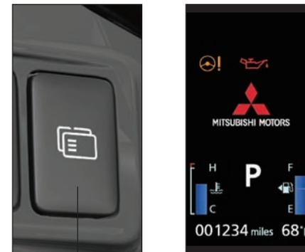
Each time the multi information display switch is operated, the buzzer sounds and the multi information display changes between information such as warnings, trip odometer, average and momentary fuel consumption, distance range, etc.
