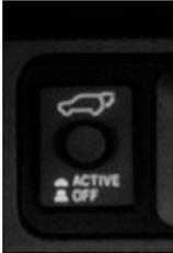
When the power liftgate main switch is ACTIVE, the power liftgate can be operated using either the power liftgate switch on the F.A.S.T.-key, the driver’s side power liftgate switch or the open/close switches on the power liftgate.
