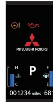
Each time the multi information display switch is operated, the buzzer sounds and the multi information display changes between information such as warnings, trip odometer, average and momentary fuel consumption, distance range, etc.
