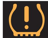
The Tire Pressure Monitoring System light illuminates when one or more of your tires is significantly under inflated. Please note that changes in the outside temperature may decrease tire pressure causing the TPMS light to turn on. If the TPMS light remains illuminated, check your tire pressure.
