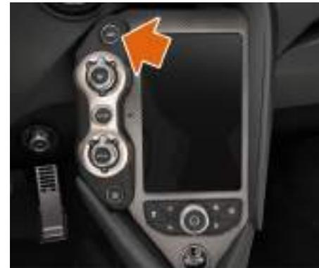
2. Press the AERO button and the Airbrake deploys.
