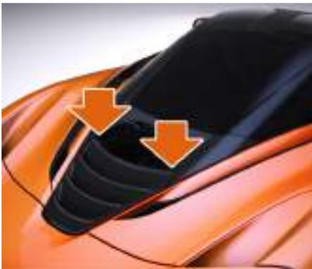
2. Apply pressure to the service cover as shown. Positive clicks will be heard when the two fixings engage.
