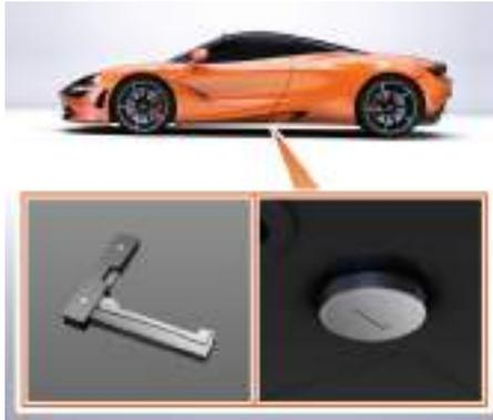
3. Insert the mechanical key into the lock and, turn the key counter-clockwise until mechanical resistance is preventing full release of the door.
