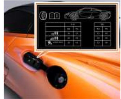
**i** NOTE: In some markets, the tire pressure label is attached to the base of the driver's side door aperture.
