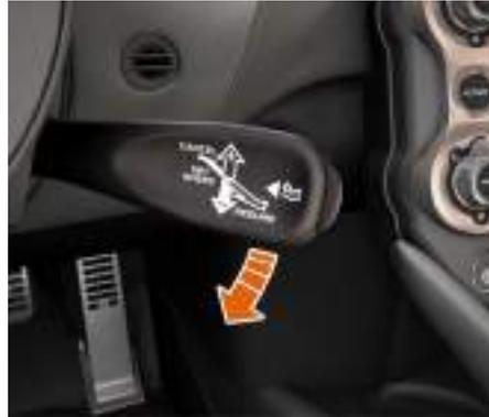
1. Accelerate or decelerate to the maximum permitted speed and push the stalk down briefly, to activate Active Speed Limiter (ASL).
