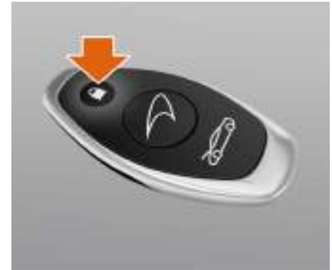
If either the doors or the luggage compartment lid are left open, or the key fob is still inside the vehicle, the horn will sound indicating mislock when an attempt to lock the vehicle is made.
