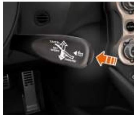
Access to nose lift is obtained by pressing the button on the control stalk on the right of the steering column, whenever the engine is running and the doors are closed.
