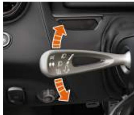
**i** NOTE: The parking lights can only be activated when the ignition is switched off.
