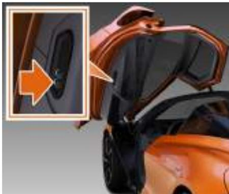
1. To disable the interior motion sensor, switch off the ignition, open the driver's door and press the button on the rear edge of the driver's door. The light in the switch will illuminate to indicate that the interior motion sensor has been disabled.
