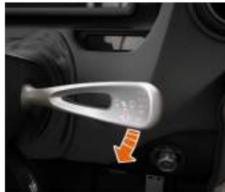
1. For a slow single wipe, briefly push the wiper stalk down and release. The wipers will operate once at slow speed, without washers.
