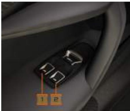
Push switches (1) and (2) downwards until the windows are open and hold them in this position for 5 seconds.
