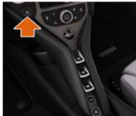
Press the Eco Start-Stop system OFF button to deactivate the system. The light in the button will illuminate and the status light on the Driver Display will be extinguished.
