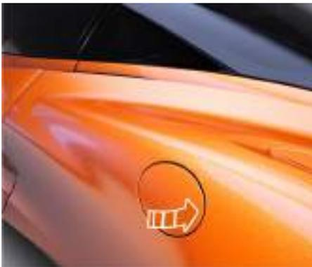
2. Press the rear edge of the fuel filler flap, the latch will release.
