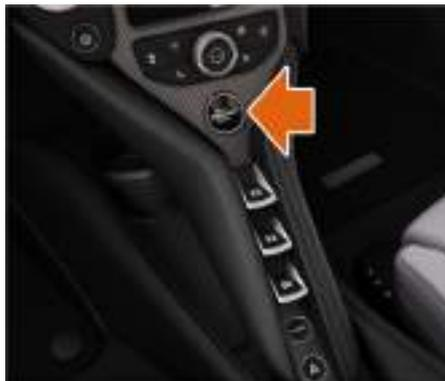
3. Press the START/STOP button. The engine stops, the vehicle enters Awake mode, see Vehicle electrical status, page 2.2. The immobilizer is activated.
