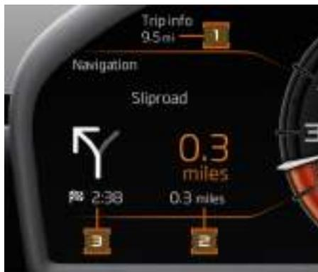
The current navigation turn-by-turn guidance will be displayed on the Driver Display if route guidance has been started using the Central Display.
