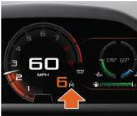
The gearbox mode indicator displays M and the currently selected gear. All forward gear changes are made by operating the gearshift paddles, see Gearshift paddles, page 2.20.
