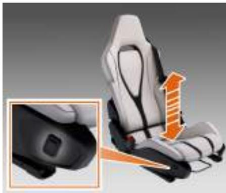
Press the switch up or down until the seat reaches the desired height.
