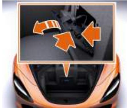
3. Open the top of the battery access cover and disconnect the 2 electrical connectors on the back of the cover.
