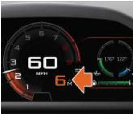
When in manual mode and driving more economically, the gear shift indicator (GSI) will illuminate when an upshift would maintain optimum economy. The GSI will not illuminate if the requested acceleration or deceleration cannot be met with a higher gear. See Economical driving, page 2.11.
