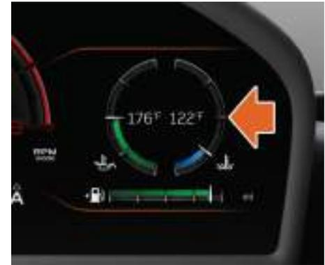
The water temperature is displayed in the form of a colored gauge on the right-hand side of the Driver Display.
