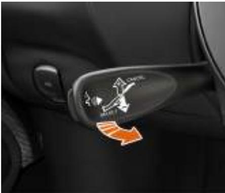
6. When the function required is selected or a setting is made, pull the stalk towards you (**FORWARD**) to confirm.
