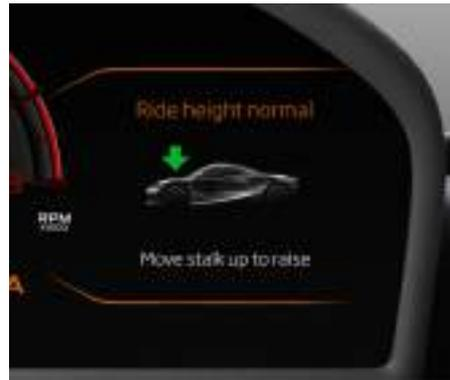
**Ⓛ** The change in nose ride height is confirmed by an ascending audible tone. 'Vehicle raising' appears on the Driver Display and the nose lift icon will flash.
