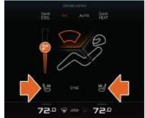
Touch the button once to switch seat heating on to the low temperature setting, one bar on the button will illuminate. Touch the button again to switch to the medium temperature setting, two bars on the button will illuminate. Touch the button again to switch to the full temperature setting, three bars on the button will illuminate.
