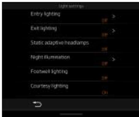
Entry and exit lighting illuminates the exterior lights when the vehicle is unlocked and locked. To activate these features, set the duration of each to **15 seconds, 30 seconds, 45 seconds** or **60 seconds**. To deactivate, select **Off**.
