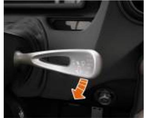
1. For a slow single wipe, briefly push the wiper stalk down and release. The wipers will operate once at slow speed, without washers.
