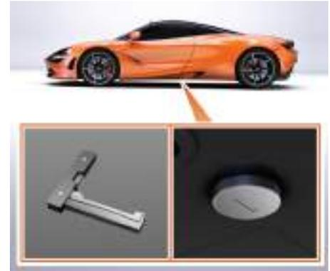
3. Insert the mechanical key into the lock and, turn the key counter-clockwise until mechanical resistance is preventing full release of the door.
