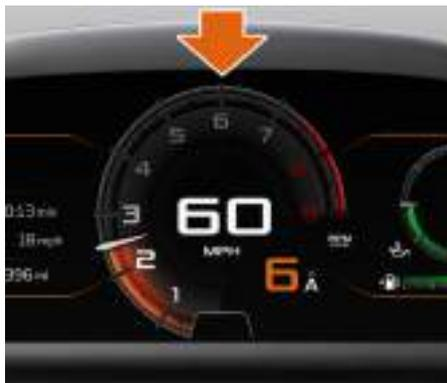
The tachometer display appears in the center of the Driver Display when in Non-Active or Comfort powertrain and handling modes. The red number on the display indicates the engine's maximum RPM.
