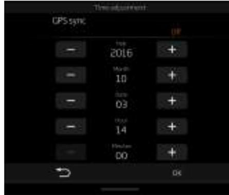
Select GPS sync to automatically adjust the time using the GPS signal. On will be highlighted when GPS sync is activated.
