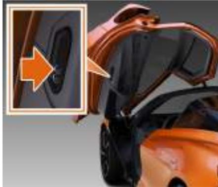
1. To disable tow-away protection, switch off the ignition, open the driver's door and press the button on the rear edge of the driver's door. The light in the switch will illuminate to indicate that tow-away protection has been disabled.
