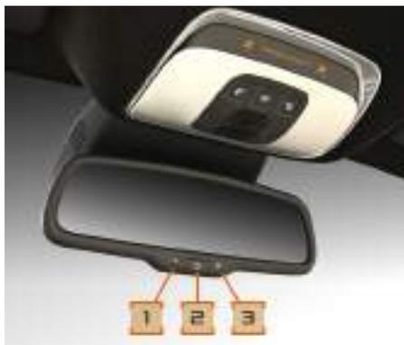
The automatic dimming function of the interior mirror is activated or deactivated by pressing the switch (2) on the bottom of the mirror. The indicator light (1) will illuminate when automatic dimming is active.
