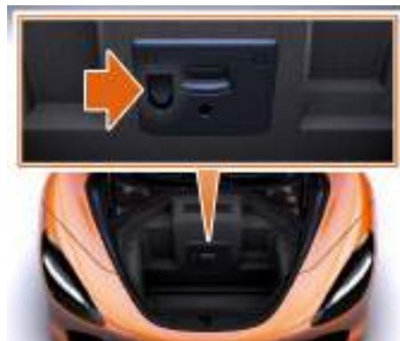
Refer to the instructions supplied with the battery charger. The charger connects to the accessory socket in the luggage compartment.
