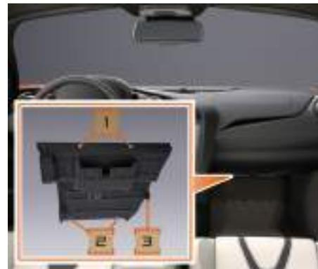
2. Remove the two front screws (1).
