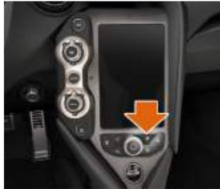
The climate control system is operated using the Central Display. Press the button to switch on the climate control screen.
