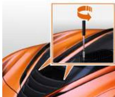
2. Insert the service cover opening tool into each fixing located underneath the lower corners of the service cover. Rotate each fixing 90° counter-clockwise to release both sides of the service cover.
