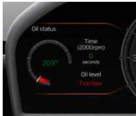
5. If the engine oil is below the target level, top up the oil in accordance with the following procedure.
