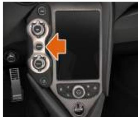
1. Press the ACTIVE button to switch on the Active Dynamics Panel.
