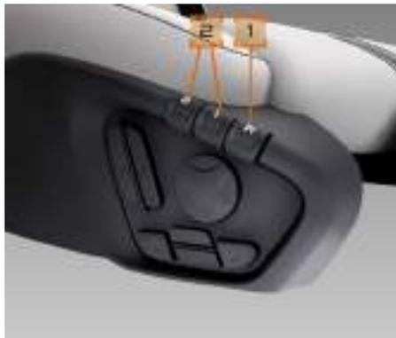
Press the button (2) where the required setting is stored, and hold until the seat, exterior mirrors and steering wheel have completed their adjustment.
