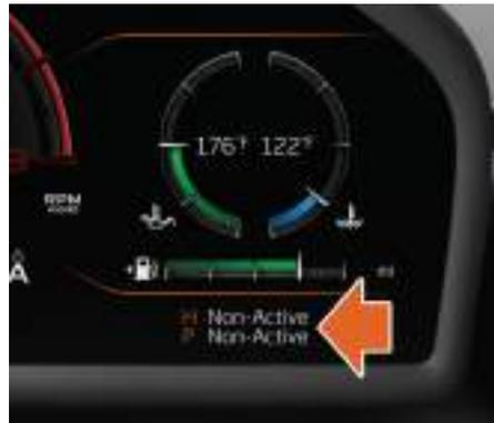
Confirmation that the ACTIVE button has not been pressed (Active Dynamics Panel is off), the handling and powertrain displays will both show Non-Active and will be displayed in white. The mode will not be implemented if all pre-conditions are not met, if the handling and powertrain mode selected is displayed. For more information on the different settings that are available, see Active dynamics control, page 2.22.
