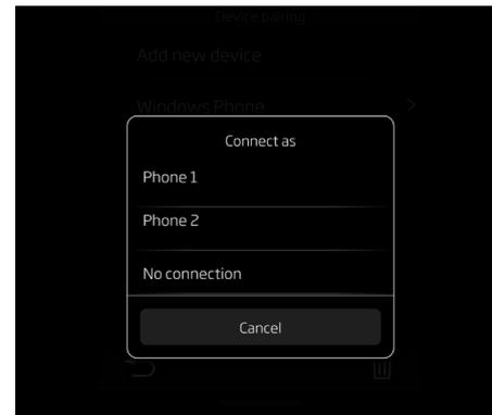
7. Once your phone has paired and connected to the MIS, select whether to connect as **Phone 1** or **Phone 2**. Select **No connection** if the Bluetooth® device is to be used for audio streaming only.
