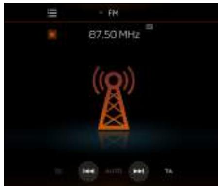
A station can be selected by either manually tuning or selecting a favorite. The frequency will be displayed on the screen along with the station name if available.
