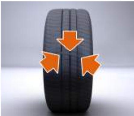
When the tread is worn to 1.6 mm, the wear indicators appear on the surface of the tread pattern, producing a continuous band of rubber across the width of the tire. Tires must be replaced as soon as the wear indicator becomes visible, or sooner if legislation dictates replacement at a greater tread depth.
