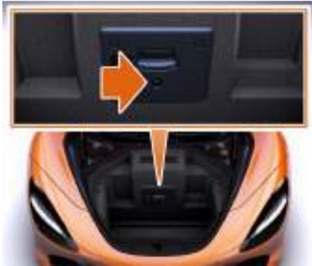
The button is located in the luggage compartment area. The button is illuminated green when the car is awake and flashes green when the vehicle is locked or shut down. This operation is completely independent of ignition state. There are 2 modes to the button:
