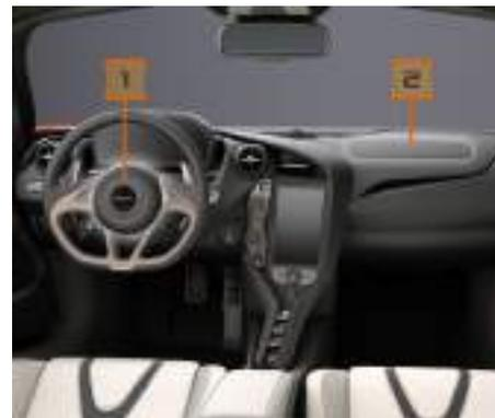
The driver's front air bag (1) deploys in front of the steering wheel and the passenger's front air bag (2) deploys in front of and above the dashboard.
