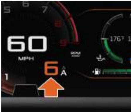
The gear indicator shows the current gear position selected: Neutral, Gear 1-7, or Reverse. The indicator will also show A or M depending on whether automatic or manual mode is selected.
