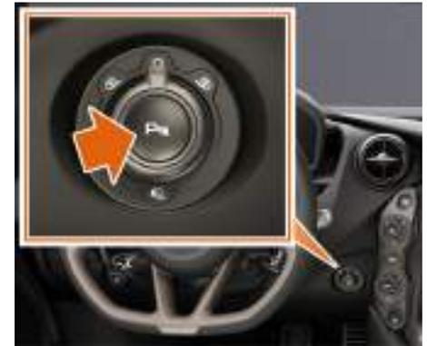
360 Park Assist will display a live video showing a 360 degree view around the vehicle in the Central Display.
