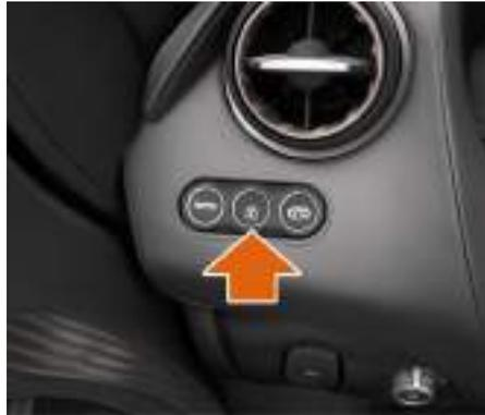
The light in the central locking button will illuminate for approximately 60 seconds after locking the vehicle, the light will continue to flash beyond this time.
