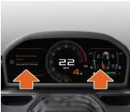
The display shows the pressures of each of the four tires. If the pressure figure appears in green, no action is required. If it appears as red text, inflate the associated tire to the correct pressure as soon as possible.
