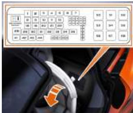
2. Release the two lower clips securing the panel to the bulkhead and remove the panel
