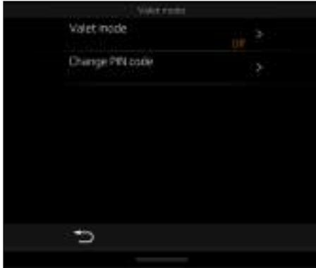
With valet mode on, the speed of the vehicle is limited to 35 mph (55 km/h), the Active Dynamics Panel is disabled, the luggage compartment, center console stowage compartment and service cover remain locked, and a confirmation message appears on the instrument cluster.
