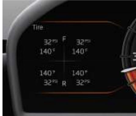
This shows the pressures and temperatures of each of the 4 tires. If the figures appear in white, no action is required. If they appear as amber or red text, have the tires inspected and pressures rectified as soon as possible.
