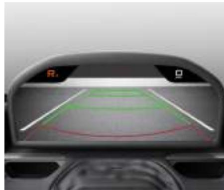
A colored grid is overlaid onto the live video feed as a guide to the proximity of visible objects to the rear of the vehicle.
