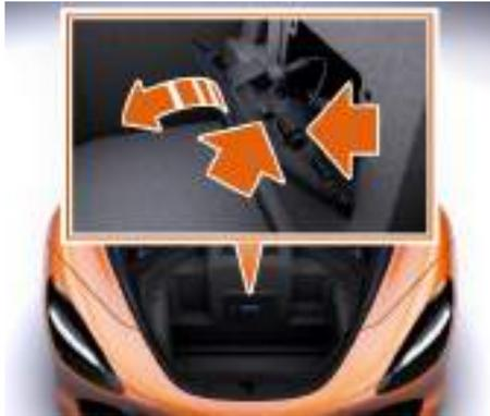
6. Open the top of the battery access cover and disconnect the 2 electrical connectors on the back of the cover.
