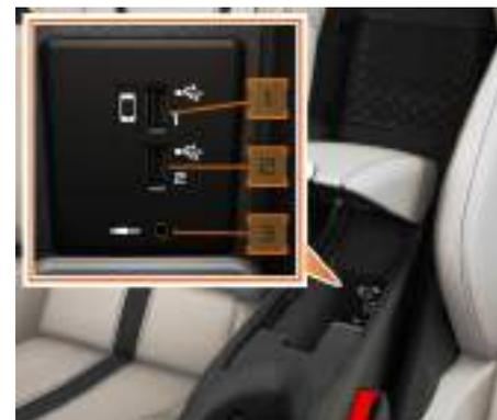
The media USB sockets are located inside the center console stowage compartment.
