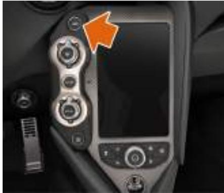
2. Press the **AERO** button. The Airbrake rises and locks in the downforce position.
