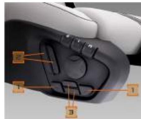
Press the switches (2) until the backrest is in the required position.
