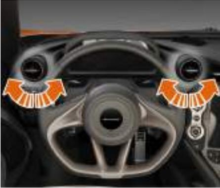
Turn a quarter turn in either direction until the vent is open or closed.
