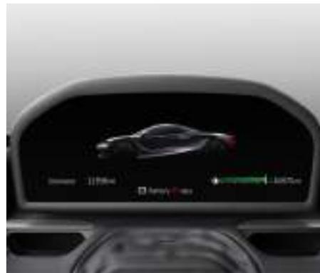
When the vehicle is in Awake mode the number of "days parking" remaining will be displayed on the Driver Display. This indicates how many days the vehicle can be
