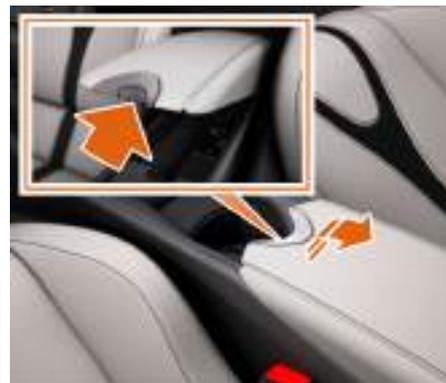
A compartment is fitted in the center console for storing small items.
