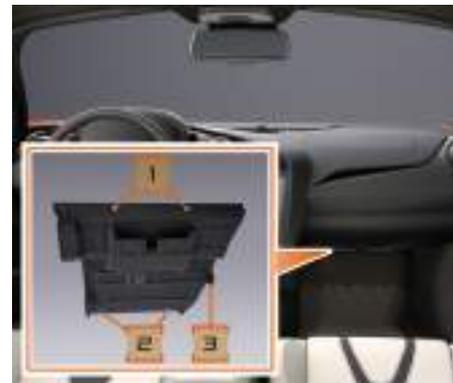
2. Remove the two front screws (1).
