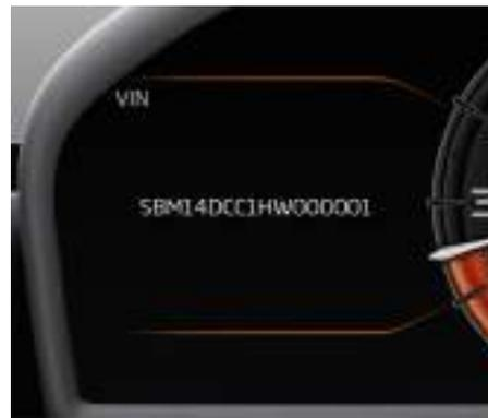
Displays the vehicle identification number (VIN).
