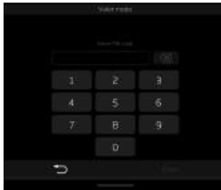
Enter the four digit PIN code using on-screen key pad, then touch **Enter** to confirm. An asterisk replaces each number as it is entered.
