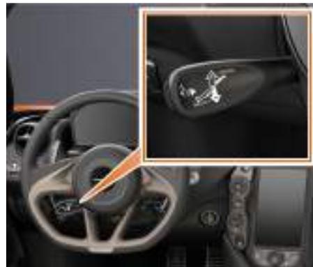
Navigation through the menu structure is achieved using the control stalk mounted on the left of the steering column.
