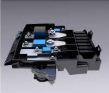
6. Remove the appropriate fuse and replace it with a fuse of the same value as the original. If in doubt, see Battery fuse box fuse specification chart, page 6.22.
