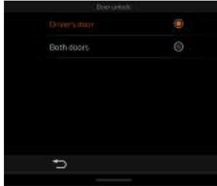
When **Driver's door** is selected, only the driver's door will unlock when the vehicle is unlocked with either the key fob or door button.
