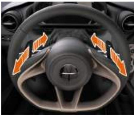
To upshift, pull the right-hand paddle towards you. To downshift pull the left-hand paddle towards you. The current gear position appears on the gear position display, see Gear position indicator, page 3.14.
