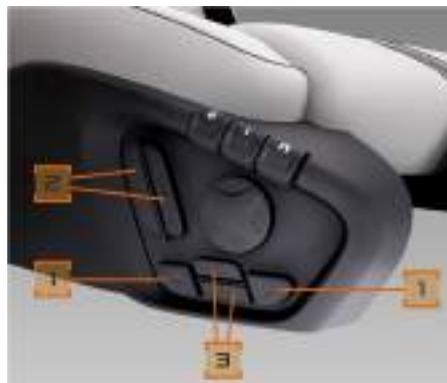
Press the switches (1) until the seat reaches the desired position.
