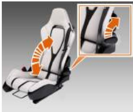
Lift the lever, move the seat backrest to the position required, and release the lever.
