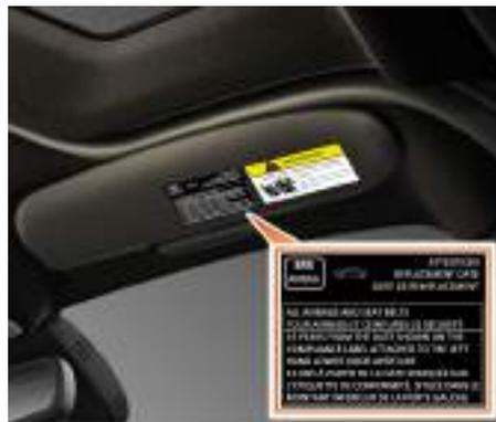
**⚠ WARNING:** McLaren recommend that air bags are replaced every 15 years to prevent air bags from not firing due to component operating life.
