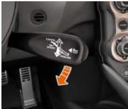
To lower the nose of the vehicle, activate the nose lift menu (see Nose lift operation, page 1.44) and then move the menu control stalk downwards.
