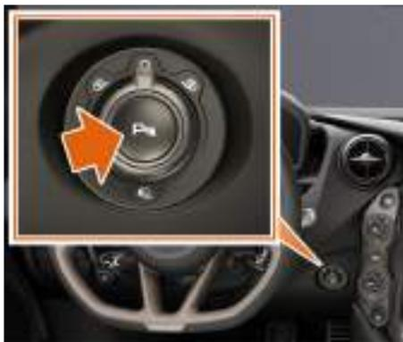
The parking sensors alert the driver to any obstructions while maneuvering at low speeds. The system comprises four ultrasonic sensors in the front bumper, four ultrasonic sensors in the rear bumper and two sounders. Each sounder has a different pitch to indicate whether the obstruction is at the front or the rear of the vehicle.
