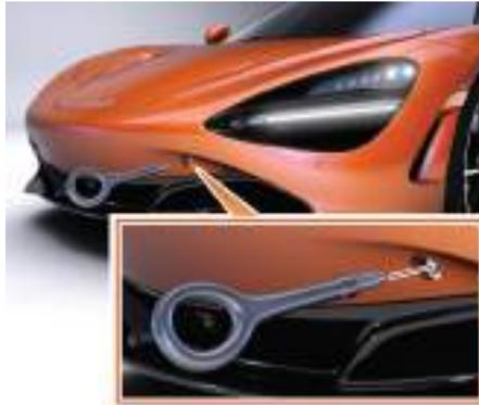
2. Screw the towing eye clockwise into the mounting hole, ensuring that it is screwed in to the full extent of the thread.
