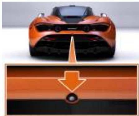
The rear view camera (RVC) is mounted in the center of the rear bumper. The live video feed is displayed on the Driver Display when the function is active.
