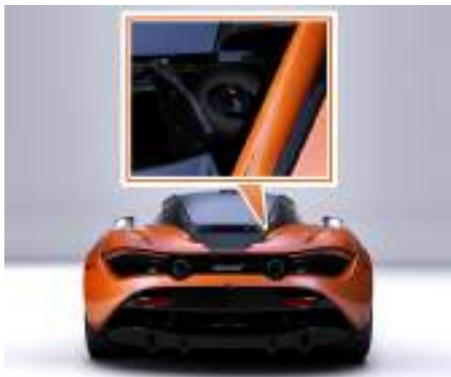
2. Unscrew the engine oil filler cap.
