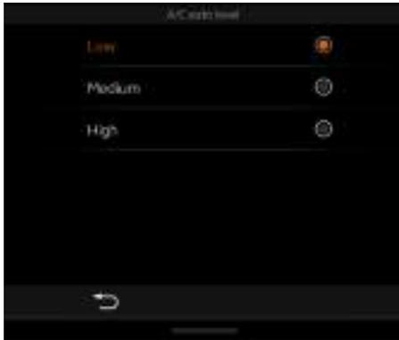
The A/C auto level selected will have an effect on the fan speed used by the climate control system, when in AUTO mode.
