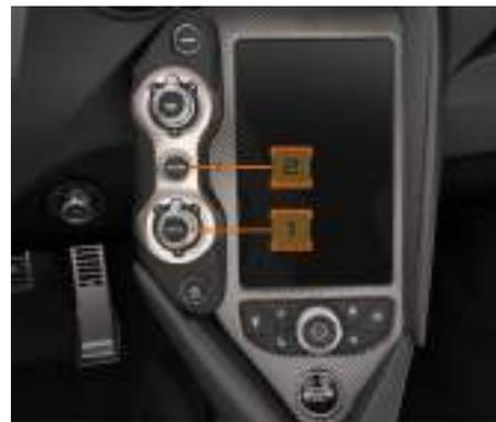
Press the ACTIVE button (1) to switch on the Active Dynamics Panel.
