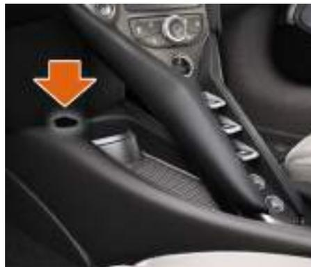
The interior accessory 12 V socket is located adjacent to the front cup holder in the center console and has a maximum load rating of 15 Amps.
