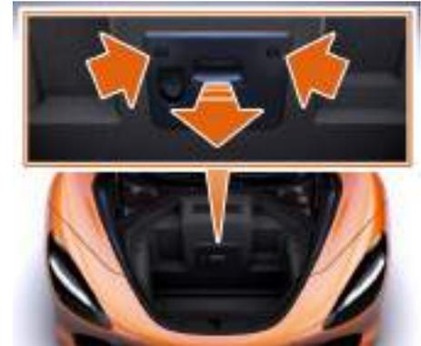
5. Remove the 2 quarter turn screws securing the top of the battery access cover.
