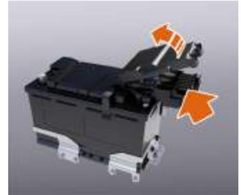
5. Press the 2 catches on the right-hand side of the cover and remove the cover from the fuse box.
