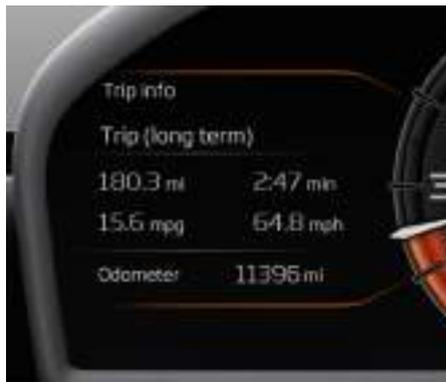
Displays distance, time, average fuel consumption and average speed since the last trip reset.
