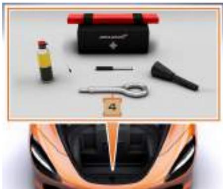
The towing eye (4) is located inside the first aid kit case at the front of the luggage compartment.
