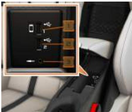
Open the center console and connect the device as required.
