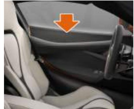
The side head air bags are located in the upper area of each door panel, and are deployed if the system determines they can offer additional protection for the head of the occupant on the side of the vehicle on which the impact occurs.
