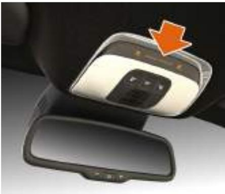
The status of the air bags is indicated by the PASSENGER AIR BAG OFF warning light on the overhead console.
