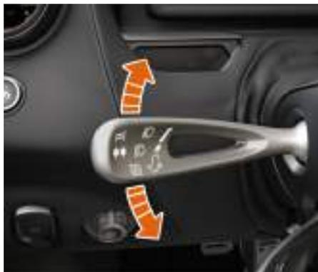
Push the turn signal/hi beam stalk downwards (1) to switch on the left-hand turn signal.
