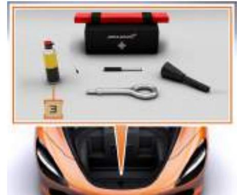
The tire sealant (3) is located at the front of the luggage compartment.
