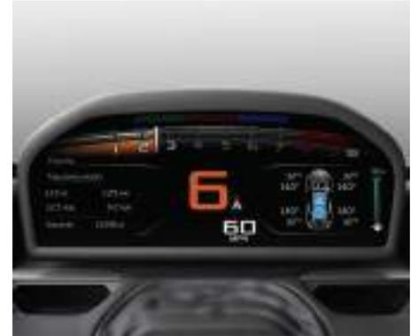
The display window provides the driver with visual access to the control settings and current performance values of the vehicle. The Driver Display, as indicated above, is displayed when the vehicle is in Track mode.
