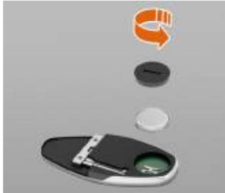
2. Unscrew the battery cover and remove the discharged battery.
