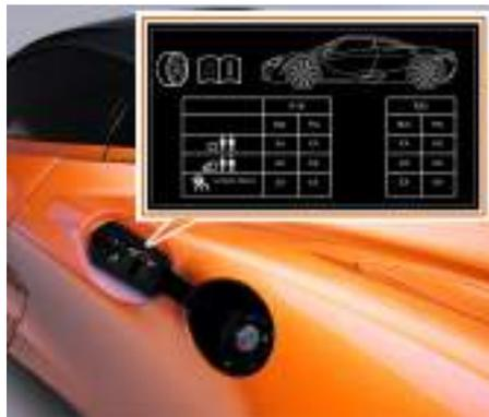
For the tire pressures for various operating conditions, see Tire pressures, page 7.8. They are also printed on a label attached to the fuel filler flap.
