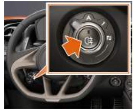
Press the rear fog lamp button in the center of the light switch.
