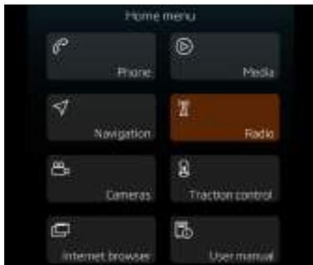
When Radio is selected from the McLaren Infotainment System (MIS) Home screen, or using the Radio button, the radio will launch and tune to the previously selected station.
