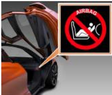
**⚠️ WARNING:** If the PASSENGER AIR BAG OFF indicator does not illuminate, do not use a rearward facing child restraint system on the passenger seat. You may use a forward-facing child restraint system on the passenger's seat. The warning label on the passenger's side is there to remind you of this.
