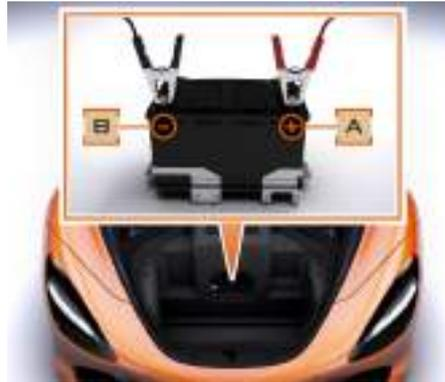
8. Connect one end of the positive (+) booster cable to the positive (+) terminal on the donor vehicle's battery.
