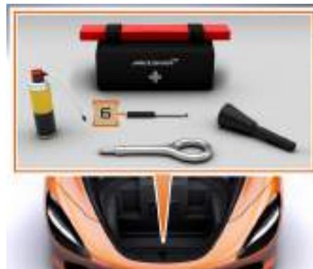
The engine cover release tool (6) is located inside the first aid kit case at the front of the luggage compartment.
