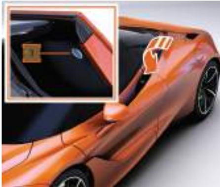
3. If using the keyless entry feature, press the touch sensitive switch (1) located within the side duct.
