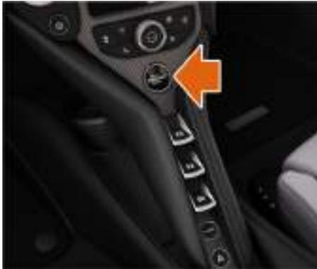
2. Depress the brake pedal, press and release the START/STOP button and the engine will start.
