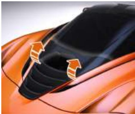
3. From the side of the vehicle, grasp the two rear edges of the service cover and rotate the service cover upwards towards the rear windscreen to remove.
