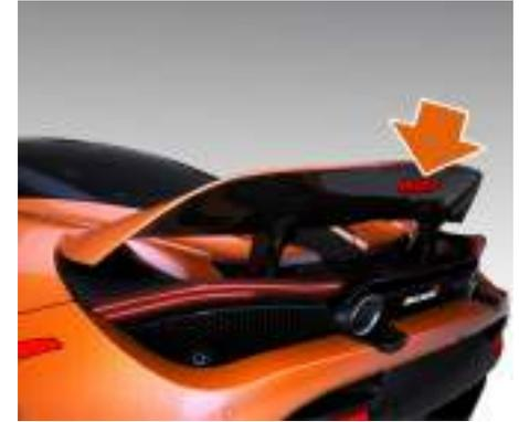
The active central high mounted stop lamp, located in the Airbrake, will illuminate under braking if the Airbrake is deployed as the Airbrake will obscure the static central high mounted stop lamp.
