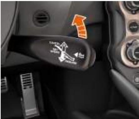
Before nose lift can be activated, the engine must be running. To raise the nose of the vehicle, activate the nose lift menu (see Nose lift operation, page 1.44) and then move the control stalk upwards.
