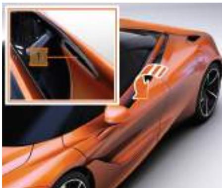
1. Press the button (1) firmly to unlock and unlatch the door.
