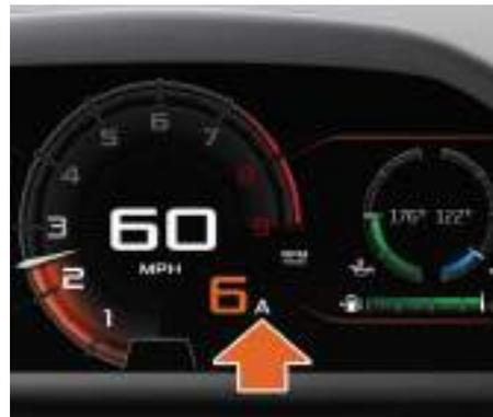
The gearbox mode indicator displays A. All gear changes occur automatically, but if a gearshift paddle is operated the gearbox will adopt a temporary manual mode. This mode will remain active for as long as the driver continues to make manual gear changes, each within an eight second period. The gearbox mode indicator displays A/M, see Gear position indicator, page 3.14.
