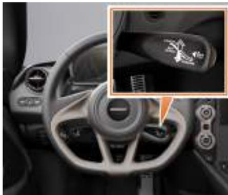
All cruise control functions are operated by the cruise control stalk, positioned on the right of the steering column.
