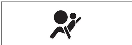
If the "AIR BAG" light on the instrument cluster does not blink or come on when the ignition switch is first turned to the "ON" position, or the "AIR BAG" light stays on, or comes on while driving, the air bag system (or the seat belt pretensioner system) may not work properly. Have the air bag system inspected by an authorized MARUTI SUZUKI dealer as soon as possible.
