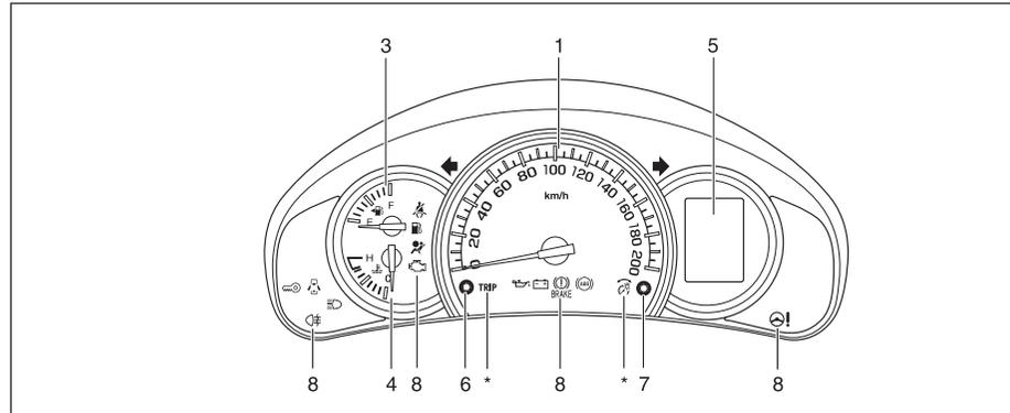
\* These marks are explanation of the knobs 6 and 7. Refer to "Brightness Control" or "Information Display" in this section for detail of knobs.
