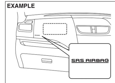
The driver's front air bag is located behind the center pad of the steering wheel and the front passenger's front air bag is located behind the passenger's side of the dashboard. The words "SRS AIRBAG" are molded into the air bag covers to identify the location of the air bags.
